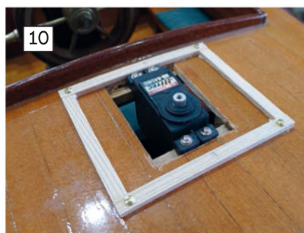
The first stage of the hatch was to make a simple locating frame, screwed to the deck to force the wood to follow the camber.
