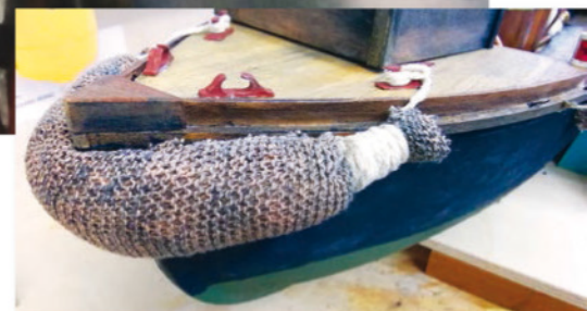
ABOVE: The fenders were made from pre-dyed mutton cloth, simply rolled up and tied off at each end. For dye, John used diluted wood stain.
