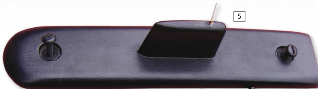
The Spook's hatch seal made from rubber tubing.
