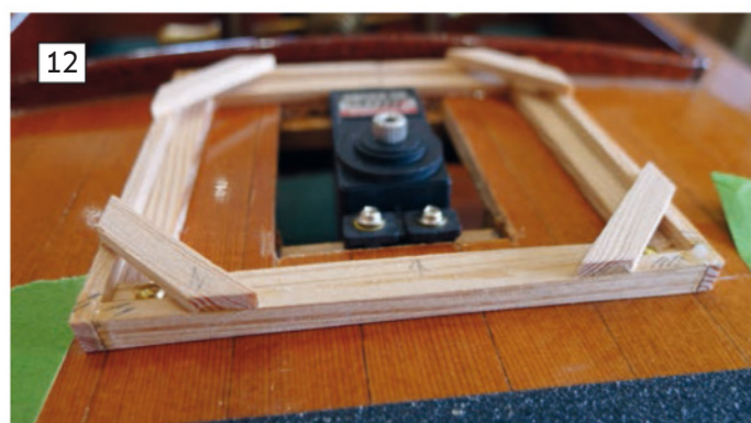
ABOVE LEFT: Around that another frame was made to perfectly fit the inner frame, which could then be removed to have the transverse edges sanded down to fit the camber. The rise of the camber was only around 15mm, which doesn't sound much but which would give a horrible gap at the base of the coaming if not addressed. ABOVE RIGHT: The effort was worth it, as the final frame fit the camber of the deck perfectly, without a gap at any point. BELOW LEFT: When the frame was then built up to full height, with cuts outs included for the servo rods and the outsides clad with mahogany veneer cut to match the shape of the base, it all came together as a nice neatly fitting structure. BELOW RIGHT: The outside frame was varnished and glued down, and a cover made by simply constructing another frame around the top edge, which was then covered with some more deck planking. Painted with a gloss varnish and with all the painted-up linkages fitted, it looks suitably realistic and neat.
