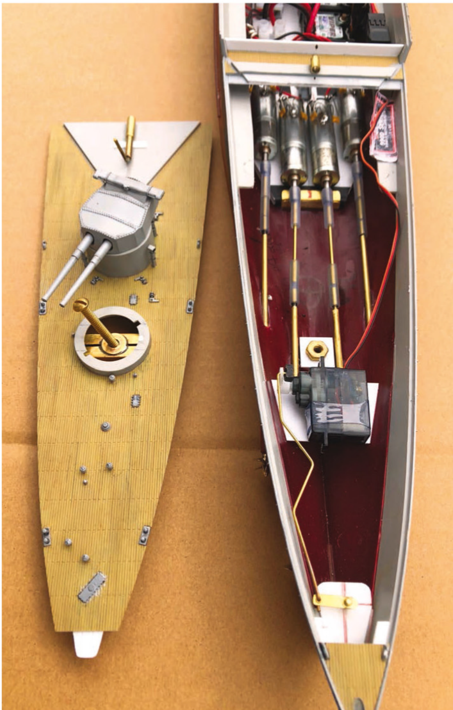
ABOVE: The firmly attachable quarterdeck. This won't wash off. BELOW: The four motors are glued to a small plate that can be easily removed if necessary.
