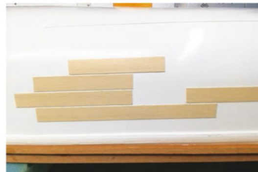
ABOVE: The fibreglass outer hull in its original pristine condition required 'spoiling', and John felt he was just the man for that job! Patches of self-adhesive Formica surface edging were added to create the impression of repairs.
