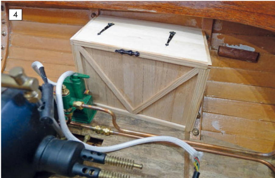
LEFT: The outside framework is purely decorative, but the lower frame piece of the inboard face is actually glued to the deck not the locker, so it acts as a secure locating part.
