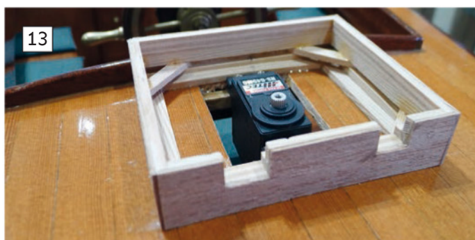
ABOVE LEFT: Around that another frame was made to perfectly fit the inner frame, which could then be removed to have the transverse edges sanded down to fit the camber. The rise of the camber was only around 15mm, which doesn't sound much but which would give a horrible gap at the base of the coaming if not addressed. ABOVE RIGHT: The effort was worth it, as the final frame fit the camber of the deck perfectly, without a gap at any point. BELOW LEFT: When the frame was then built up to full height, with cuts outs included for the servo rods and the outsides clad with mahogany veneer cut to match the shape of the base, it all came together as a nice neatly fitting structure. BELOW RIGHT: The outside frame was varnished and glued down, and a cover made by simply constructing another frame around the top edge, which was then covered with some more deck planking. Painted with a gloss varnish and with all the painted-up linkages fitted, it looks suitably realistic and neat.
