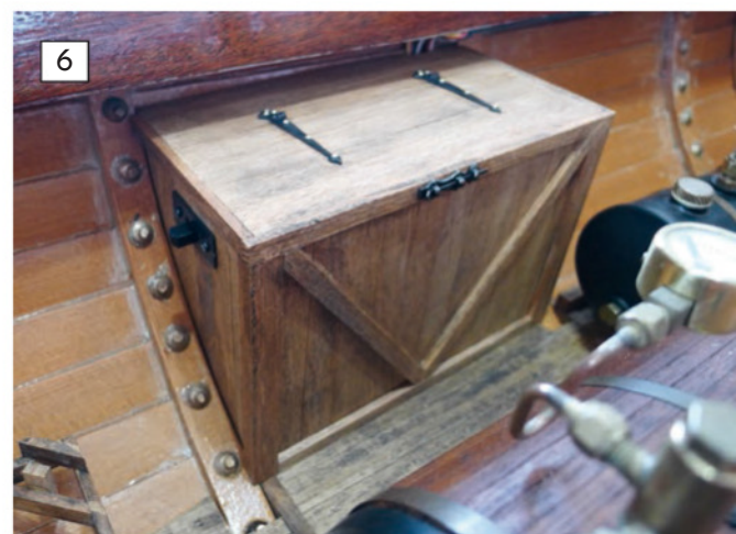
ABOVE LEFT: Both lockers in place in the hull. These neatly sit between the frames but are easily removable, while at the same time provide a reasonable volume of interior space in which to hide the electronics. Worth noting is the water control valve on the port side, the gas regulating valve on the starboard side and the gas tank frame on the starboard side. ABOVE RIGHT: To help blend the lockers in with the internal fittings, they were given the same colour wash as was used on the main deck planks. To protect and seal them, two coats of matt polyurethane varnish was then added.
