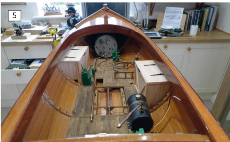
ABOVE LEFT: Both lockers in place in the hull. These neatly sit between the frames but are easily removable, while at the same time provide a reasonable volume of interior space in which to hide the electronics. Worth noting is the water control valve on the port side, the gas regulating valve on the starboard side and the gas tank frame on the starboard side. ABOVE RIGHT: To help blend the lockers in with the internal fittings, they were given the same colour wash as was used on the main deck planks. To protect and seal them, two coats of matt polyurethane varnish was then added.
