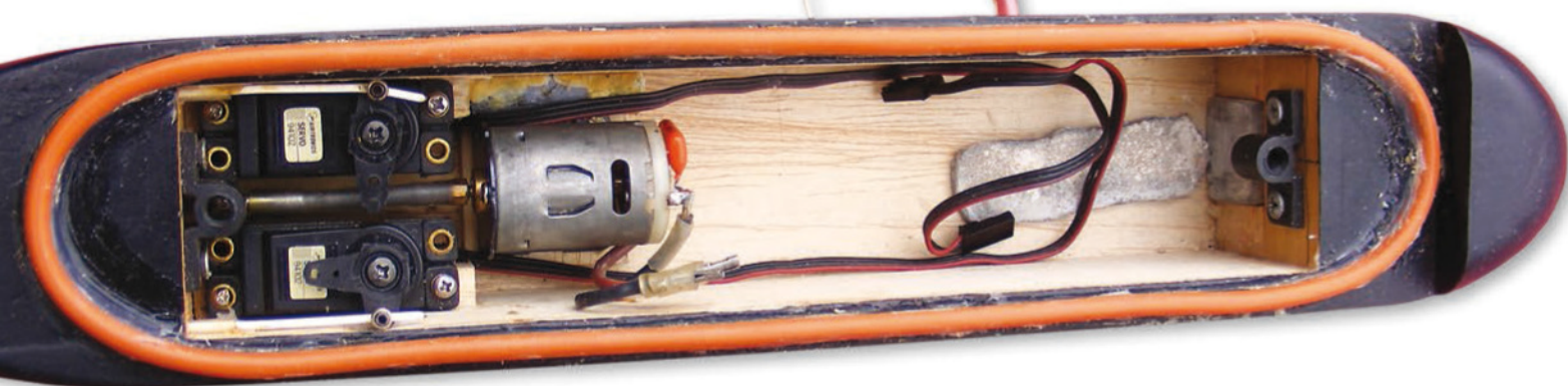
The Spook's hatch seal made from rubber tubing.
