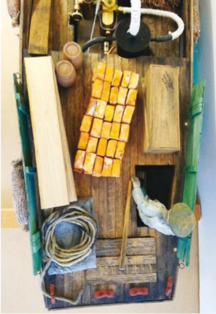
ABOVE LEFT: The rear deck, with various pieces of cargo covering the controls. The bricks were handmade from DAS modelling clay, then air dried and stuck around a cardboard box, which covers the oil feed water top and charging point. ABOVE RIGHT: The bow of the lighter. The two boxes cover the top of the gas tank and gas control valve.
