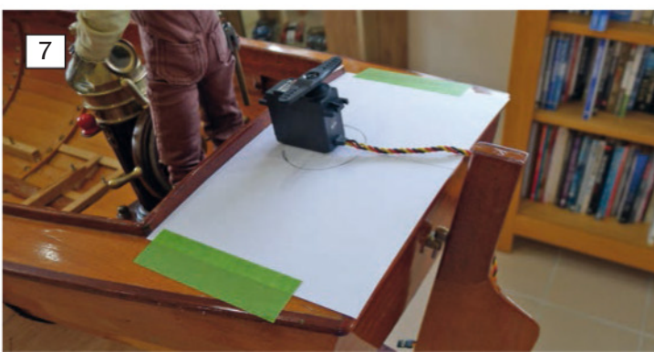
BELOW LEFT: Using a paper template makes it easy to see just where the linkages are going to end up and will give you a good idea of the limits of movement. It's a lot easier to play around at this stage than it is when cutting up bits of wood and metal. BELOW RIGHT: The Hi-Torque servo in place in the hole in the deck and all temporarily connected up with the two operating linkages. Good movement was achieved on the rudder with this set up, which is going to be needed with such a long model.
