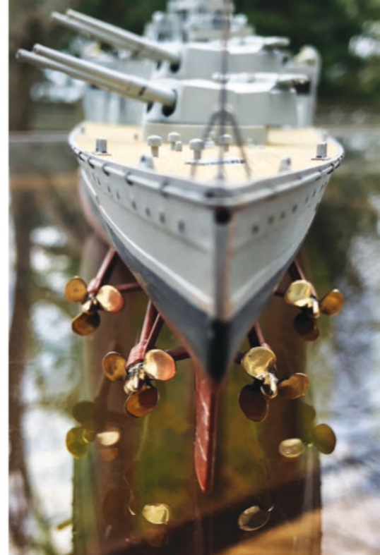
ABOVE: The four bronze Prop Shop ½-inch Standard Scale props, turning 'outwards', of course.
