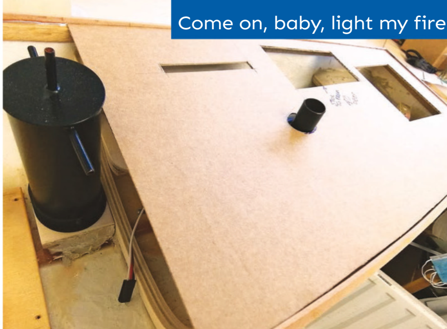
ABOVE: A card template was made to ensure the correct location of the apertures in the rear deck; these are for the water tank filler, the steering servo, cockpit, and a slot for the manual water pump handle. The tank on the left is the condenser tank.
