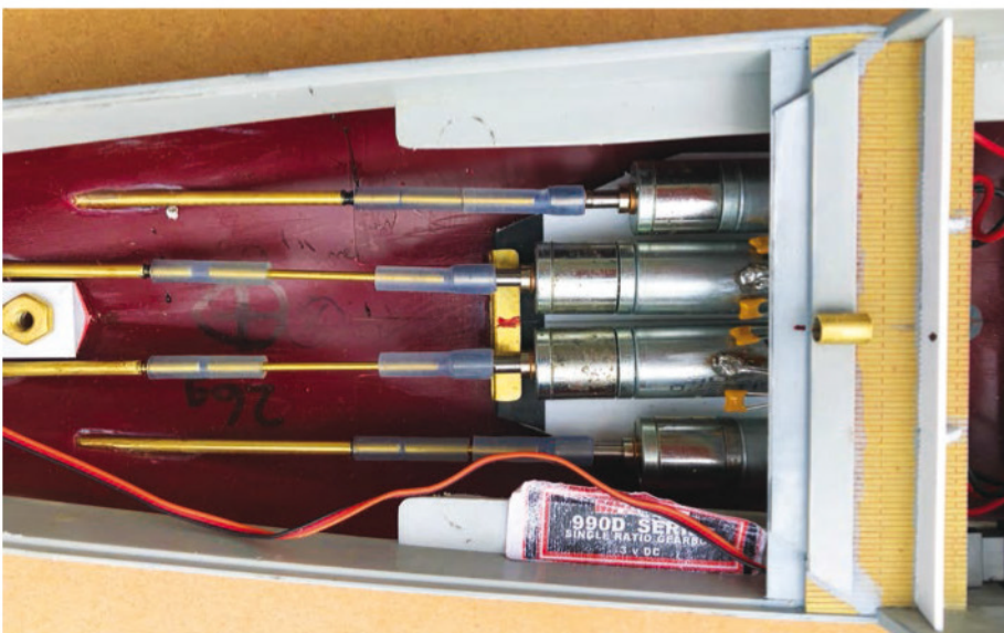
ABOVE: The firmly attachable quarterdeck. This won't wash off. BELOW: The four motors are glued to a small plate that can be easily removed if necessary.
