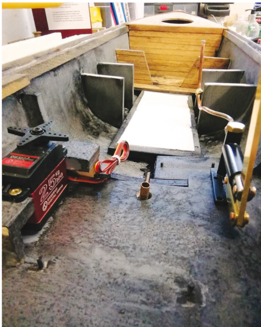
ABOVE: Planking has been added to the foredeck and coal bunker area. At this stage, the locations for the boiler, etc, were checked. BELOW: The inside of the hull. The white pad in the centre is thin insulation material. Not necessary, John points out, but he had some kicking around so thought he would use it.
