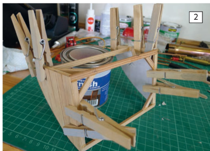
ABOVE LEFT: Once the glue has set on the frame it's strong enough to be removed and worked on as a much more convenient separate item. Here you can see how the sides, which have been cut from a paper template taken from the hull, have been clad with more planking. ABOVE RIGHT: The inboard face has also been clad in this planking to create a very neat locker that fits the hull perfectly and looks as if it is built in.
