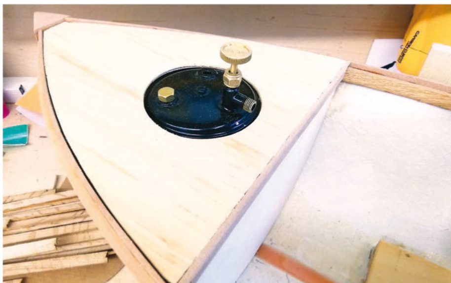
ABOVE: The gas tank is located in the bow /foredeck. John's concern was that, as a permanent location, the gap between the tank and the foredeck needed to be well sealed with silicone sealer to prevent gas, when filling the tank, from seeping into the cavity under the deck. BELOW: Servos for the steering and steam regulator in place. The inner hull has been brush painted using Halford's grey primer.
