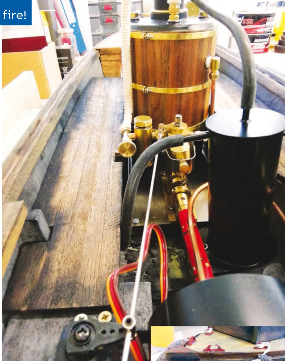
ABOVE: The coal bunker at the bow of the lighter. RIGHT: The Clevedon Steam boiler and engine fitted. This still looks rather new, as here John, points out, his courage failed!
