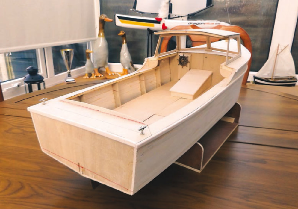
ABOVE: A transom view, with mooring cleats installed.
