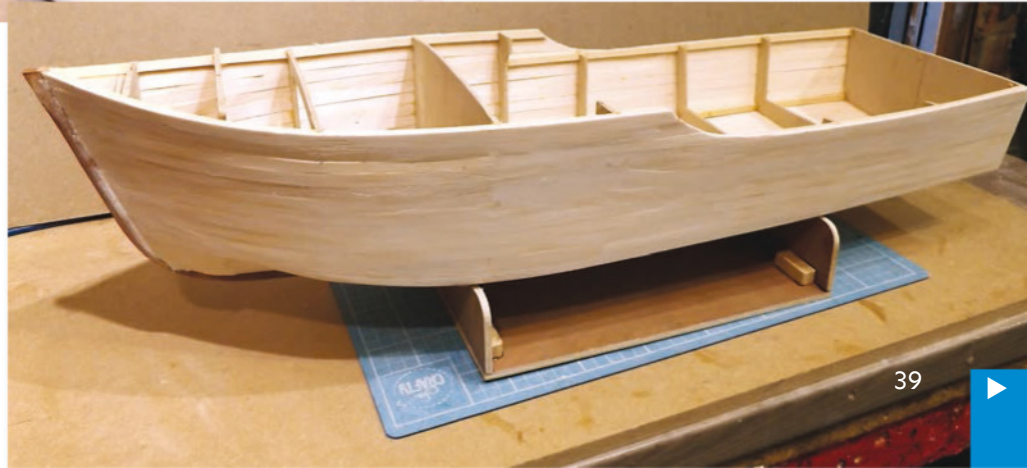
ABOVE: Keel and bulkheads mounted on the building board.
