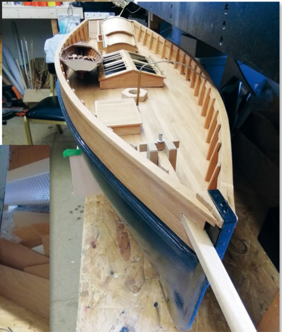
ABOVE: The exterior of the fiberglass hull was brush painted using Phoenix enamel paint. While appearing black, the colour is actually a mix of black and white, giving a dark grey finish.
