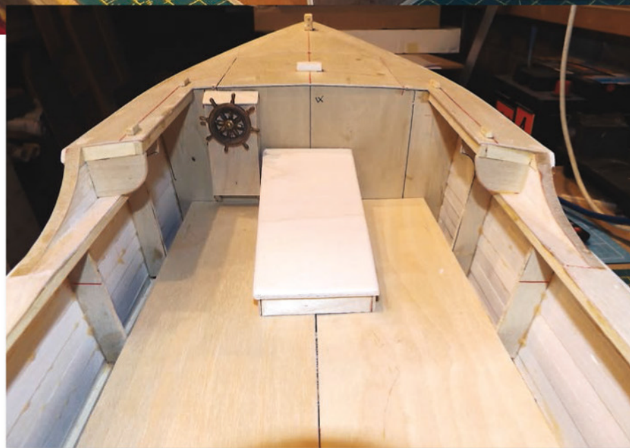
ABOVE: The cockpit floor and engine/motor cover. BELOW: The rudder servo and linkage installation under the rear deck.
