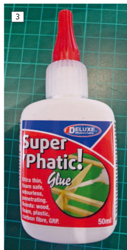
Aliphatic glues share properties similar to those found in PVAs, but they're very thin and particularly good at soaking into close fitted joints by capillary action, while at the same time maintaining their strength.
