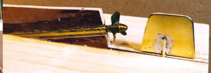
LEFT: The keel shaped and partly cut, ready for the stern tube and doublers to be glued.
