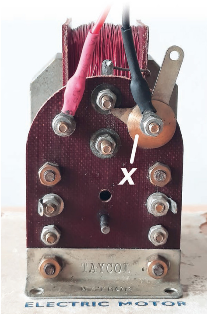
ABOVE LEFT: Meteor, Asteroid – remove switch lever ‘X’. ABOVE RIGHT: Meteor, Asteroid – reversing diodes fitted. BELOW LEFT: Standard – reversing diodes fitted.
