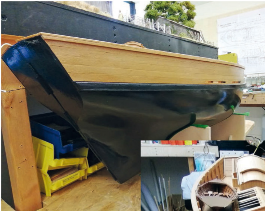
ABOVE: The exterior of the fiberglass hull was brush painted using Phoenix enamel paint. While appearing black, the colour is actually a mix of black and white, giving a dark grey finish.
