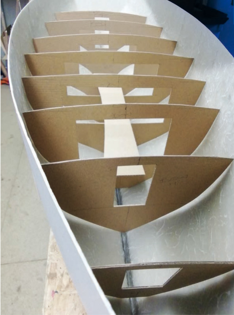
ABOVE LEFT: The finished card templates located in the hull. ABOVE RIGHT: Using the card templates, plywood versions of the bulkheads were cut out and fitted.
