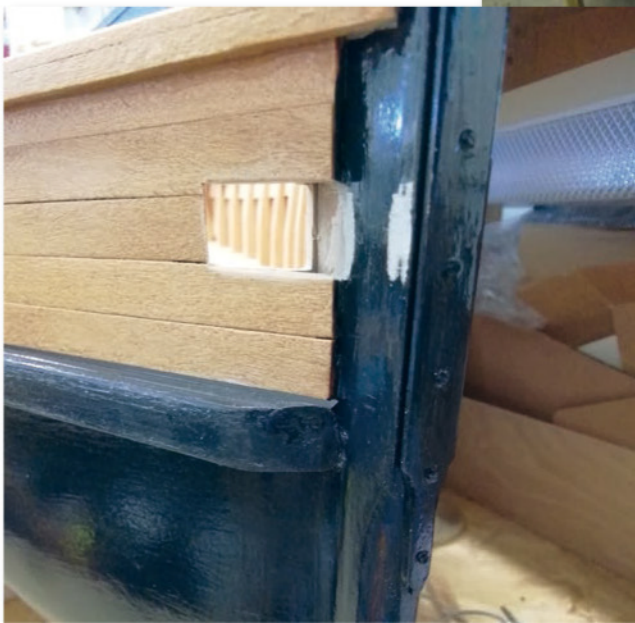
INSET BELOW: John forgot to cut a hole in the bulkhead to allow the bowsprit to come through, which looked a bit ragged to start with. RIGHT: The bowsprit in place.
