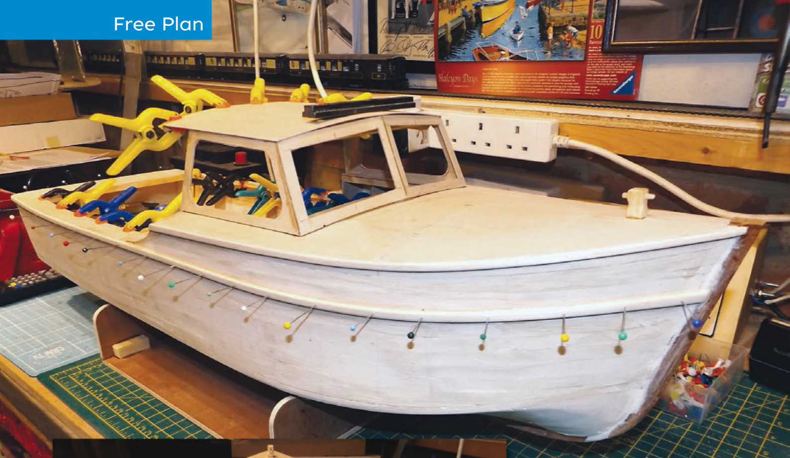
ABOVE: The hull complete, with rubbing strips attached and cabin in place.
