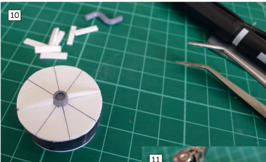
ABOVE: Discs of polystyrene sheet were added to both sides, and stiffeners made out of cut up plastic strip were added around a plastic pipe fitting looted from a model railway pipe set.
