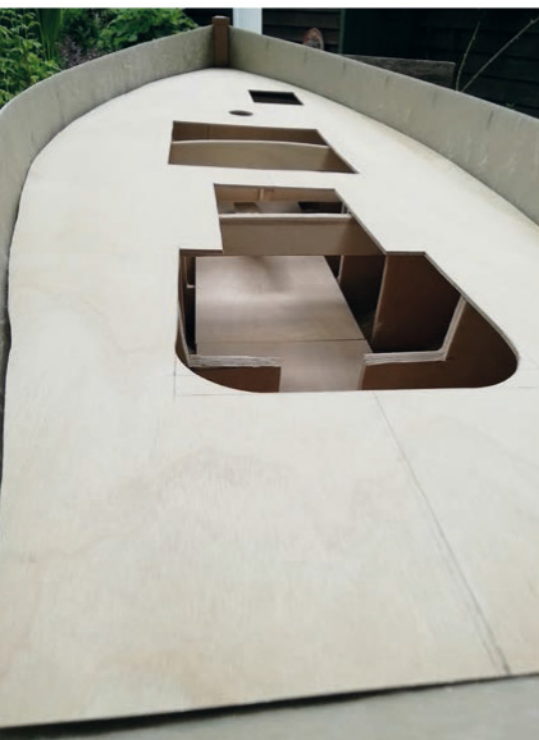
ABOVE LEFT: The plywood deck being tried on to ensure a reasonable fit. BELOW LEFT: The steering servo was fitted with a long vertical arm, which was to locate in the long slot in the tiller arm. BELOW RIGHT: The arrangement of the guide tubes to lead the sheets from below the deck up to the sails.
