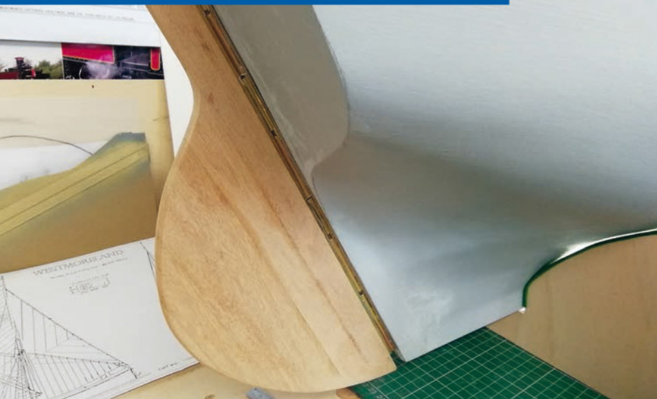
ABOVE LEFT: The teak rudder attached to the transom with a homemade hinge. ABOVE RIGHT: The sail servo in place. This serves both the main and foresails.
