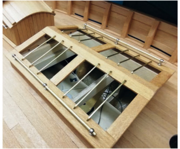
ABOVE LEFT: The cockpit and companionway were clad in teak. The arc slot in the floor of the cockpit is to allow the vertical servo arm to operate.
