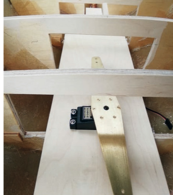
ABOVE LEFT: The teak rudder attached to the transom with a homemade hinge. ABOVE RIGHT: The sail servo in place. This serves both the main and foresails.
