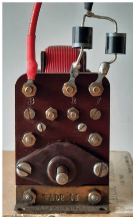
ABOVE LEFT: Meteor, Asteroid – remove switch lever ‘X’. ABOVE RIGHT: Meteor, Asteroid – reversing diodes fitted. BELOW LEFT: Standard – reversing diodes fitted.
