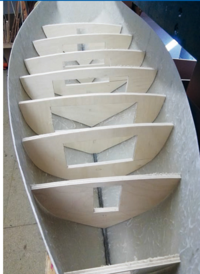
ABOVE LEFT: The finished card templates located in the hull. ABOVE RIGHT: Using the card templates, plywood versions of the bulkheads were cut out and fitted.
