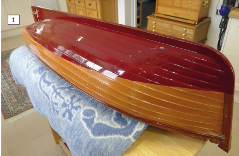
ABOVE: A lot of care and attention is required to mask a waterline on a clinker-built hull. Get it right, however, and it looks simply superb and greatly enhances the overall look of the model. BELOW: Richard has never before used an enamel paint that goes on as satisfyingly as the one he selected for this project from the Craftmaster Paint range. The brush, he explains, seems to glide over the surface of the hull and the paint settles to a beautiful full gloss shine.
