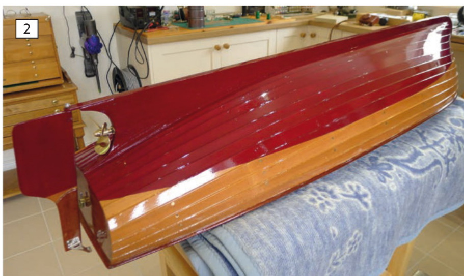
ABOVE: A lot of care and attention is required to mask a waterline on a clinker-built hull. Get it right, however, and it looks simply superb and greatly enhances the overall look of the model. BELOW: Richard has never before used an enamel paint that goes on as satisfyingly as the one he selected for this project from the Craftmaster Paint range. The brush, he explains, seems to glide over the surface of the hull and the paint settles to a beautiful full gloss shine.
