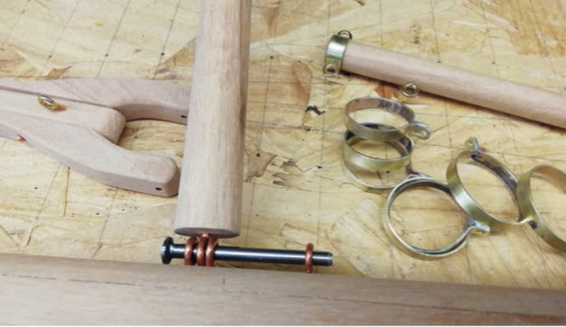
ABOVE: Having carved the mast and boom, etc, from solid teak, this photo shows a variety of the mast fittings.
