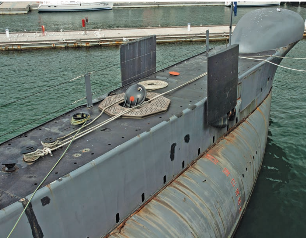
ABOVE: Bow section with post-SWUP sonar dome. BELOW LEFT: Forward torpedo tubes. BELOW RIGHT: Engine room, looking aft.
