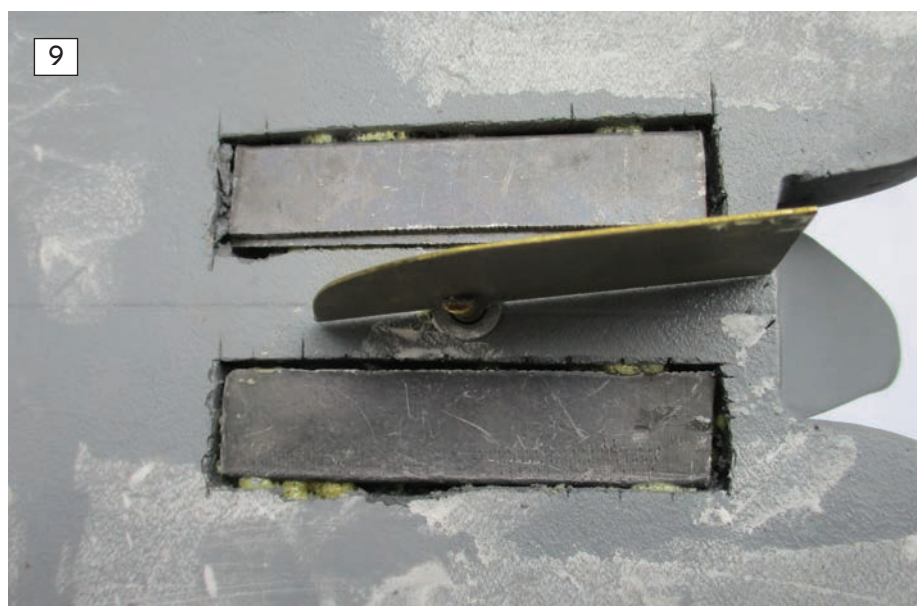
40-gram lead weights inset into the foam underside to the rear. A bias weight has been inset further forward.
