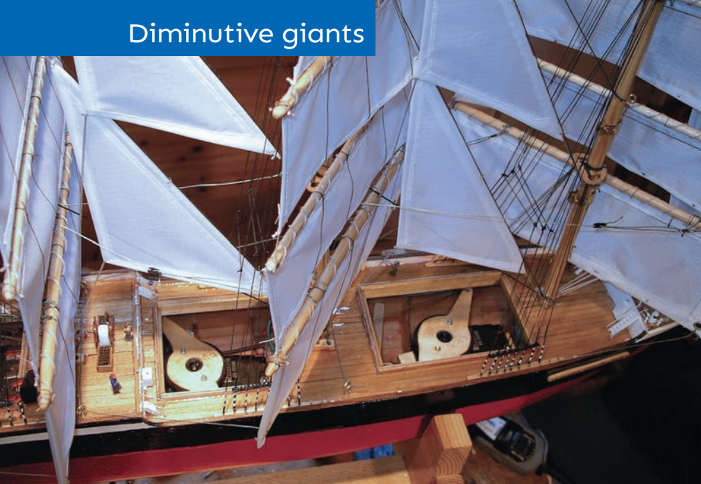
The insides of Nev's model of Potosi, after the retro-fit of HiTec sail arms. The one on the right controls the foremast yards, the one on the left, those on the main mast (in the centre of the picture). The sails on the left are those of the middle (third) mast.
