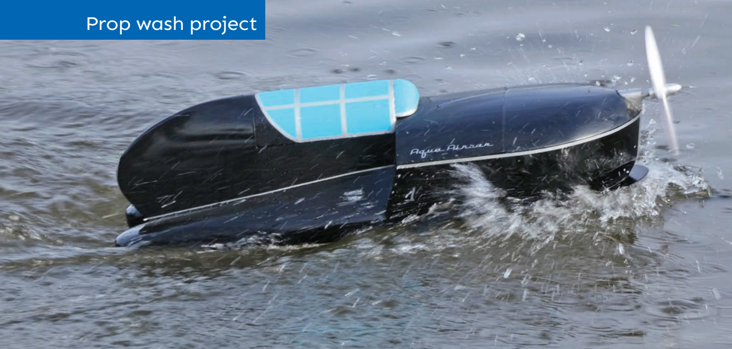
ABOVE: As fast as the Aircar goes note the bow wave below the shelf. The spray is due to prop wash blowing on the bow wave. BELOW: Note how at slow speed, the board sits on the water in the exact same way as evidenced in the full speed shot (above).
