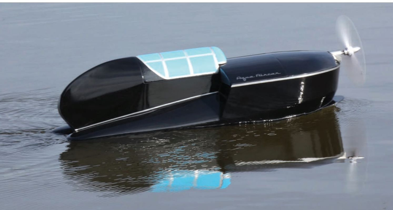
ABOVE: As fast as the Aircar goes note the bow wave below the shelf. The spray is due to prop wash blowing on the bow wave. BELOW: Note how at slow speed, the board sits on the water in the exact same way as evidenced in the full speed shot (above).
