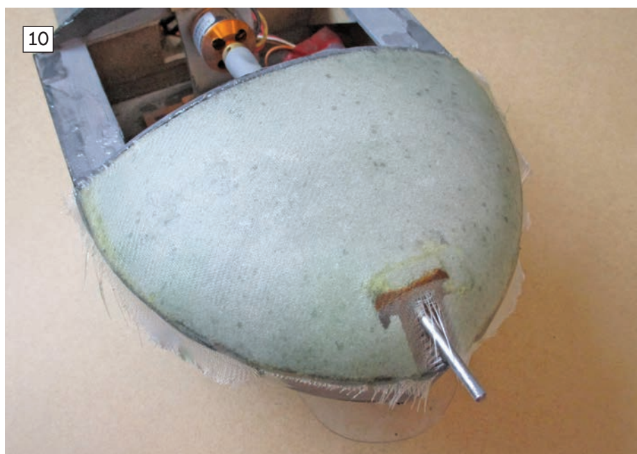
The new foam top coated with glass fibre and resin epoxy. A single curved hatch covers the aft section over the motor.
