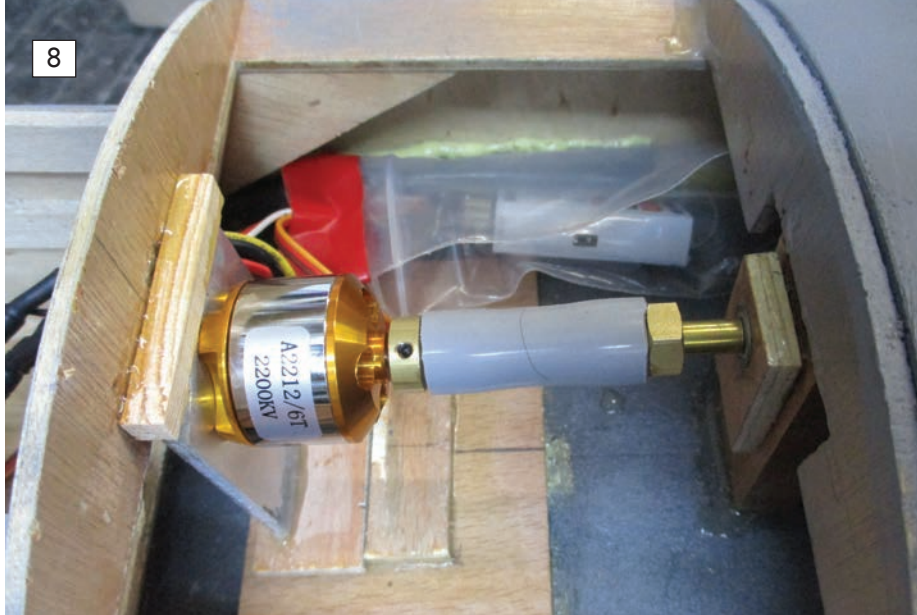
The small outrunner that replaced the original motor, along with ESC, waterproofed receiver protected yet further by a plastic bag and extra thrust bearing (to the right).
