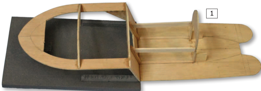
The basic frame and foam lower bow section. The battery will be fitted in the aft section with the rudder, servo, ESC, etc.
