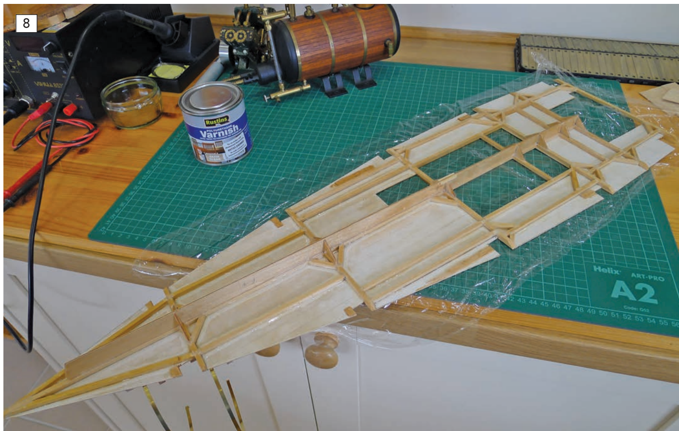
To completely seal the undersides of the deck after construction was finished, it was given two liberal coats of polyurethane varnish. In this view, it's easy to see the transverse beams that locate alongside the hull frames, the longitudinals, including the main beam that sits on the keel, and the braces to keep everything rigid.
