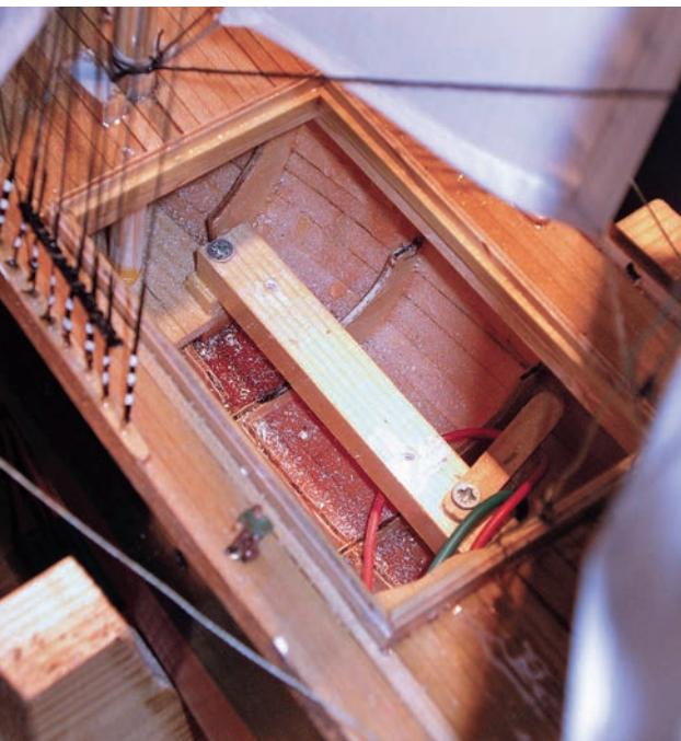
LEFT: The original mounting point for one of the high torque servos. ABOVE: A similar mounting point, after being cut away, to allow fitting of a HiTec sail arm. The amount of destruction is painfully obvious, as is the lack of access!
