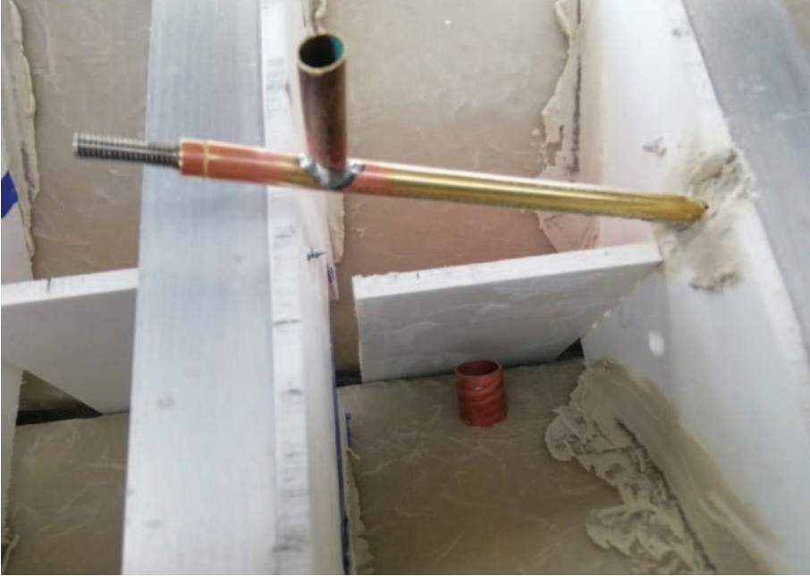
ABOVE LEFT: Looking into the hull, the propellor shaft was bonded in and six small lengths of 15mm central heating copper pipe located along the keel. These would allow water to enter and exit the hold. ABOVE RIGHT: The first bath test. A lot more baffles have been added, plus some lead. This was required to stabilise the hull and prevent it turning turtle.
