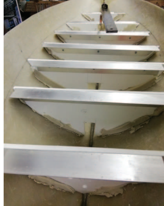
ABOVE: To convert the hold into a 'water tank' plastic was used for the bulkheads and deck. Aluminium angle was used to give additional rigidity and allow the deck to be screwed to the bulkheads. BELOW: With all the bulkheads in place it was important to ensure water could pass along the length of the boat. Holes and slots were cut in the plastic bulkheads.
