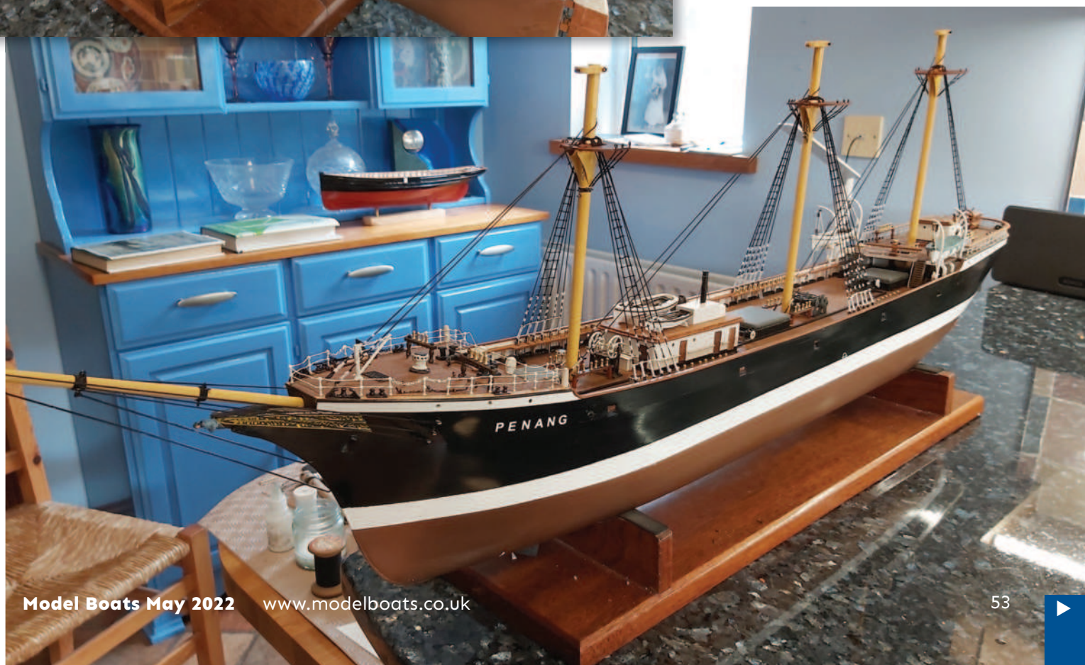
BELOW: All lower mast standing rigging complete.
