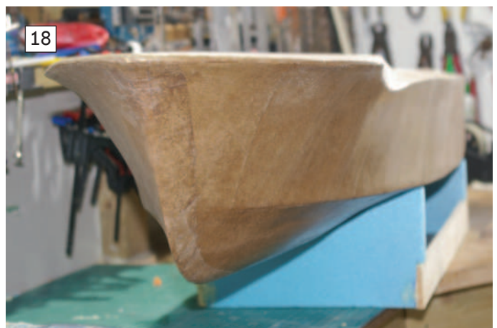
ABOVE LEFT: Getting started on the brown paper wallpapering. If attempting this yourself, use waterproof PVA glue, not the non-waterproof glue I used, Michael points out! ABOVE RIGHT: Small pieces of brown paper were cut and glued at the composite curves. Once dry, any remaining wrinkles can be lightly sanded with fine sandpaper. The stand seen here was formed from a couple of Styrofoam templates originally used to check the shape of the hull.
