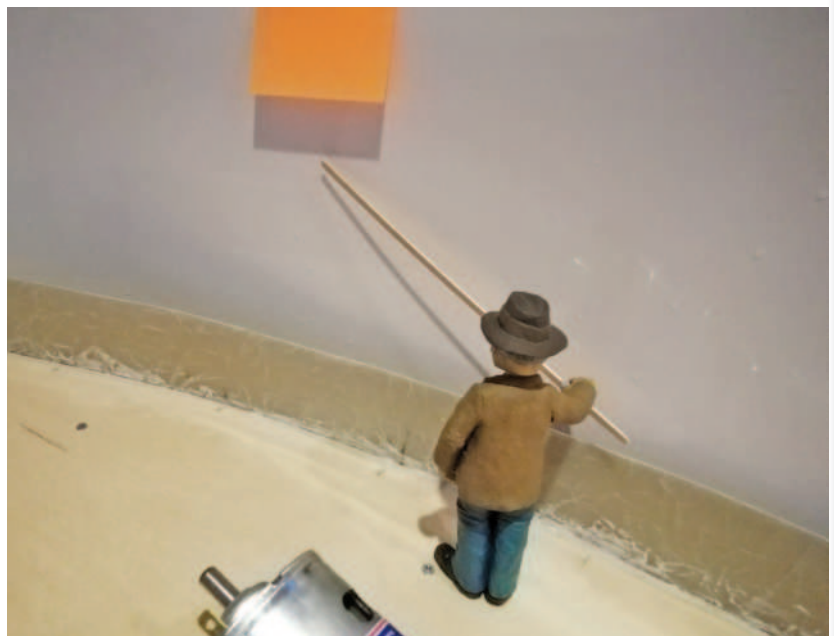
BELOW LEFT: The next bath test. 'George' is indicating the starting point of the test, prior to the exhaust valve being opened. BELOW RIGHT: Here we see the amount the vessel has 'sunk', about 30 mm. This can of course be adjusted by the amount of water allowed into the hold. John's test proved the principle does work.
