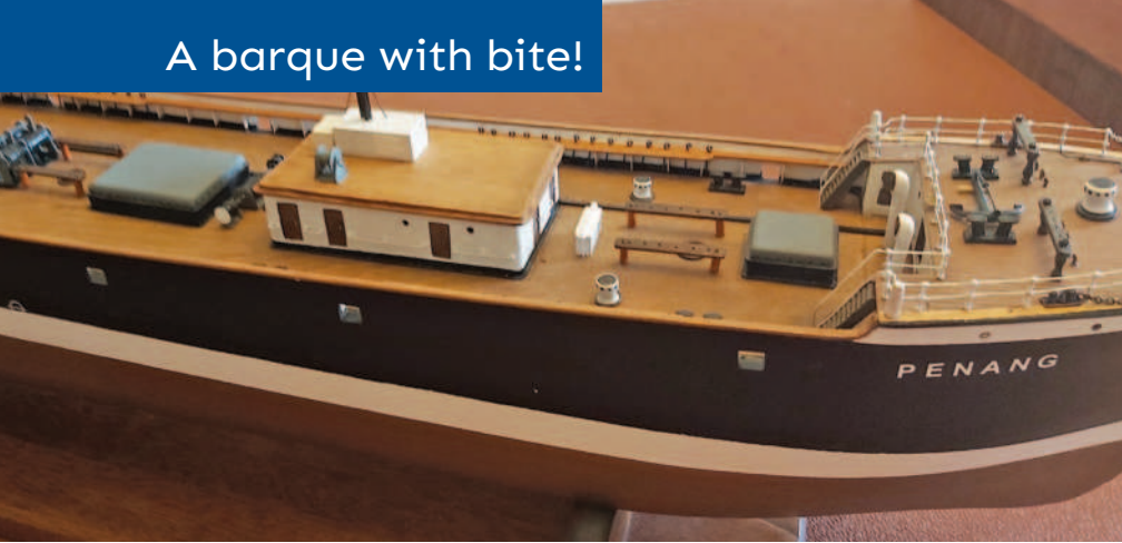
ABOVE: Fore end detail: the donkey boiler is located in the deckhouse. BELOW: The masts, spars and boats ready for finishing.
