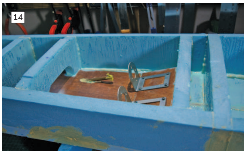
ABOVE LEFT: Inevitably a couple of skims of wood filler are needed to smooth the surface irregularities. ABOVE RIGHT: The engine mounts and prop shafts installed, with the battery tunnel visible. The hull sides aft of the bow section are almost flat so need minimal shaping.
