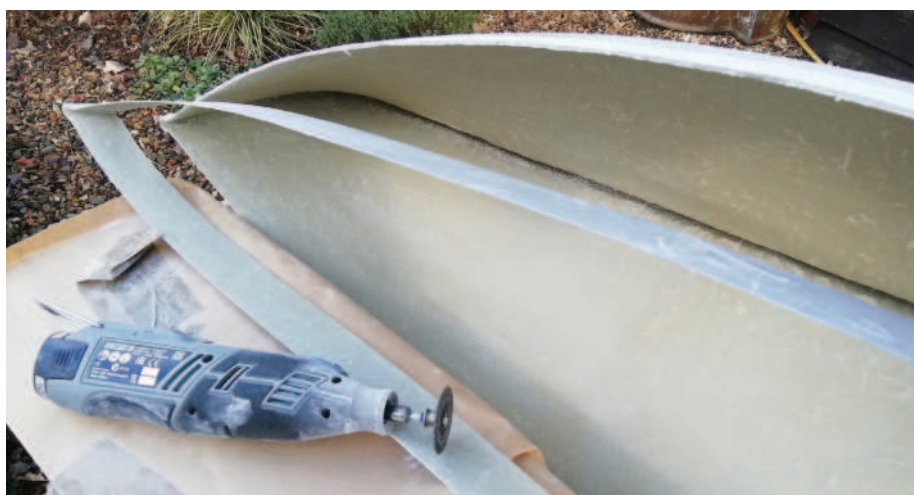
ABOVE: To make the 'Katie' hull look anything like that of the Soleil D'or, great lumps of fibreglass had to be hacked off using a Dremel and cutting disc.
