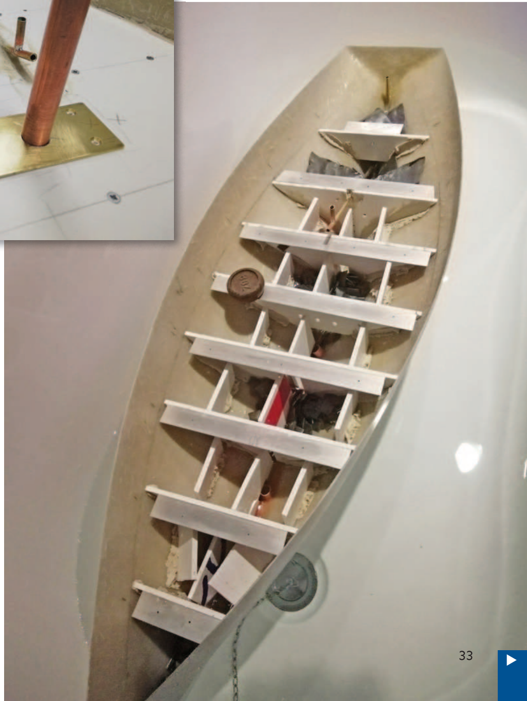
BELOW: To allow the last vestiges of water to escape, a 6mm diameter short length of brass tube was fitted as low as possible along the keel line.
