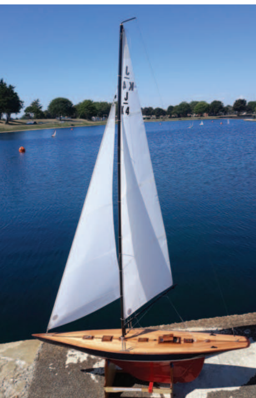
BELOW: The Nottingham 'J' is a representation of Endeavour, as built in 1934. She measures 48 inches in overall length and features twin sail winches for the Genoa and the main sails.
