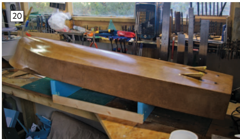
ABOVE LEFT: Wallpapering finished. Michael added a frame around the edge of the engine and rudder bays, which are slightly proud of the deck. As the deck is cambered, this enables a snug, watertight fit for the hatches. Michael's frame was cut from an old venetian blind. If you look carefully, you can see glorious Devon sunshine through his workshop windows! ABOVE RIGHT: The gleaming hull after five, slightly thinned, coats of PVA glue. Wait for each one to dry before applying the next.
