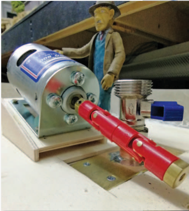
ABOVE: The electric motor set (hopefully!) at correct angle. To compensate for misalignment, a double universal joint has been used.
