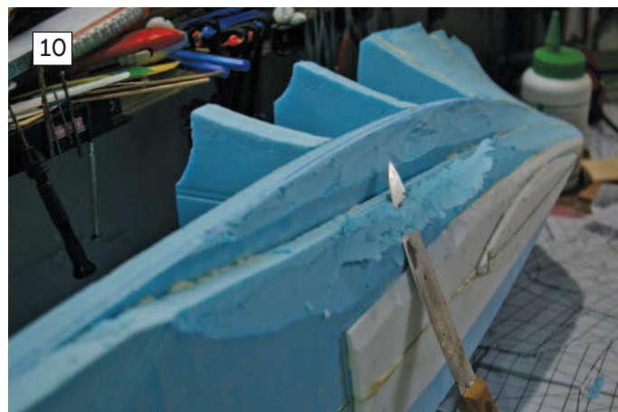
ABOVE LEFT: The roughly cut solid foam bow section with the distinctive 'gooseneck' taking shape. The forefoot needs to be sharp where it cuts through the water and the bow then flares and expands towards the deck, which gives buoyancy when it meets an oncoming wave. ABOVE RIGHT: The fun bit! Whittling the foam to shape with Michael's curved carving knife. Note the pen line marking the chine.
