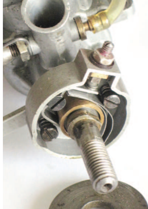
The Frog 500 5cc petrol 2-stroke of 1952 and its contact breaker in close-up.
