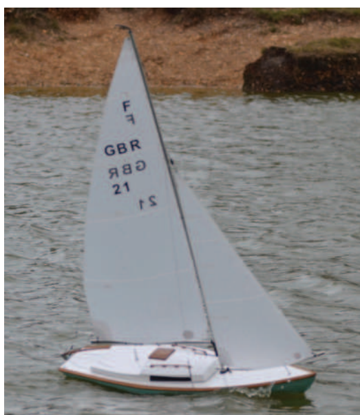
BELOW: The Nottingham 'J' is a representation of Endeavour, as built in 1934. She measures 48 inches in overall length and features twin sail winches for the Genoa and the main sails.
