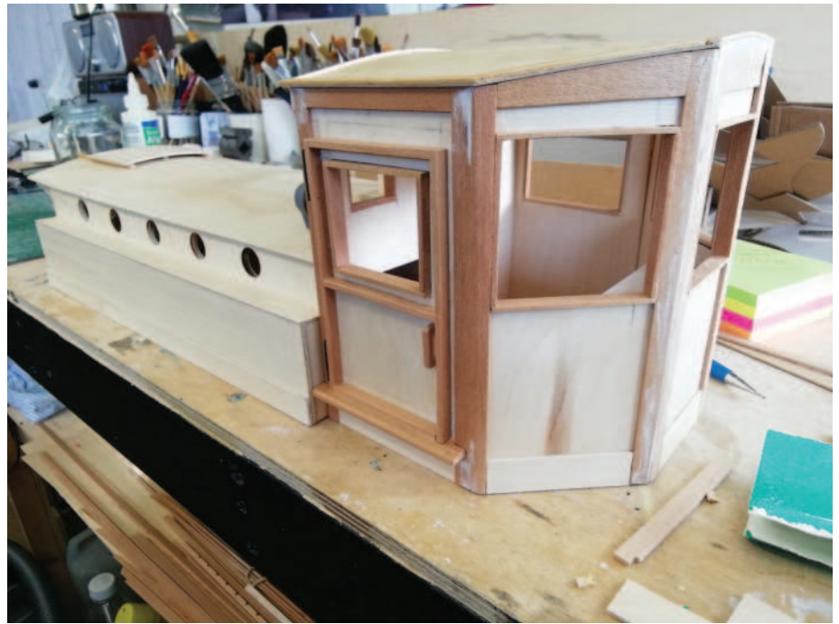
ABOVE: The deck houses under construction. Made from 2 and 3 mm plywood, these will lift off to gain access to the motor and electronics, etc.
