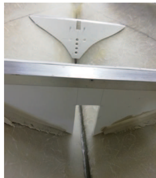
ABOVE: To convert the hold into a 'water tank' plastic was used for the bulkheads and deck. Aluminium angle was used to give additional rigidity and allow the deck to be screwed to the bulkheads. BELOW: With all the bulkheads in place it was important to ensure water could pass along the length of the boat. Holes and slots were cut in the plastic bulkheads.
