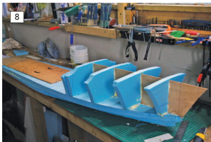
ABOVE LEFT: Michael's hot wire cutter showing a paper template pinned to Styrofoam. ABOVE RIGHT: The Styrofoam hull frames have been glued accurately in place on their marks with polyurethane wood glue.
