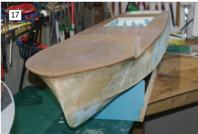
ABOVE LEFT: Getting started on the brown paper wallpapering. If attempting this yourself, use waterproof PVA glue, not the non-waterproof glue I used, Michael points out! ABOVE RIGHT: Small pieces of brown paper were cut and glued at the composite curves. Once dry, any remaining wrinkles can be lightly sanded with fine sandpaper. The stand seen here was formed from a couple of Styrofoam templates originally used to check the shape of the hull.
