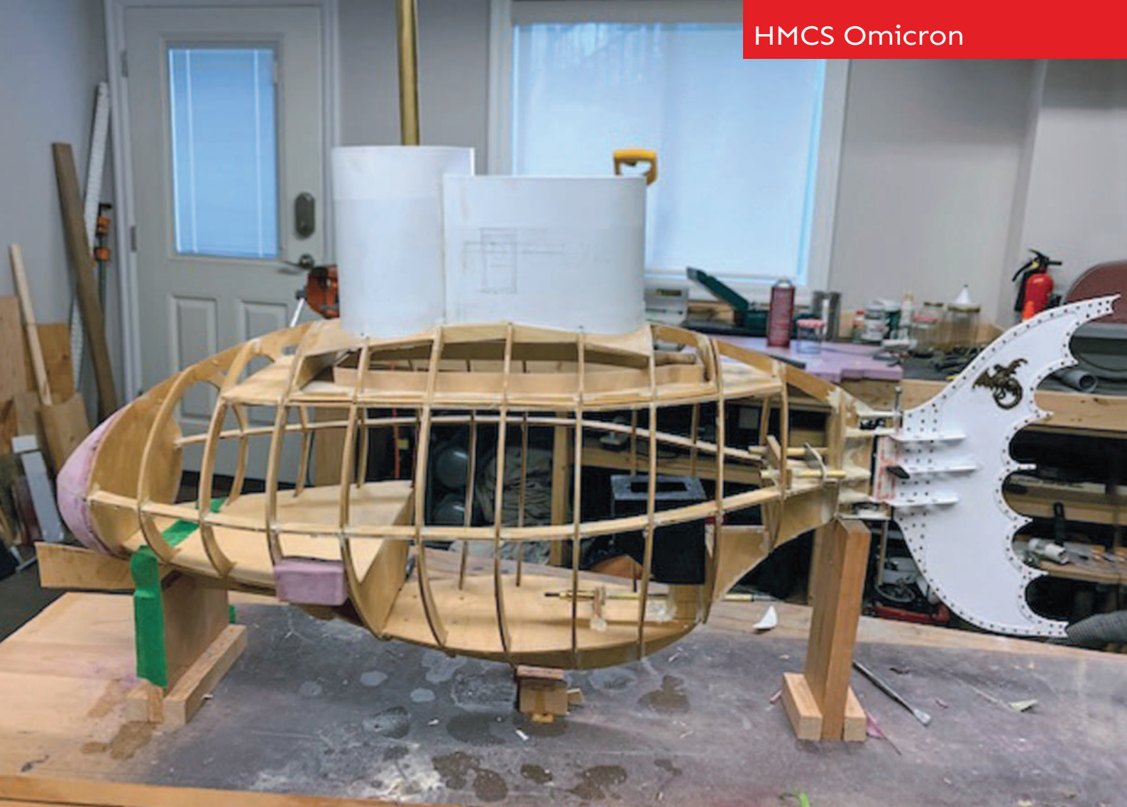
ABOVE: A photo of Omicron under construction showing frames and internal deck structure.
