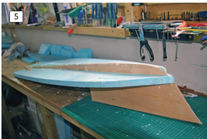
ABOVE: The foam MTB lifting onto the plane under full power. BELOW LEFT: The 2mm ply backbone of the hull with the first layers of Styrofoam. BELOW RIGHT: The engine plate is 6mm marine ply. Before assembly I aligned the motors and prop shafts then drilled the tunnels for the shafts and glued on their skegs. The hull frames and the remaining horizontal foam layer can be seen cut and ready to assemble.
