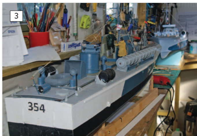
ABOVE: Vosper 70 ft MTB on the plane. BELOW LEFT: John Lambert's 1:24 lines for 70 ft MTB, which Michael scaled up on a photocopier to 1:18 scale. BELOW RIGHT: In the foreground is the original heavyweight MTB (fore) and, in the background, her younger, more lightweight, foam sister. The crew were sculpted from Milliput.
