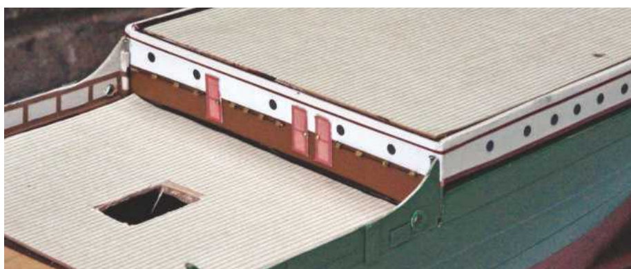
ABOVE: At small scales all you need is a PC and printer/scanner. The doors and windows here were constructed to a larger scale, scanned in and then printed out at the model scale. BELOW: The planking on this 1:150 scale model was produced on an Excel spreadsheet and printed onto cream coloured heavy cartridge paper before being stuck to the deck and varnished over.
