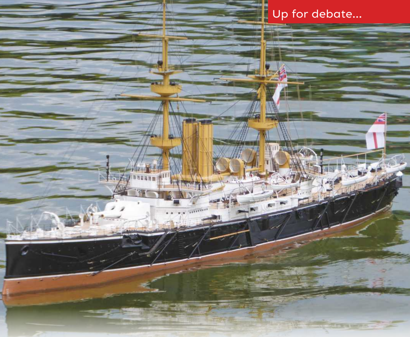
Andrew Dalton's Victorian battleship HMS Renown is another model that was many years in the making using traditional techniques, although various castings, mouldings, and etched brass patterns were employed.
