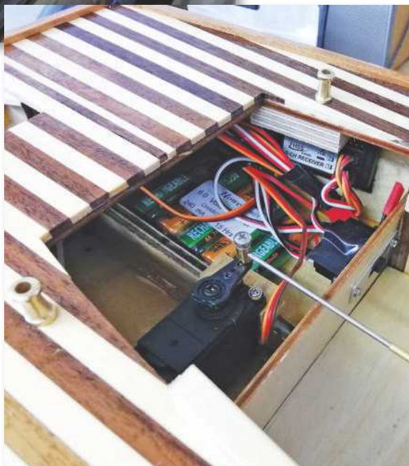
BELOW: Beneath the rear seat are the servos for the steam regulator and the rudder, plus batteries and electronics.
