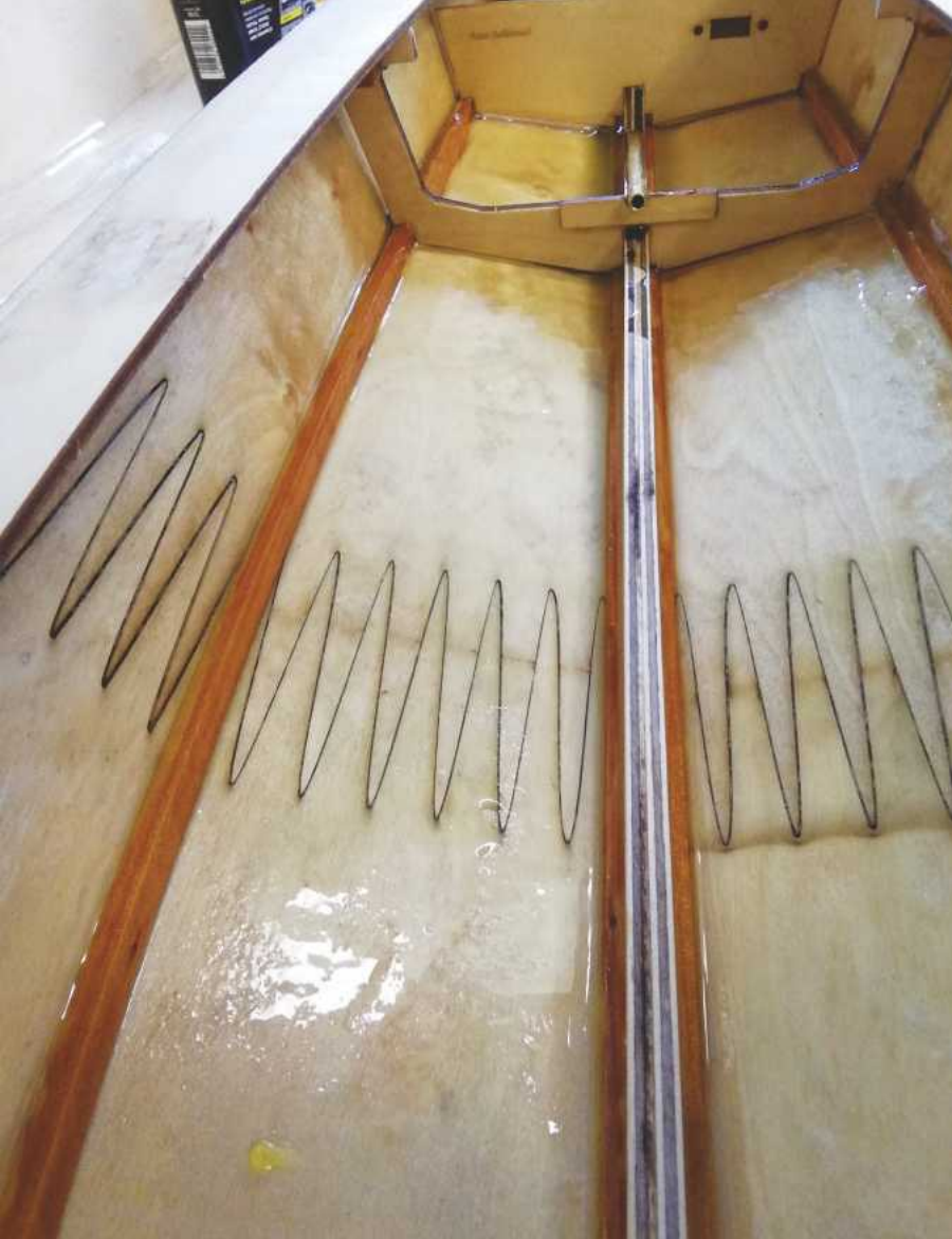
ABOVE: The inside of the hull looking reasonable after 'gallons' of resin were poured in to attempt to seal the unseen gaps.
