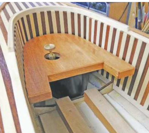
ABOVE: The gas tank is hidden beneath the removable front seat. It's advisable to remove the tank prior to it being filled with the Butane/Propane gas.
