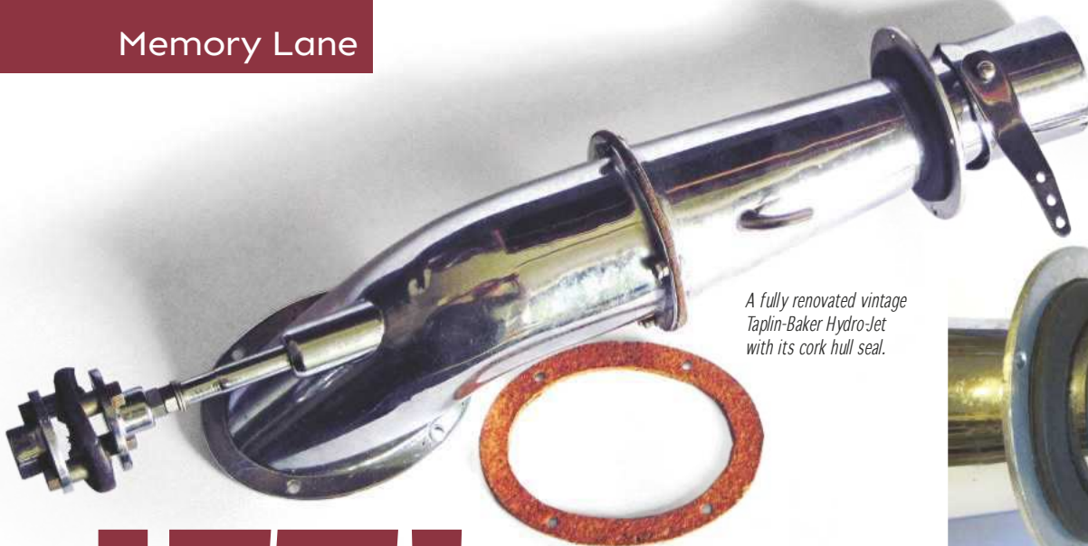
ABOVE: A closer look at the Hydro-jets steerable nozzle with transom rubber seal.
