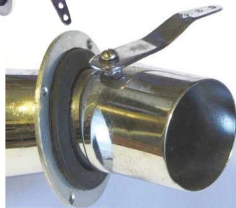
ABOVE: A closer look at the Hydro-jets steerable nozzle with transom rubber seal.
