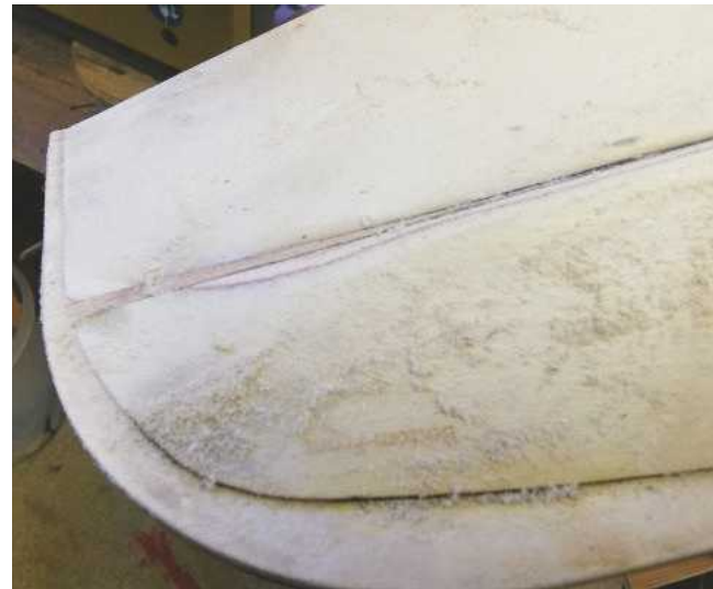
ABOVE: Once the joint line had been sanded down in order to blend the plywood panels, long 'slots' appeared.
