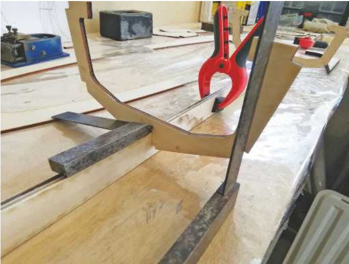
A critical operation: getting the keel and bulkheads square in all planes.
