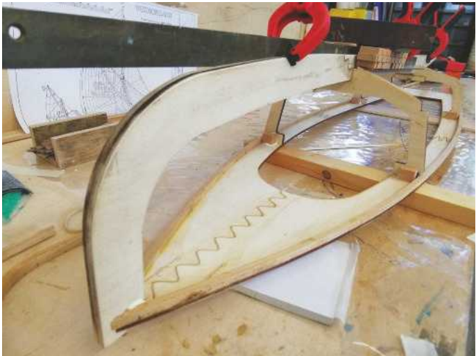
ABOVE: The deck and keel in situ. At this stage the assembly becomes more robust.
