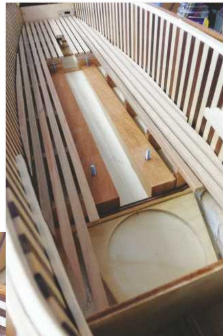
RIGHT: The duckboard flooring is cut from Parana pine and fitted around the boiler/engine. This is removable.
