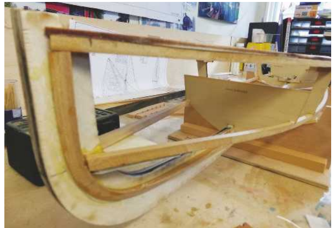
BELOW: All the stringers in place, ready for the plywood bottom and side panels to be fitted.
