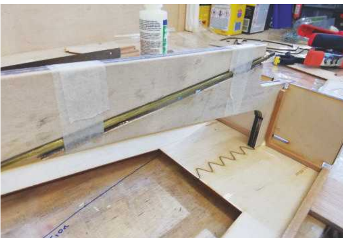
BELOW: The stern and propellor shaft glued in. Correct alignment of the shaft is imperative.
