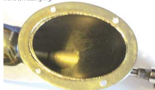
BELOW: A close-up view of the water inlet: this is equipped with a cork sealing ring.
