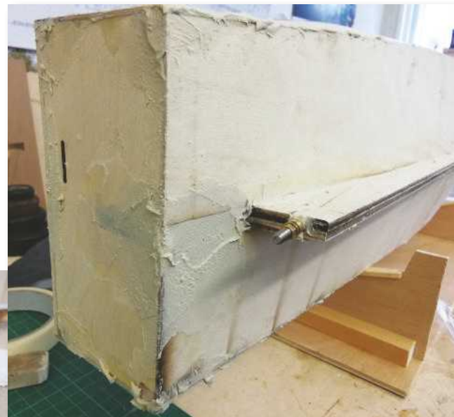
BELOW: Lashings of P38 body filler were required to bung up the slots after sanding.
