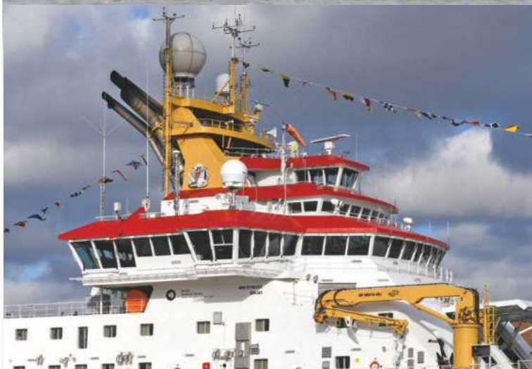
The bridge and satellite communications systems. Below the bridge are the open doors of the helideck hanger, which house two small helicopters to transfer scientists and their equipment to shore. The helideck is also used to launch aerial drones for scientific missions.
