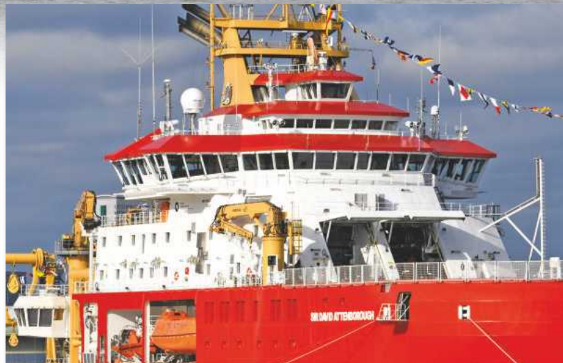
The bridge and satellite communications systems. Below the bridge are the open doors of the helideck hanger, which house two small helicopters to transfer scientists and their equipment to shore. The helideck is also used to launch aerial drones for scientific missions.
