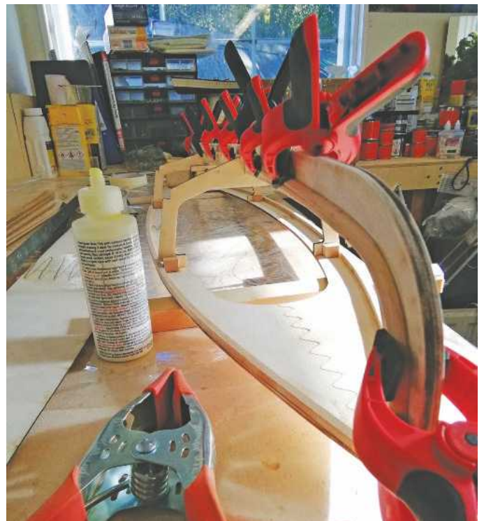
ABOVE: The bow stringers in place: these were roughly contoured by removing excess material prior to fitting.
