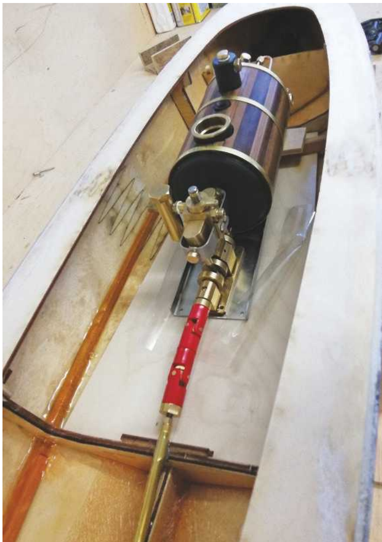
ABOVE LEFT: Offering up the boiler assembly to the launch to check for clearances. ABOVE RIGHT: Additional supports were bonded into the hull using P38: a lovely, neat job!
