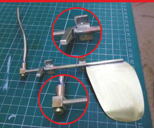
ABOVE: The rudder assembly was 'macked up' from scrap brass and parts from an old 13-amp plug.
