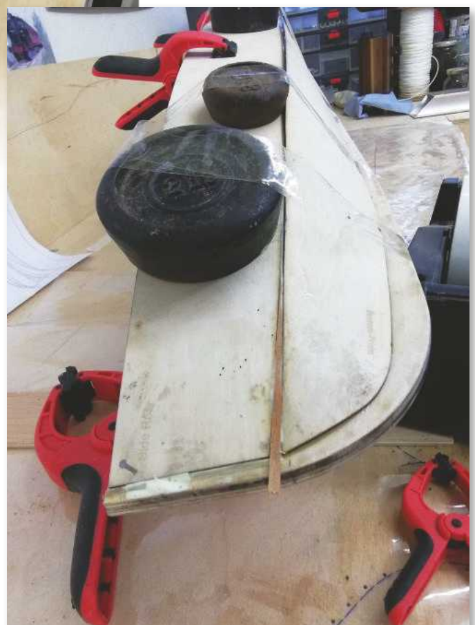
ABOVE LEFT: John's poorly fitting side panel at the stern. ABOVE RIGHT: And at the bow. Not the sliver of wood that fills the gap.
