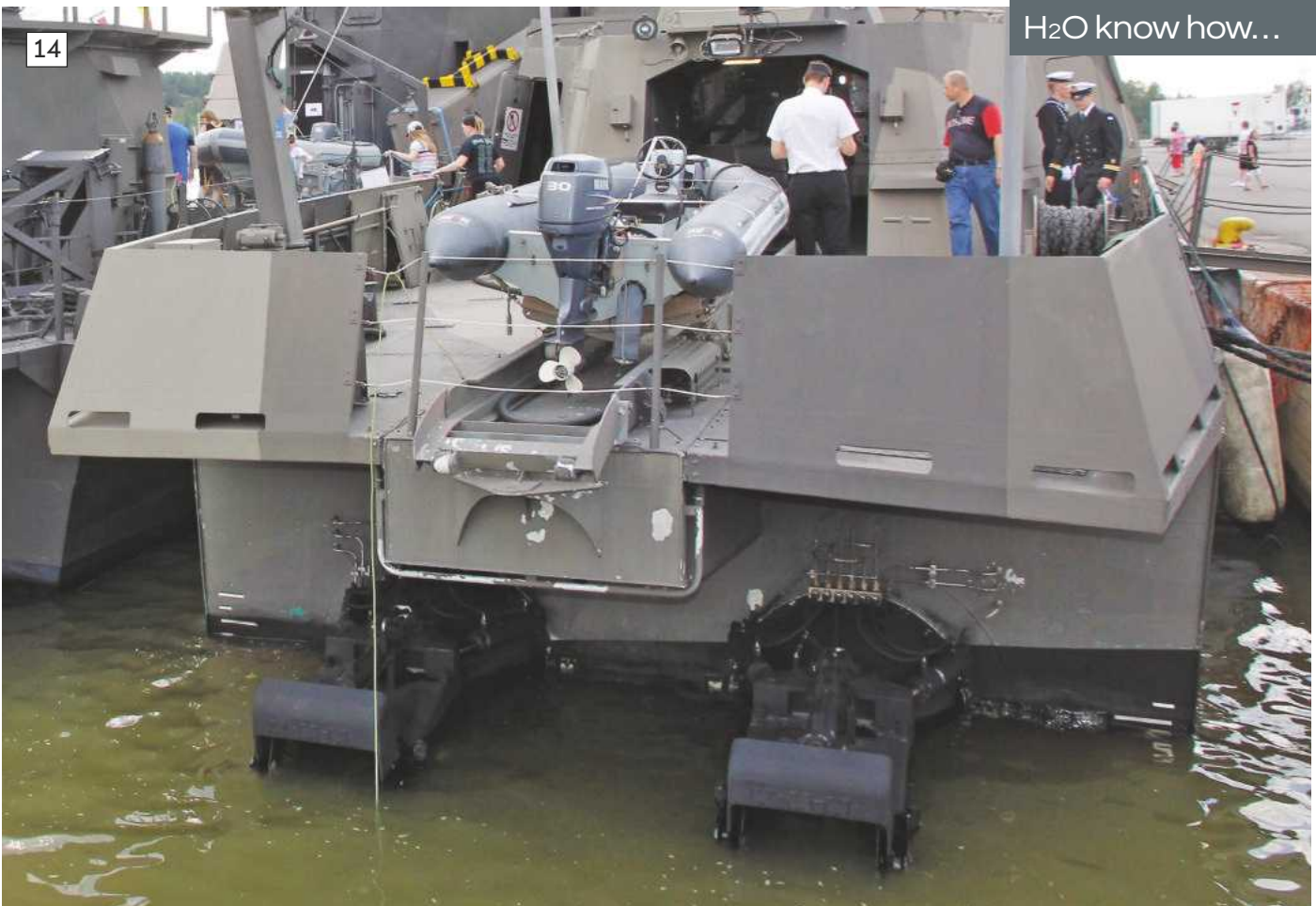
ABOVE: The Jetavator some 50% immersed on the full-sized Hamina. BELOW LEFT: With the Jetavator partially immersed, Dave powers up to check out what his drives can do. BELOW RIGHT: The water cooling as connected to the small inlet nipples on top of the stators.
