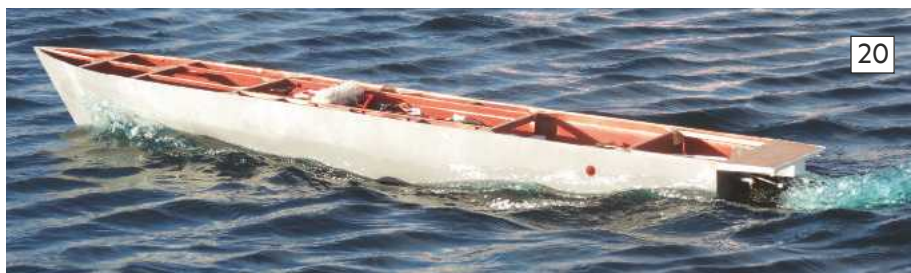
ABOVE: The hull attitude for the Hamina class missile boat at about half speed. BELOW: The model at about 50% thrust, giving a reasonable comparison to the full-size Missile Boat.
