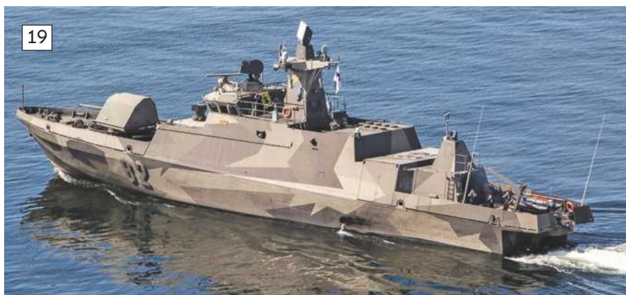
ABOVE: The hull attitude for the Hamina class missile boat at about half speed. BELOW: The model at about 50% thrust, giving a reasonable comparison to the full-size Missile Boat.
