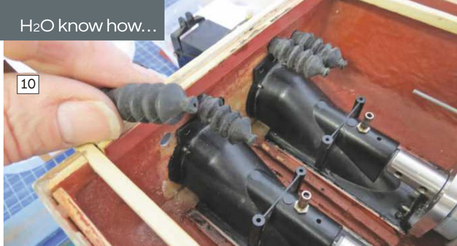
ABOVE: The four linkages have their own flexible sealing rubber rings that fit through the transom. BELOW: The fully installed and working servos and their respective linkages.
