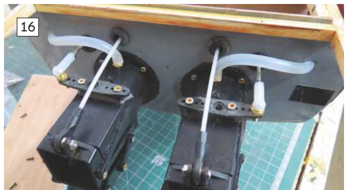
ABOVE: The Jetavator some 50% immersed on the full-sized Hamina. BELOW LEFT: With the Jetavator partially immersed, Dave powers up to check out what his drives can do. BELOW RIGHT: The water cooling as connected to the small inlet nipples on top of the stators.
