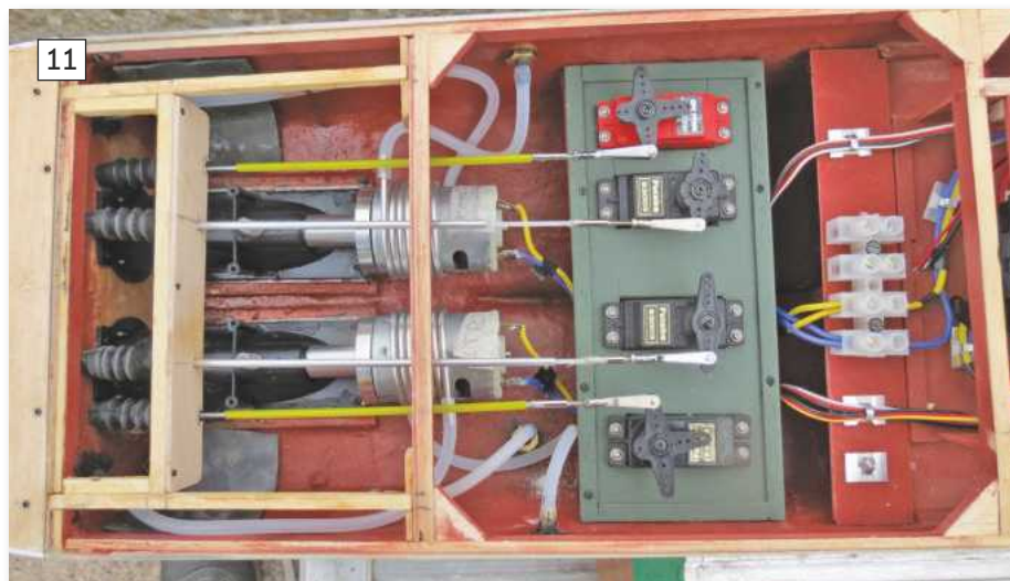
ABOVE: The four linkages have their own flexible sealing rubber rings that fit through the transom. BELOW: The fully installed and working servos and their respective linkages.
