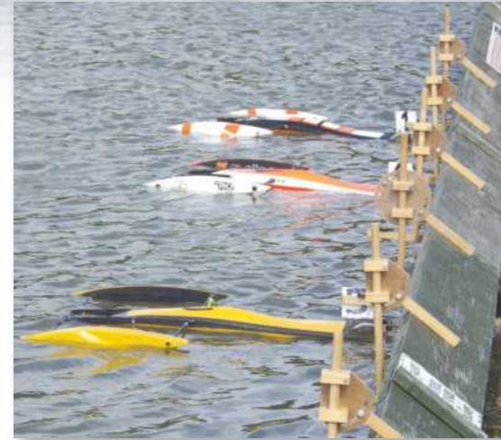
Ready for the off: three Hydro 2s held in the auto launch devices. These negate the need for human launchers.
