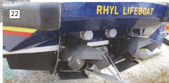
ABOVE: The superb 1:12 scale waterjet-powered Shannon class lifeboat, based on the RNLB vessel Anthony Kenneth Heard operating out of Rhyl. RIGHT: The type of reverse bucket fitted to the model is close to that seen here on the full-size craft.
