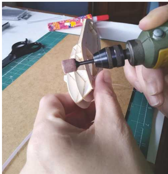
Card models are stronger than you might think. As can be seen here, a modeller's rotary tool is being used to sand the edges of the internal laser cut formers of a hull to ensure the outer printed hull parts fit onto a smooth surface.
