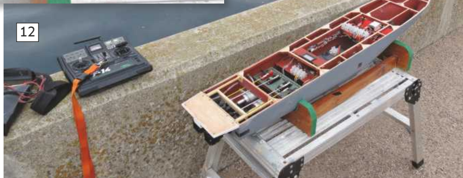
ABOVE: Following a change of R/C to the F14 this project was ready for the water. BELOW: Assessing the hull for ballast and trim but remembering the golden rule of jet drives: at least 50% of the jetavator must below water.
