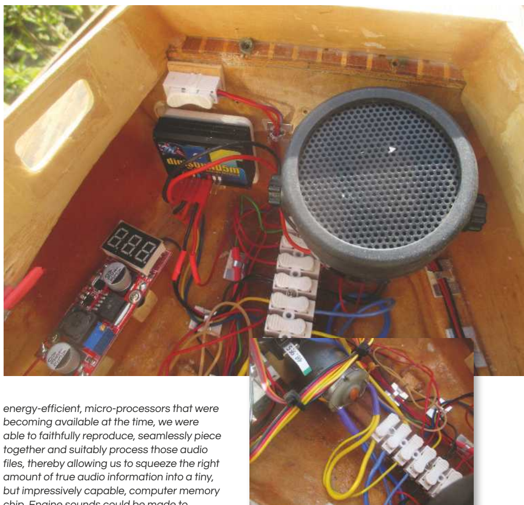
ABOVE: A close up of the Mtroniks digiSOUND unit Stan was supplied with, clearly illustrating the connection points. BELOW: The sound unit and speaker in situ.
