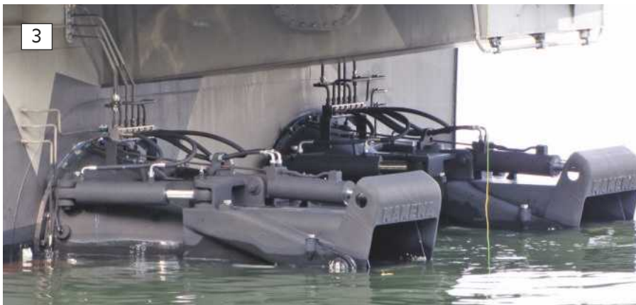
ABOVE: The RR Kamewa S11 waterjet drives, as fitted to the Finnish Hamina class fast missile boats.
