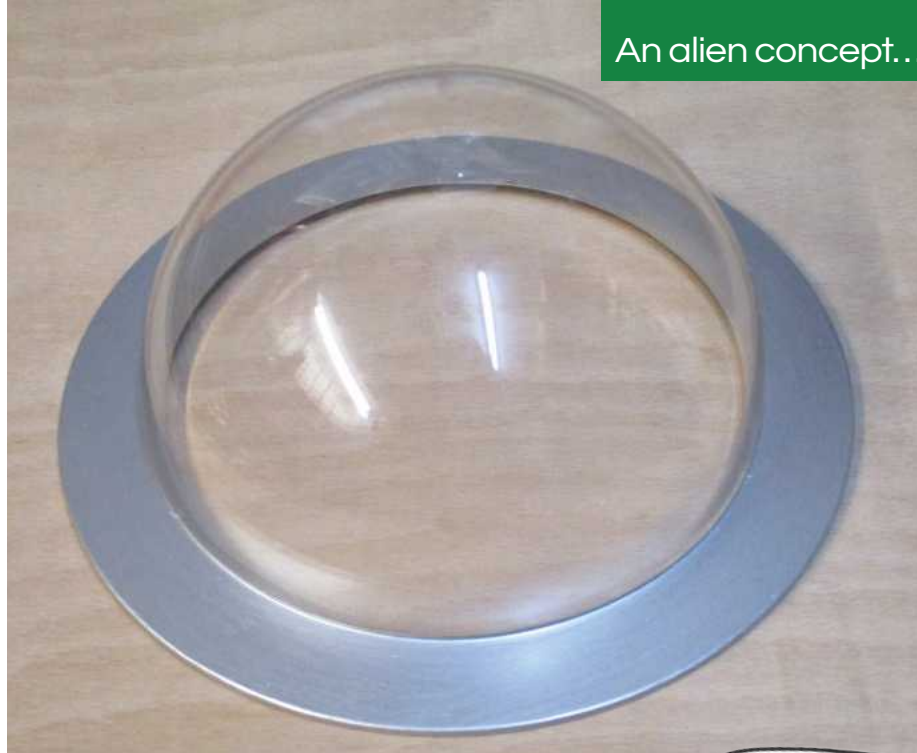
ABOVE: The acrylic dome with its flange painted.
