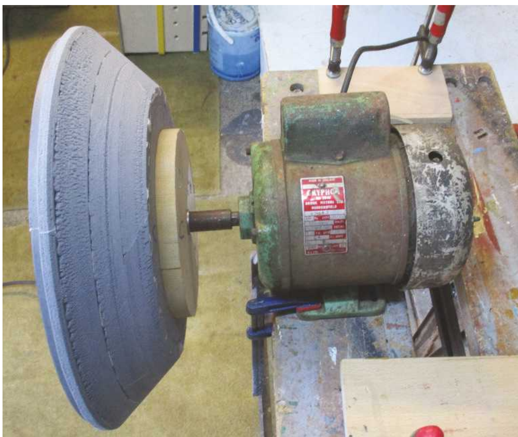
ABOVE: Ashley's temporary lathe, well tested before use. BELOW: The bottom hull half on Ashley's temporary lathe, awaiting more clamps for motor?
