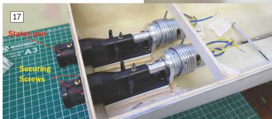
ABOVE: Motor mounting plate and motors were added to the intake body and coupled to the drive shaft. Also, the stator was combined with the intake body via the transom. BELOW: A tray was fitted forward to house the electronic speed controllers and radio receiver.
