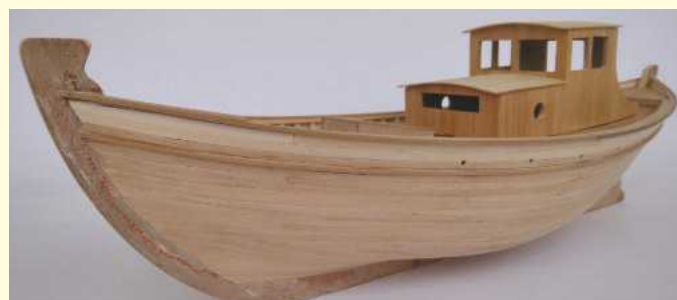
ABOVE: The kit contains everything required to build the 550mm in length model and supporting paperwork includes a 680 x 600mm sheet with two profiles and one bird's eye view, a parts list, three A3 detail plans, four A4 plans and four A4 building instructions (in both Greek and English). BELOW: Two layers of strips are suggested for hull planking: the first being 5 x 1mm lime wood and the second 0.6 x 4mm beech strips.
