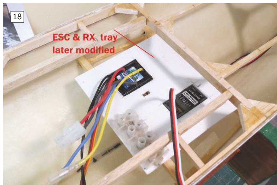
ABOVE: Motor mounting plate and motors were added to the intake body and coupled to the drive shaft. Also, the stator was combined with the intake body via the transom. BELOW: A tray was fitted forward to house the electronic speed controllers and radio receiver.
