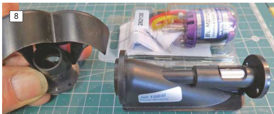
The Bower waterjet drive with the reverse bucket attached to the stator bowl.
