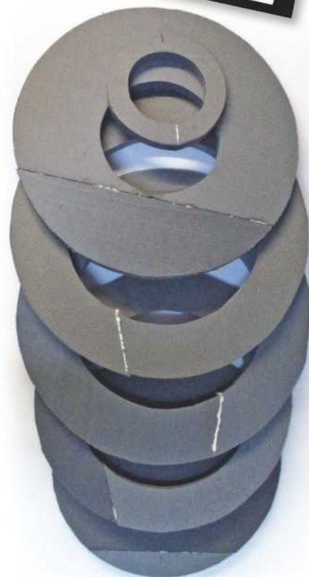
The rings of foam cut ready to be stacked and glued together.
