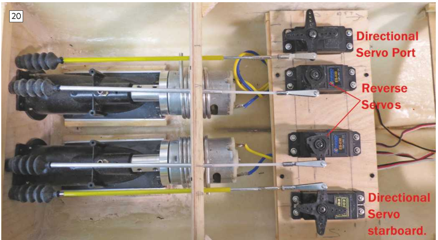
ABOVE: A platform was fitted to support the four servos (which control direction and reverse thrust) for the jetavator. BELOW: The servos were bolted to the platform. As Dave points out, it's advisable to include the rubber seating.
