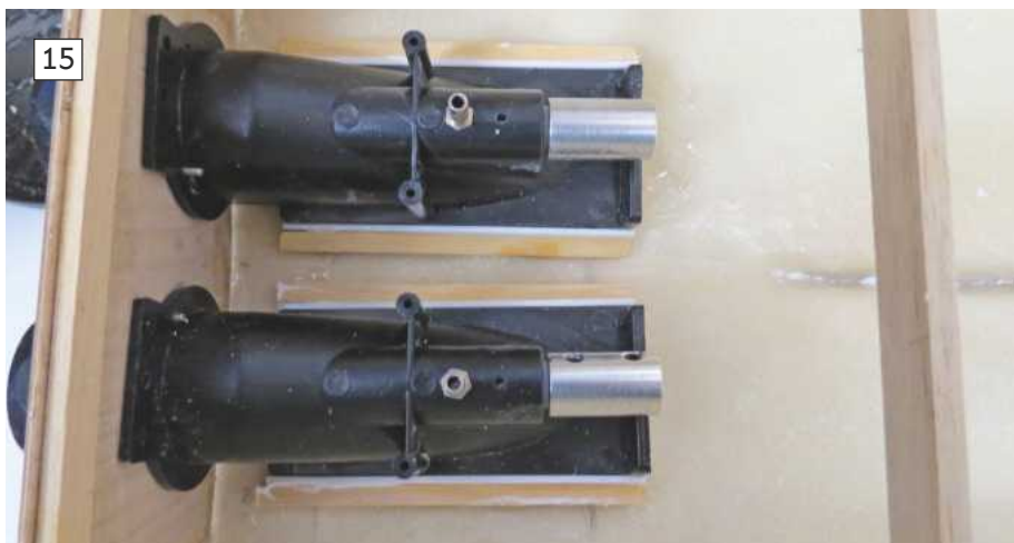
ABOVE: Preparing the seating into which the intake body would be fitted. BELOW: The seating for the intake body looking towards the transom.
