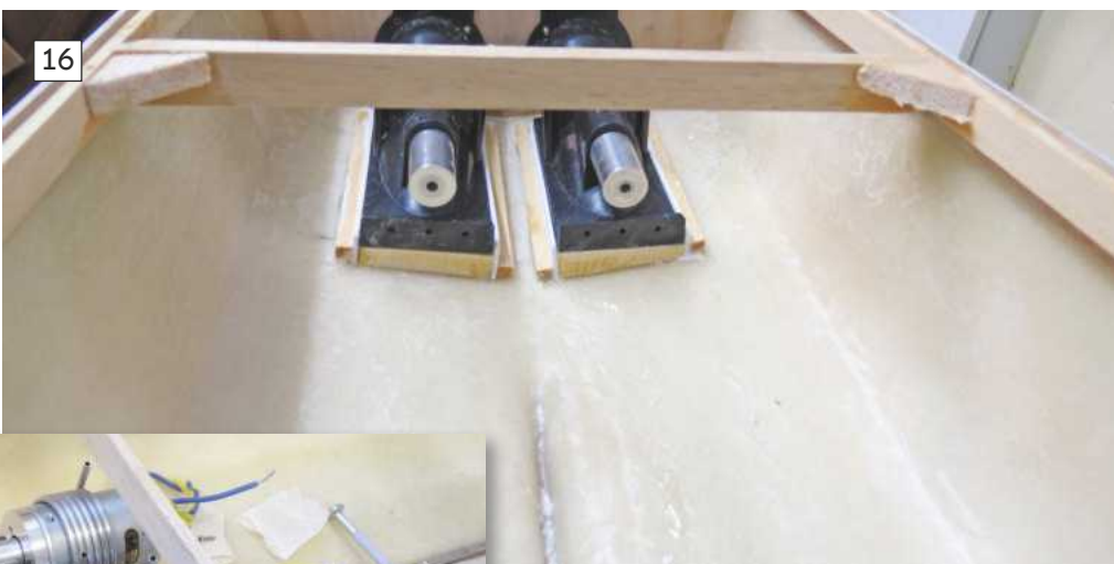
ABOVE: Preparing the seating into which the intake body would be fitted. BELOW: The seating for the intake body looking towards the transom.
