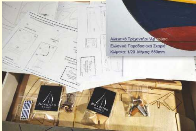
ABOVE: The kit contains everything required to build the 550mm in length model and supporting paperwork includes a 680 x 600mm sheet with two profiles and one bird's eye view, a parts list, three A3 detail plans, four A4 plans and four A4 building instructions (in both Greek and English). BELOW: Two layers of strips are suggested for hull planking: the first being 5 x 1mm lime wood and the second 0.6 x 4mm beech strips.
