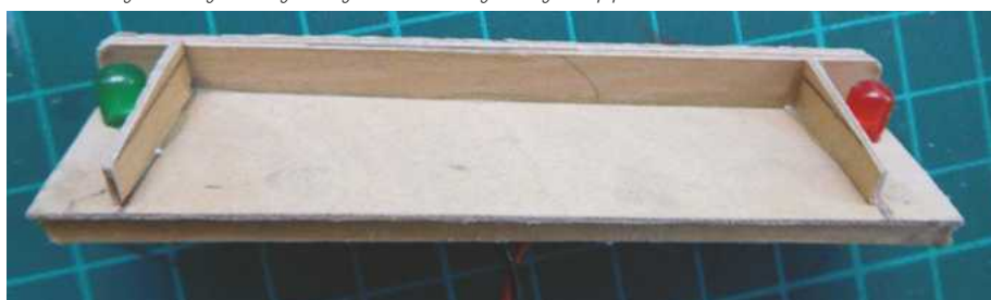
ABOVE: Showing the wiring for navigation lights. BELOW: Navigation lights top panel.
