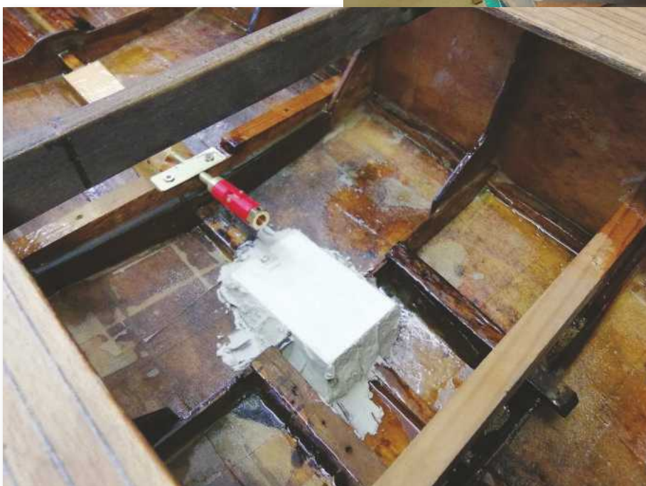
Although looking a bit messy at this stage, note the new motor pad and transmission, plus the fibre glassed hull.
