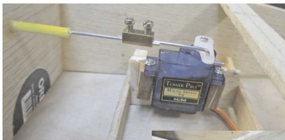
ABOVE: The rudder servo forward; note electrical connector for adjustment. RIGHT: The rudder arrangement, later this would be made a little larger.
