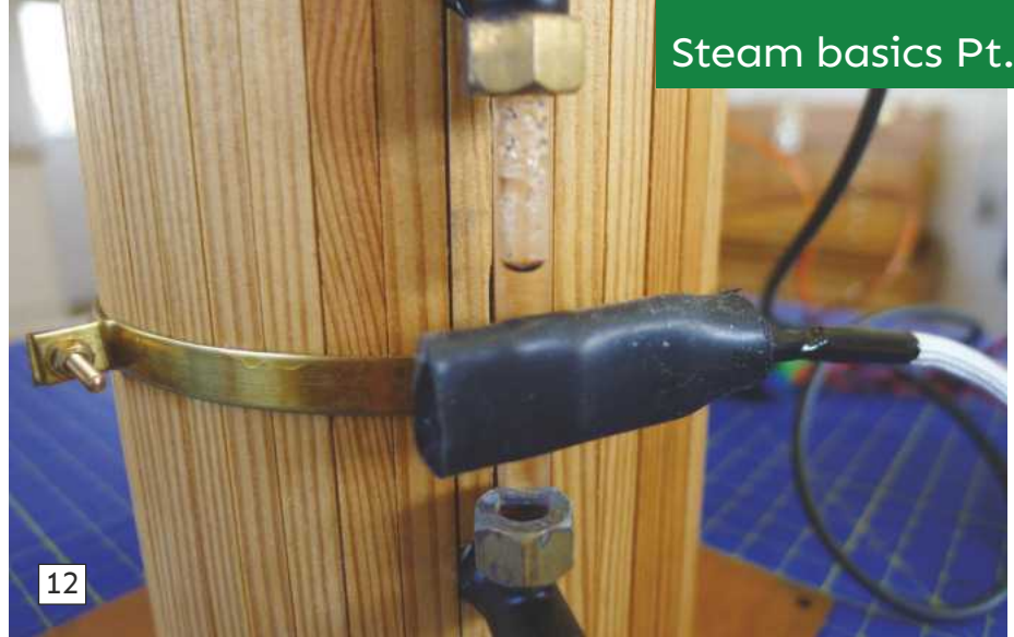
ABOVE: Starting off with the sensor below the water level the water valve servo was in the ‘closed’ position and the appropriate LED remained off. BELOW: Moving the sensor up into the steam space and leaving it there for over five seconds operated the water valve servo and permanently illuminated the LED.
