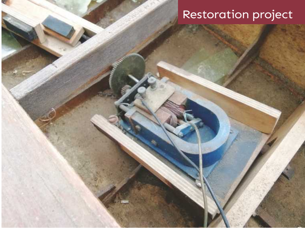
ABOVE: The original Bassett-Lowke motor and gearbox in situ. BELOW: The original state of the inside of the hull.
