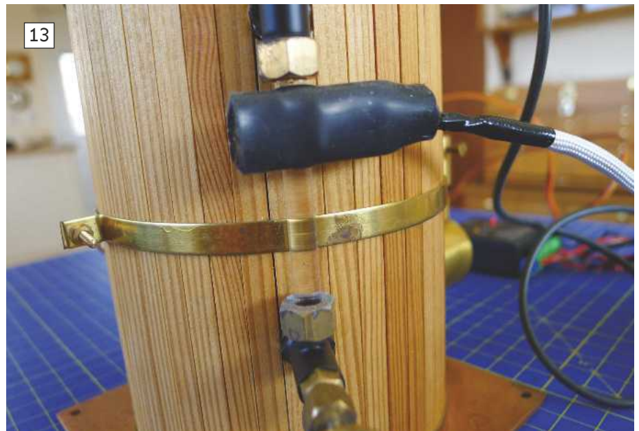
ABOVE: Starting off with the sensor below the water level the water valve servo was in the ‘closed’ position and the appropriate LED remained off. BELOW: Moving the sensor up into the steam space and leaving it there for over five seconds operated the water valve servo and permanently illuminated the LED.
