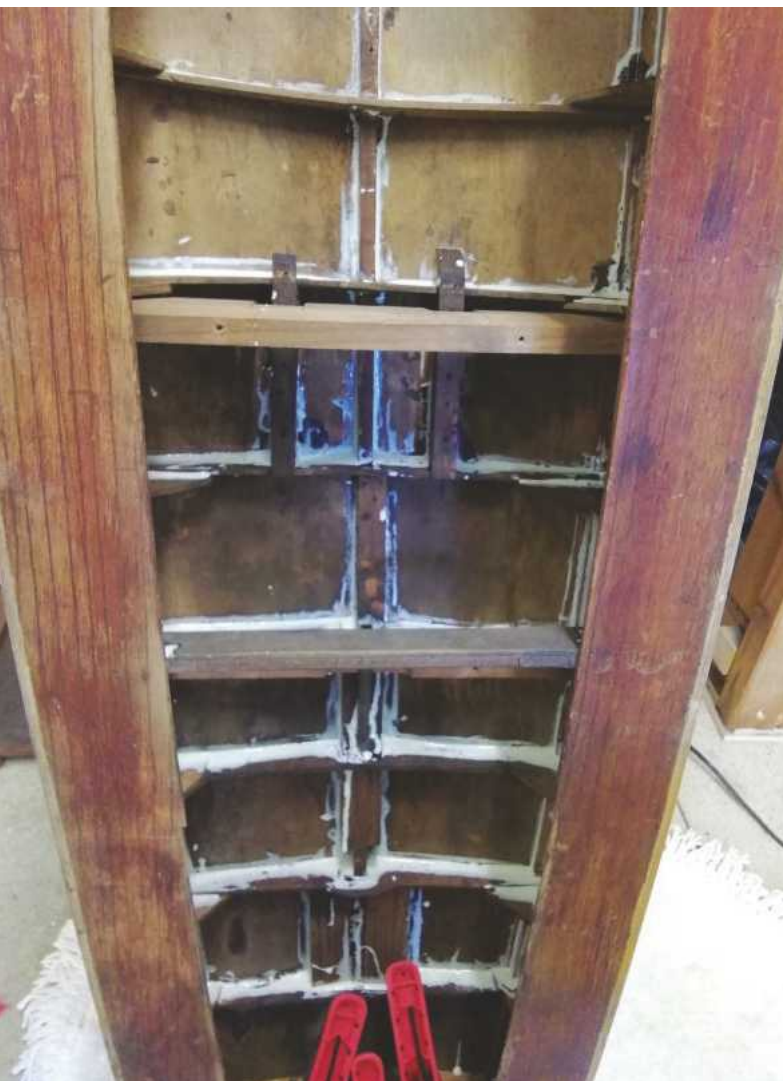
ABOVE LEFT: Aliphatic resin applied to all the internal joints. ABOVE RIGHT: Various stages of paint and varnish removal can be seen here. The bottom section shows the original coating; the centre, the stripper applied; while the top illustrates the finished stripped surface. BELOW: The hull having been completely stripped.
