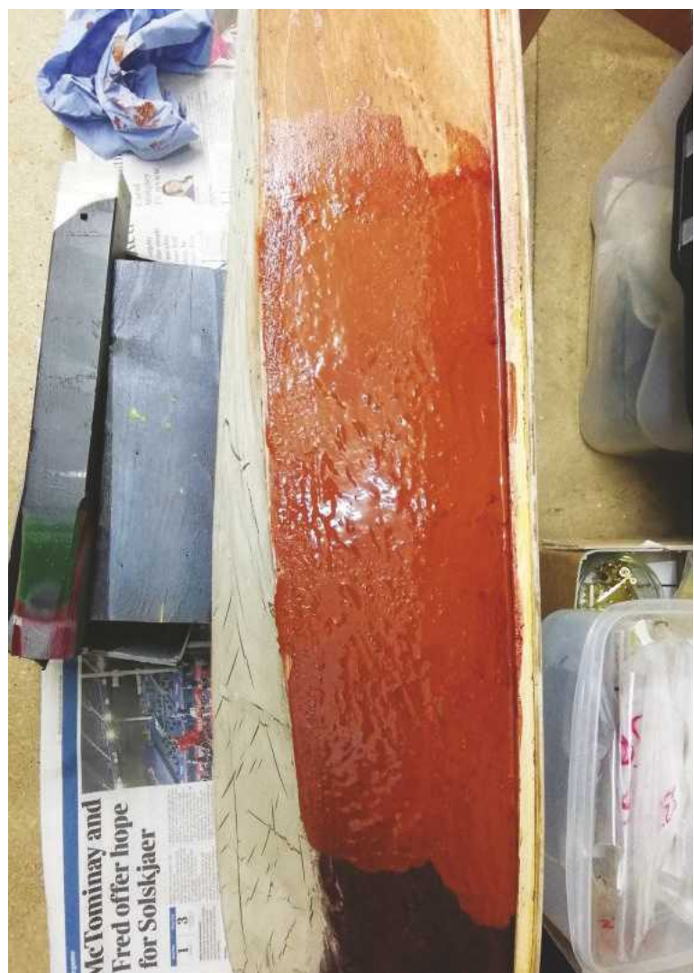
ABOVE LEFT: Aliphatic resin applied to all the internal joints. ABOVE RIGHT: Various stages of paint and varnish removal can be seen here. The bottom section shows the original coating; the centre, the stripper applied; while the top illustrates the finished stripped surface. BELOW: The hull having been completely stripped.
