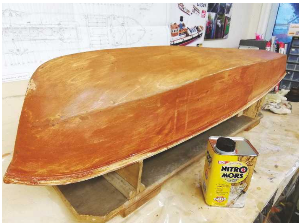
ABOVE LEFT: Aliphatic resin applied to all the internal joints. ABOVE RIGHT: Various stages of paint and varnish removal can be seen here. The bottom section shows the original coating; the centre, the stripper applied; while the top illustrates the finished stripped surface. BELOW: The hull having been completely stripped.
