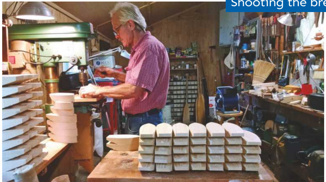
ABOVE: George in his workshop using the drill press to make mast steps and holes for pegs for Bermuda hulls in the Pine Wood Sailer series. BELOW: Seaworthy Small Ships' Pine Wood Sailer Neon Tetra diving submarine superimposed on a photo Marla took at the Baltimore Aquarium.
