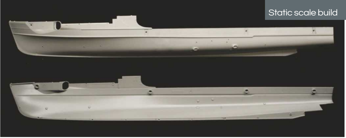
ABOVE: The largest parts in Italeri's new S38 kit are two huge hull halves. These have to be screwed together.
