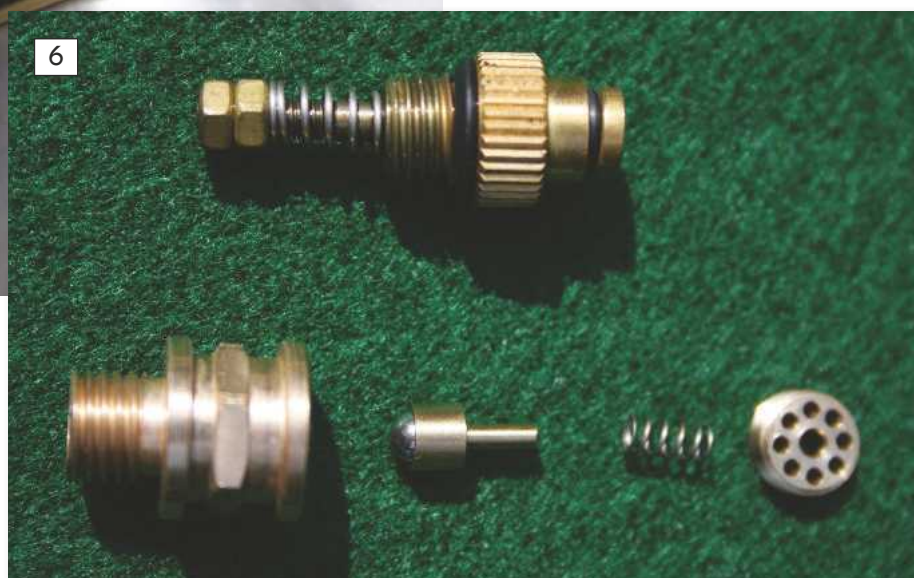
Prolonged periods of inactivity can lead to safety valves sticking. A good clean is well worth the effort and will give you confidence that it will work for the test.
