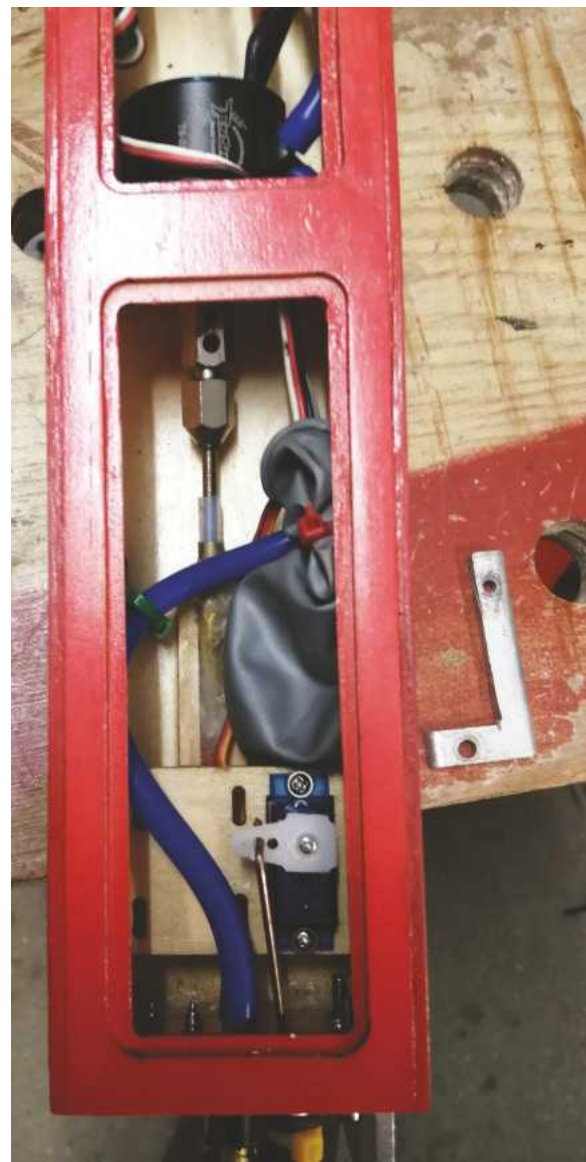
ABOVE LEFT: Almost complete: the white tape seen here is to hold the booms and tubes in place during drilling. ABOVE RIGHT: The radio compartment: the receiver is in the grey balloon. BELOW: The little tool I made to aid with fitting the motor: a simple rigid plastic tube and a little fuel tube (see text at the end of the previous page).
