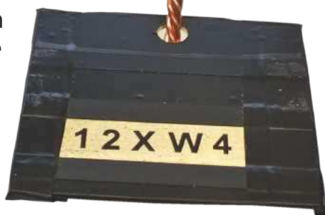
Photo 3: Here we see Dave's brass plate masked and with letters and numbers 'blacked out' by 5mm BECC transfers ready for the 'alchemy' part of the exercise.
