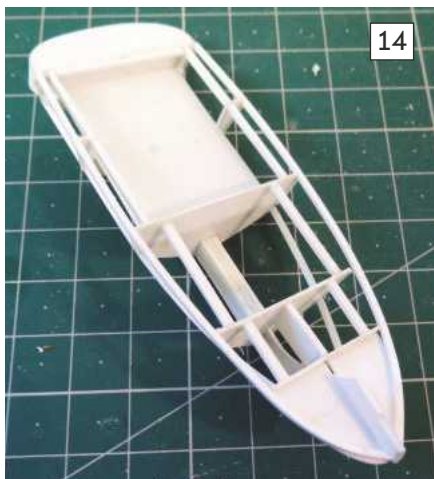
Photo 14: The Crew Boat was modelled in Dave's tried and tested method of construction, but in this instance using styrene. Photo 15: Fully assembled, but the deck, cab and hull can be separated for ease of painting.
