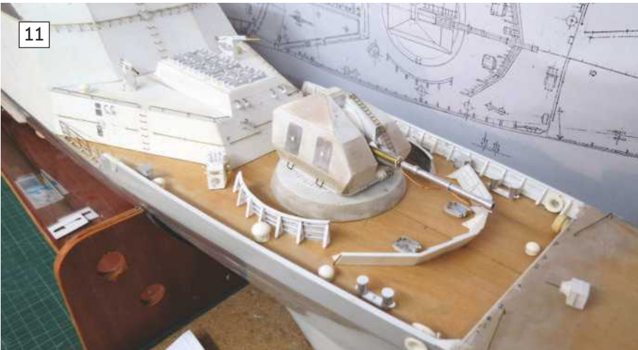
Photo 11: Fully assembled and fitted into place, the 100mm main gun. Photo 12: Each of the parts for the PUMA targeting radar housing. Photo 13: Ringed in red, the fully assembled PUMA radar in place.
