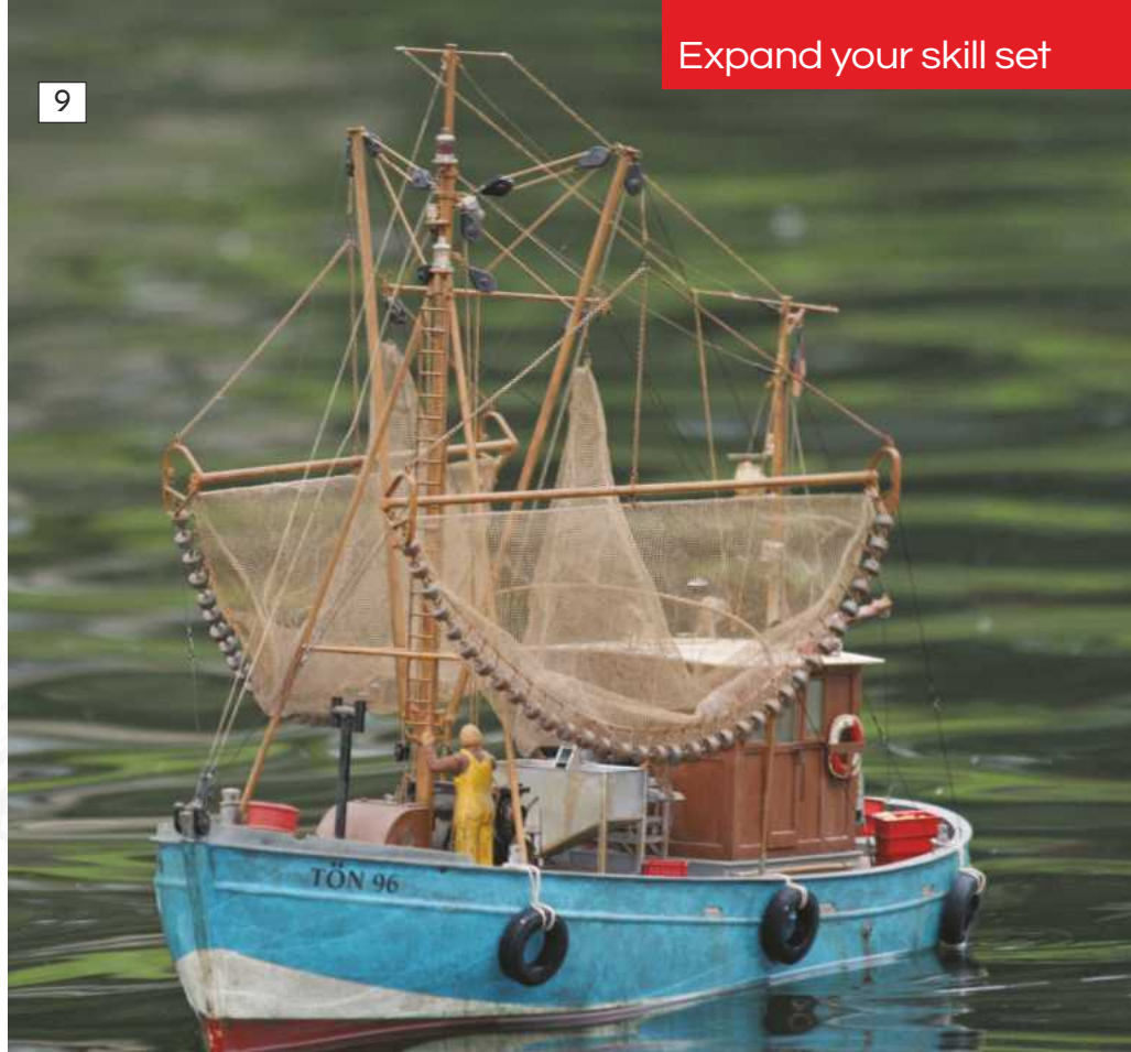
A number of pieces of the standing rigging on this trawler have been made from a solid rod. Painted up appropriately, they fit in perfectly and will not start to sag with age.
