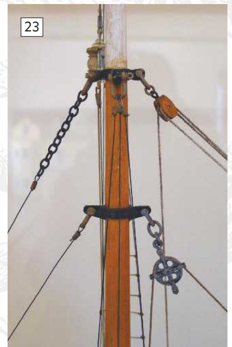
ABOVE: Boat decks can certainly benefit from some rigging and a combination of standing rigging and running rigging adds to the interest. Note the bottle screws on the mast shrouds here.
