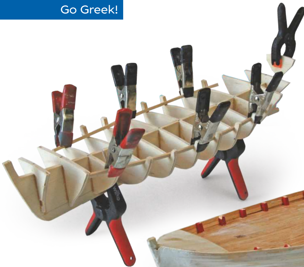
LEFT: The basic CNC cut framework with deck support stringers in place.
