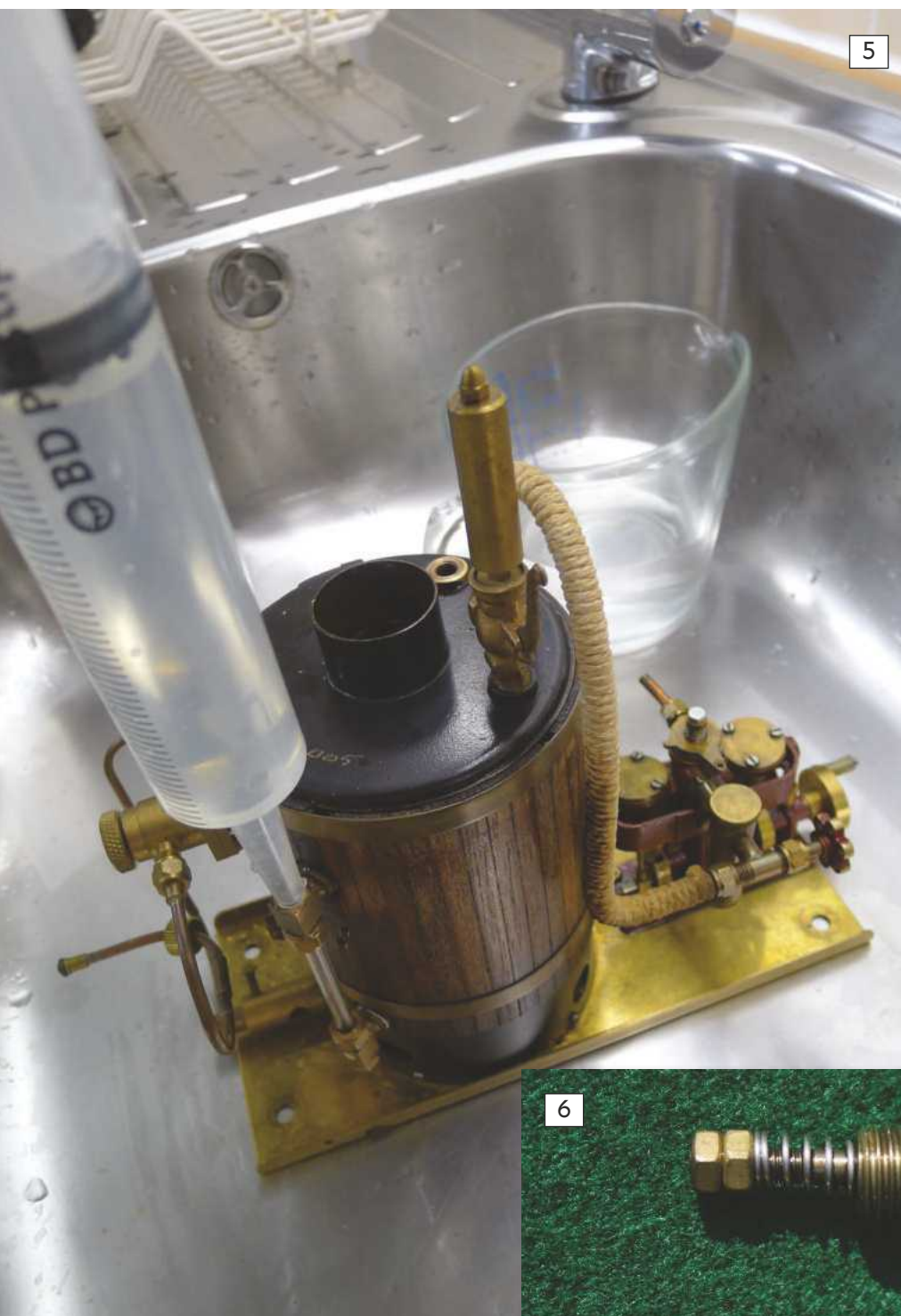
ABOVE: A good blow through with a large syringe should ensure that any restrictions around the glass connections are removed, ensuring the glass reads correctly.
