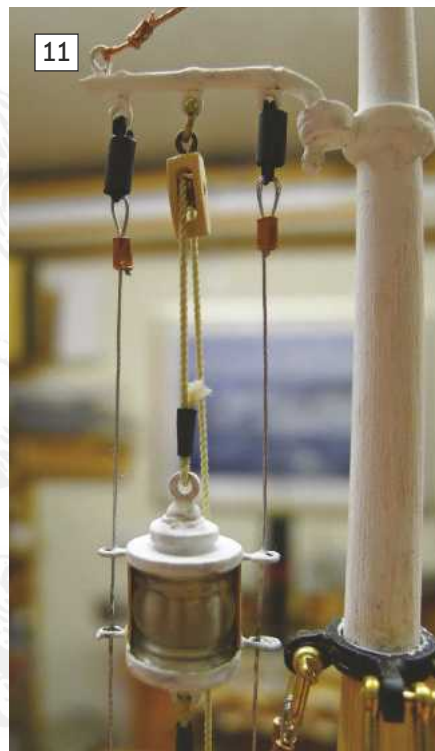
ABOVE: Halyards, particularly for flags and signals and, in this case, oil lamps, will usually be a complete loop of rope, allowing for raising and lowering from the deck level. This will then be tied off to a cleat to hold it in position.
