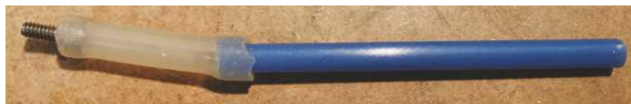
ABOVE LEFT: Almost complete: the white tape seen here is to hold the booms and tubes in place during drilling. ABOVE RIGHT: The radio compartment: the receiver is in the grey balloon. BELOW: The little tool I made to aid with fitting the motor: a simple rigid plastic tube and a little fuel tube (see text at the end of the previous page).
