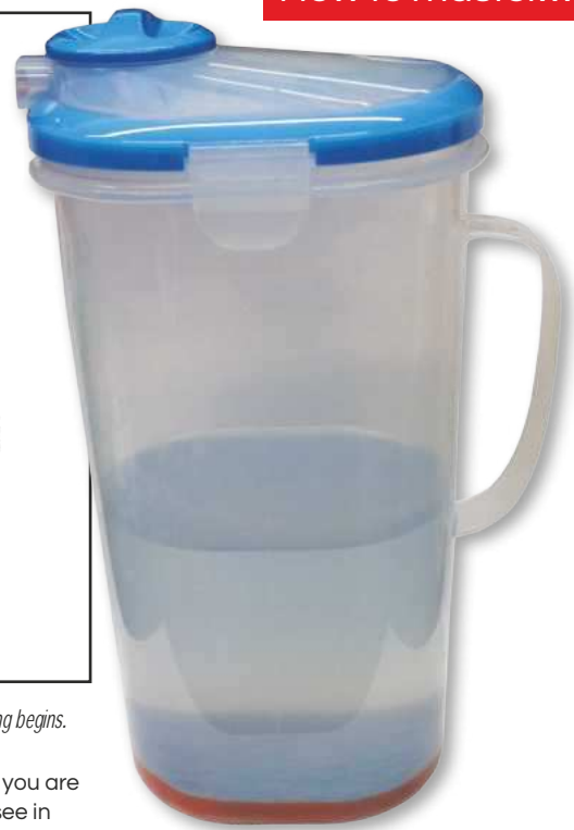
Photo 7: After use, a layer of brown salt/brass sediment will settle at the bottom of the saturated salt solution in your plastic container, as shown here. This doesn't mean your solution can't be reused, although Dave would not recommend doing this more than three or four times.
