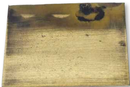
Photo 2: Your brass plate will need to be prepped, i.e. lightly sanded and cleaned, before you begin masking off the areas to be etched.
