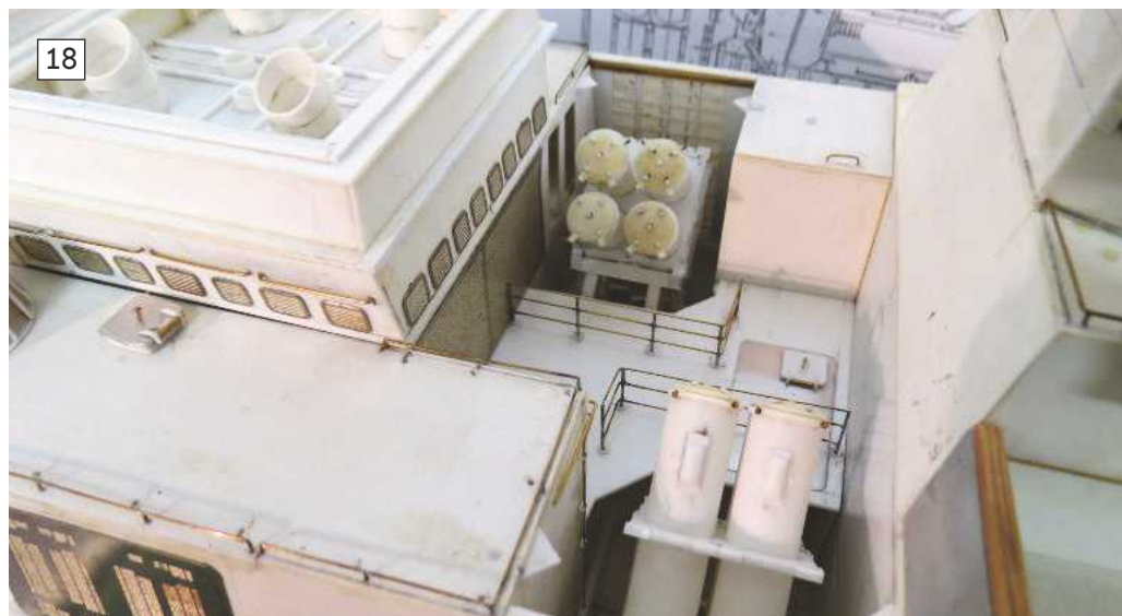
Photo 18: The two sets of launch tubes slotted into bays amidships. Photo 19: The fully prepared hangar interior. Photo 20: The hangar painted and with lighting added.
