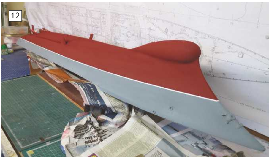
Photo 12: The anti-foul and white boot topping completed. Photo 13: The blue used for the Crew Boat's hull.
