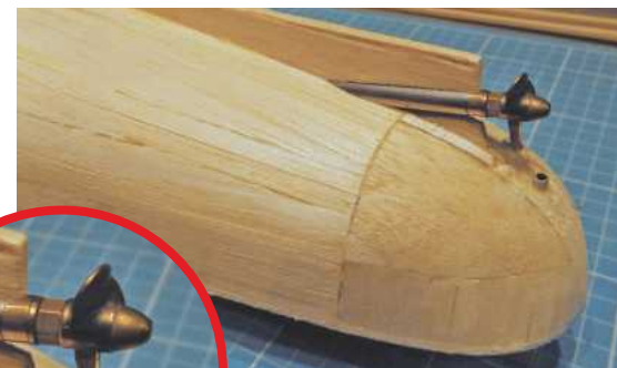
BELOW: The stern tube and 25mm three-blade propeller in place.
