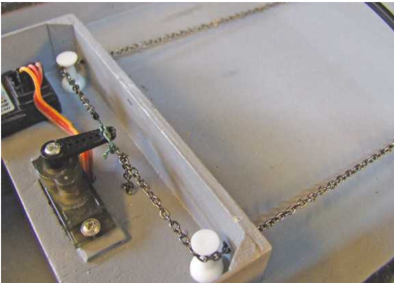
ABOVE: The twin motors and mount bracket. BELOW LEFT: The steering gear, servo end. BELOW RIGHT: The steering gear, tiller end.
