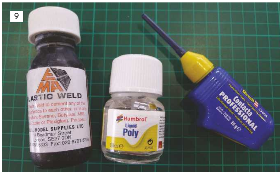
Things have moved on from the tubes of polystyrene cement we all used as youngsters. Nowadays very thin liquid cement that can be applied by brush is available. There's also relatively thin cement that can be very precisely applied via an applicator pipette. Or we can still, of course, opt for a good old tube of thicker cement.
