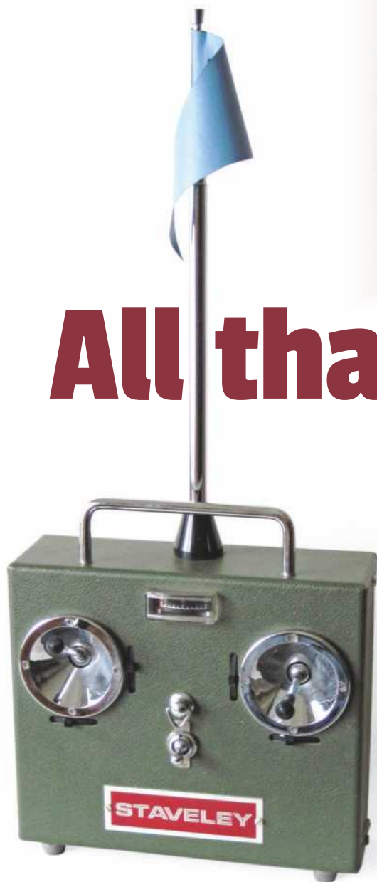
ABOVE: The Staveley-4 transmitter with American Kraft sticks in its most expensive guise was the last British analogue full house proportional to resist the digital takeover.
