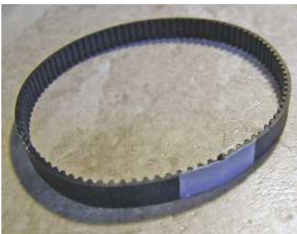
ABOVE LEFT: 3D printer belt, showing its join. ABOVE RIGHT: The motors and electronics used.
