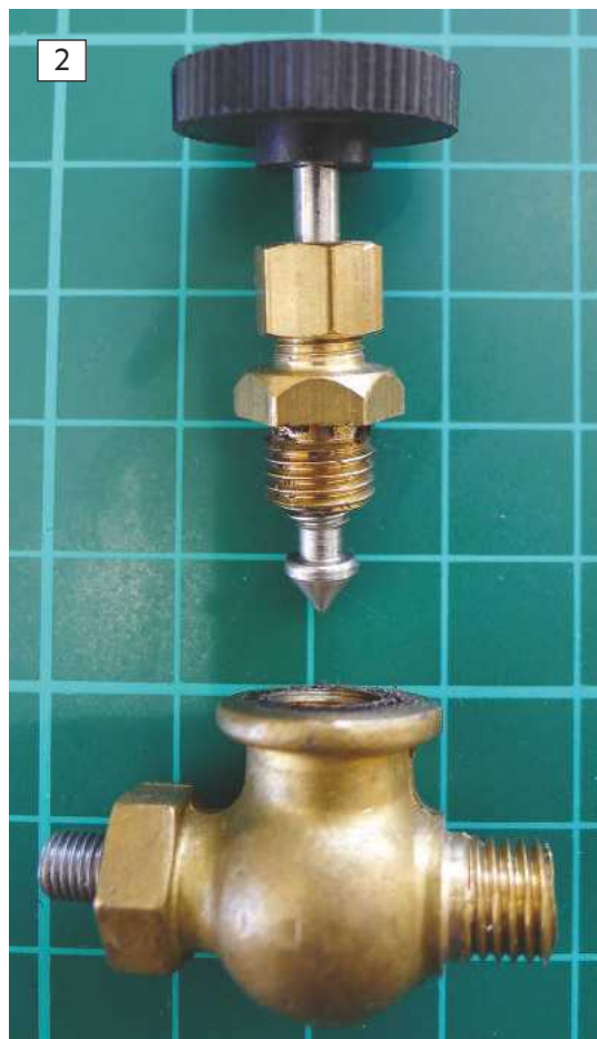
ABOVE LEFT: Just about the simplest valve you can get: this cone shaped valve sits on a narrow ground seat in the valve body. The removable workings contain the spindle, threaded into the valve ‘bonnet’ and the gland to allow rotation while sealing the spindle. ABOVE RIGHT: An excellent example of two valve types in a single item. The fine needle valve offers control but can be damaged with the excessive force used to shut off flow. The on/off valve for the drain is much sturdier and more robust for tightening down on the seat for a complete shut off.
