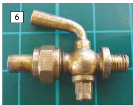
Frequently used as cylinder drain valves, this type of valve can be seen at a glance to be either open or closed. Usually, the convention is that the port drilling in the plug is in line with the position of the handle. Consequently, this valve is open.
