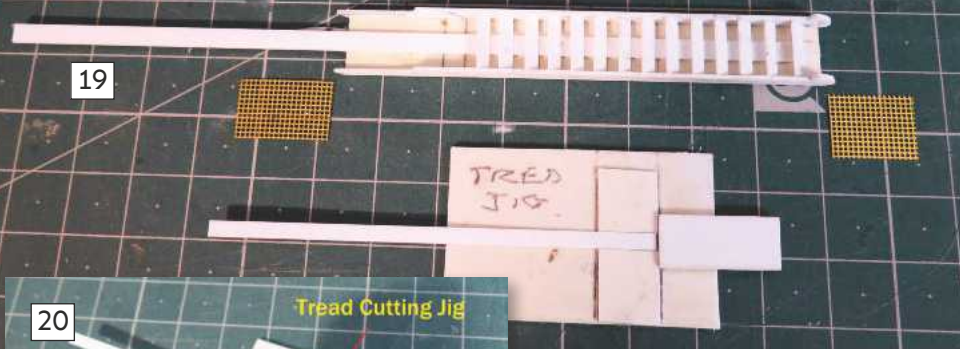
Photo 19: Two nifty techniques are applied to ensure the treads for the accommodation ladder are set at the required height and angle and are cut to the exact width to fit between the stringer boards.
