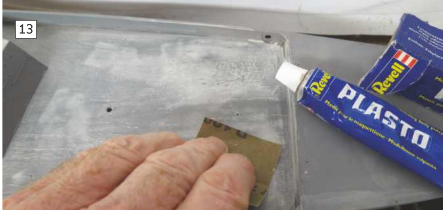
Photo 13: Refining the surface of the forecastle with a coat of Revell Plasto and rubbing down with 800 wet and dry sandpaper.
