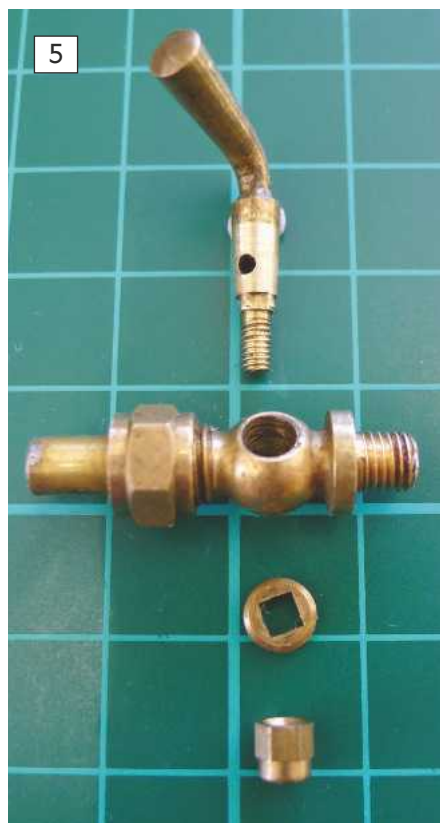
Taper plug valves can either be left with minimum clearance to get the best seal or the nut can be tightened for a complete shut off. It will then require slackening off to operate the valve.
