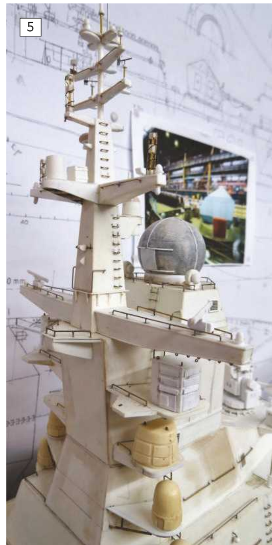
Photo 4: The combined life raft containers and container frames: the containers simply slot into the frame. Photo 5: The 3D printed radar dome sits forward of the prepared foremast.
