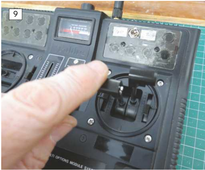
Photo 8: Dave's 20-year-old Futaba-Robbie F14, originally 40MHz, has been converted to operate selectively at both 24 GHz and 40 MHz. Photo 9: Added to Dave's original F14 is the duel stick throttle control; he explains that operation initially required some practice but that it's something he wouldn't want to be without now.
