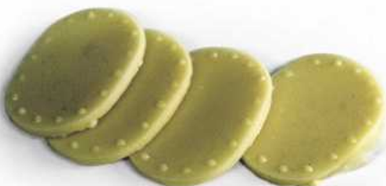
ABOVE: The oval manholes are located on either side of the tank well; cast in resin, they require sanding to reduce their thickness.
