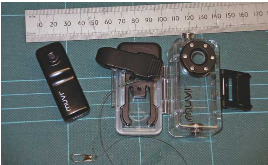
ABOVE LEFT: Nev's tiny miniature video camera and its waterproof case. ABOVE RIGHT: The lanyard attached to the case is Nev's own innovative addition. As well as clipping the camera case to the model, he also clips on the lanyard so that should the manufacturer's clip fail and the case and camera go in the water he doesn't lose the lot! BELOW: The miniature camera clipped to a model barque.
