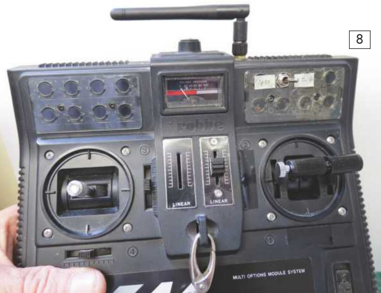
Photo 8: Dave's 20-year-old Futaba-Robbie F14, originally 40MHz, has been converted to operate selectively at both 24 GHz and 40 MHz. Photo 9: Added to Dave's original F14 is the duel stick throttle control; he explains that operation initially required some practice but that it's something he wouldn't want to be without now.
