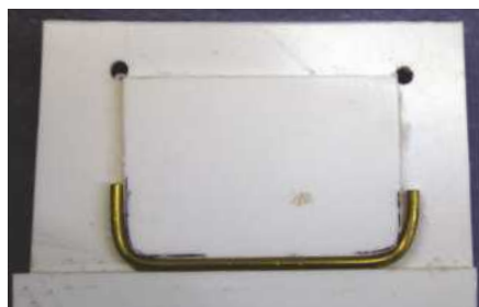
Not mentioned in the main text, Nick’s homemade jig, inspired by David Wooley’s methodology, creating four identical rungs for the ladder in the tank well rear bulkhead.
