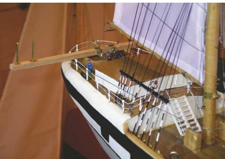
ABOVE LEFT: A still from an on-board video camera positioned to look forward from an 'outrigger' located near the stern. Check out that water coming over the bulwarks! ABOVE RIGHT: You will find it pays to experiment with the positioning of your camera. Here Nev has it set up in the rigging. BELOW: Screwing an 'outrigger' onto your model permits you to clip/affix a miniature camera to it, thereby enabling some superb and dramatic 'over the side' shots/footage as a model heels.
