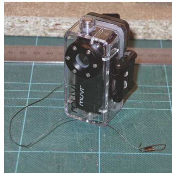
ABOVE LEFT: Nev's tiny miniature video camera and its waterproof case. ABOVE RIGHT: The lanyard attached to the case is Nev's own innovative addition. As well as clipping the camera case to the model, he also clips on the lanyard so that should the manufacturer's clip fail and the case and camera go in the water he doesn't lose the lot! BELOW: The miniature camera clipped to a model barque.
