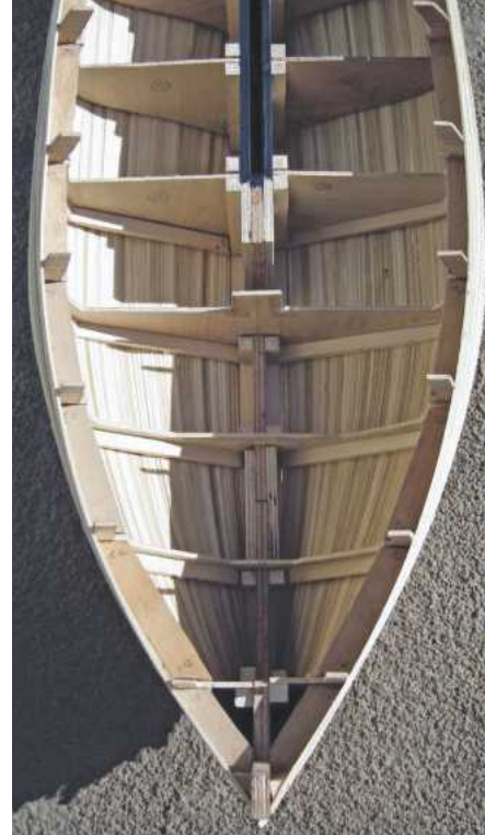
Hull interior, strip planked, from forward.
