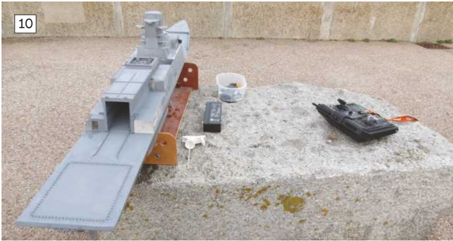
Photo 10: Preparing the last of the ballast trimming trials prior to final painting and assembly of the model.
