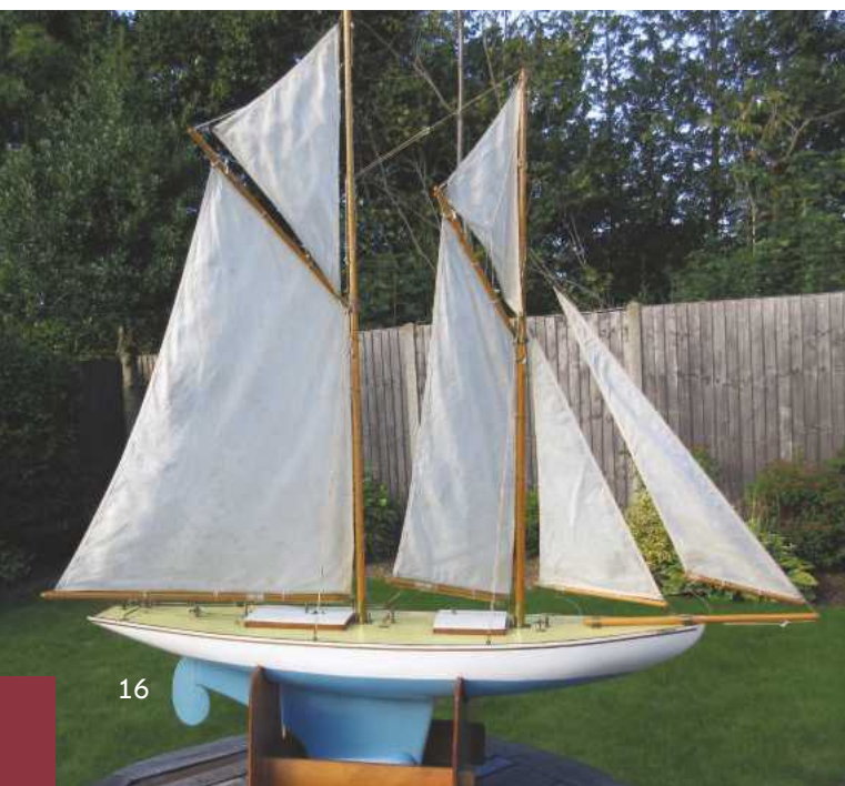
ABOVE: RC adaption showing pulley system for sails and rudder linkage - sail winch and rudder servo are under the deck (Image courtesy of R. Verden).
