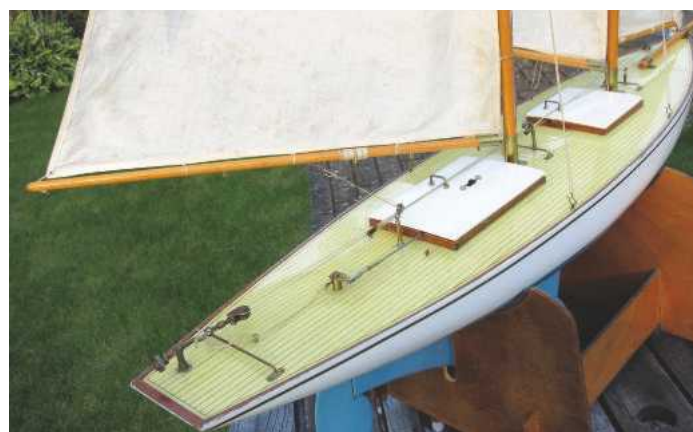
ABOVE: RC adaption showing pulley system for sails and rudder linkage - sail winch and rudder servo are under the deck (Image courtesy of R. Verden).
