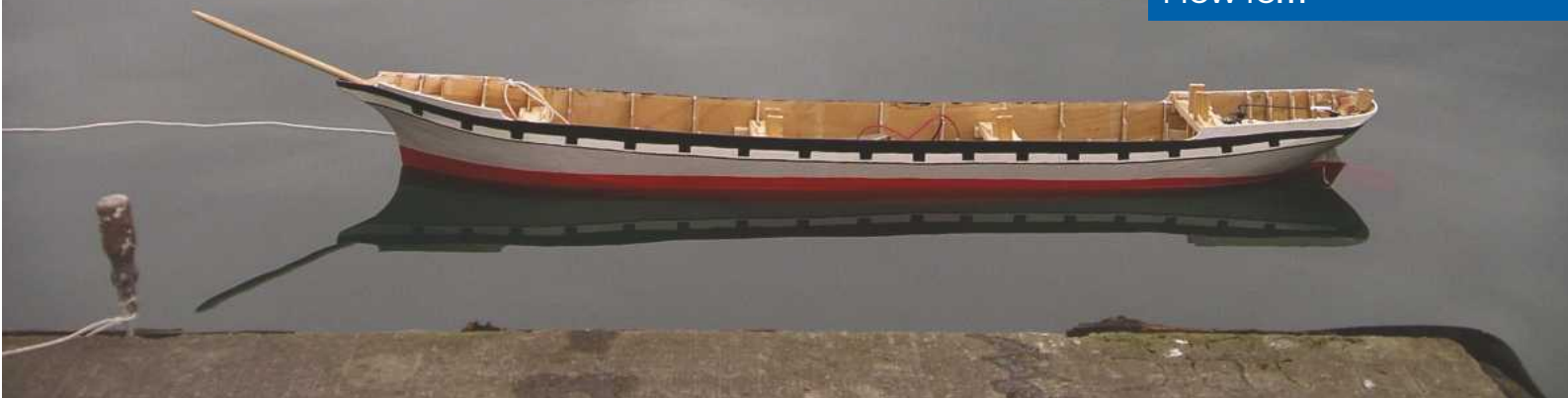
The 'Keeping a record' shot, in this case of a waterline test, taken so that you don't have to try and remember how the trim actually was when making adjustments at a later stage. It's a good example of how a photo taken on a 'point and shoot' type camera can be much improved with a little digital cropping on a PC.
