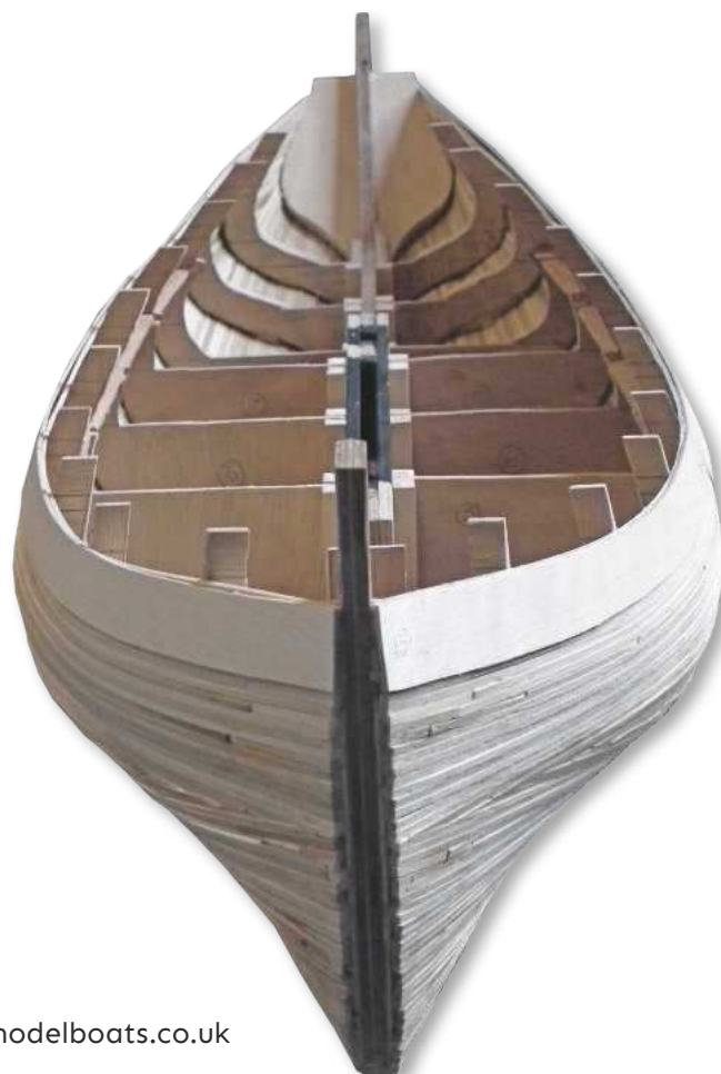
ABOVE: Strip planking at the stern.
