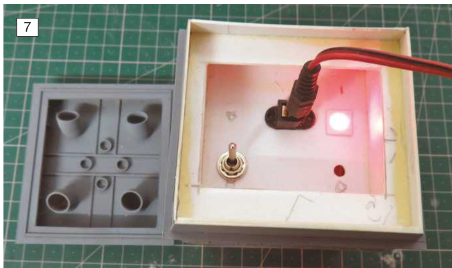
Photo 6: Both the hangar and funnel casing are still removable in this shot, and the top of the funnel and the inside are yet to be painted black. Photo 7: One useful and very practical method to avoid the need of constantly removing the battery for charging is to have the top of the funnel removable, with the charging socket, indicator light and power switch already located within. The only proviso is to ensure the battery compartment is well ventilated.
