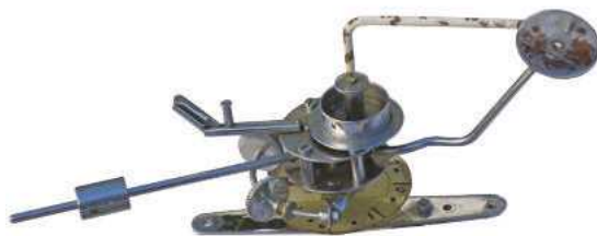
A typical vane gear (top) and some variations (Image courtesy of R. Verden/Model Maker).
