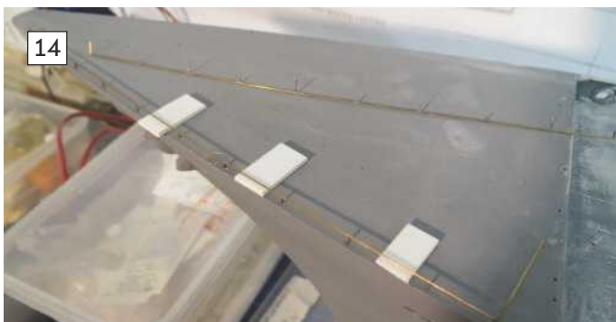
Photo 14: After a coat of primer, the safety rail is fixed into position with the help of spacers.
