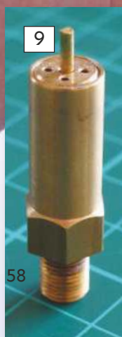
RIGHT: This valve is supplied with a Miniature Steam boiler and has a locking ring around the top plate. Once this is released, the plate can be rotated to adjust the pressure on the spring. It's a very neat and easy to adjust arrangement.
