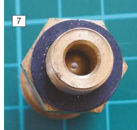
ABOVE LEFT: Still used today on such boilers as Mamod, Wilesco and Tony Green's boilers, these valves can almost be considered as disposable. The seat is an 'O' ring at the top, as found on the Cheddar type, but there is no means of adjusting the lifting pressure. ABOVE RIGHT: After a good clean up the ball bearing can be seen below this valve, held in place by the spring. A few drops of penetrating fluid will determine whether the seat is sealed effectively or not.
