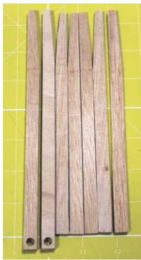
ABOVE: The ribs of the ramp structure: try to keep these items perpendicular to each other to ensure an aesthetically pleasing look to the finished ramp. BELOW: The basic structure of the ramp, complete with the resin bumper and triangle fitted to the wooden sheets.
