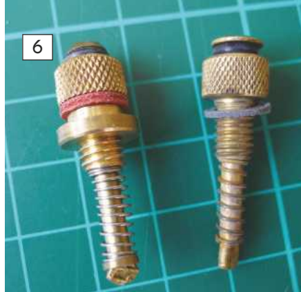
ABOVE LEFT: Still used today on such boilers as Mamod, Wilesco and Tony Green's boilers, these valves can almost be considered as disposable. The seat is an 'O' ring at the top, as found on the Cheddar type, but there is no means of adjusting the lifting pressure. ABOVE RIGHT: After a good clean up the ball bearing can be seen below this valve, held in place by the spring. A few drops of penetrating fluid will determine whether the seat is sealed effectively or not.
