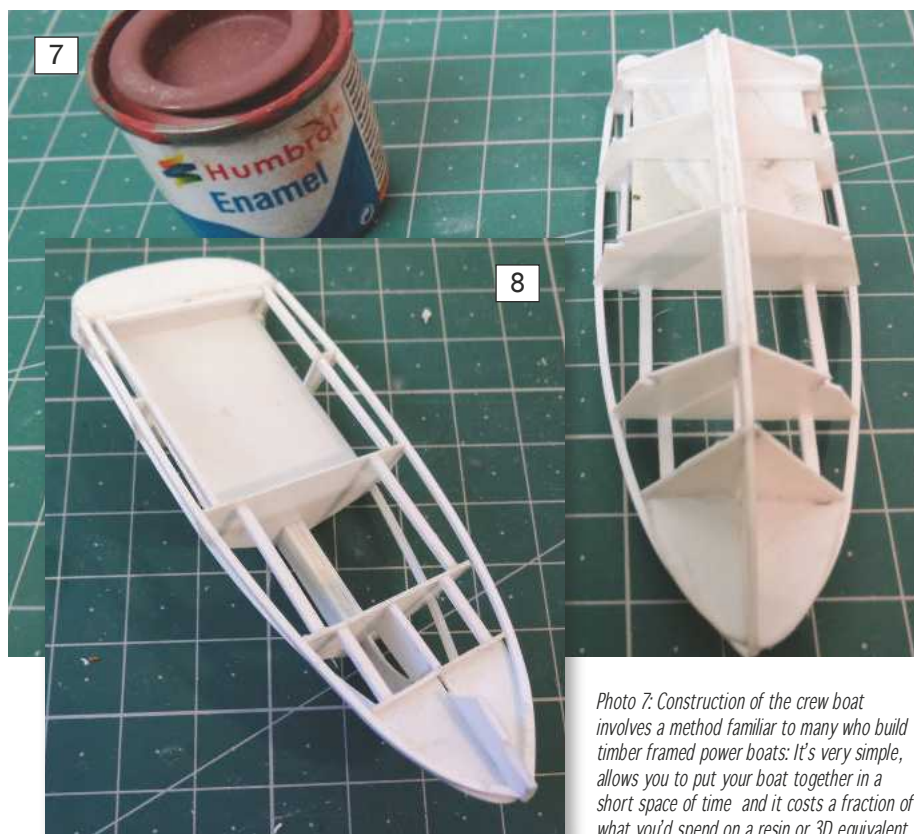
Photo 8: All the stringers from the chine to the gunwale are fixed into place using Evergreen box section.
