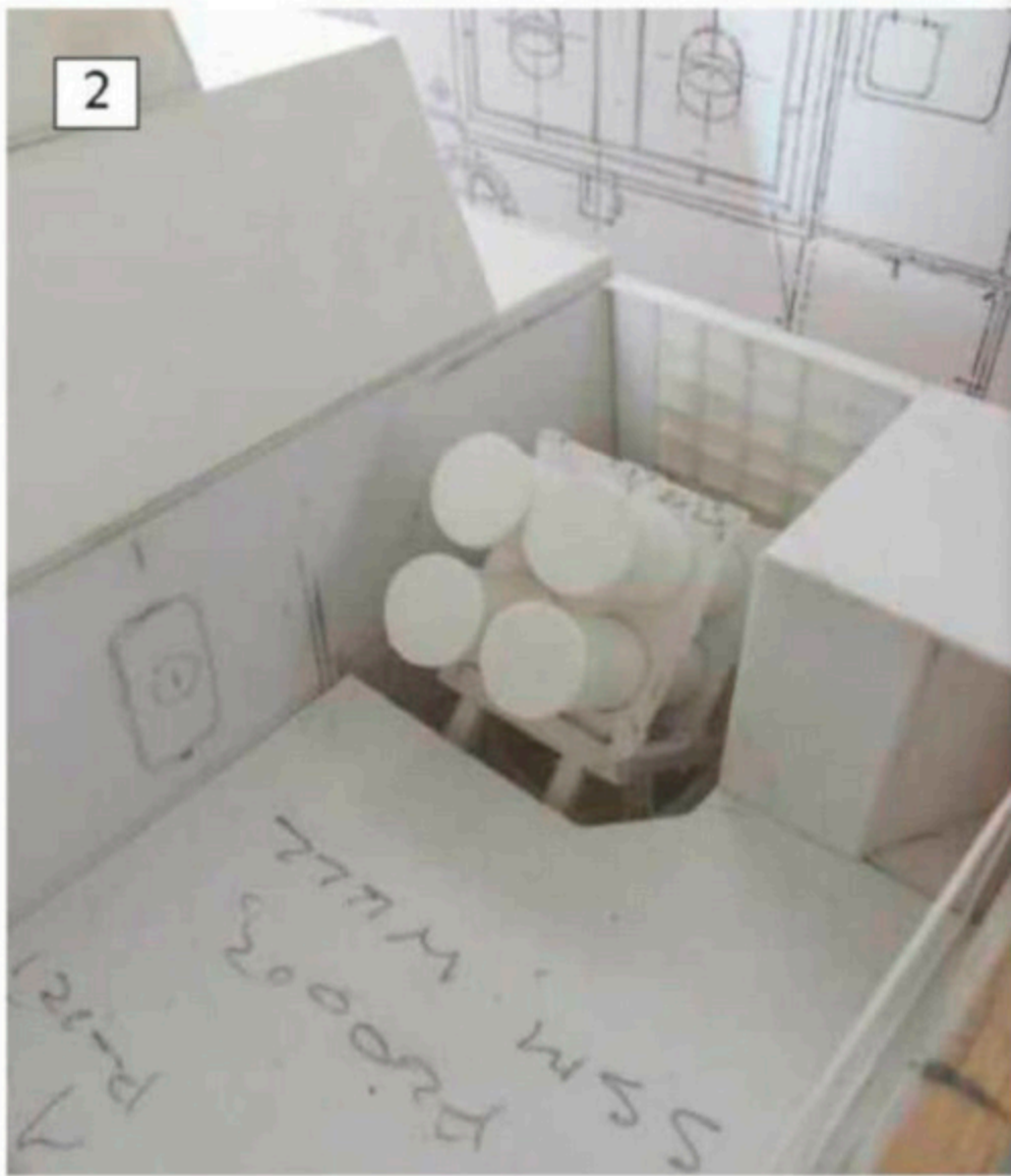
Photo 2: Provision for the SSM well during the initial construction of the superstructure.
