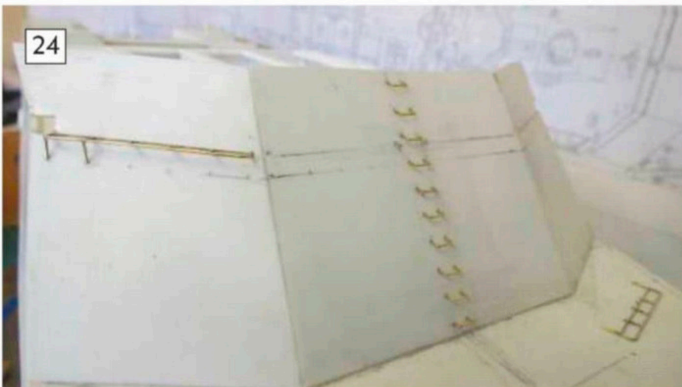
Photo 24: The remainder of the platforms can also be fitted now the rungs are. Photo 25: Platforms and rungs fixed into place. Photo 26: A reminder of the progress thus far.
