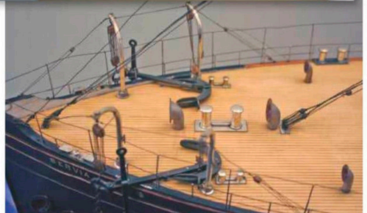
ABOVE: Cunard's famous liner Servia of 1881 featured fisherman type anchors with swivelled flukes handled by two sets of double davits. The hawseholes were right forward by the stem and presumably the windlass or capstan was under the foredeck.
