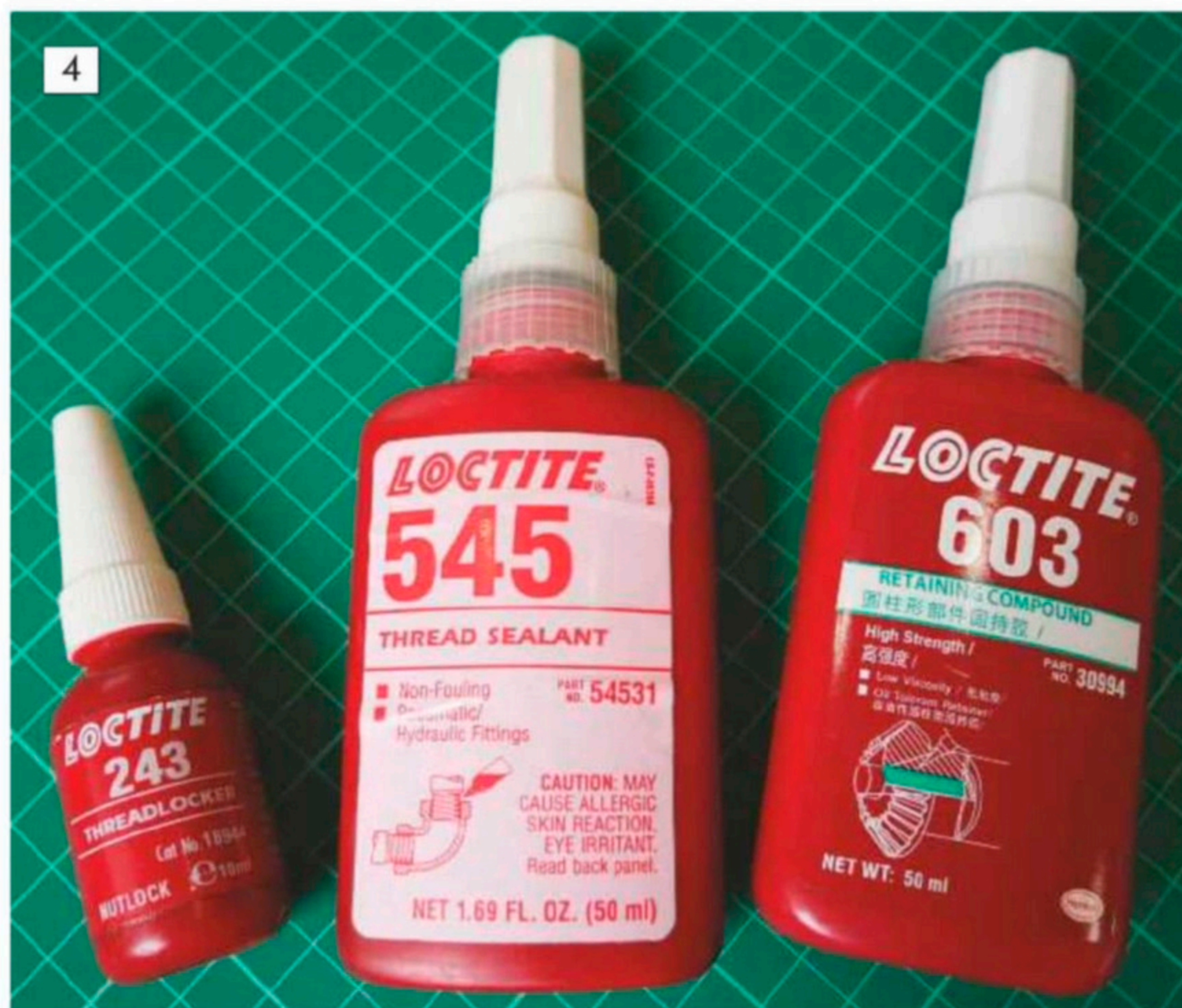
The Loctite range of products is huge, so great care has to be taken to buy the correct item. Shown here are: a hard setting retaining compound, mainly used for bearing and gear location; a thread locker, which is again a hard setting locking compound; and a hard setting thread sealant.
