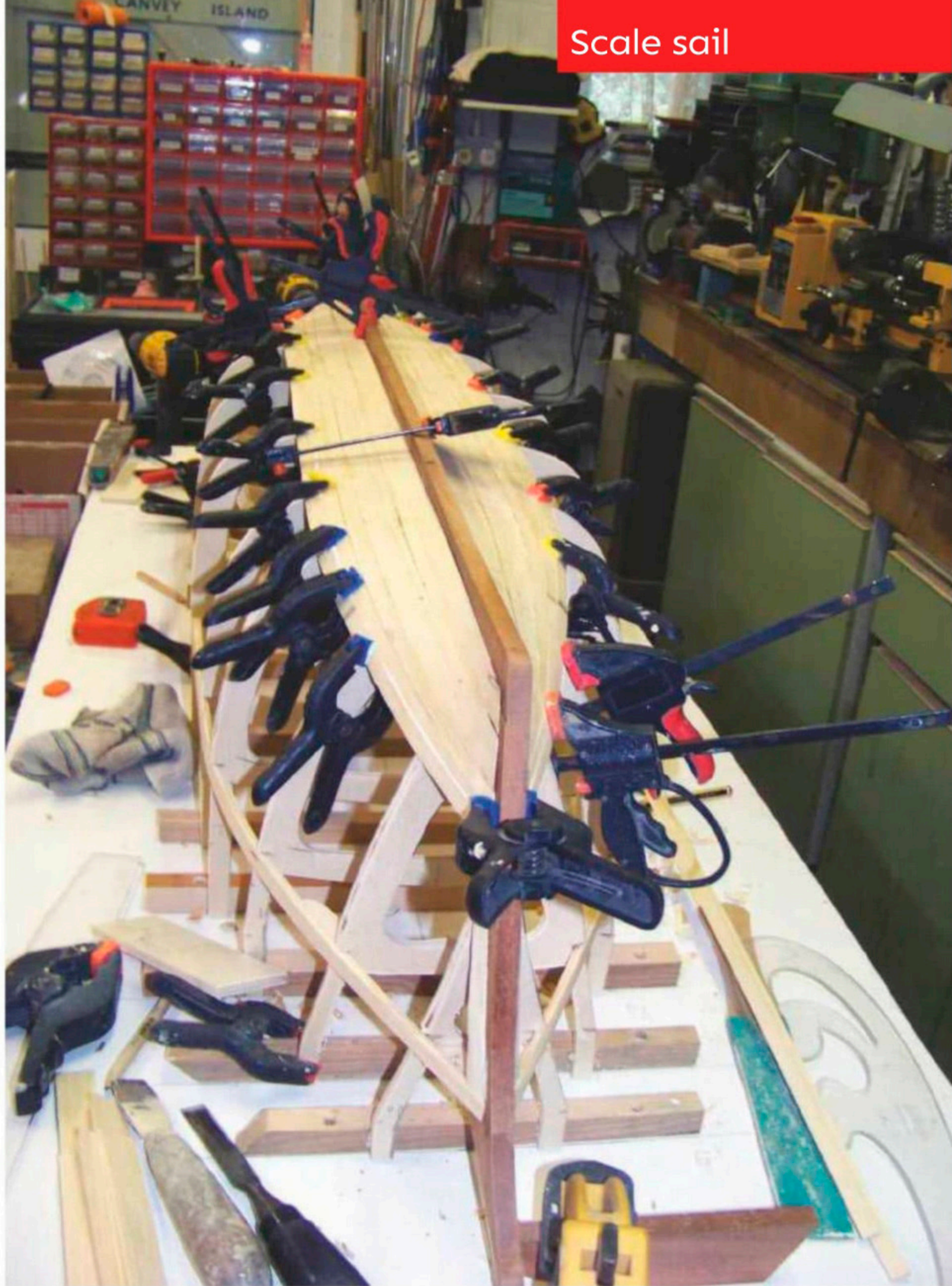
ABOVE: The first few planks glued in position.
