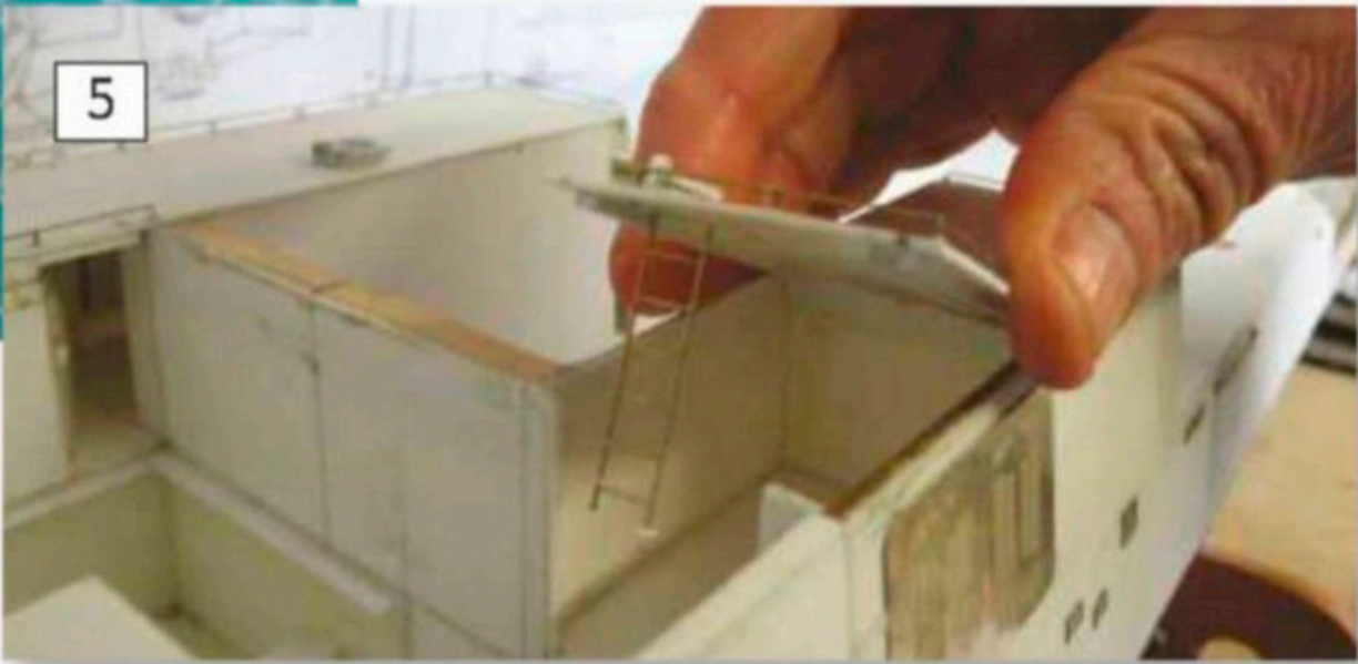
Photo 4: A fabricated ladder formed from 0.45mm brass wire.
