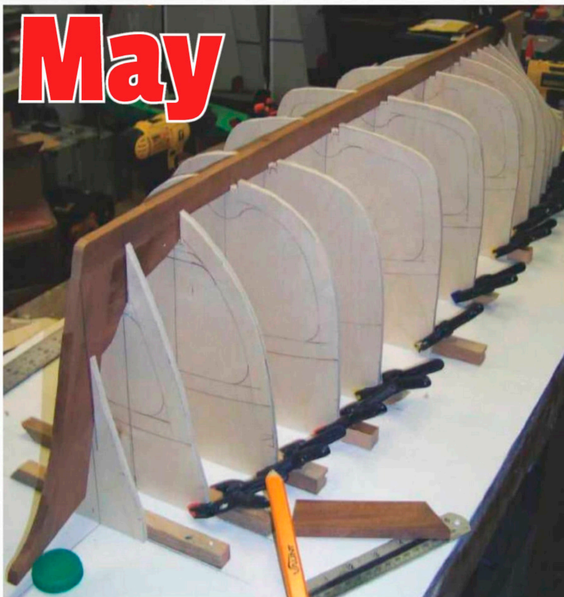
The frames and keel set up on building board.
