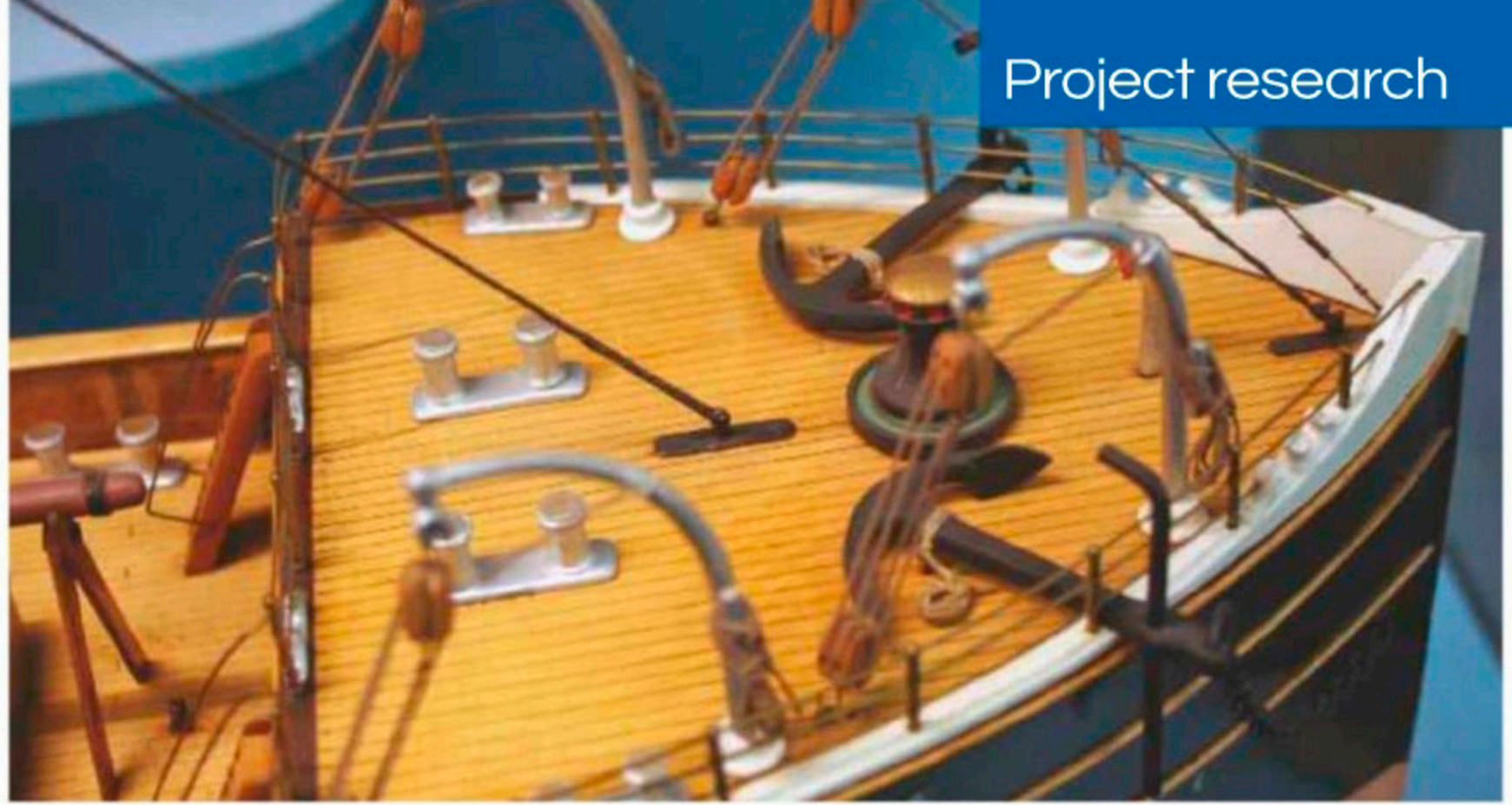
ABOVE: The anchors on the cargo vessel Iberia of 1881 were handled by two sets of double davits. The windlass, or maybe a capstan, was presumably housed under the raised foredeck.
