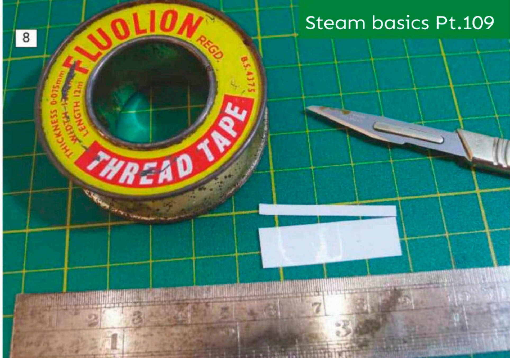
Using a sharp knife Richard trims off a suitable length, then cuts it to a width suited to the thread. You should not need more than two turns with enough of a tail to get hold of. When you pull the end off, this action should tighten the tape deep into the thread.
