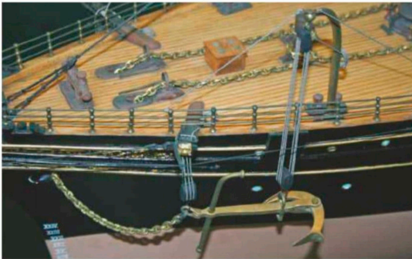
ABOVE LEFT: This interesting image shows a fisherman type anchor suspended from a small cathead and a davit. Close examination shows a plate on the hull, just in front of the davit, and a socket next to the cathead, indicating that the anchor would have been triced up against the ship's side, possibly with the stock folded. The multiple tackle would have assisted manual handling.
