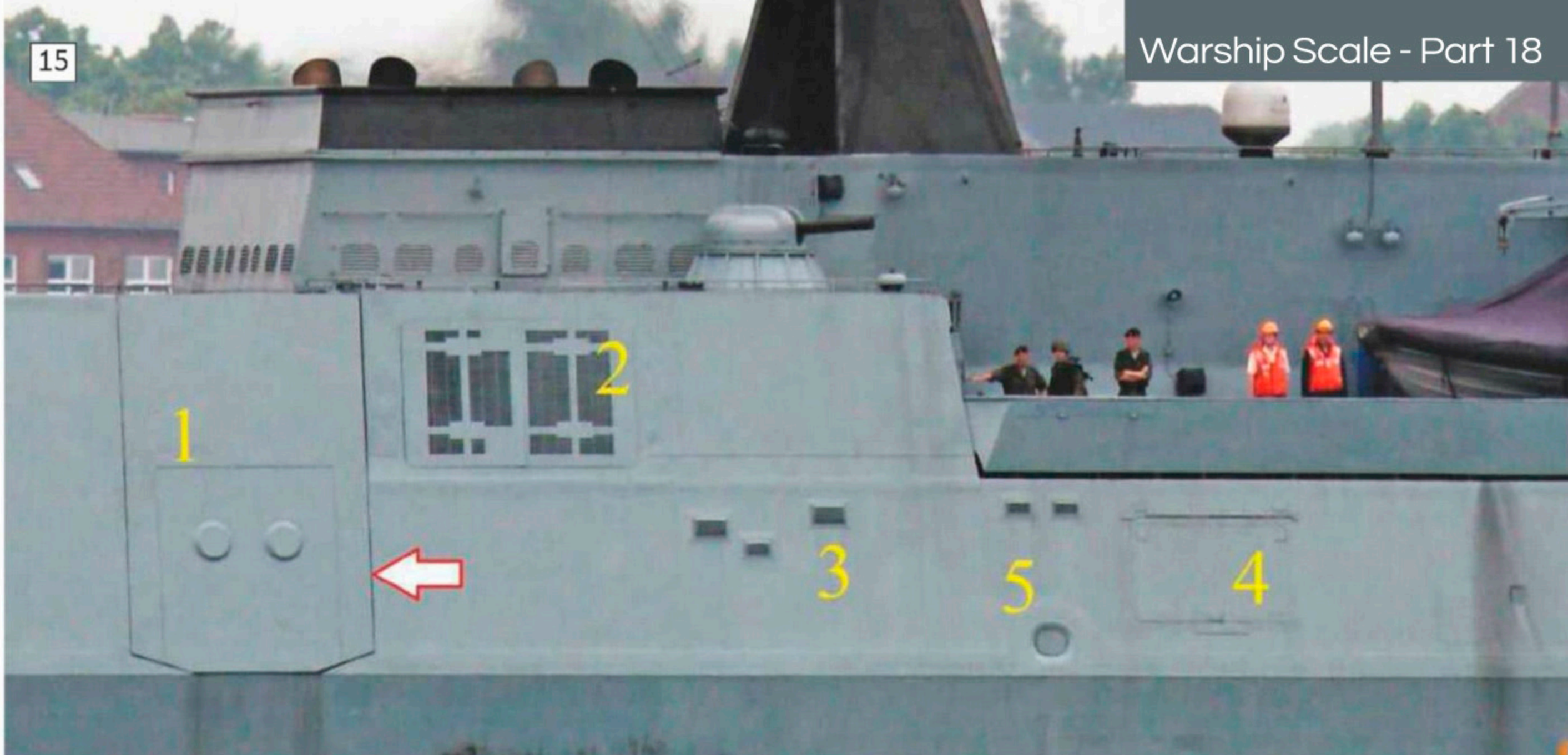
Photo 15: Fitted to each side of the superstructure are various flaps, vents and doors.
