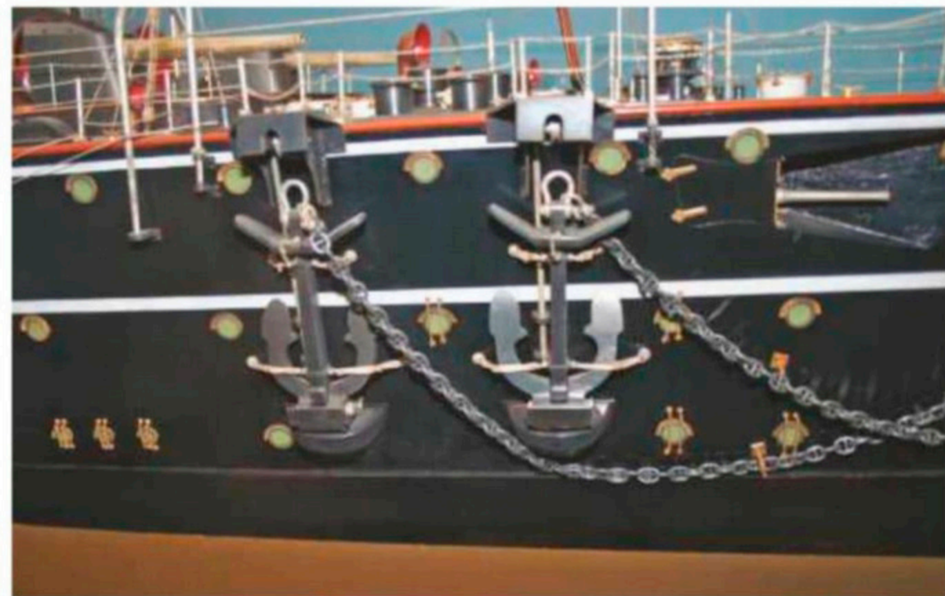
ABOVE LEFT: This interesting image shows a fisherman type anchor suspended from a small cathead and a davit. Close examination shows a plate on the hull, just in front of the davit, and a socket next to the cathead, indicating that the anchor would have been triced up against the ship's side, possibly with the stock folded. The multiple tackle would have assisted manual handling.
