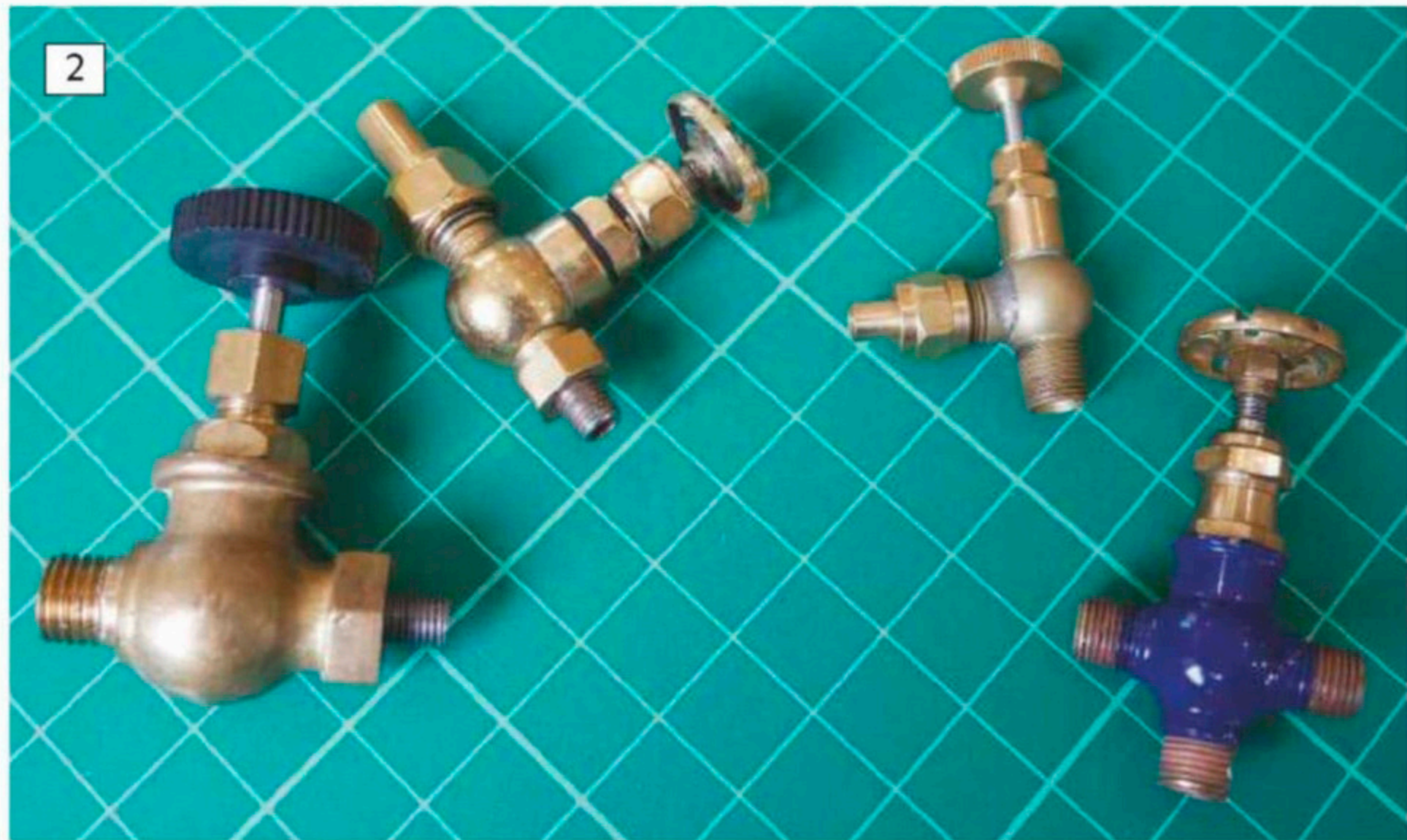
The two valves on the left both have a suitable flat surface on the mounting thread, so could be sealed with a sealing washer. The two on the right have only parallel threads so cannot be sealed with a sealing washer.
