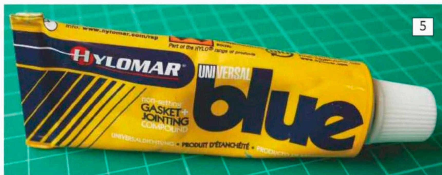
Hylomar has been used for many years and again can be bought in hard setting or soft setting compounds. The Blue Hylomar is a soft setting sealant and is excellent for thread and surface sealing.
