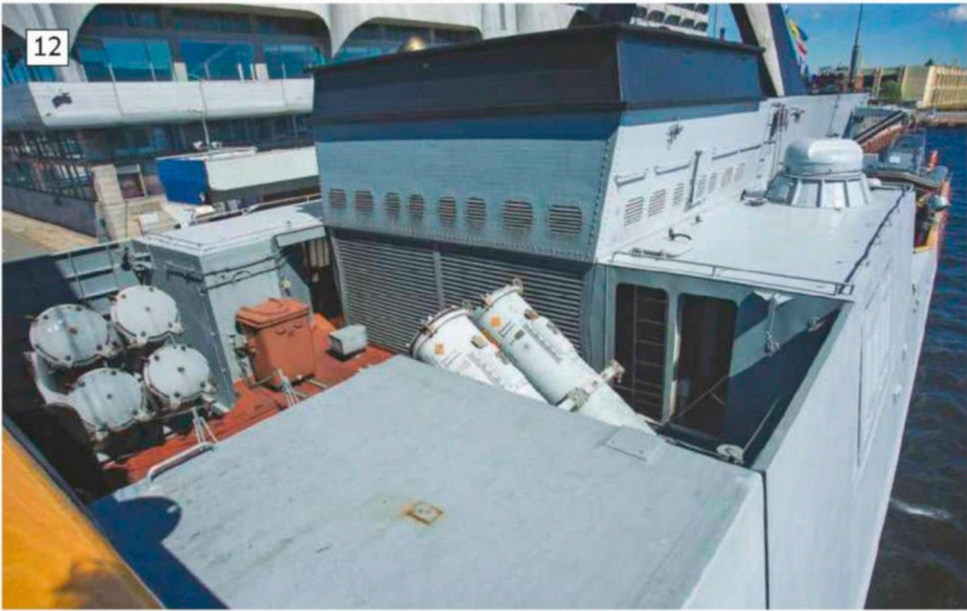
Photo 12: One of two brown storage containers within the SSM well; their purpose is unknown (an answer will be very welcome). Photo 13: A small tray provides a firm and accurate seating for the SSM launch cradle.
