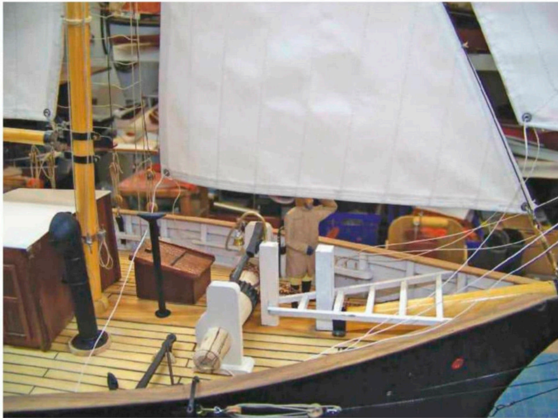
ABOVE: The skipper at the wheelhouse door, steering from the side, sailing ship style. BELOW: The fore deck with anchor winch.
