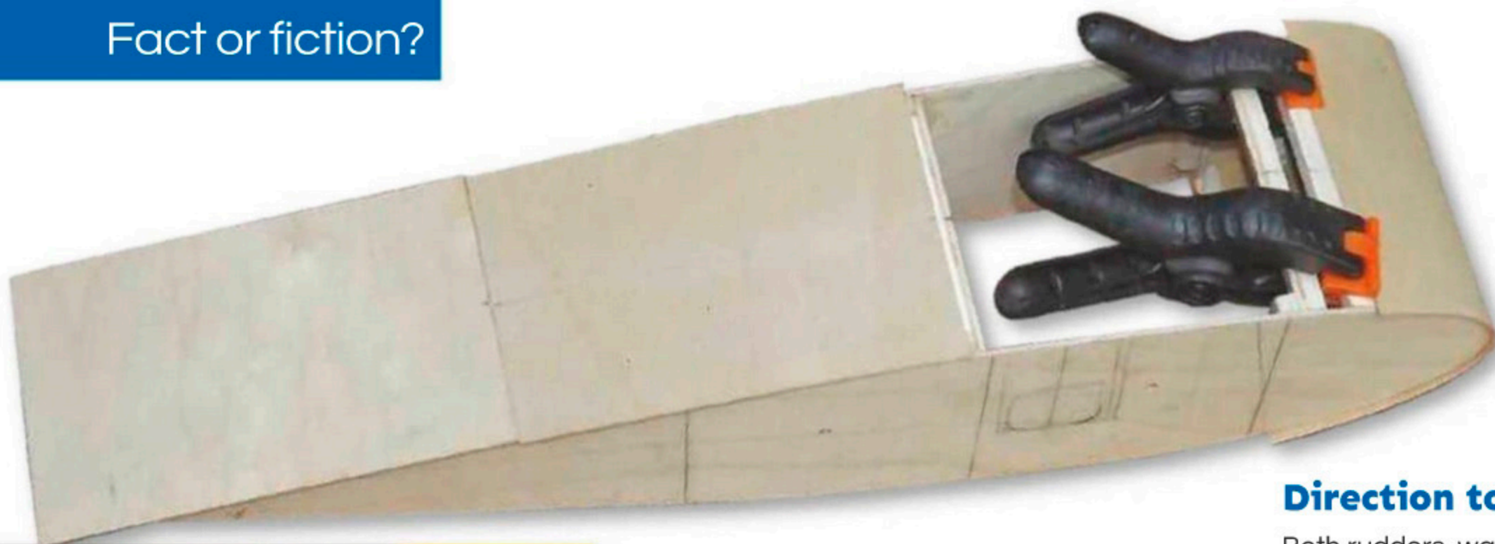
ABOVE: Skinning the hull (shown here upside down) begins.
