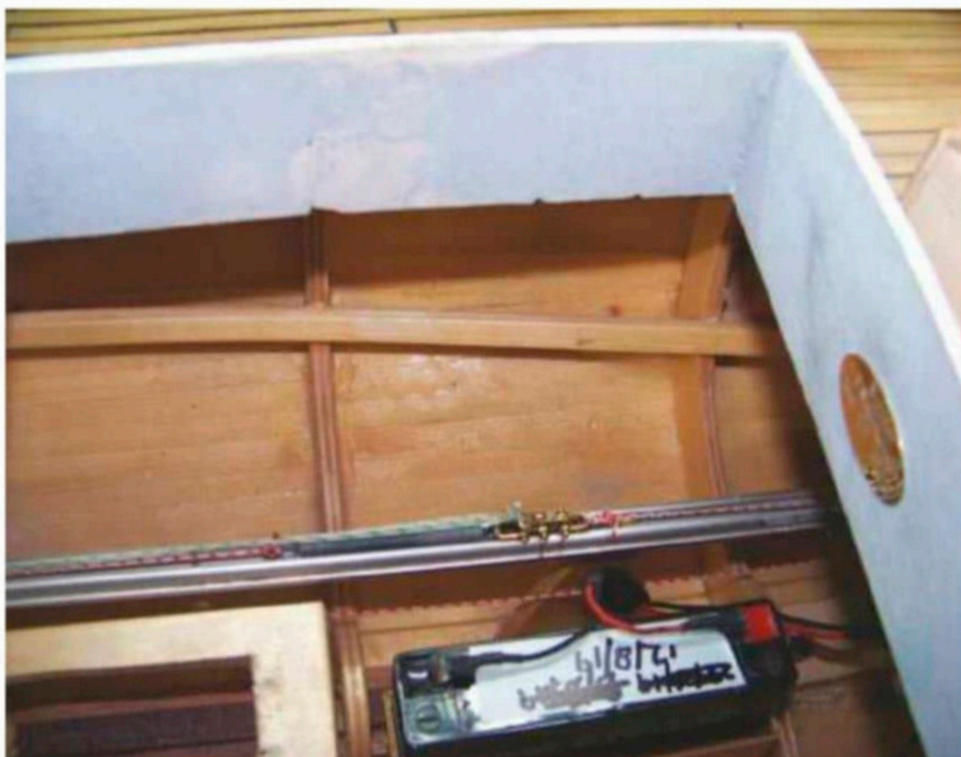
ABOVE LEFT: The brass traveller in a curtain track under fore hatch. ABOVE RIGHT: The rotary winch below lever arm servo for the yards.
