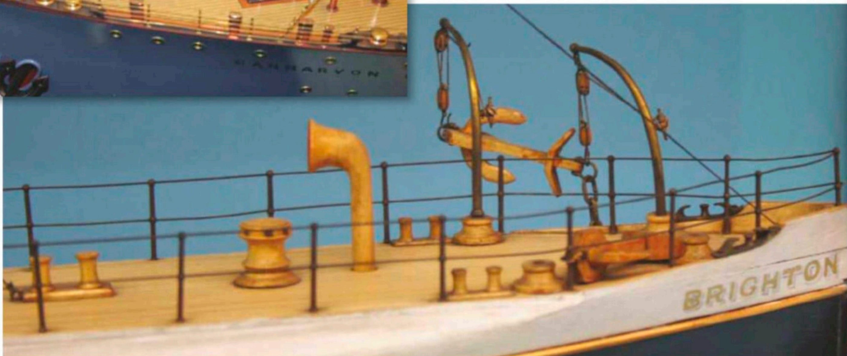
BELOW: This simple model of the cross channel paddle steamer Brighton of 1878 shows how two davits were used to manage the anchor.
