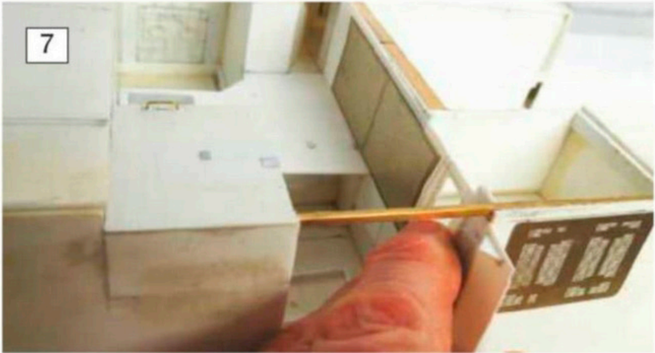
Photo 6: Here the platform deck over the well is eased into place. Photo 7: Louvre vent housing eased into its location, but not fixed. Photo 8: Cleaning up the joints of the well deck railings. Photo 9: Locating the strip of rail into the platform deck.
