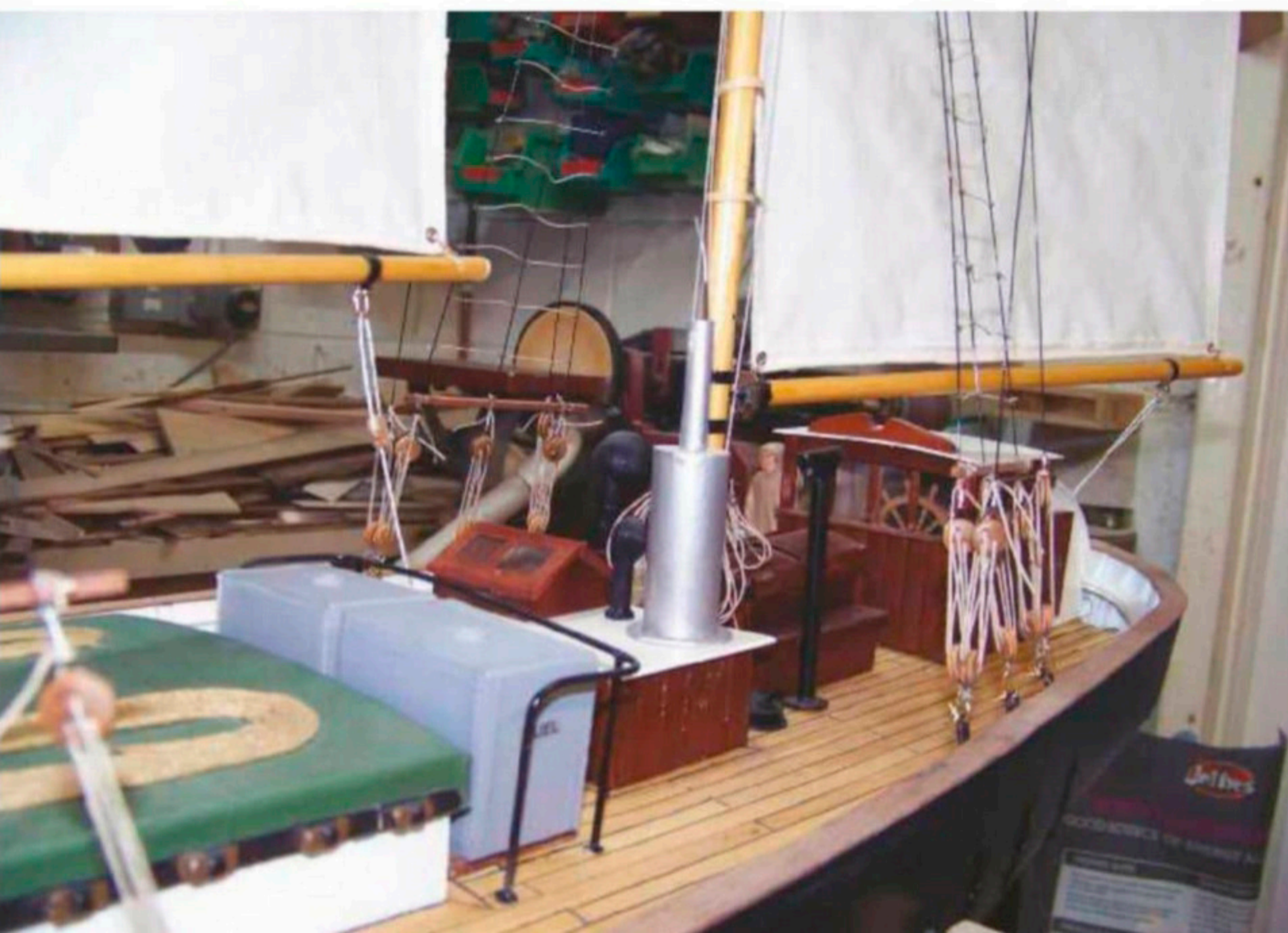
ABOVE: The fore cargo hatch with ship's boat. BELOW: Deck detail, with engine hatch and exhaust stack.
