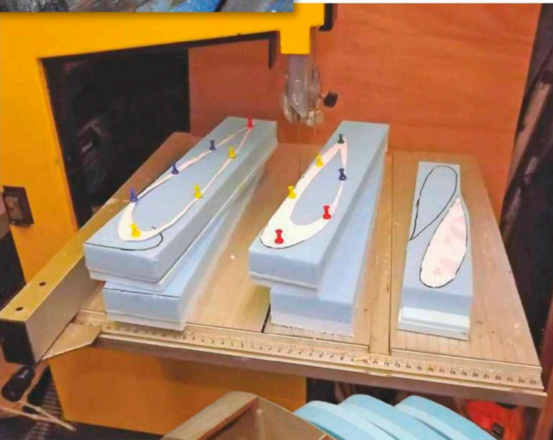
ABOVE: The wings ready to be cut from slabs of foam.
