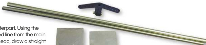
The rudder components which our reviewer, Nick, used; the tiller arm is a commercial item available from many a good model store.
