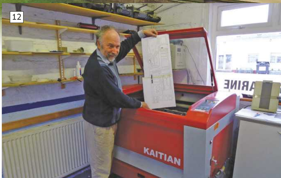
Ron showing how effective the laser printer is. He also uses this to produce card prints of model parts so that he can check the feasibility of a kit in development before its put into production.
