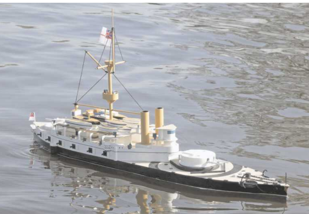
At rest you can see a slight bow-up attitude, which corrects to level running when under way.
