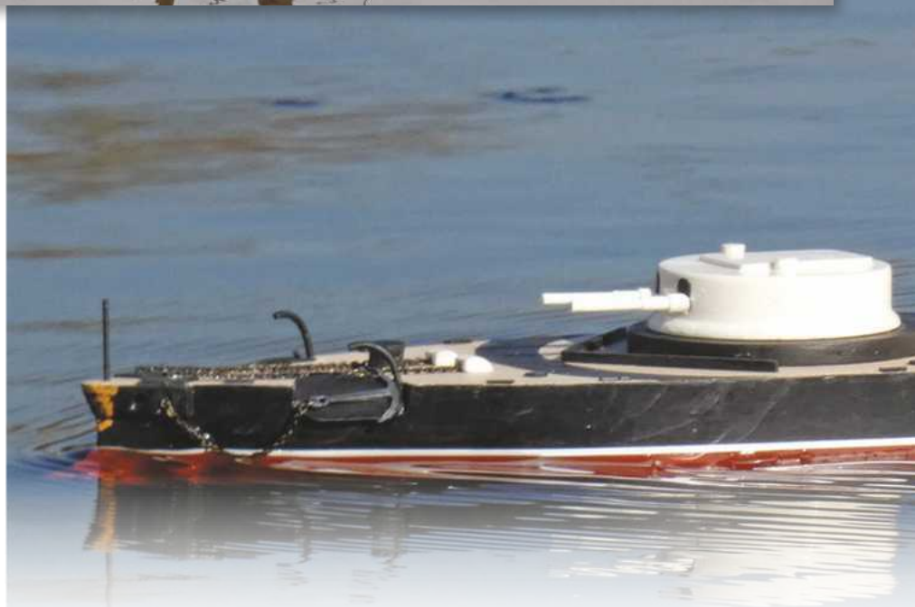
BELOW: Ballast had to be added to get the low freeboard look.
