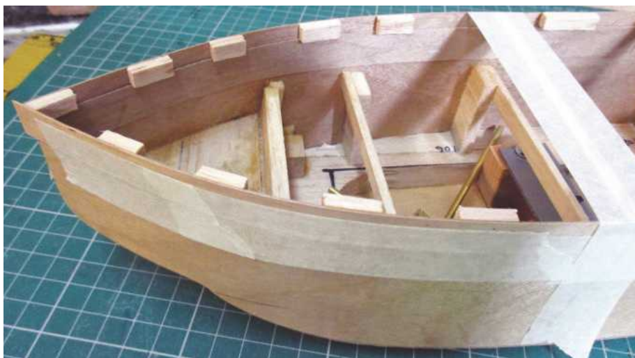
LEFT: Motor in clamp mount. Notice the coaming for the rear superstructure block. BELOW: Making the superstructure plug. Balsa blocks on the sides were used to set it to correct height.
