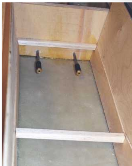
ABOVE: The left over 1/2 inch balsa used to create deck beams.
