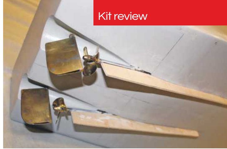
ABOVE & BELOW: The completed running and steering components shown from different angles.
