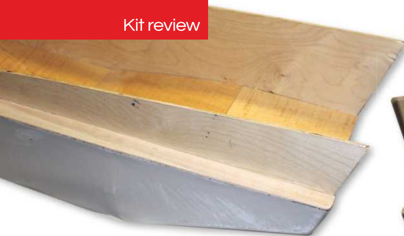
LEFT: The tank well sides and surrounding deck fitted.
