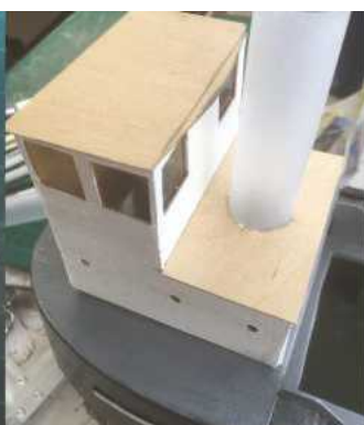
ABOVE LEFT: Testing the electronics before final fitment. ABOVE RIGHT: Slightly different designs for the rowing boats. One made from 0.08mm ply and the other is paper stiffened with PVA glue on a ply framework. Oars were made from cocktail sticks. BELOW LEFT: Constructing a wheelhouse from 0.08mm ply. A piece of scrap plastic tubing was used for the funnels. BELOW RIGHT: Two slightly different designs for the wheelhouses. Both models have working navigation lights.
