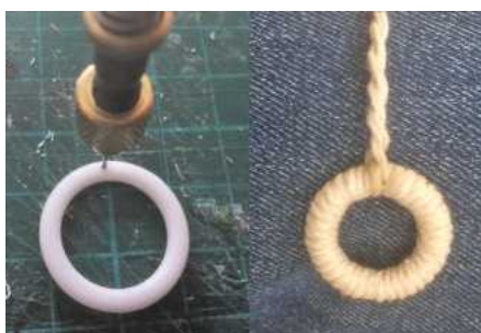
ABOVE: The side fenders were made from plastic curtain rings bound with twine. Other fenders were made using the Kumihimo Japanese weaving method.
