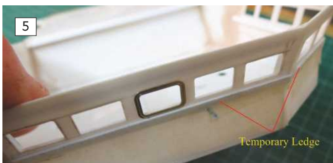
5: A temporary ledge is fitted to maintain the symmetry of fix for the window surrounds. 6: No fuss all the PE surrounds are accurately aligned. 7: With the surrounds firmly in place the temporary ledge can be removed.
