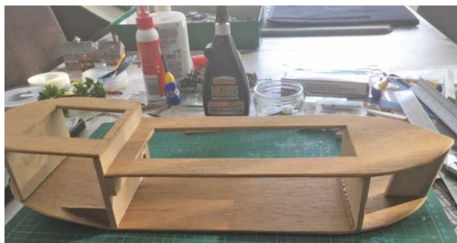
The hulls were constructed from scrap plywood.
