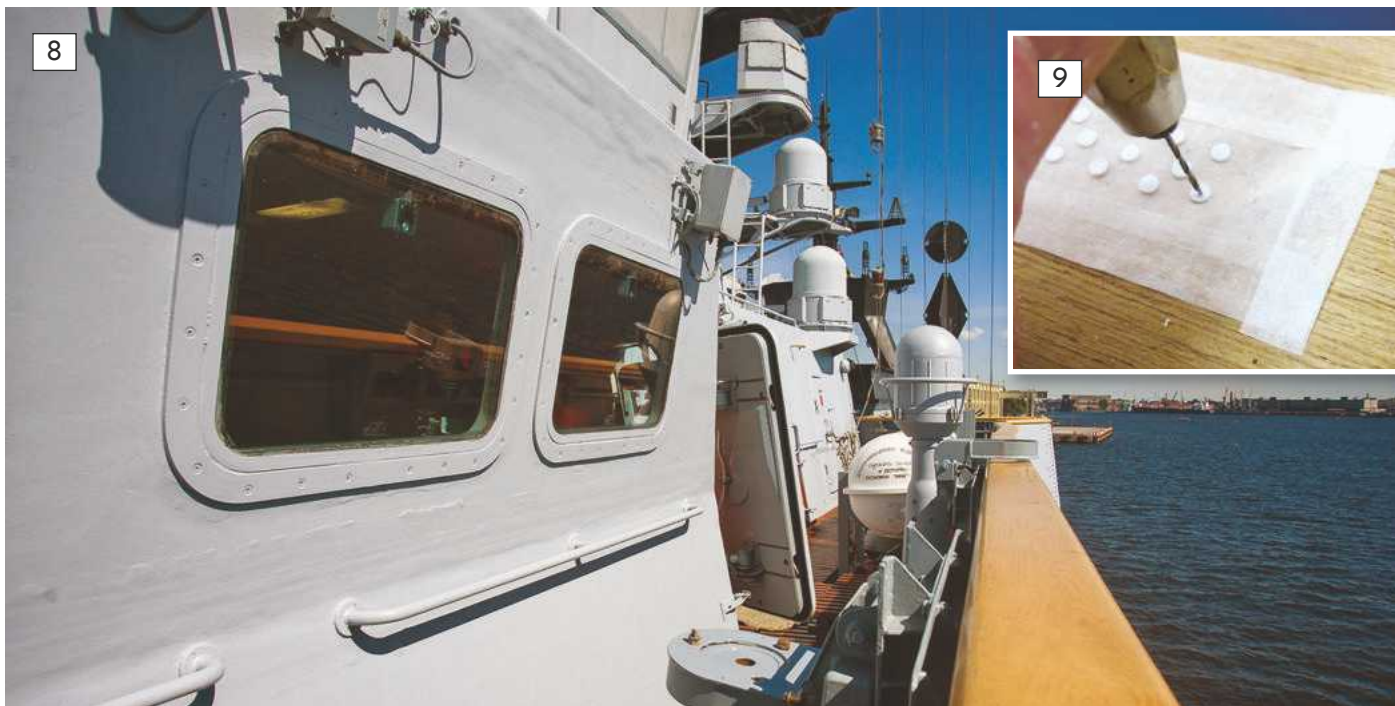
8: Here on Stoiky as on Soobrazitelnyy the handrail is positioned beneath the bridge windows. 9: Using a pin vice to drill out styrene handrail fixing plates.
