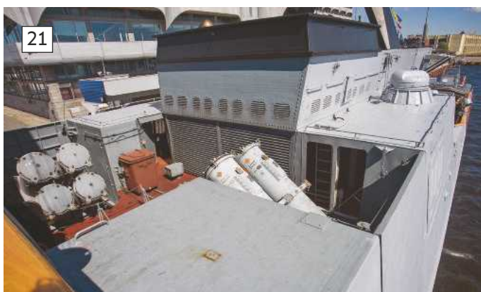
19: All the wipers fixed into position. 20 Progress thus far. The bridge area with fittings temporarily added for effect. 21: A view of the detail on Stoiky showing vents and louvre grills at the rear of the funnel casing. 22: Photo-etch vents and louver grills fitted to the rear of the funnel casing.
