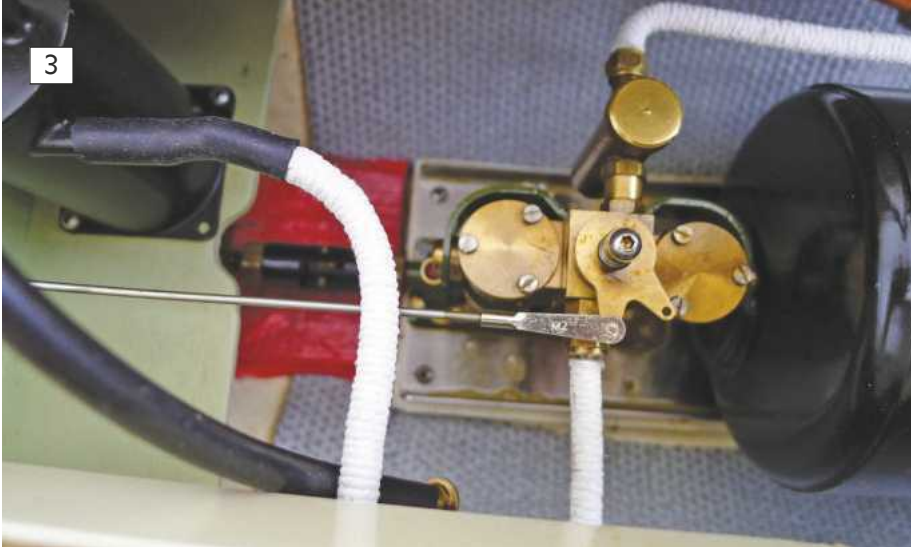
3: A Stuart Models twin oscillator provides more than enough power and, being carefully set up and looked after, does not leak too much from the port or the control valve faces.
