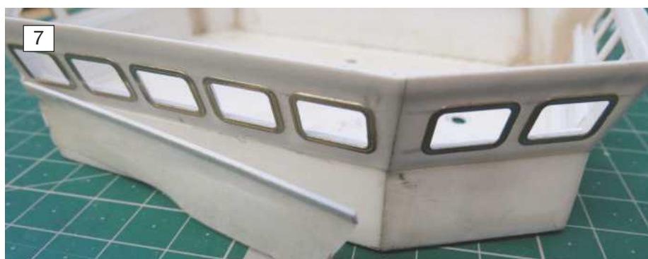
5: A temporary ledge is fitted to maintain the symmetry of fix for the window surrounds. 6: No fuss all the PE surrounds are accurately aligned. 7: With the surrounds firmly in place the temporary ledge can be removed.
