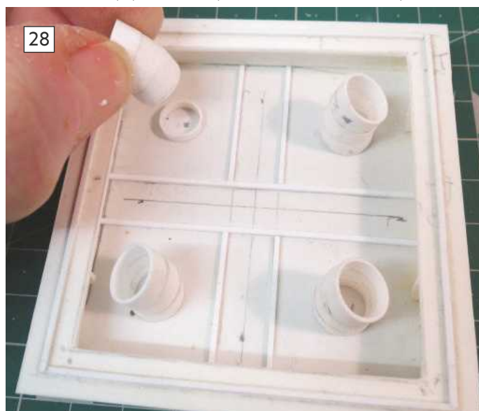
28: Each funnel exhaust is fitted to its centring ring where it can be adjusted to suit. 29: A further four smaller rings are added. 30: Fitting out the funnel is almost complete.
