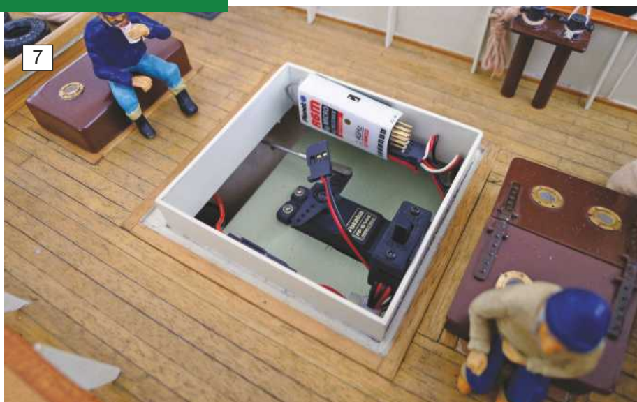
7: Although electronics are not in a separate sealed compartment they are away from heat and humidity and easily accessed via their own hatch.
