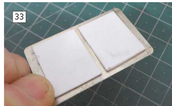
33: Adding a styrene backing to provide a snug fit.
