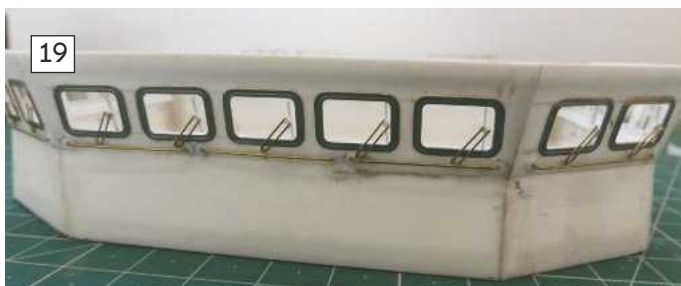
19: All the wipers fixed into position. 20 Progress thus far. The bridge area with fittings temporarily added for effect. 21: A view of the detail on Stoiky showing vents and louvre grills at the rear of the funnel casing. 22: Photo-etch vents and louver grills fitted to the rear of the funnel casing.
