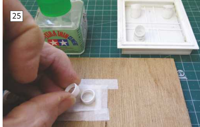
25: Assembling each of the segment rings that will form the slightly curved exhaust.
