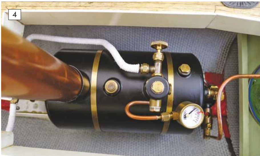
4: The Stuart Models boiler paired with the engine fits into the hull with space to spare and provides enough steam for around 20 minutes on the water between fills.
