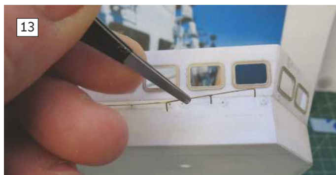
10: Prepared styrene fixing plates. 11: Preparing each of the bridge hand rails. 12: Reducing the thickness of the styrene fixing plates. 13: Positioning the starboard side bridge handrails into the fixing plates.
