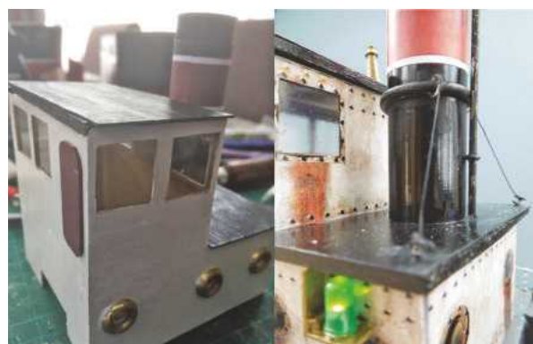
ABOVE LEFT: Testing the electronics before final fitment. ABOVE RIGHT: Slightly different designs for the rowing boats. One made from 0.08mm ply and the other is paper stiffened with PVA glue on a ply framework. Oars were made from cocktail sticks. BELOW LEFT: Constructing a wheelhouse from 0.08mm ply. A piece of scrap plastic tubing was used for the funnels. BELOW RIGHT: Two slightly different designs for the wheelhouses. Both models have working navigation lights.
