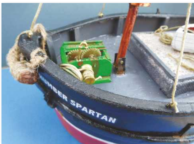
LEFT: Winches were made from spare cogs from old clocks and bits of balsa wood.
