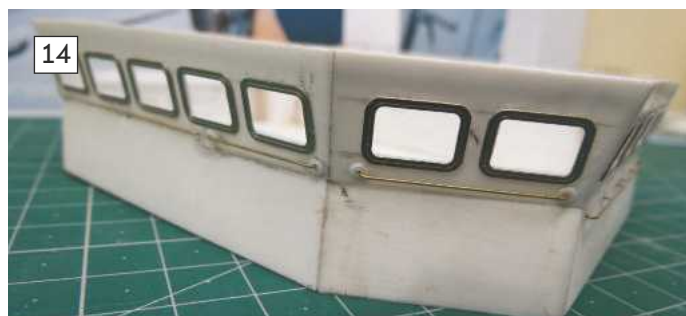
14: Bridge handrails fixed. 15: Handrails are extended aft of the bridge. 16: The bridge frontage on Soobrazitelnyy showing the positioning of the windscreen wipers.
