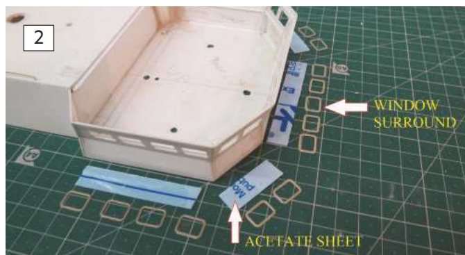
1: The photo-etch containing vent panels and window surrounds. 2: Preparing the acetate glazing and photo-etch window surrounds.
