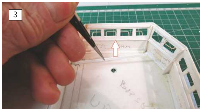
3: Completing the slot for the acetate glazing. 4: No adhesive required the acetate glazing is firmly held in place.
