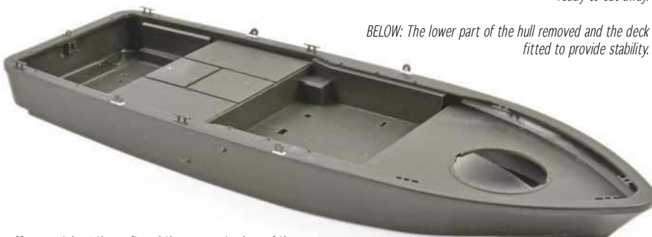
BELOW: Cleats and lifting points added to the gunwales, note the filler added around the lifting brackets.
