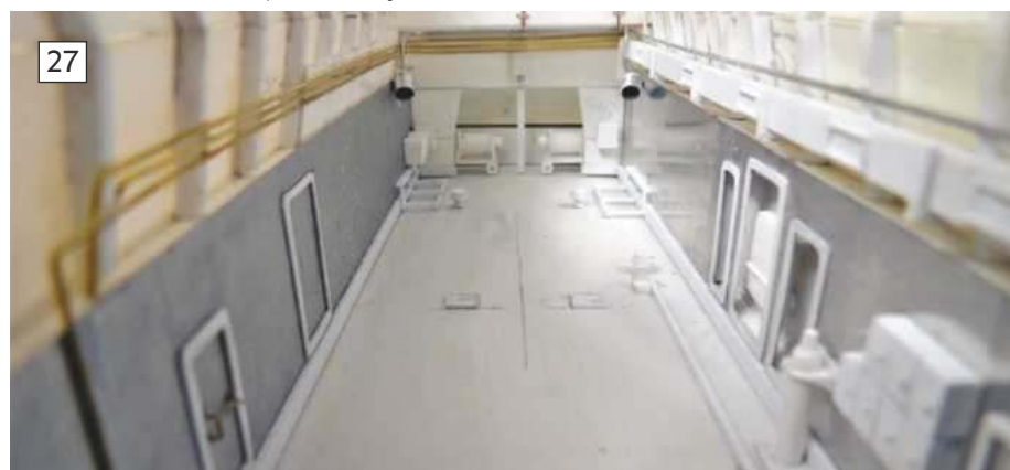
26: Returning the hangar module to the superstructure. 27: Viewing the floor of the hangar showing the guide track, wheel chock, haul in sheaves and helicopter wheel troughs.
