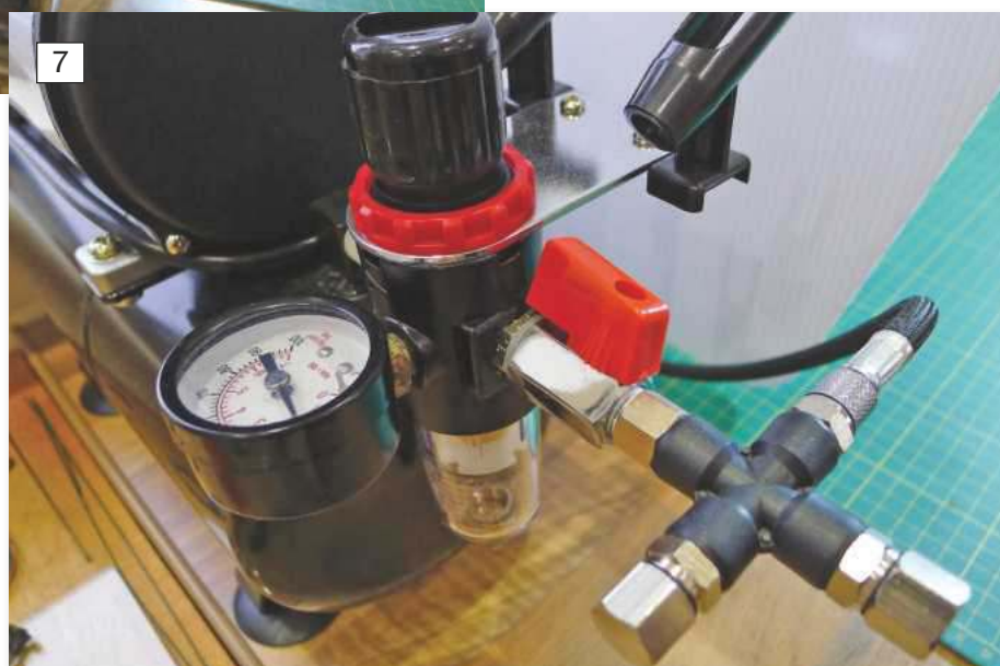
7: I added the little manifold to enable more than one air brush to be connected at a time and, with it being on the workbench next to me, pressure adjustments are very easy and convenient. 8: These little compressors are very handy for situations where you want complete portability such as for railway layout scenery or where the subject cannot be moved easily.
