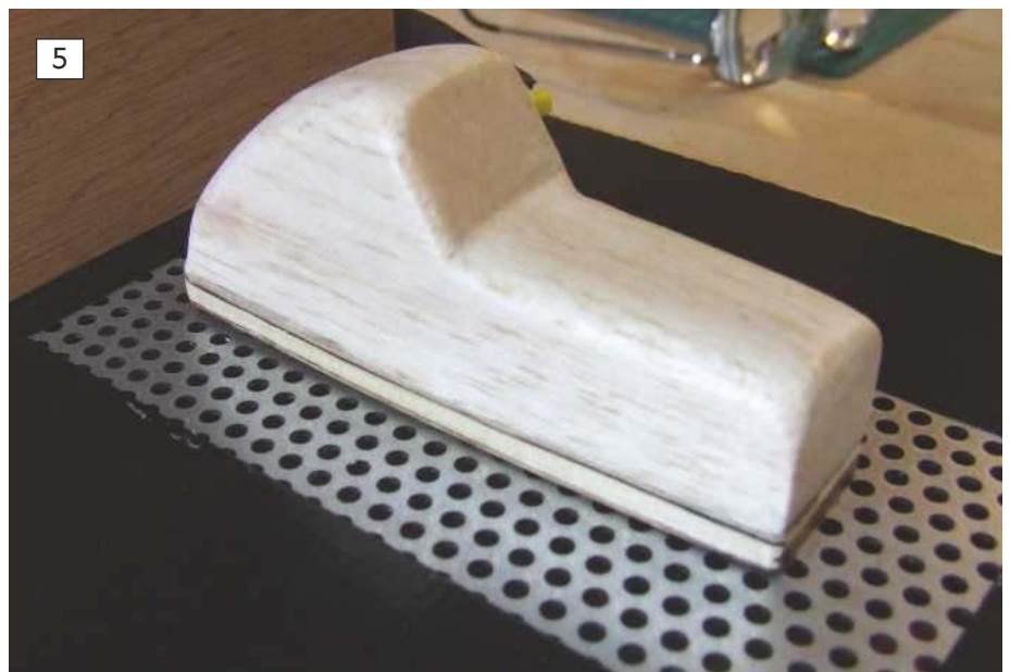
5: Shows a plug secured to the vacuum grill. 6: The kit in use. 7: The tool to remove moulded items from plug.
