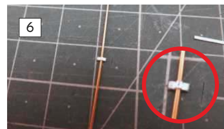
6: The cable strap formed round the copper wire and cut to size.
