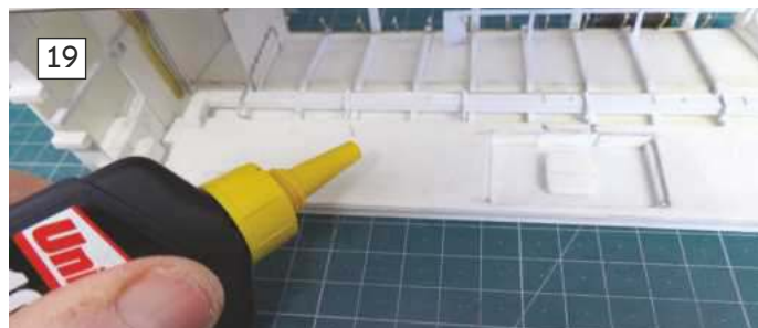
19: Carefully applying Uni-Bond Power Glue to the surface. 20: Using a spatula the Power Glue is spread evenly and thinly over the area of the lower hangar side wall. 21: The Litho plate panel is returned with time to adjust its positioning, weights are then added.
