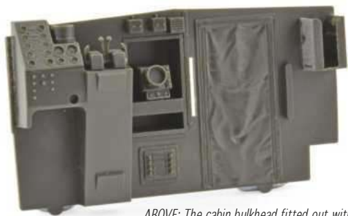
ABOVE: The cabin bulkhead fitted out with instrument panel, throttles and radar scope. The elongated protrusion where the fire extinguisher fits is easily seen to the right of the door curtain.
