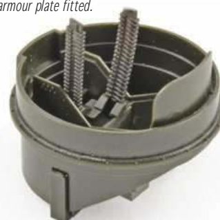
ABOVE: The rubberised flexible ammunition feed belts fitted in place. BELOW: The .50cal mounts fitted along with the gunners search light, the clear part will be left out until after the painting has been completed.
