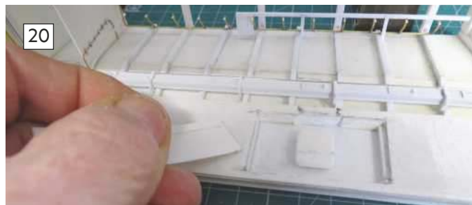
19: Carefully applying Uni-Bond Power Glue to the surface. 20: Using a spatula the Power Glue is spread evenly and thinly over the area of the lower hangar side wall. 21: The Litho plate panel is returned with time to adjust its positioning, weights are then added.
