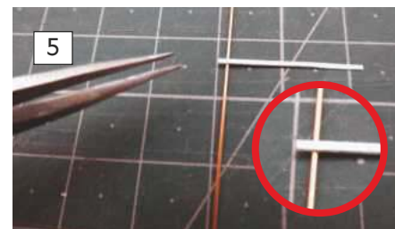
5: Copper wire for simulating electrical cable tracks, including an aluminium strip for cable straps.
