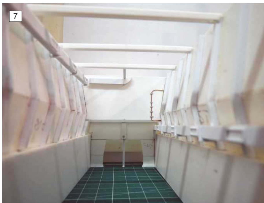
7: Fitting out the hangar, cable run and straps can be seen at the far end of the hangar.
