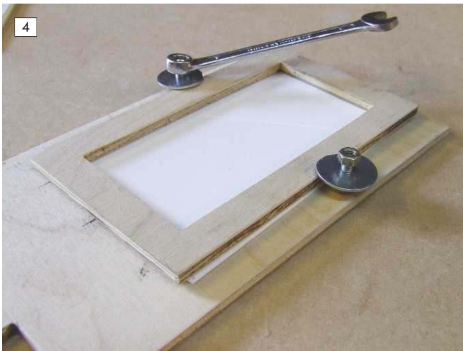
4: The material holder clamp system.
