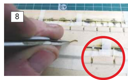
8: Preparing .8mm brass wire to simulate the sprinkler system using a jig in preparation for soldering.
