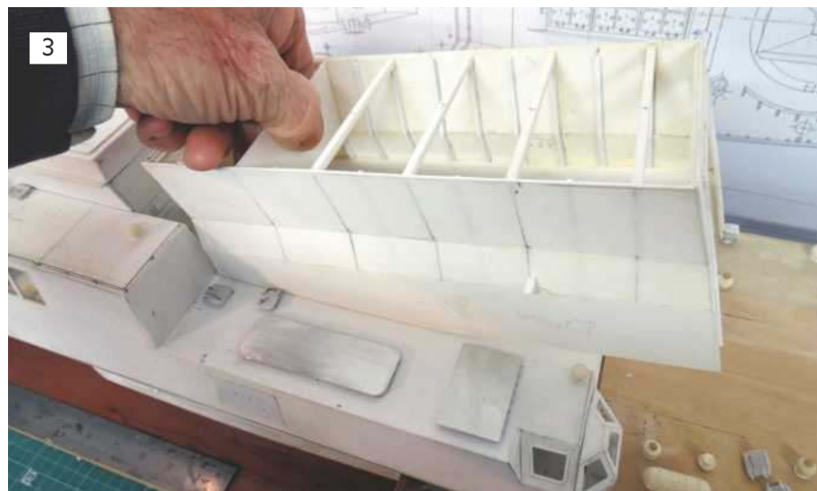
3: Preparing to undertake internal detailing with the hangar module easily withdrawn from within the superstructure.
