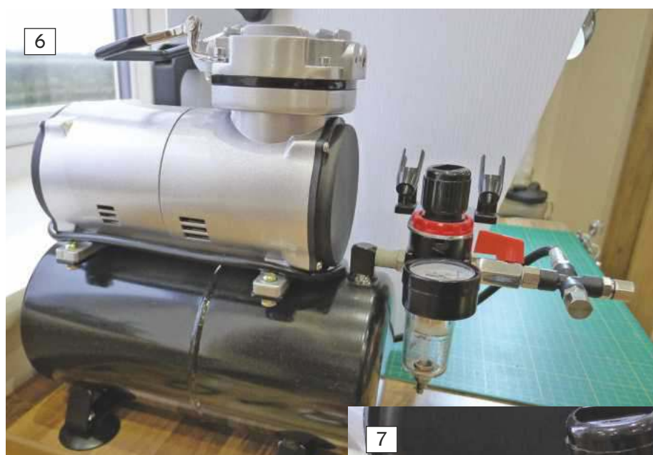
6: Although part of a complete set the two air brushes were immediately disposed of. The compressor is small and compact with a quiet unit on top and a neat built in pressure regulator and drier unit.
