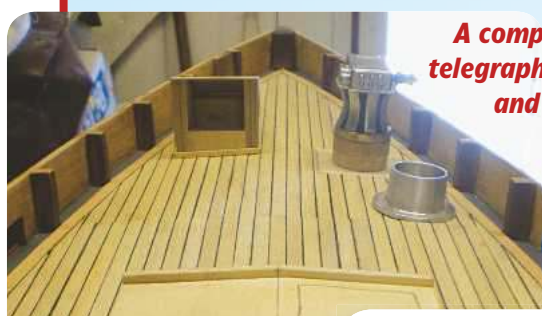
View showing the first deck planking
