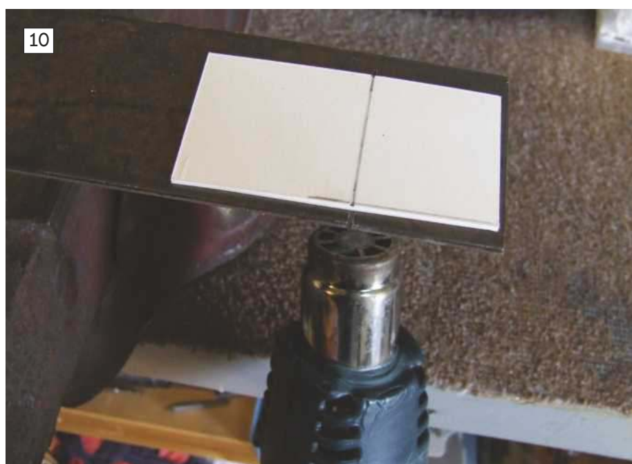
10: Heating material from below.
