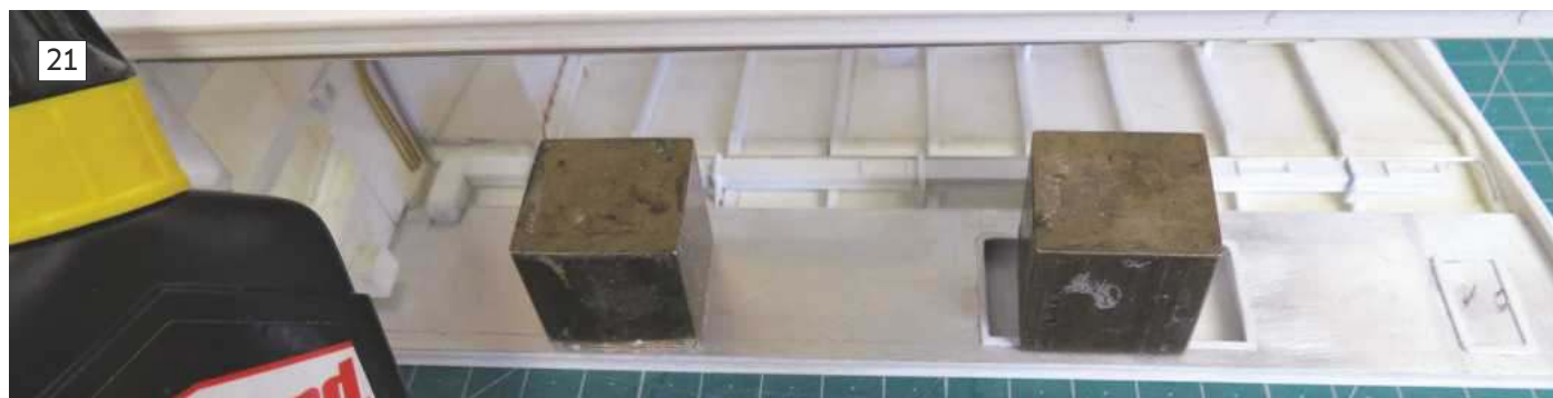
19: Carefully applying Uni-Bond Power Glue to the surface. 20: Using a spatula the Power Glue is spread evenly and thinly over the area of the lower hangar side wall. 21: The Litho plate panel is returned with time to adjust its positioning, weights are then added.
