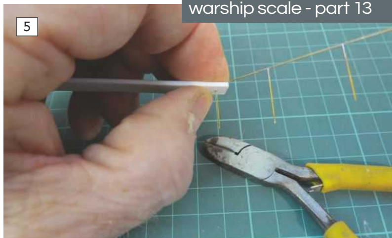
4: Using very small amounts of solder paste each joint is prepared for soldering. 5: With the length of safety rail soldered a small strip of styrene is used as both depth gauge and protecting the soldered joint when cutting each vertical length to size. 6: Spacers or depth gauge used to ensure consistency along to length of rail. 7: A standard single panel single lever action WT door as fitted to HMS Duncan.
