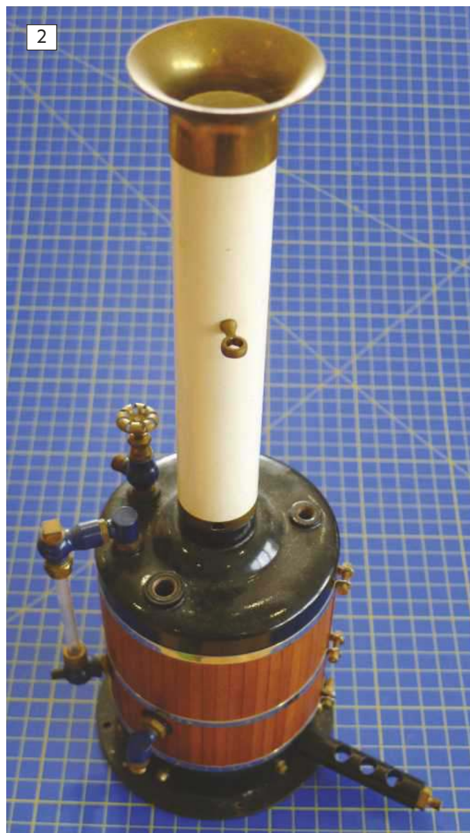
1: The Miniature Steam 3 inch vertical boiler fitted with a cast ceramic burner in the side of the furnace. This particular burner was evaluated more closely in Boiler Room Pt104. 2: A John Hemmens 3.5 inch vertical boiler fitted with a full width ceramic burner. It is supplied from a single nozzle and jet arrangement and is factory set for the optimum combustion.
