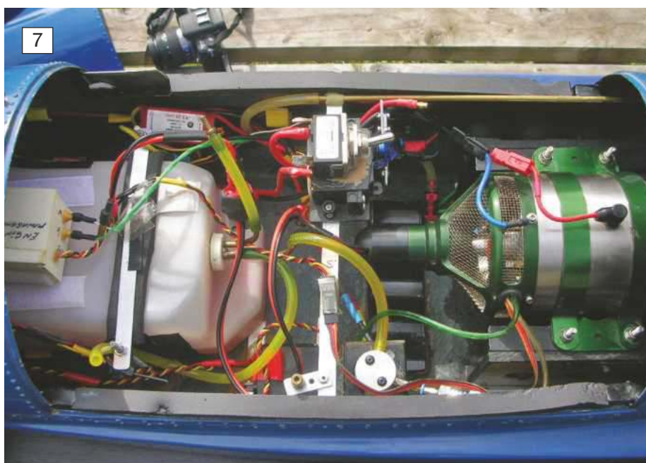
ABOVE: The servo operated/user operated kill switch to instantly cut fuel supply off. Also the Wren 54 engine and associated equipment fitted to the author's 1/6 K7 Bluebird. BELOW: The data terminal used to start a jet engine and access data relating to the use of the engine. It is useful for checking how many hours the engine has been run.
