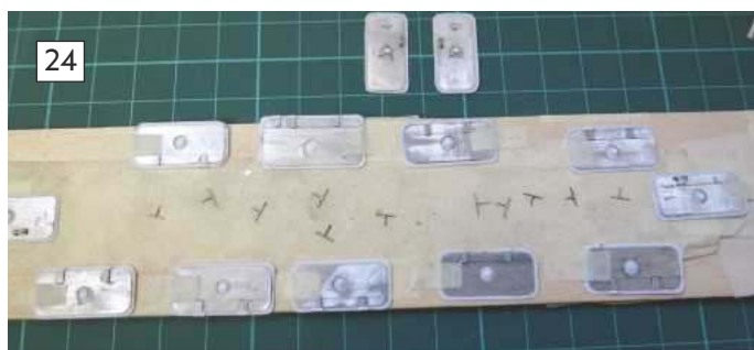
22: Using .35 brass wire to form the T-lever handles. 23: Using a profile jig to cut each lever handle to size. 24: Keeping each of the prepared T-lever handles in one place by using the sticky surface of the masking tape. 25: Fixing the T-lever handle onto the centre boss.
