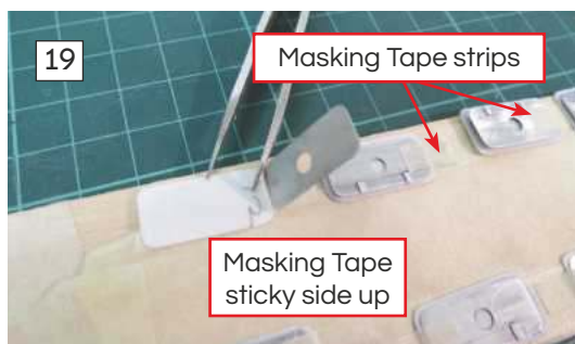
19: A simple but effective method to maintain symmetry when combining the Litho door panels with the styrene backing frame. 20: A jig for supplying all the hinge pins.
