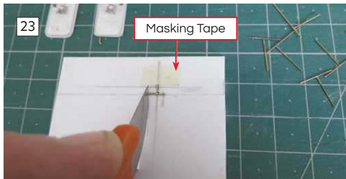
22: Using .35 brass wire to form the T-lever handles. 23: Using a profile jig to cut each lever handle to size. 24: Keeping each of the prepared T-lever handles in one place by using the sticky surface of the masking tape. 25: Fixing the T-lever handle onto the centre boss.
