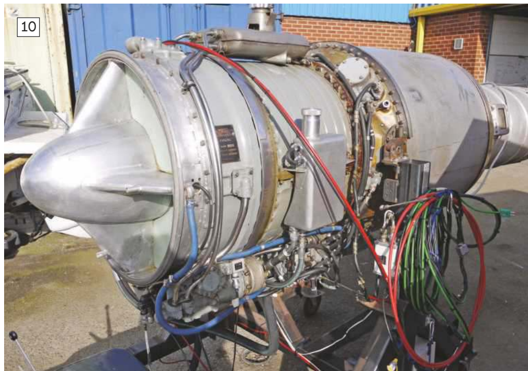
ABOVE & BELOW: The Bristol Orpheus engine used in K7 during testing in 2018; several of the parts on the engine have been taken from the original and restored to full working order.
