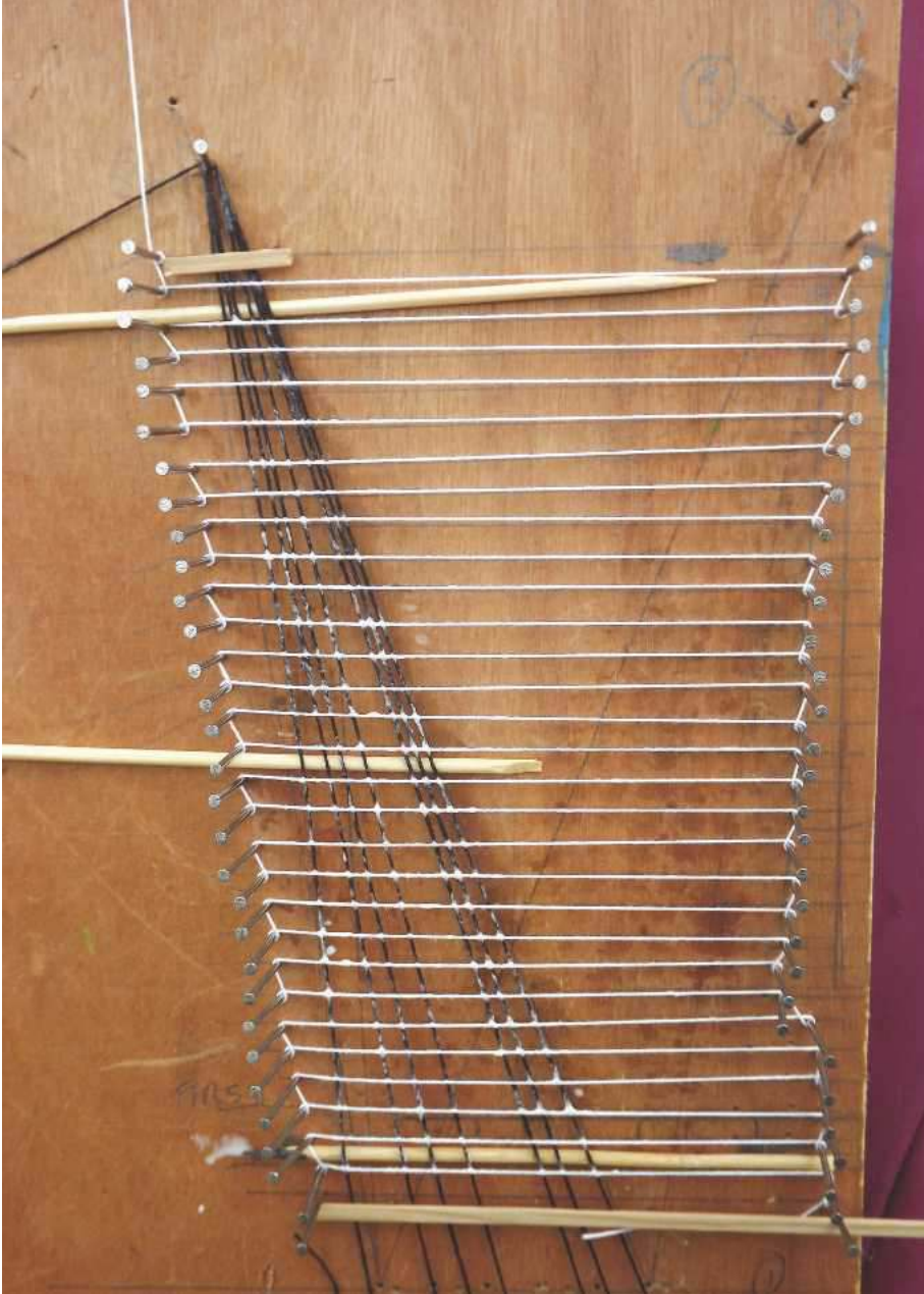
ABOVE: Shroud and ratline jig. BELOW: The bare masts in the storage tray.
