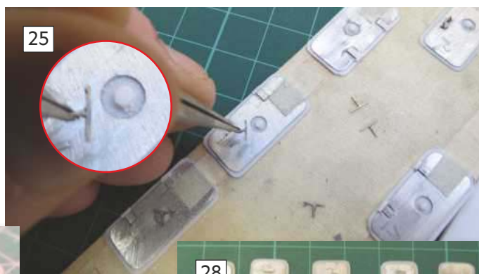
22: Using .35 brass wire to form the T-lever handles. 23: Using a profile jig to cut each lever handle to size. 24: Keeping each of the prepared T-lever handles in one place by using the sticky surface of the masking tape. 25: Fixing the T-lever handle onto the centre boss.
