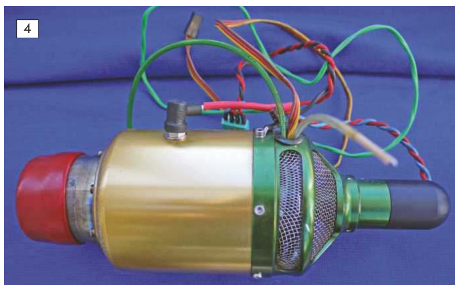
A Wren engine with the green protective screen and electric motor housing; the glow plug is on the top.
