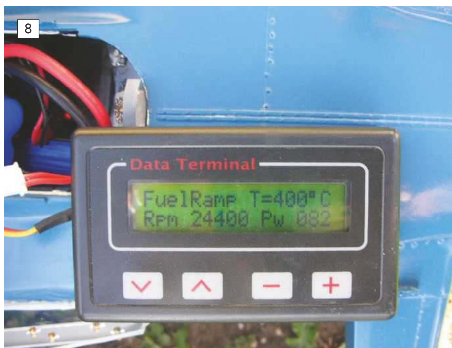
ABOVE: The servo operated/user operated kill switch to instantly cut fuel supply off. Also the Wren 54 engine and associated equipment fitted to the author's 1/6 K7 Bluebird. BELOW: The data terminal used to start a jet engine and access data relating to the use of the engine. It is useful for checking how many hours the engine has been run.
