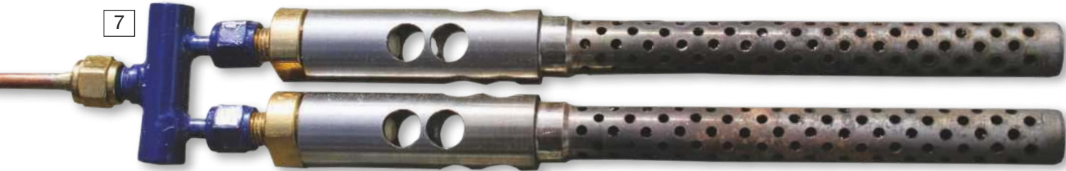
7: A twin poker burner arrangement of the same type as fitted to the Hemmens Caton boiler. This is a burner unit from the same manufacturer's Ribbersdale boiler.
