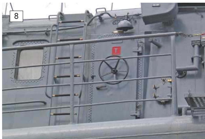
8: Typical example of a type of WT door favoured by the Soviet Navy in the early 1980s as fitted to the Admiral Levchenko. 9: In 2001 the Russian navy began introducing the single panel single lever action door for the Steregushchiy.
