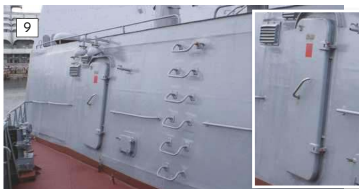
8: Typical example of a type of WT door favoured by the Soviet Navy in the early 1980s as fitted to the Admiral Levchenko. 9: In 2001 the Russian navy began introducing the single panel single lever action door for the Steregushchiy.
