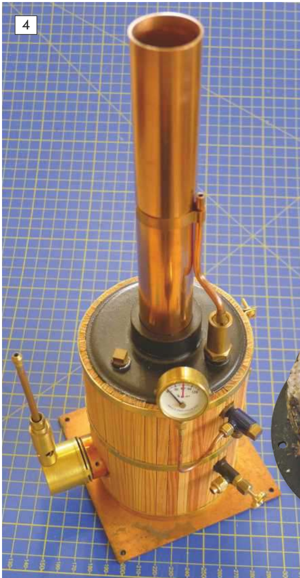
4: A Pendle 3.5 inch vertical boiler with a drilled brass disc type burner fitted to the side of the furnace space.
