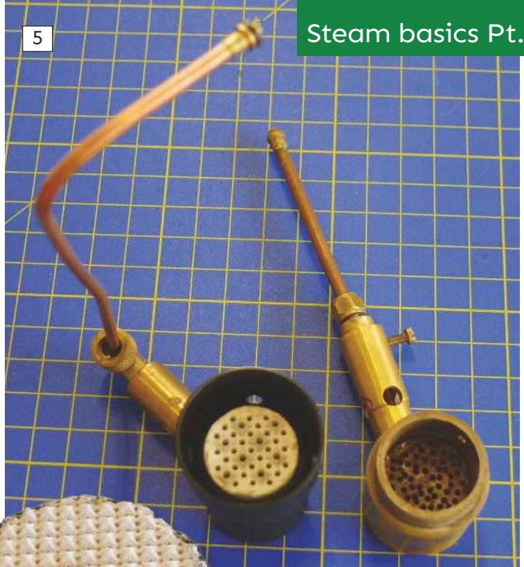
5: The burner for the Miniature Steam boiler is the cast ceramic unit on the left. Of a similar size is the drilled disc type from Pendle on the right. Both these burners are factory fitted with a number 5 jet and do have similar gas consumptions.
