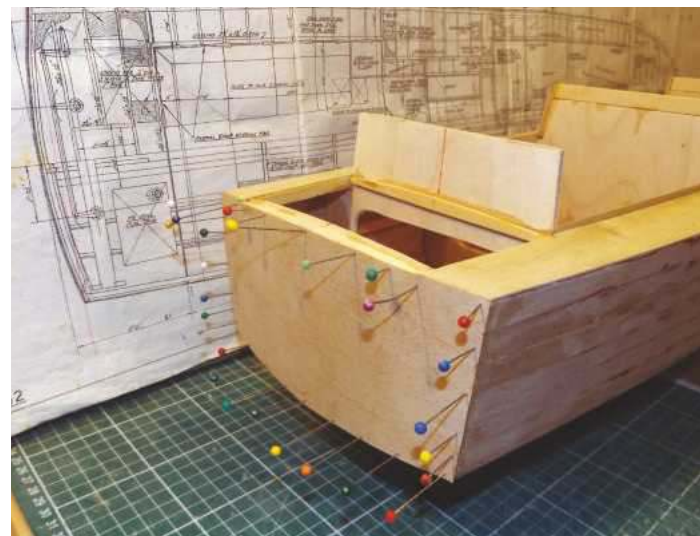
ABOVE LEFT: Hull with planking complete with Thorneycroft drawing behind. ABOVE RIGHT: Transom 1/32in sheeting glued and pinned in place. BELOW LEFT: Twin propeller shafts in location with one prop fitted and ply blank ready for epoxy. BELOW RIGHT: Twin rudder linkage and steering servo in place.
