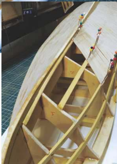
ABOVE: Starboard side first layer of diagonal planking.
