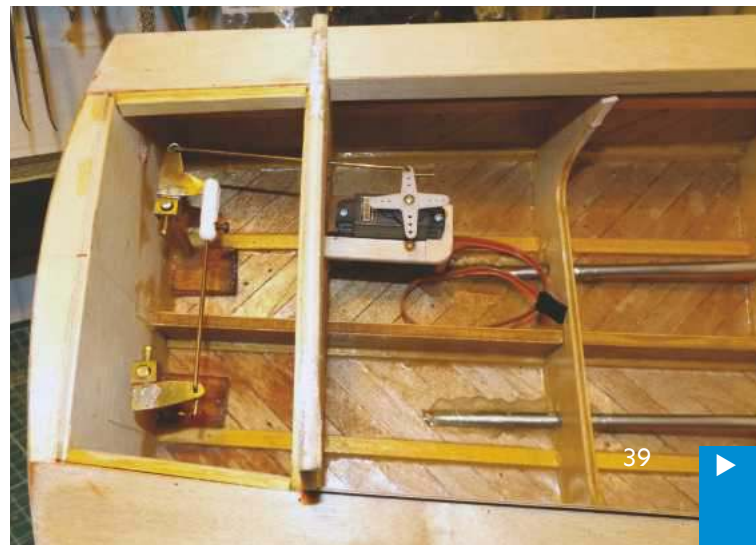
ABOVE LEFT: Hull with planking complete with Thorneycroft drawing behind. ABOVE RIGHT: Transom 1/32in sheeting glued and pinned in place. BELOW LEFT: Twin propeller shafts in location with one prop fitted and ply blank ready for epoxy. BELOW RIGHT: Twin rudder linkage and steering servo in place.
