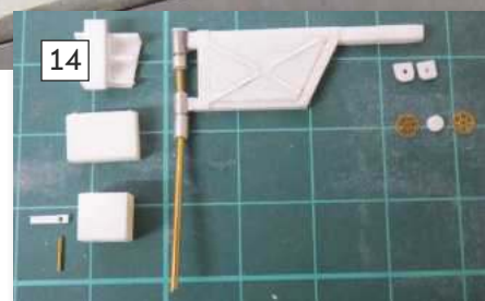
14: Assembly underway, here the common shaft is slightly inclined to mirror the incline of the deck housing.
