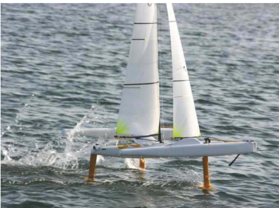
Skyfall, foiling, but not as we expected it - heavy and slow, complete with T foils on the floats and big wands up in the bows.
