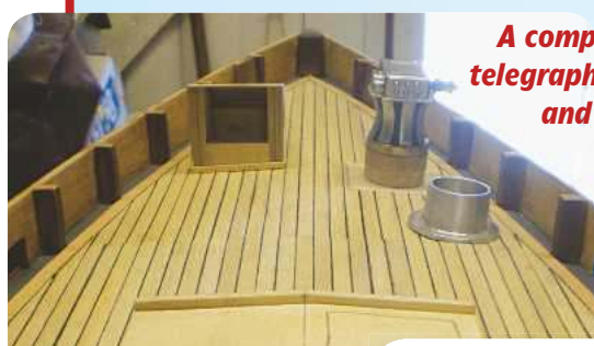
View showing the first deck planking
