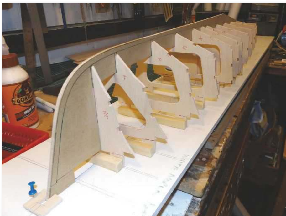
ABOVE LEFT: Complete set of bulkheads cut from 1/8in birch plywood. ABOVE RIGHT: Bulkheads and keel mounted on building board with extensions to common datum.
