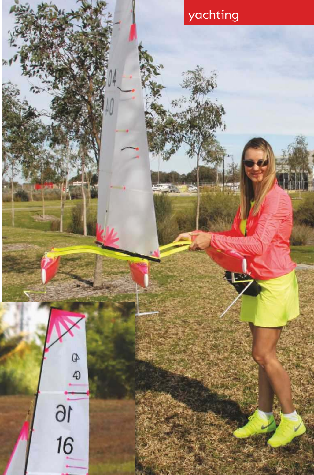
ABOVE: Box Number 4 with Z foils. LEFT: The new Box-on-Steroids (BOS) foiling in light winds with its #1 rig up. This rig is smaller than the maximum allowed under the Mini 40 class rules but is as big as I dared put on such a small platform. Sails by David Potter.
