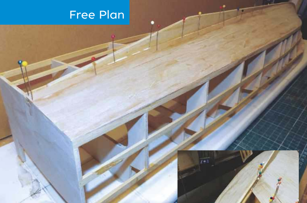
LEFT: Completion of carvel planking parallel to the keel.
