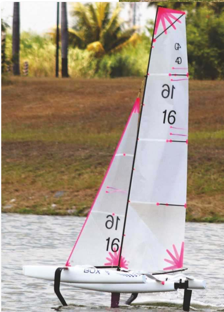
ABOVE: Box Number 4 with Z foils. LEFT: The new Box-on-Steroids (BOS) foiling in light winds with its #1 rig up. This rig is smaller than the maximum allowed under the Mini 40 class rules but is as big as I dared put on such a small platform. Sails by David Potter.
