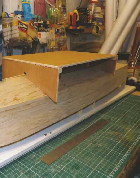
BELOW: Trial fitting of 1/4in plywood stand/cradle on the hull.
