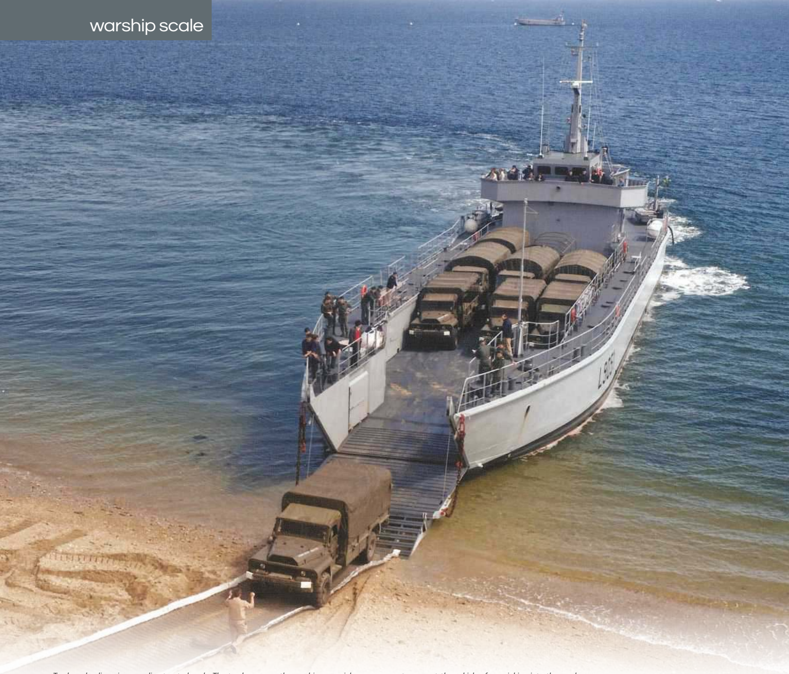
Trucks unloading via ramp direct onto beach. The trackway over the sand is a special canvas cover to prevent the vehicles from sinking into the sand.
