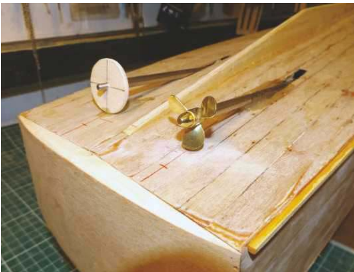
ABOVE LEFT: Hull with planking complete with Thorneycroft drawing behind. ABOVE RIGHT: Transom 1/32in sheeting glued and pinned in place. BELOW LEFT: Twin propeller shafts in location with one prop fitted and ply blank ready for epoxy. BELOW RIGHT: Twin rudder linkage and steering servo in place.
