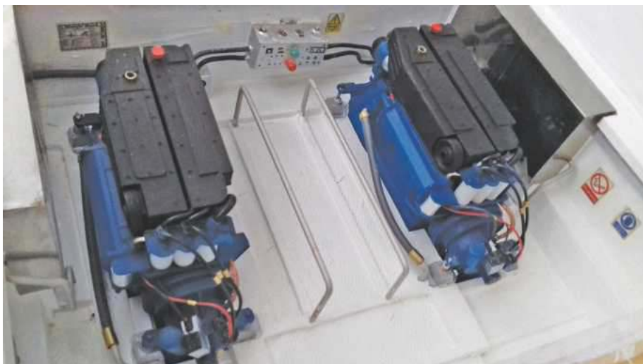
ABOVE: James Thompson's scratch-built Princess 65. LEFT: The interior of the Princess 65 is as luxurious as the real yacht. BELOW: Scratch-built Volvo Penta engines conceal a pair of 540 electric motors.
