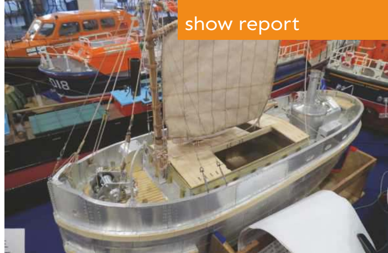
ABOVE LEFT: Arun No1 (52-01) at 1/12 scale by Arthur Barlow of the Ship Modelling Society. Plank on frame construction. Dave Wooley ABOVE RIGHT: An all scratch-built aluminium plated 1886 Clyde Puffer Otter by George Barrett and rigged with a Gaff Trysail. The original sank in 1893. Dave Wooley
