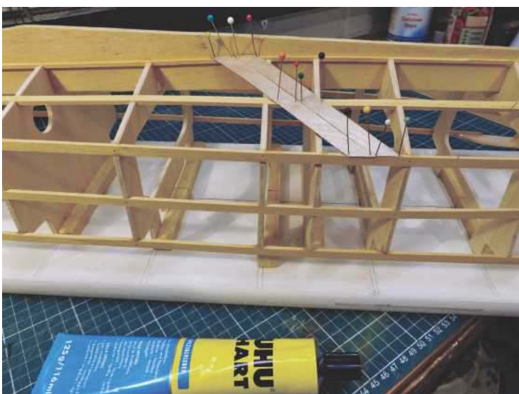
ABOVE LEFT: First of the base layer of diagonal planking at 45^\circ to the keel. ABOVE RIGHT: Commencement of second carvel layer of planking length ways bow to stern.
