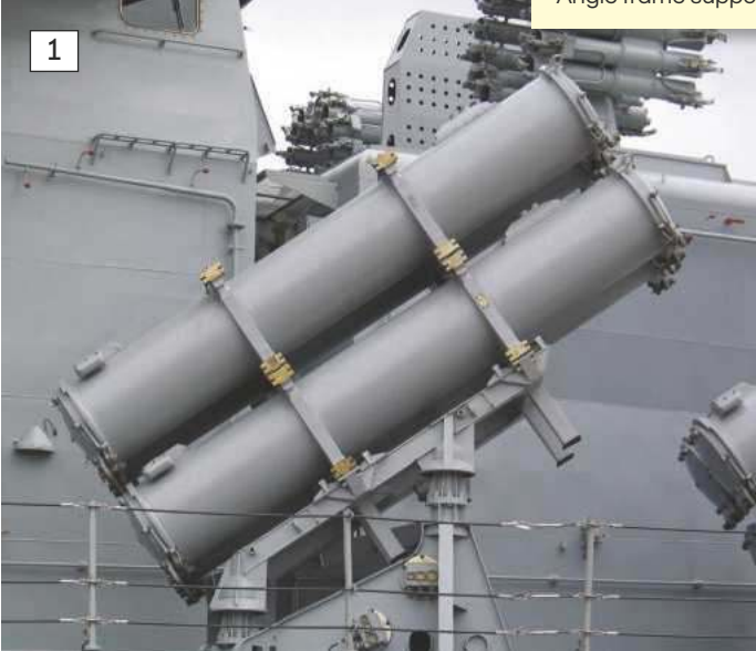
1: One of four quad Launch tubes and support frame designated Kh35E a lightweight export variant of the KE35 SSM aboard the Delhi-class DDG IN Mumbai. 2: The launch system as fitted to the IN Mumbai in the late 1990s is similar in many respects to that fitted to Soobrazitelnyy in 2004.
