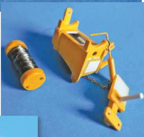
ABOVE: The assembly with the modified trip weight arm fitted; also the membrane can be seen fitted to the main body.
