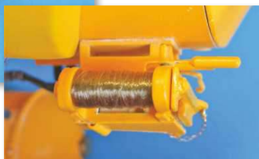
BELOW: The emergency buoy fitted to the stern of the model. Note: under the trip weight an additional lever can be seen.
