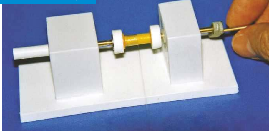
ABOVE: The buoy's winding jig made from plastic card. The two larger white pads hold the buoy in place, while the fishing line is wound on. BELOW: The completed emergency buoy assembly.
