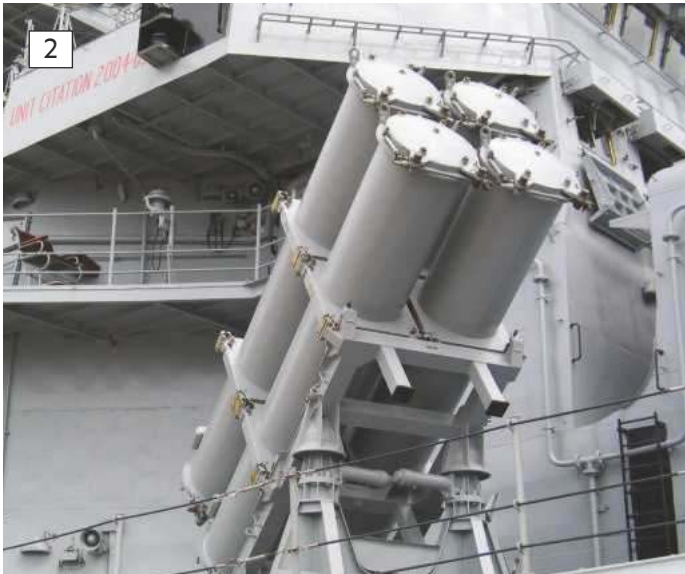
1: One of four quad Launch tubes and support frame designated Kh35E a lightweight export variant of the KE35 SSM aboard the Delhi-class DDG IN Mumbai. 2: The launch system as fitted to the IN Mumbai in the late 1990s is similar in many respects to that fitted to Soobrazitelnyy in 2004.
