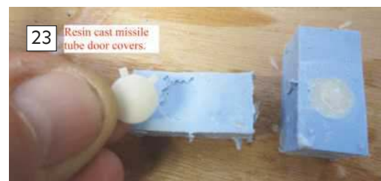
23: Fresh from the rubber mould one of 16 resin tube door covers.
