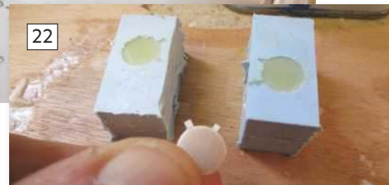
22: The master from which all door covers are cast in resin from a rubber mould.
