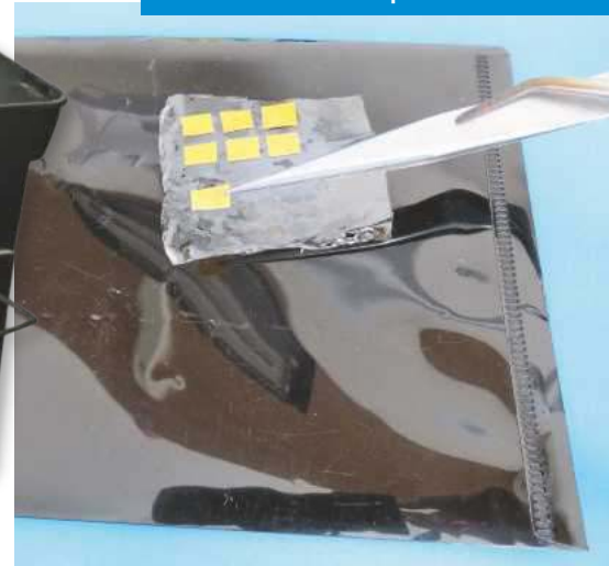
ABOVE: The membrane being lifted off the plastic sheet. BELOW: The double-sided applied to both sides of the membrane.
