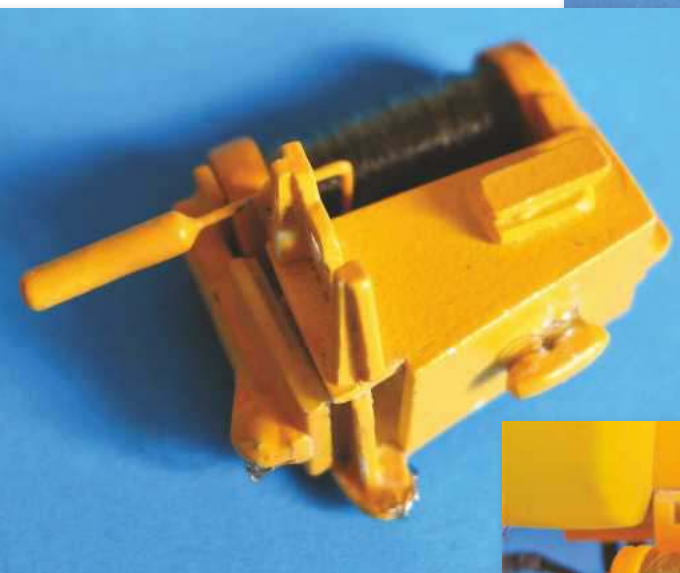
ABOVE: The assembly with the modified trip weight arm fitted; also the membrane can be seen fitted to the main body.
