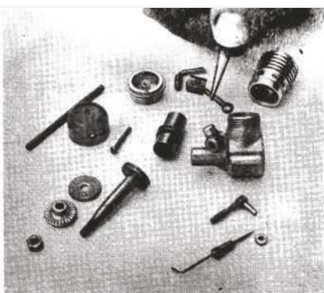
Breakdown of parts gives an idea of the diminutive sizes involved. The thread on the crankcase indicates where the cylinder head screws down, at the same time locking the cylinder timer in position.
