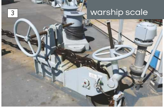
2: Right forward towards the panama bows. 3: Medway has no screw or blake slips securing the anchor cable, thus a return to the past with a seldom used controller or bow stopper.
