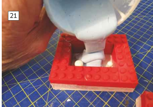
20: A simple coffer dam made from Lego bricks to retain the rubber prior to setting. 21: Adding the rubber to create the mould. 22: After a period between 8-24hrs the Lego coffer dam can be easily dismantled.
