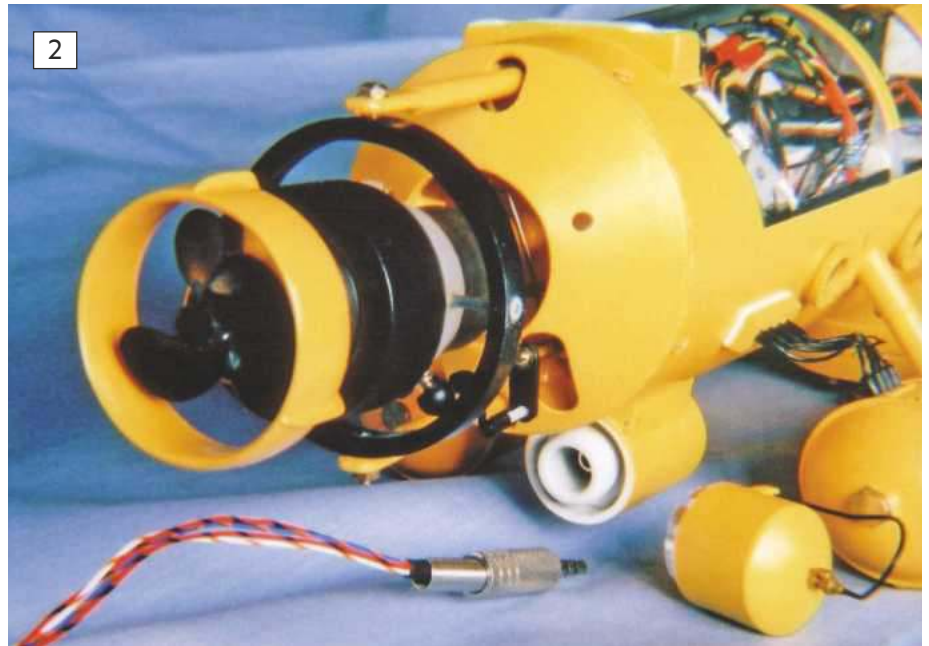
Photo 2: Another, but smaller tank on the underside; again I don't know its function on the vessel. On the model, the back of the tank can be removed revealing the charging port. The cap contains the valve as described in the text.
