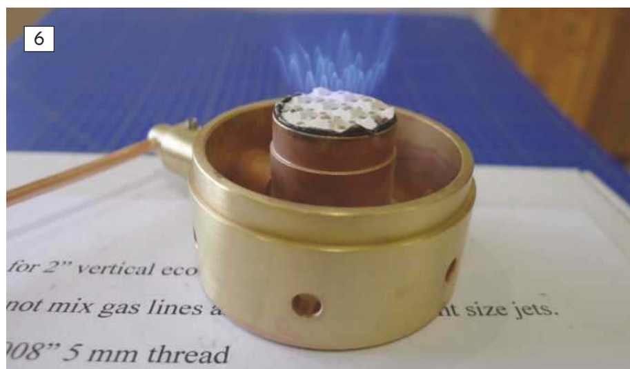
Pulling the holder all the way out admits too much air and consequently a 'Weak' mixture.
