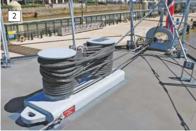
2: Right forward towards the panama bows. 3: Medway has no screw or blake slips securing the anchor cable, thus a return to the past with a seldom used controller or bow stopper.
