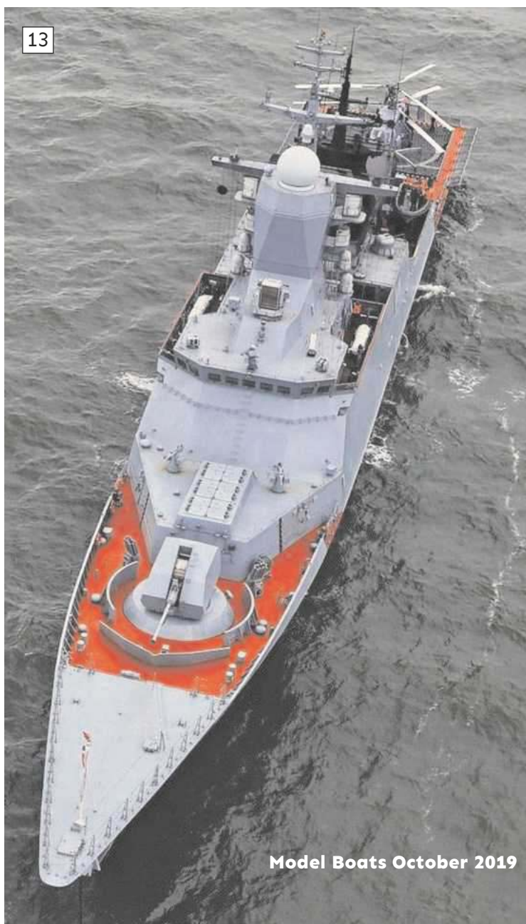
11: All twelve hatch covers are prepared, ready to be fixed to the hatch bed. 12: A dedicated mounting which makes assembly so much easier. 13: This superb official image of the Soobrazitelnyy shows clearly the positioning of the VLS forward of the bridge. Official Image.
