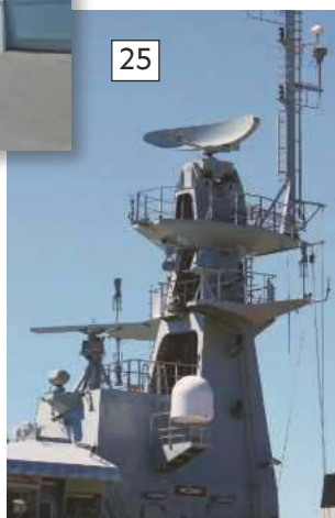
25: On the middle platform over to port is the Sharp Eye E/F band Radar and mounted on the top platform the air/surface search radar.
