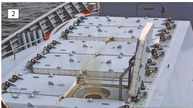
1: Immediately forward of the bridge in a raised housing containing twelve Redut VLS cells.
