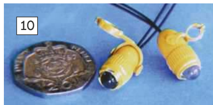
Photo 10: The LED spot lights. Note the difference around the outer lens area.
