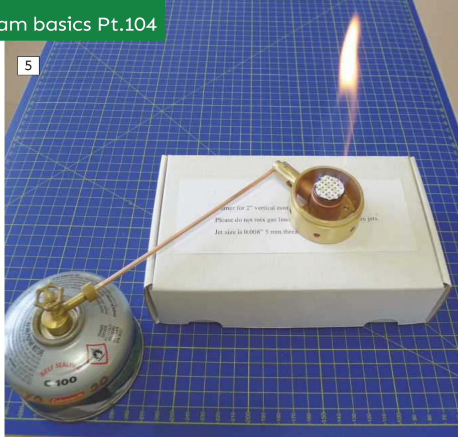
Pushing the nozzle holder all the way into the burner pipe, turning on the gas and igniting the burner produces a very 'Rich' mixture that burns weak and relatively cool.
