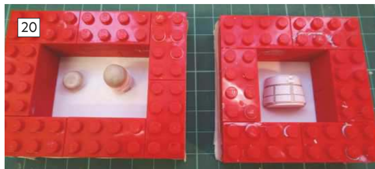
20: A simple coffer dam made from Lego bricks to retain the rubber prior to setting. 21: Adding the rubber to create the mould. 22: After a period between 8-24hrs the Lego coffer dam can be easily dismantled.
