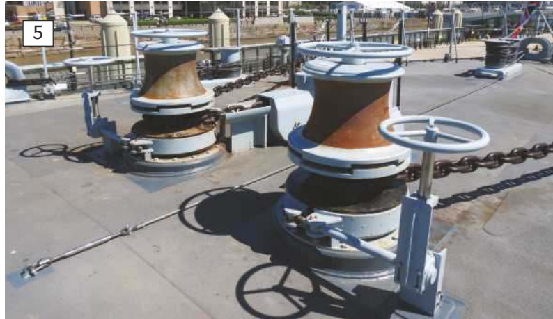
4: An excellent view of the bollard and stanchions. 5: Cable holders; note the brake handwheels either side. 5: Cable holders; note the brake handwheels either side.
