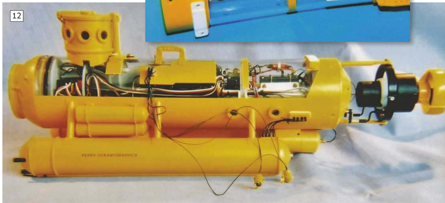
Photo 12: The model without its canopy and protective frame. The top of the tube was not painted, leaving the acrylic tube see-through making assembly easier.
