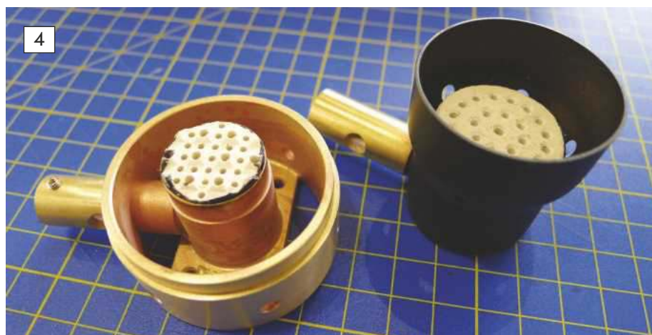
Even the construction of the 2in and the 3in burner units are quite different with additional air holes in the periphery of the burner to admit further air supply.
