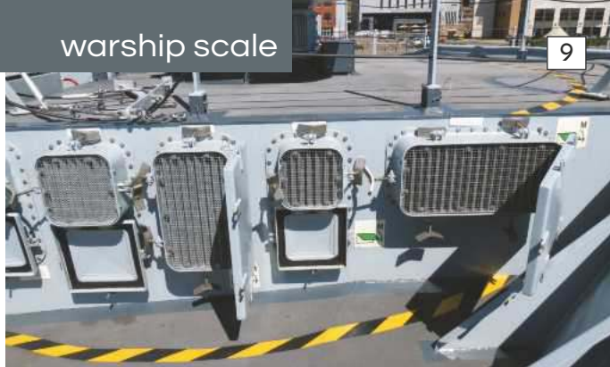
9: Various types of louvered vents attached to the side of the 30mm gun platform. 10: The vent arrangement over to port is different to that on the starboard side of the 30mm gun platform.
