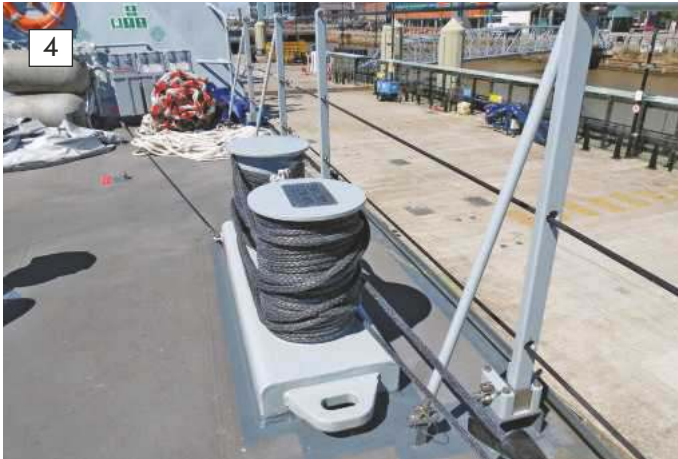
4: An excellent view of the bollard and stanchions. 5: Cable holders; note the brake handwheels either side. 5: Cable holders; note the brake handwheels either side.
