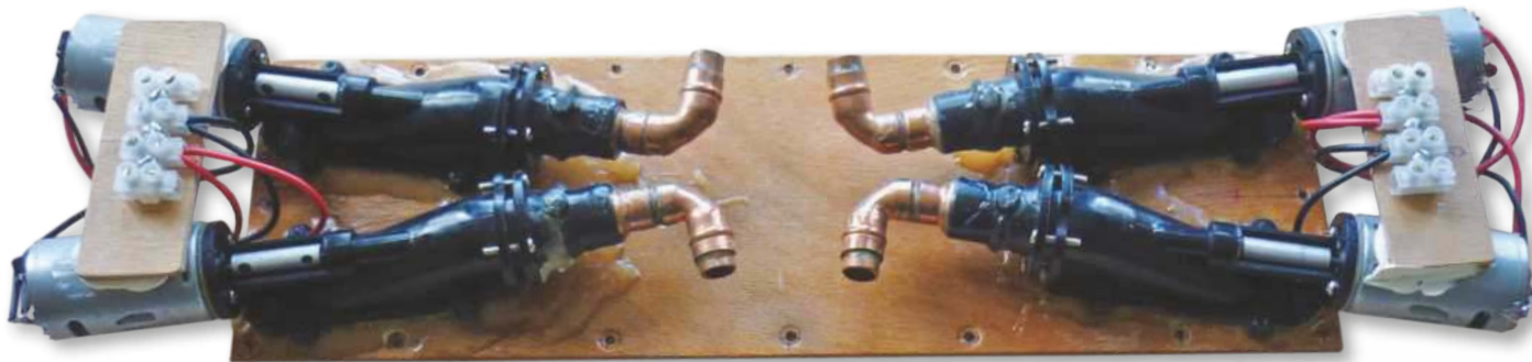
ABOVE: Modified NQD water jets on baseplate.
