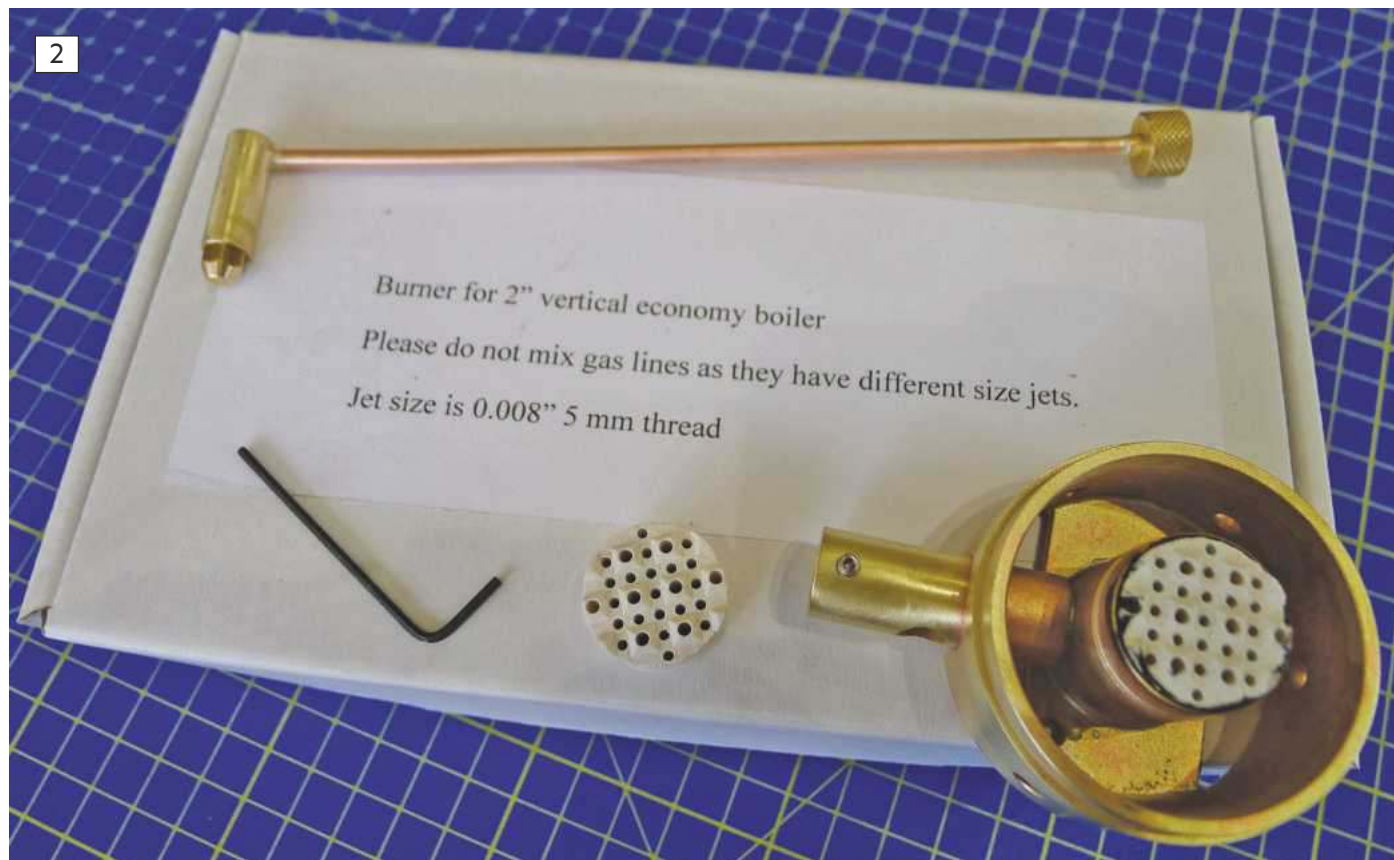
ABOVE: Each burner unit comes complete with its own gas pipe, pre-fitted with the appropriate sized jet, an Allen key to adjust the nozzle position, comprehensive set up instructions and a spare ceramic disc.
