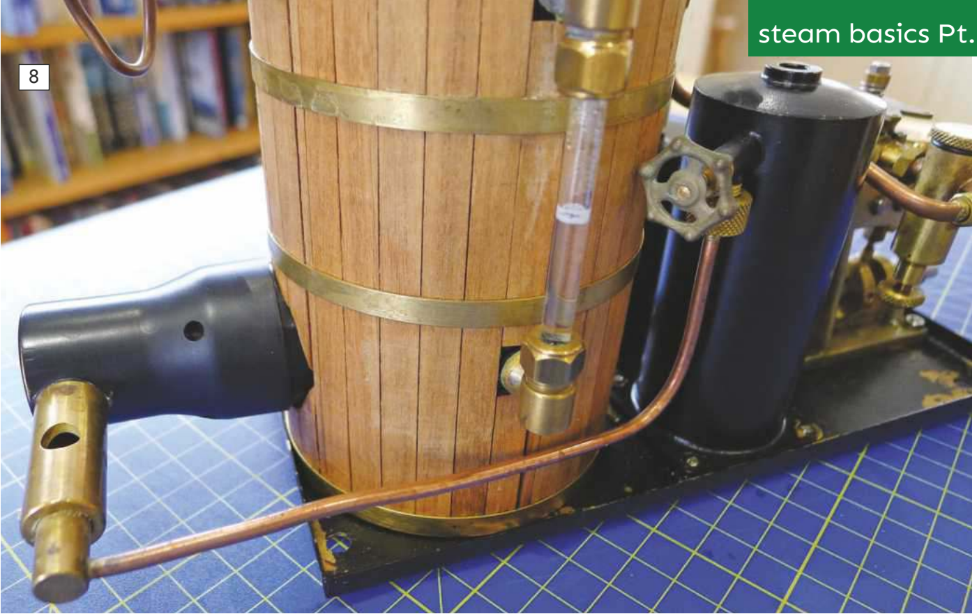
ABOVE: The 2in cast ceramic burner in place in a Clyde 3in vertical boiler plant.
