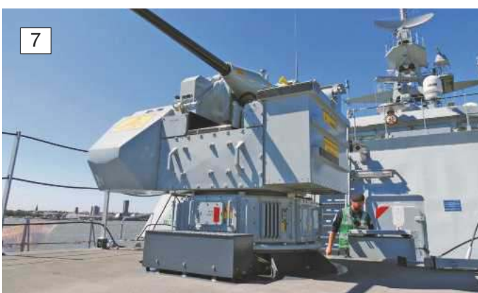
7: The DS30M 30mm automatic/manual naval gun. 8: The 30mm gun is mounted on a raised platform immediately abaft of the breakwater.
