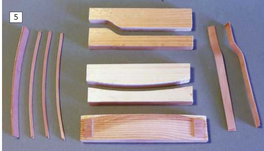
ABOVE: Templates/moulds for cabin roof laminations.
