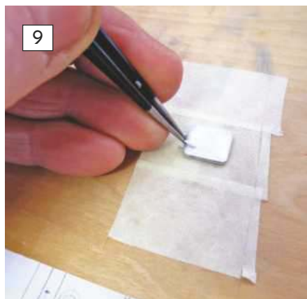
9: Using masking tape to hold the hatch cover in place whilst fixing each of the prepared fittings.
