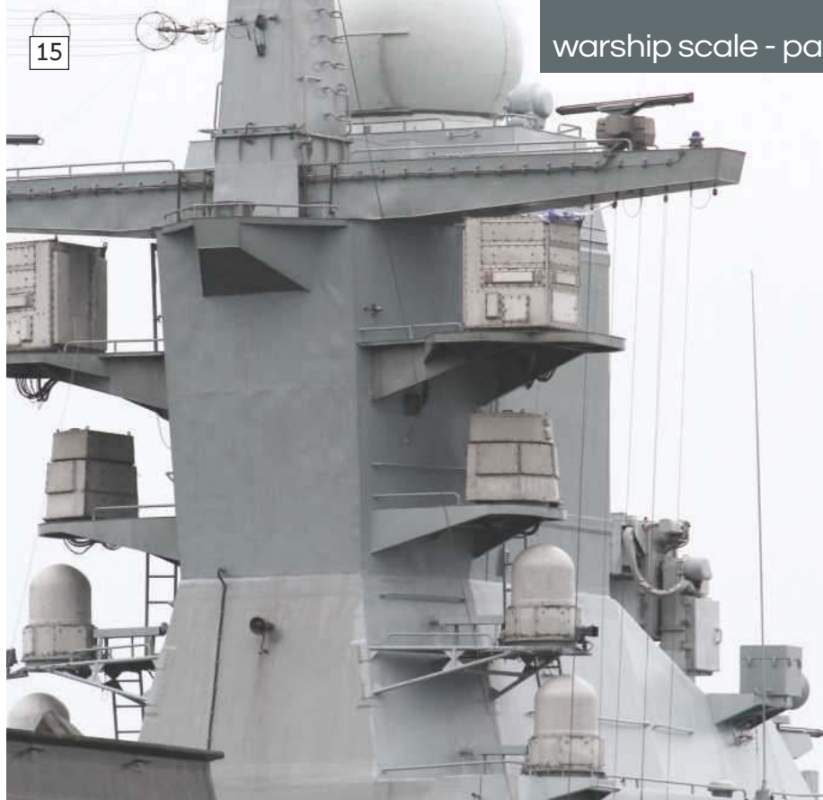
15: The foremast with the various EW sensors mounted on platforms either side.
