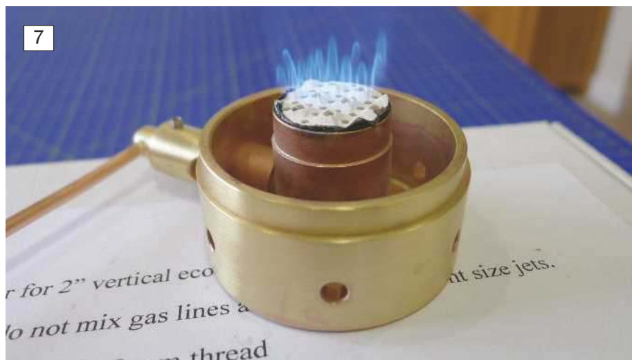
Get it just right and the flame cones should be just sat above the ceramic disc.
