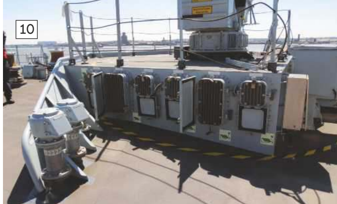
9: Various types of louvered vents attached to the side of the 30mm gun platform. 10: The vent arrangement over to port is different to that on the starboard side of the 30mm gun platform.
