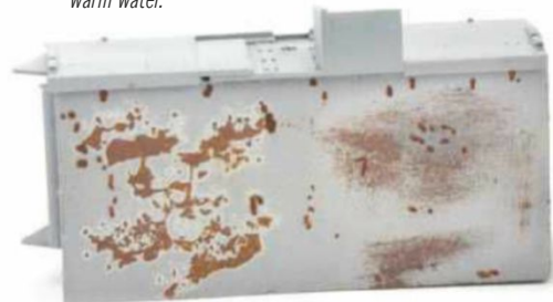
...and the result after the top coat has been removed with warm water.
