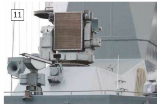
11: The PUMA fire control looking towards the left-hand side.
