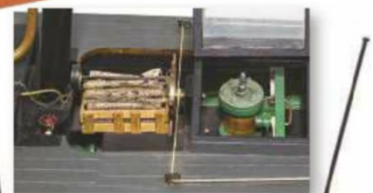
BELOW: Detail of the Dolly showing the engine, steering gear and wood logs for the boiler.
