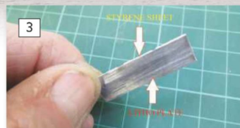
3: The styrene is bonded to the Litho and each hatch cut to size.
