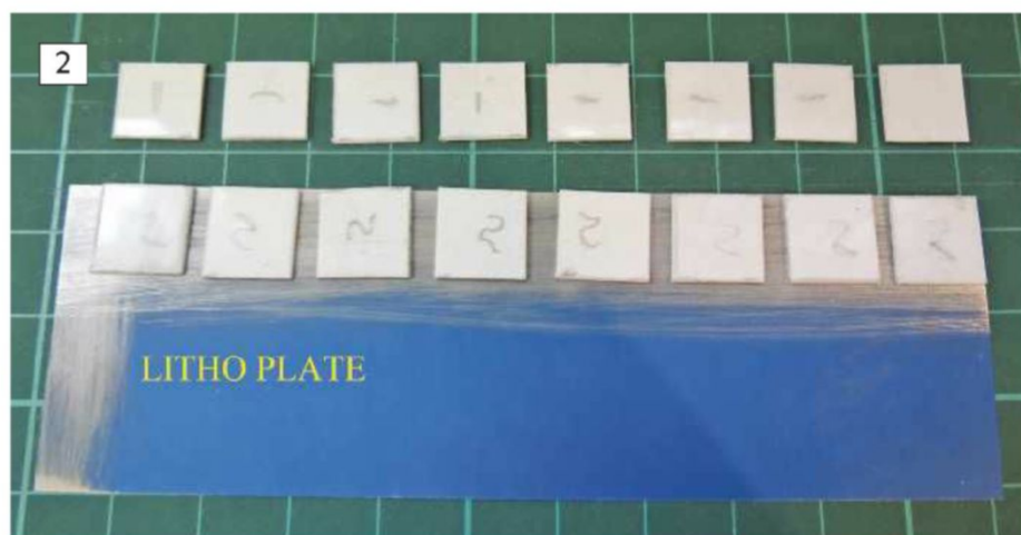
2: The two basic sets of material, litho and styrene for forming the hatches.
