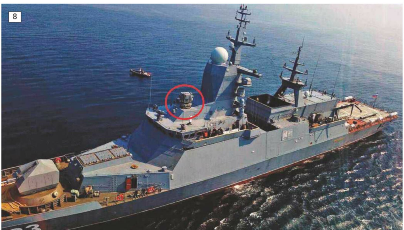
7: Fifteen deck hatches, but twelve types. 8: Ringed in red is the PUMA fire control radar as fitted to the Sovershenyy prior to commissioning on 20 July, 2017.
