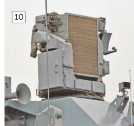
10: A high resolution view of the PUMA fire control radar showing the front and right-hand side.
