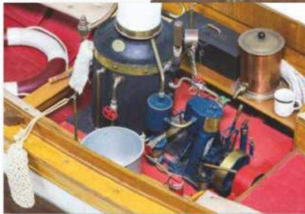
ABOVE: Detail on the Lady Elizabeth showing the engine, boiler, 'Windermere kettle' and cup!
