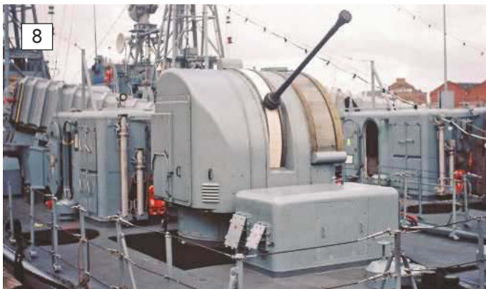
8: Looking towards the front of the GRP gun-house. The aimer's position is over to the right side of the gun-house which can be opened. 9: Viewing over to starboard aft which reveals a differing arrangement on this side of the 40mm. 10: Deck detail right aft.
