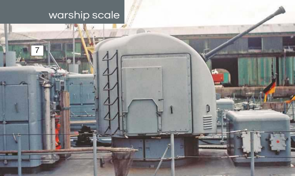
7: Unrecognizable but within this Mauser GRP gun-house is a Bofors 40mm gun.
