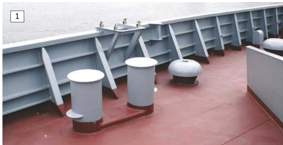
1: Deck detail aboard Project 20380 Soobrazitelnyy, double bollards and one of many different types of mushroom vents. Plus, the structural arrangement along the bulwark. 2: Prepared parts for the double bollard. 3: The assembled double bollard.
