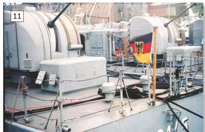
11: In this image it's worth noting just how the flexible rails are secured to the corner stanchions.
