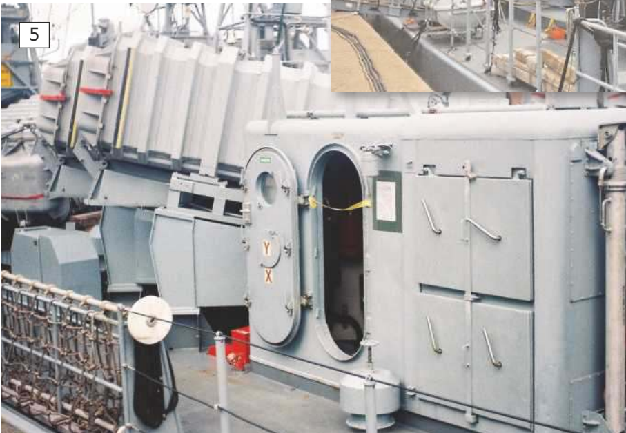
5: This small deck housing gives access below to the 4 MTU 16-cylinder diesels. The 148s has capacity for 39tons of fuel. 6: Jacks and shoring up timbers.
