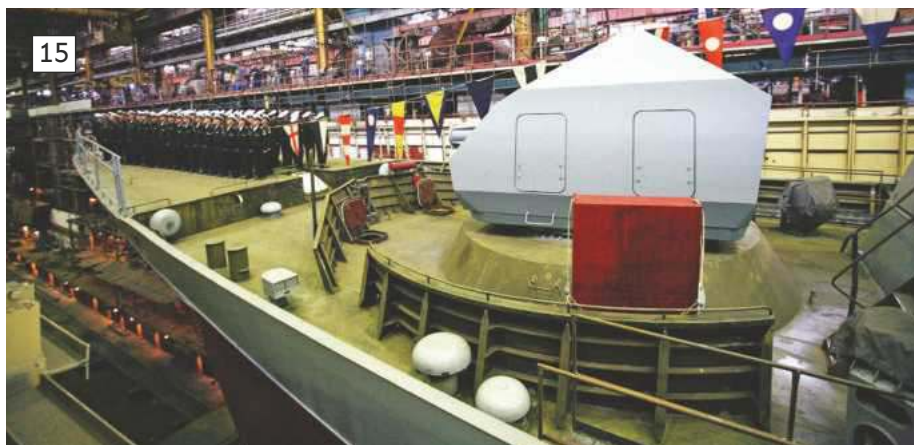
13: The capping has a flush edge with the hull side and a 2mm lip inboard. 14: Providing a push fit the prepared styrene bulwark is slotted into place. 15: Viewing the area of the Forecastle around the gun mounting showing the breakwater and spent round retaining barriers.
