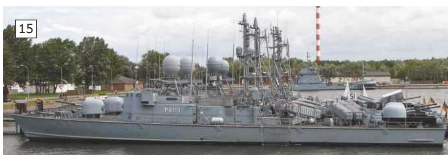
15: Larger and more powerful, these Lürssen-designed and Rensburg-built Type 143's had a similar task as the older 148s but differed in fire control and marginally in armament.
