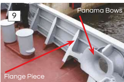
9: The Panama Bows and flange piece across the bulwark support.
