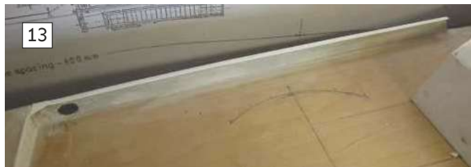
13: The capping has a flush edge with the hull side and a 2mm lip inboard. 14: Providing a push fit the prepared styrene bulwark is slotted into place. 15: Viewing the area of the Forecastle around the gun mounting showing the breakwater and spent round retaining barriers.
