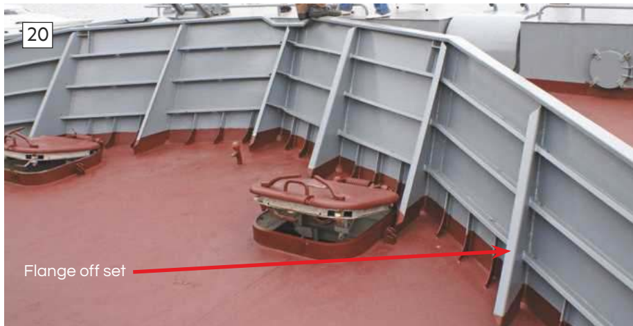
18: A jig for cutting the chevron into the top and bottom of the flange pieces. 19: 45mm brass locating pins added to each end, hidden behind the flange piece. 20: On the break water the flange piece is off set.
