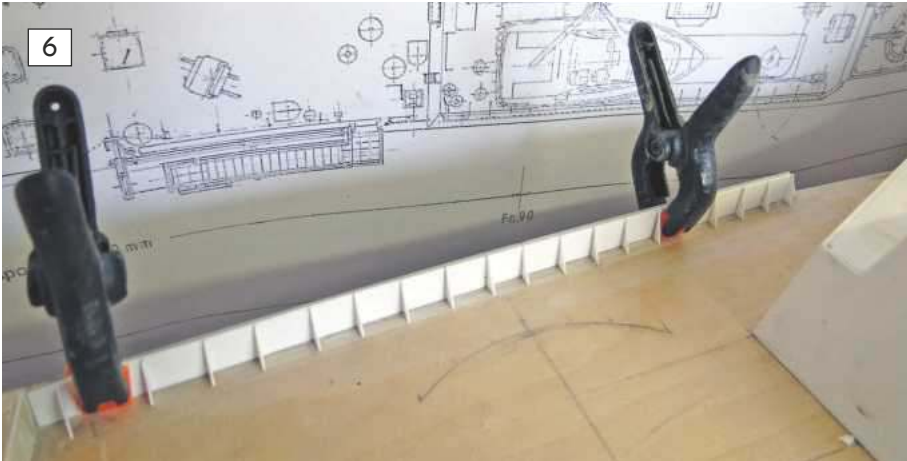
6: All the supports in place along the length of the styrene bulwark.
