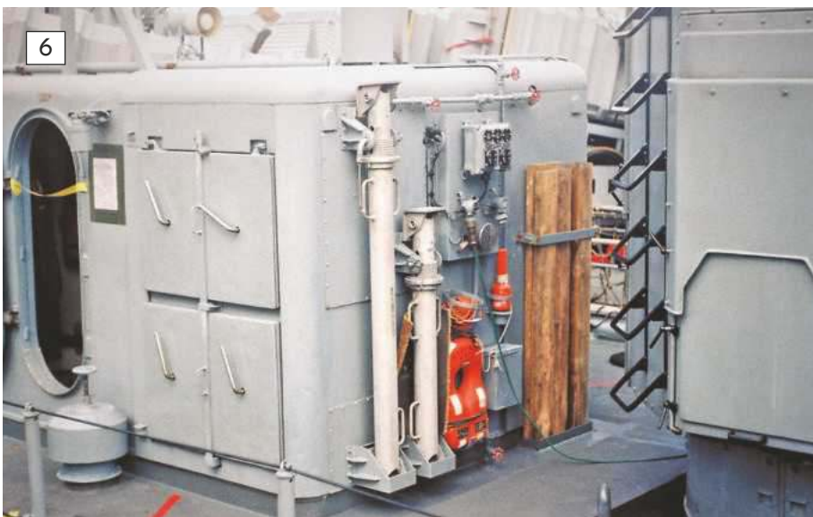
5: This small deck housing gives access below to the 4 MTU 16-cylinder diesels. The 148s has capacity for 39tons of fuel. 6: Jacks and shoring up timbers.
