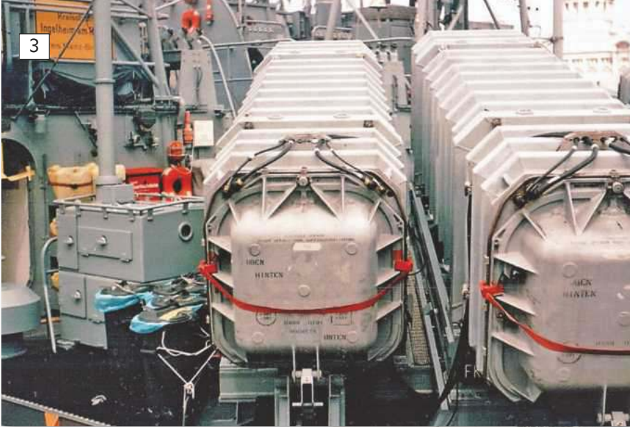
3: Exocet MM38 launch containers with the two forward pair angled to starboard at 12° elevation with this image detailing the loading doors
