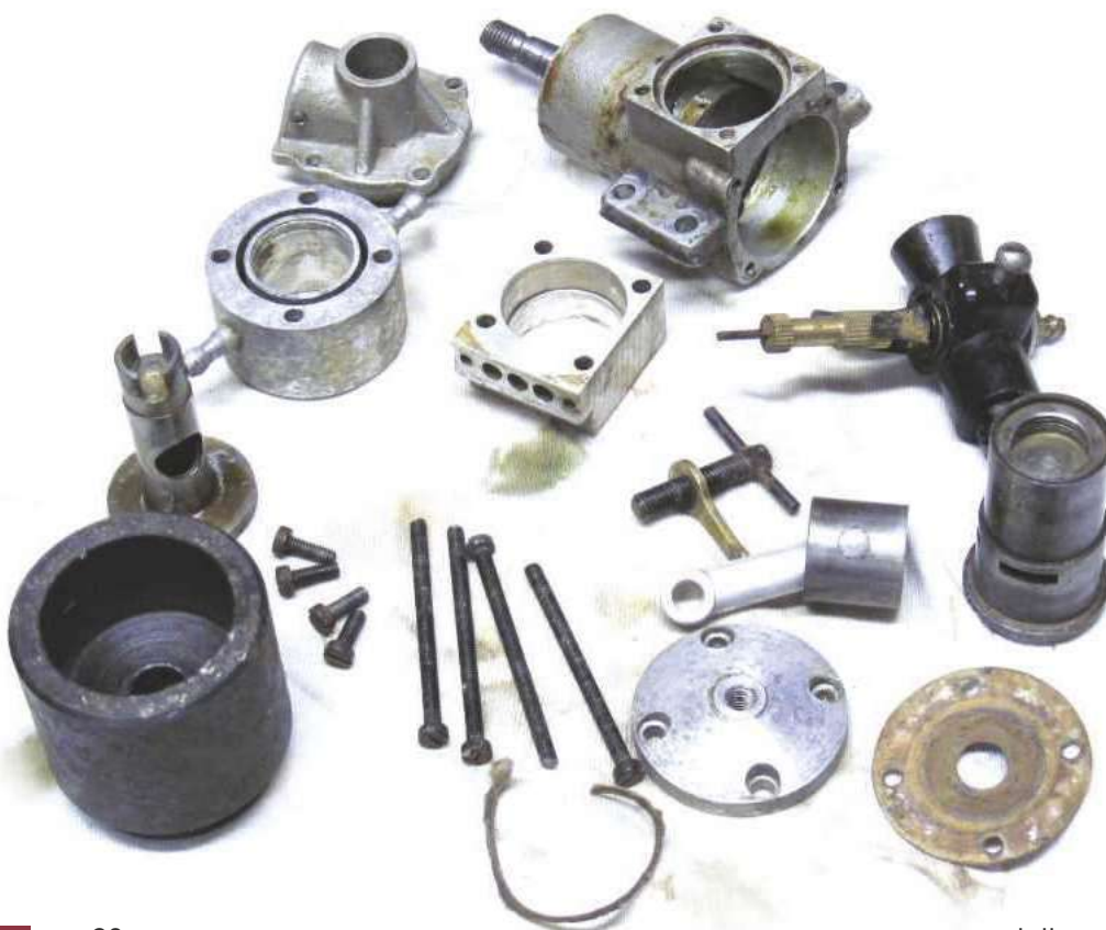
LEFT: A stripped Mk.III E.D. 'Sea Otter' marine diesel engine. Courtesy Simon Knachbull
