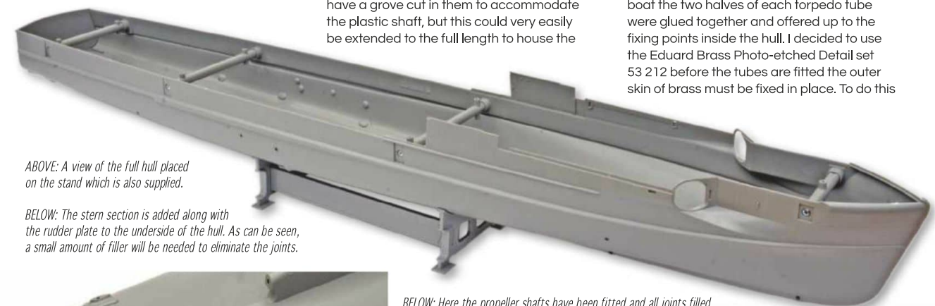
BELOW: Here the propeller shafts have been fitted and all joints filled and sanded smooth.
