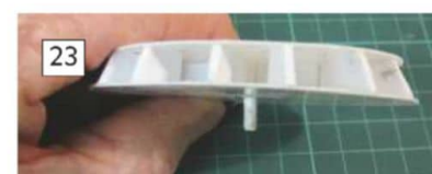
23: Incorporating sheer and camber into the mounting.
