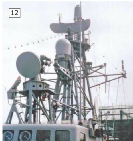
12: The various radar arrays fitted to the Type 148.
