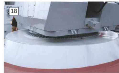
17: Starting to take shape with the fore and main mast temporarily positioned onto the model. 18: Gun mounting and gun ring as fitted to the Soobrazitelnyy A-190 100mm/59calibre naval gun.
