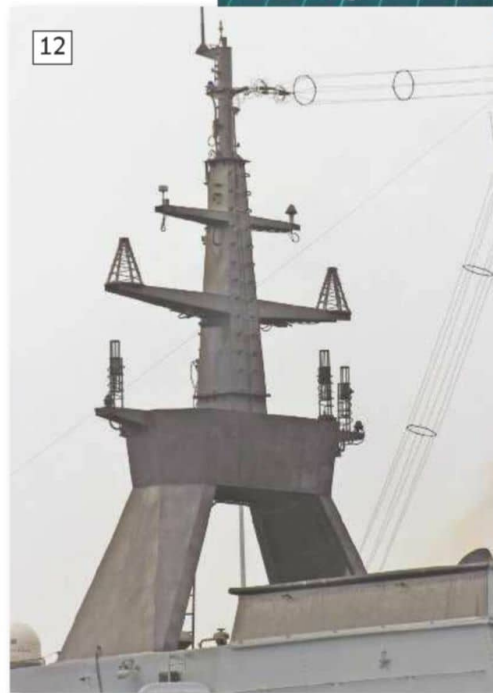
12: The main or comms mast using a goal post configuration.
