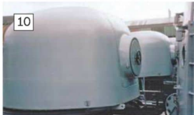
10: Access into the GRP gun house is through this hatch in the rear of the turret.
