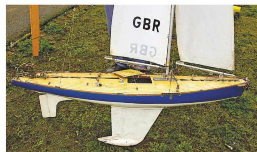
M Class Gretel - This is a modified Elusive that was produced by Albert Sinar and Ron Harris from the original Gretel that my brother George and I sailed that first time. I have restored it from deck level retaining some of the original fittings. The mast and booms are completely new from my own design. The mast height is 80in (2032mm) in top rig.
