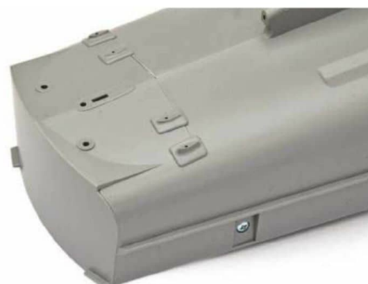
BELOW: The stern section is added along with the rudder plate to the underside of the hull. As can be seen, a small amount of filler will be needed to eliminate the joints.
