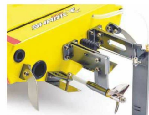
ABOVE: A purposeful stern complete with the usual array of attachments associated with a performance fast-electric boat.
