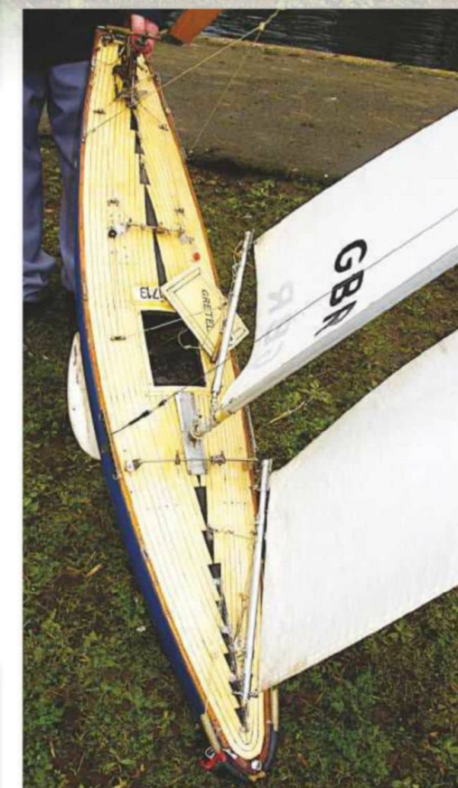
M Class Gretel - This is a modified Elusive that was produced by Albert Sinar and Ron Harris from the original Gretel that my brother George and I sailed that first time. I have restored it from deck level retaining some of the original fittings. The mast and booms are completely new from my own design. The mast height is 80in (2032mm) in top rig.
