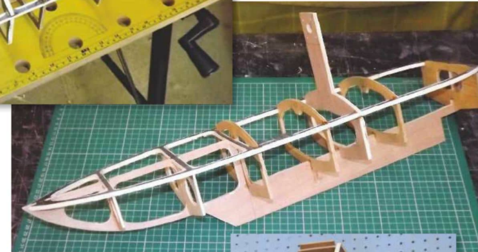
BELOW: The frame now tacked together with superglue.
