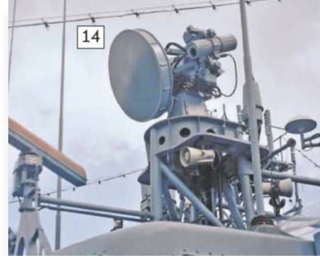
14: Mounted on the bridge roof close to the upper helm position is the Caster 11 fire control radar.
