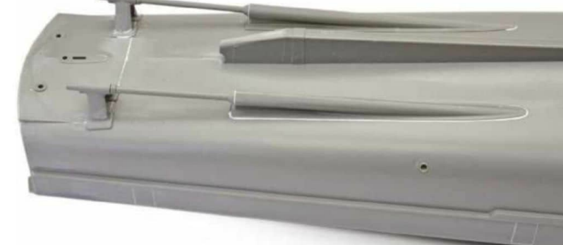
BELOW: Here the propeller shafts have been fitted and all joints filled and sanded smooth.
