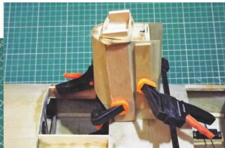
Clamping ply onto the tower.
