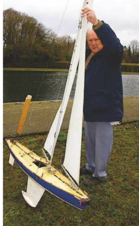
M Class Gretel - This is a modified Elusive that was produced by Albert Sinar and Ron Harris from the original Gretel that my brother George and I sailed that first time. I have restored it from deck level retaining some of the original fittings. The mast and booms are completely new from my own design. The mast height is 80in (2032mm) in top rig.
