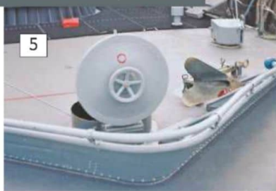
5: A view inboard of the breakwater showing the type of hatches and deck vents fitted to the Type 148.
