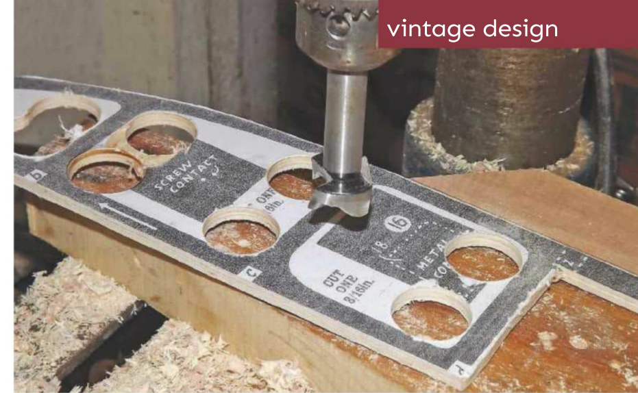
ABOVE: Cutting holes before jigsaw work.
