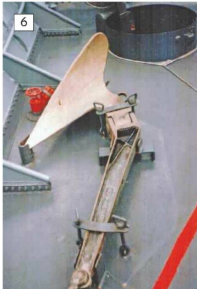
6: The 148s are fitted with plough anchors.
