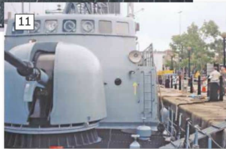
11: Access along the side of the bridge is via these ladders fitted to both port and starboard.
