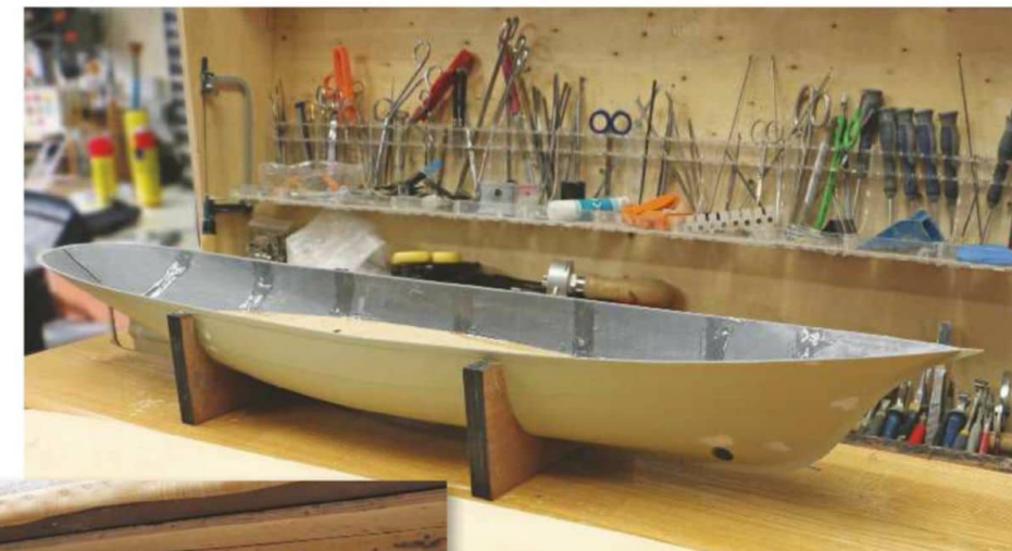
BELOW: 3D printed in sections which are 'welded' together, you can clearly see how the hull of this river launch has been fabricated.
