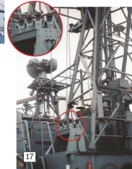
17: Mounted on either side close to the base of the foremast are the six pack decoy launcher.
