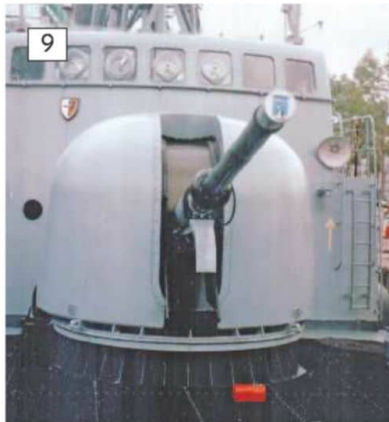
9: This OTO Malera 76mm/62calibre automatic light weight naval gun is in use by many navies around the world.
