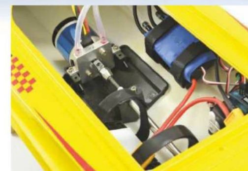
ABOVE: All very neat and tidy inside; note the water-cooled brushless motor and ESC. BELOW: Most useful extras purchased separately; named a pair of Voltz 2200mah batteries and an Etronix Powerpal EZ-4 charger.
