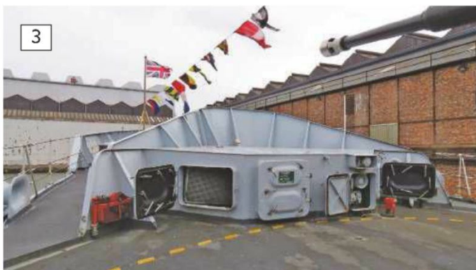
3: The inboard arrangement of the forward breakwater. 4: Affectionately referred to as Kryton, this is the reduced radar cross section turret housing for the Vickers Mk8 dual purpose 4.5in naval gun.
