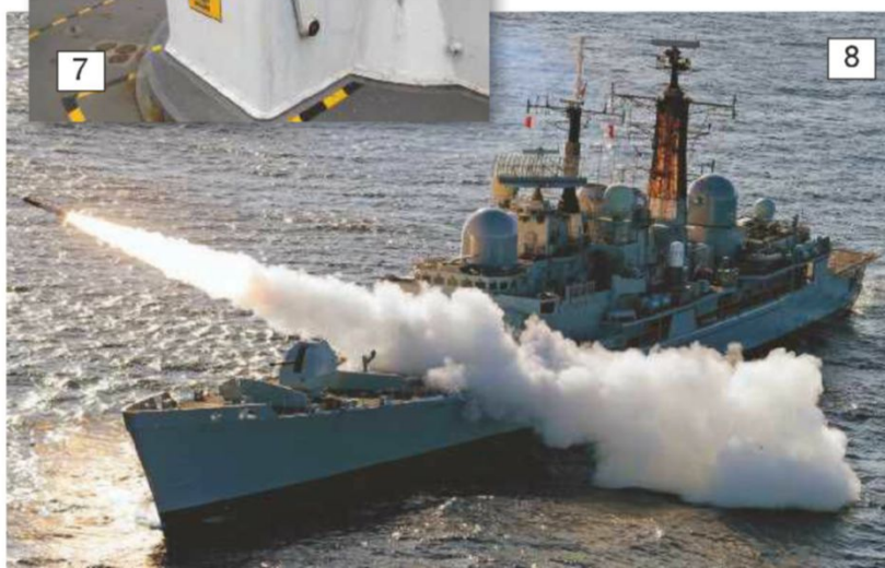
7: These flash doors open out to allow the Sea Dart Missile to engage with the launcher arm.
