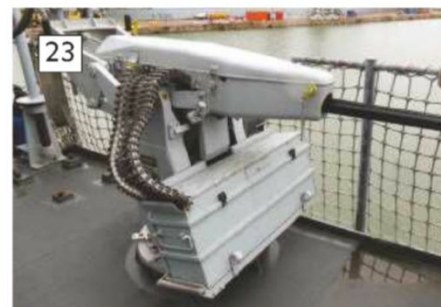
21: The foremast. 23: Mounted on either side on 01 deck is the manually-operated CAM-B01 20mm gun.
