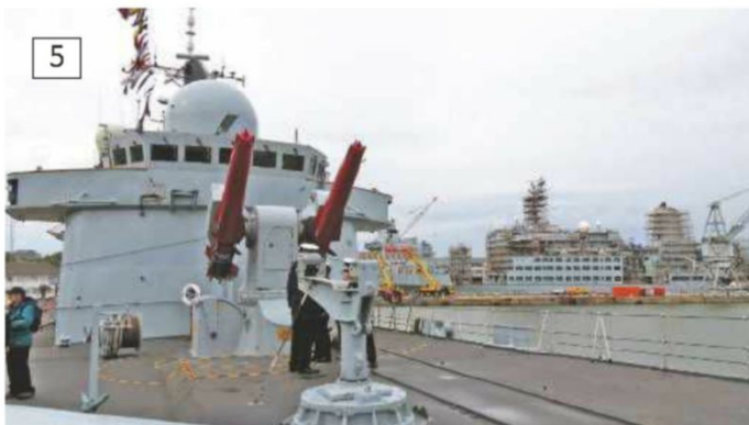
5: Immediately abaft of the second breakwater and, in the foreground of this image, is the RAS (Replenishment at Sea) arm. 6: A shot of the Sea Dart launcher revealing plenty of detail.
