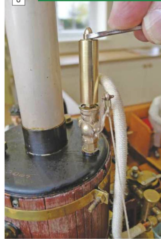
8: With the boiler up to pressure the operating arm can be touched to test the whistle. Slackening off the top nut and screwing the brass cylinder up and down can vary the tone of the whistle to your preference. Always make sure there is enough thread left available for the nut to lock on to.
