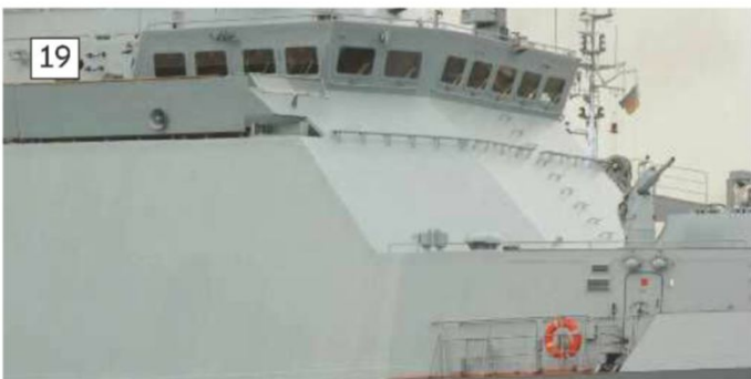
19: Seen on the full-size ship is how the sloping frontage butts up against the lower half of the bridge window surround. 20: This section of the sloping side fits to port but measurements are critical. 21: With the bridge frontage in place the rest of the deck housings thus far prepared are temporarily fitted into place. 22: A view along the starboard side of the prepared deck housings; in the background is the drawing used for the construction of this model.
