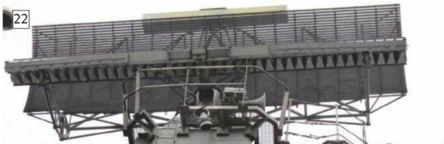
19: The SCOTT dome platforms for satellite communication. 20: A view around the foremast which included the signalling platform. 22: Surveillance and target indication radar was the 1022. A challenging array to make from scratch but a photo etch fret is available. Mounted on the top of the array, is the Mk10 IFF interrogator.
