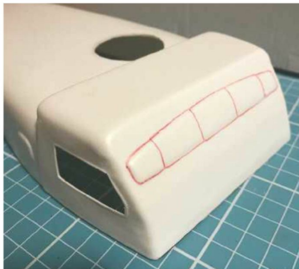
ABOVE LEFT: Areas to be removed internally are marked in red pen. ABOVE RIGHT: The cockpit windscreen marked ready for removal, note that the turret tub and side window have already been cut away.
