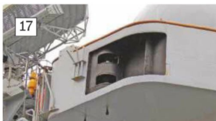
17: A detailed view of the starboard navigation lights. 18: A life buoy chute might be considered vintage technology, but even the Type 45 has them fitted.
