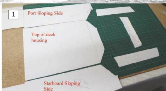
1: The outer cladding for the sloping sides and top of the deck housing. 2: Each side is worked to suit the deck sheer.
