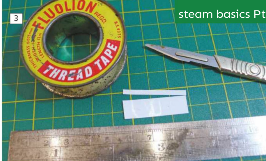
3: I'll probably get comment again regarding the age of my thread tape reel. I have had it for over 40 years and it is still the best way to seal a steam thread.
