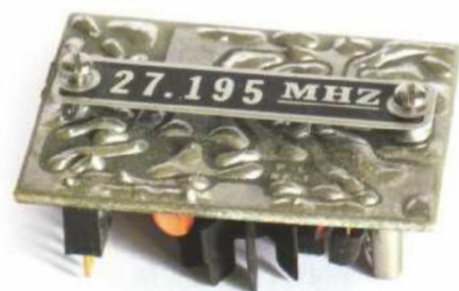
A new 27MHz RF deck (pcboard) for a mid-1970's Pro-Line radio transmitter.
