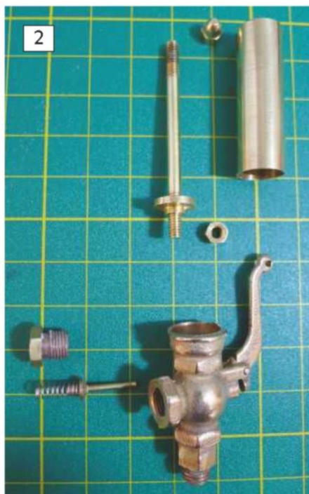
2: Most model boat whistles tend follow this basic layout in one way or another. At the bottom is a valve, which sits on a rubber seat and is held in place by a spring. The lever acts on the end of the valve spindle to lift the valve and let the steam into the resonating chamber, created by the brass cylinder.
