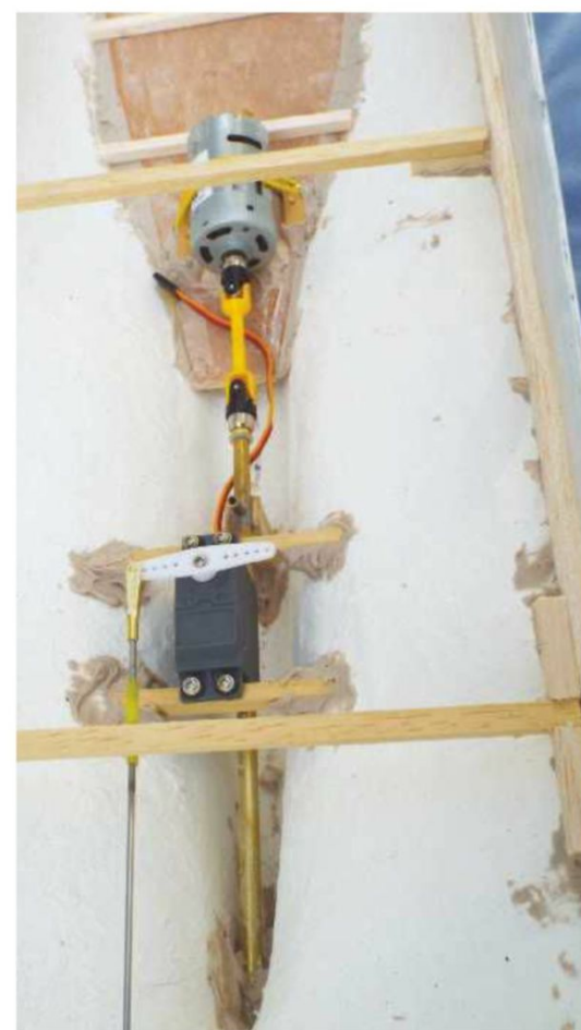
ABOVE: Running gear fitted.
