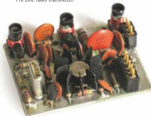
A new 27MHz RF deck (pcboard) for a mid-1970's Pro-Line radio transmitter.
