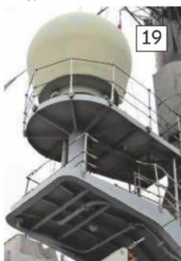
19: The SCOTT dome platforms for satellite communication. 20: A view around the foremast which included the signalling platform. 22: Surveillance and target indication radar was the 1022. A challenging array to make from scratch but a photo etch fret is available. Mounted on the top of the array, is the Mk10 IFF interrogator.
