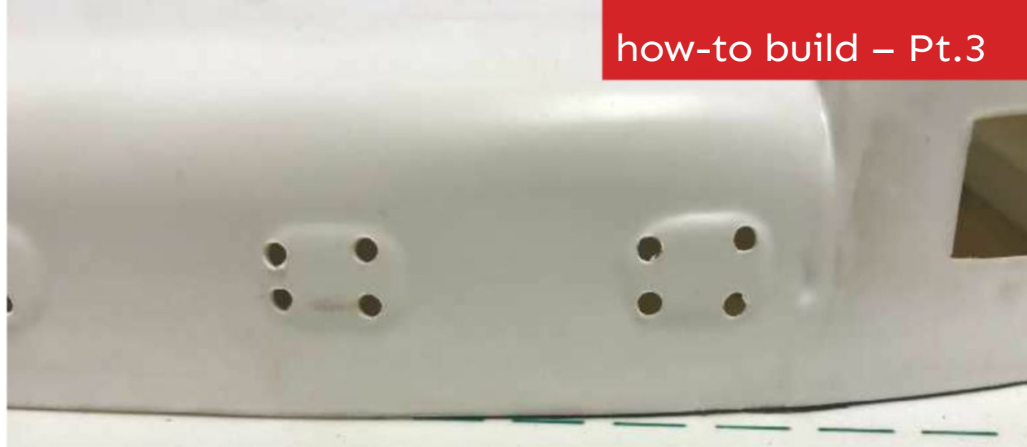
ABOVE: The cabin windows drilled in each corner.
