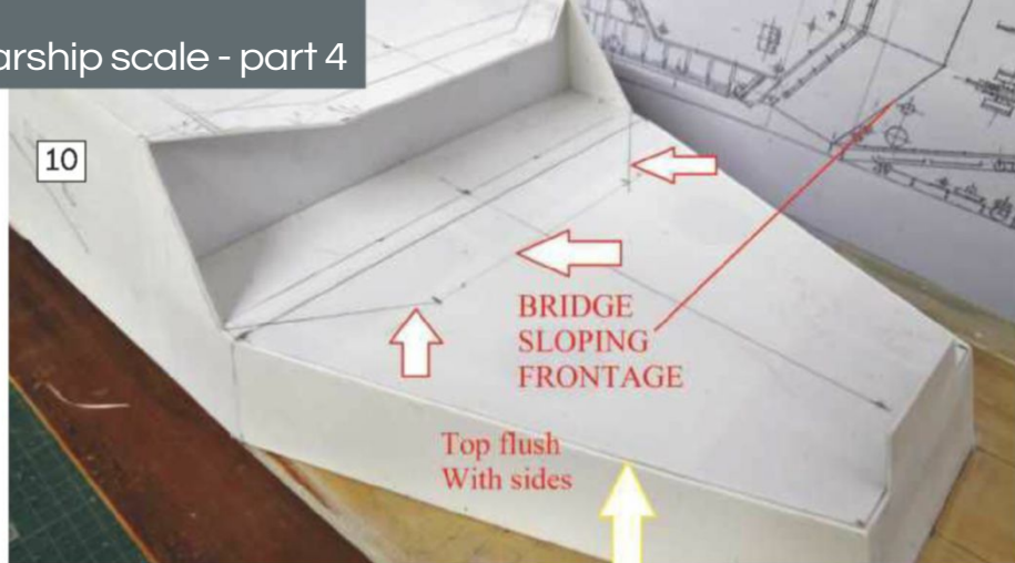
10: A good fit within the top of the VSL deck housing. 11: All the parts that will form the bridge are ready for assembly.
