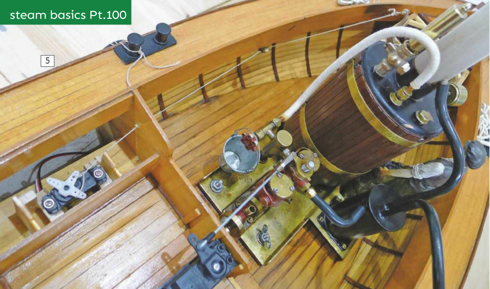
5: Simple is best. If you can use only a single pulley so much the better as there is less stress on everything and more chance of things working reliably. The cord should be always under a slight degree of tension to prevent it coming off the pulley and the brass thimble should help prevent chaffing.
