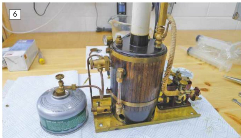
6: Bench testing is always worthwhile and is why the plant should always be easily removable. This plant comes out of the boat, complete, in less than a minute so can be run on the bench to test anything you might want to have a play with. 7: Descaling tablets are easy to get from most hardware stores and a lot of places that sell coffee machines. I use them to clean boilers as well as most steam related fittings such as safety valves.
