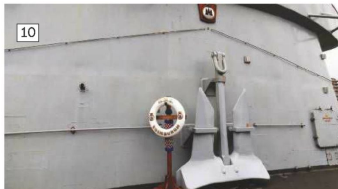
9: Bridge frontage. 10: Spare AC14 holding-type stockless anchor. 11: Bridge front over to port. 12: A general view along the starboard side.
