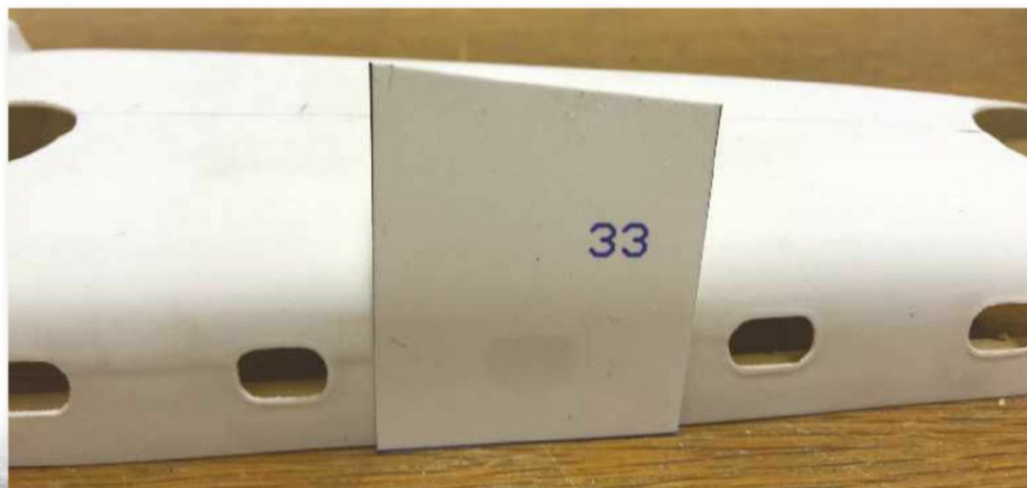
ABOVE: And finished, a file creates the oval window. BELOW: The template mentioned in the main text for the sickbay hatch.
