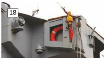
17: A detailed view of the starboard navigation lights. 18: A life buoy chute might be considered vintage technology, but even the Type 45 has them fitted.
