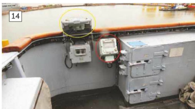
13: Starboard side looking forward on the bridge wing. 14: Port side bridge wing aft; in the frame is the Pelorus ringed in yellow with the rudder angle indicator ringed in red. 15: Of its time, analogue instrumentation. 16: Starboard bridge wing.
