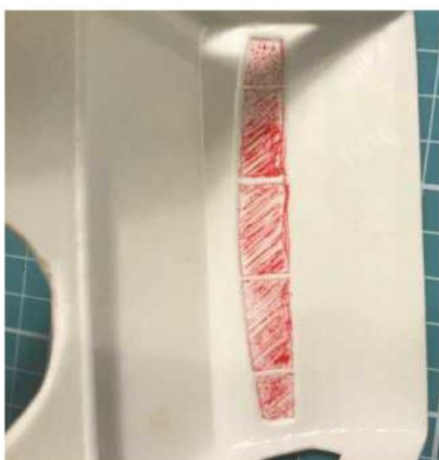
ABOVE: The inside view of the windscreen showing the area to be removed; not easy on the hands!
