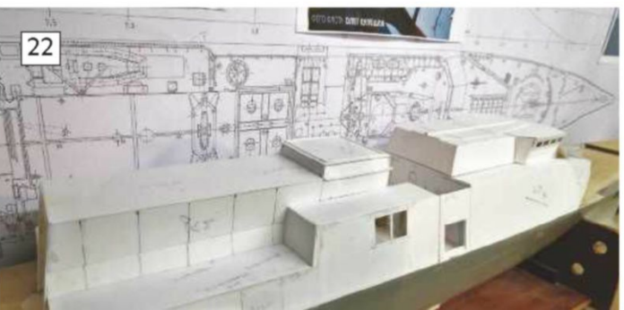
19: Seen on the full-size ship is how the sloping frontage butts up against the lower half of the bridge window surround. 20: This section of the sloping side fits to port but measurements are critical. 21: With the bridge frontage in place the rest of the deck housings thus far prepared are temporarily fitted into place. 22: A view along the starboard side of the prepared deck housings; in the background is the drawing used for the construction of this model.
