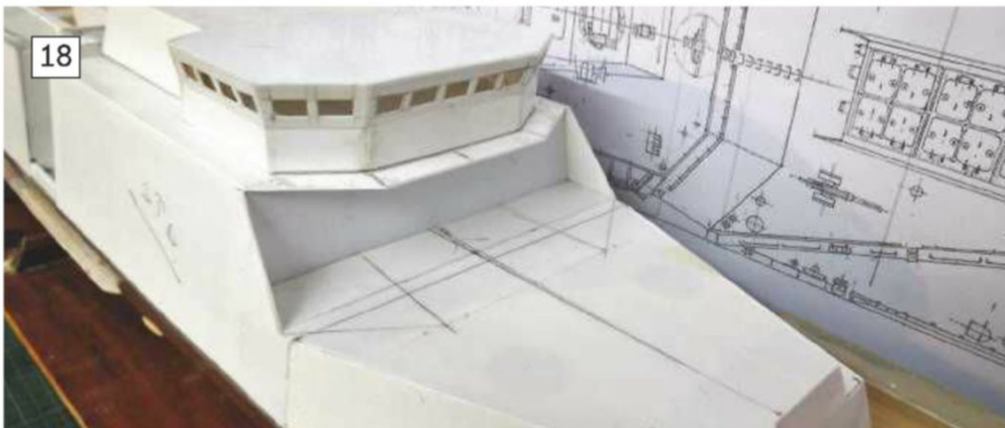
18: Here the bridge housing is located. It's worth noting that the bridge is set back from the edge of the top of the superstructure.
