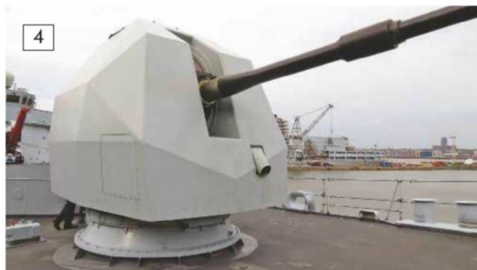
3: The inboard arrangement of the forward breakwater. 4: Affectionately referred to as Kryton, this is the reduced radar cross section turret housing for the Vickers Mk8 dual purpose 4.5in naval gun.
