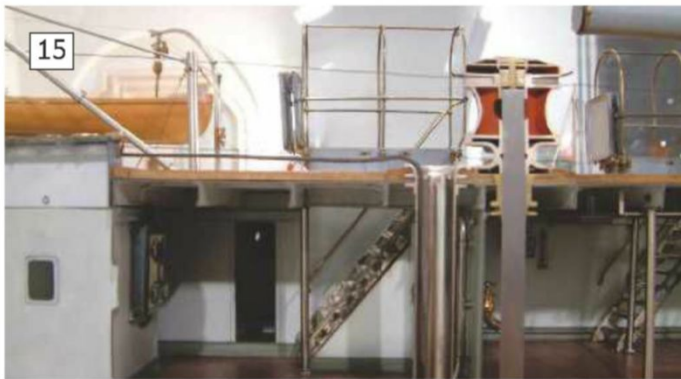
13: The engineering for training and elevating the main armament. 14: After accommodation ladder and associated davit. 15: On the quarter deck is the aft cable holder with the deck pipe leading below decks. 16: Right aft the Captains accommodation in miniature.
