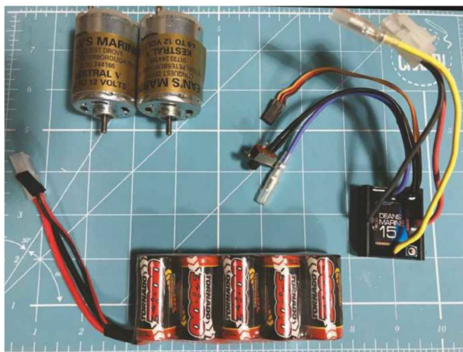
ABOVE: An electrical diagram showing the proposed layout for the RC equipment. BELOW: The basics required to power the model: motors, battery and ESC.
