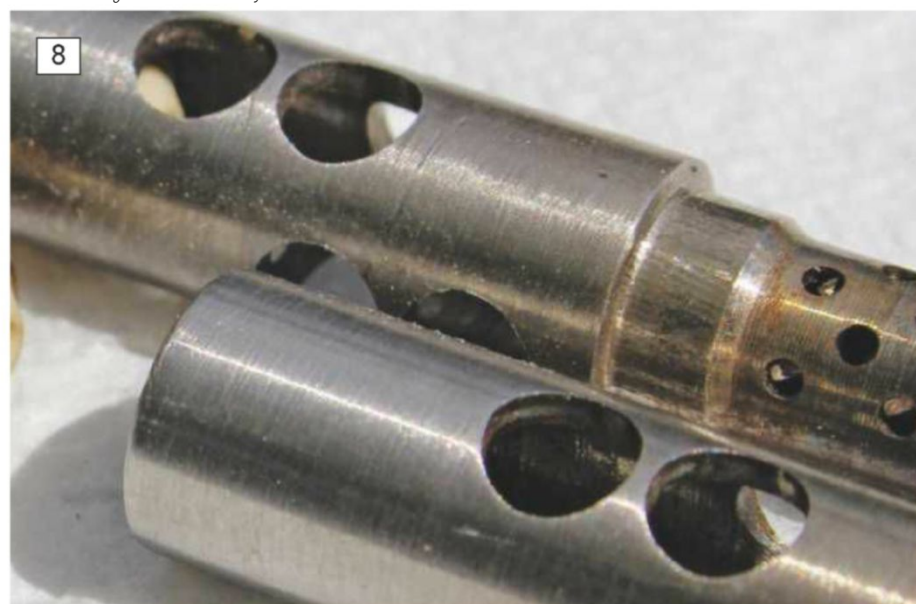
8: The air holes on the twin poker burner. These are not an adjustable type with the optimum position of the jet being designed into the device to give the best performance. The holes must remain unobstructed in the model and adequate ventilation provided to allow the best flow of air.
