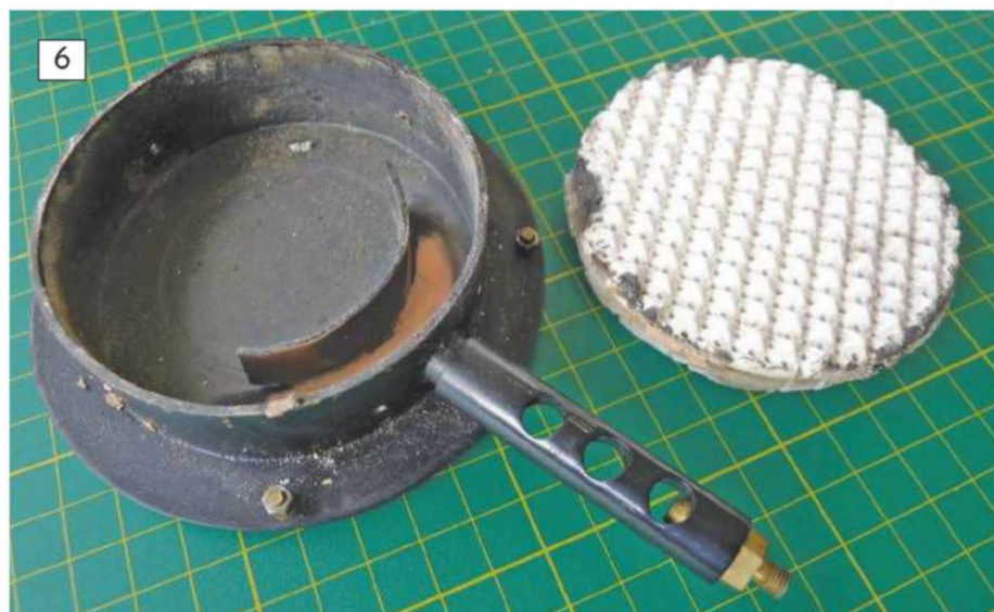
6: The ceramic discs are easily replaceable and can even be trimmed to suit the size of your burner perfectly. They should be set in a high temperature sealant such as that supplied for fitting the rope seals around the doors of wood burning stoves.
