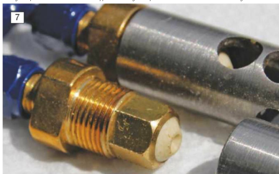
7: Removing the poker tube reveals the jet unit, screwed into the holder. The jet size will be stamped on one of the flats in the form of a number. The larger the number, the bigger the jet diameter. Clean with warm soapy water and then compressed air, I would advise against the use of any mechanical tool.
