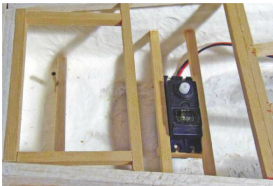
RIGHT: A step backwards to last month to show the structure supporting the re-located servo.
