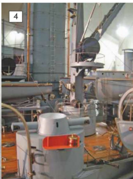
2: Viribus has four powered pinnaces and two enclosed two open. 3: The open powered pinnace. 4: Inboard of the deck edge range finder for the 15cm waist guns is the crane for shipping the ships boats. 5: Starboard side amidships an almost complete internal arrangement showing engine and boiler rooms. 6: Part of the boiler room.
