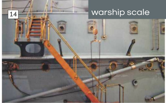
13: The engineering for training and elevating the main armament. 14: After accommodation ladder and associated davit. 15: On the quarter deck is the aft cable holder with the deck pipe leading below decks. 16: Right aft the Captains accommodation in miniature.
