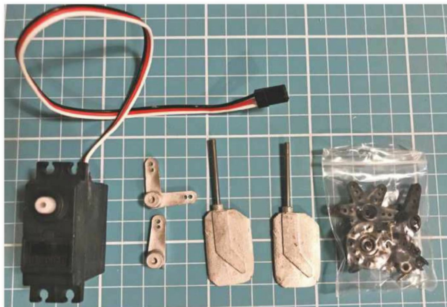
LEFT: The steering system: a servo, servo arms, rudders and tillers (these were replaced later with plastic items).
