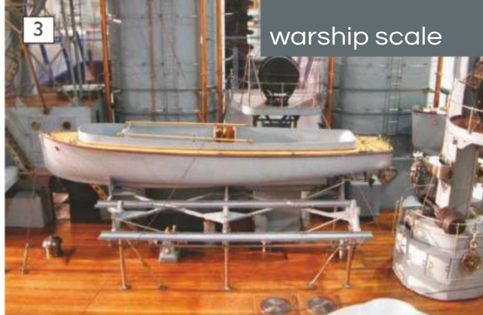
2: Viribus has four powered pinnaces and two enclosed two open. 3: The open powered pinnace. 4: Inboard of the deck edge range finder for the 15cm waist guns is the crane for shipping the ships boats. 5: Starboard side amidships an almost complete internal arrangement showing engine and boiler rooms. 6: Part of the boiler room.
