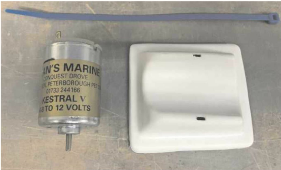
ABOVE LEFT: The components required to mount the motors in position: the mount, motor and the tie-wrap. ABOVE RIGHT: The motor on its mount; don't forget to cut the tie-wrap tag off to make it neat and tidy.
