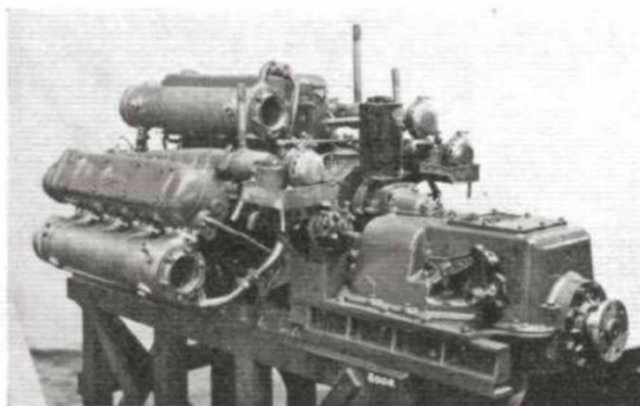
A three-quarter view of the "Sea Lion" which gives a good idea of how accessible are the carburettors and other vital parts of the engine.
