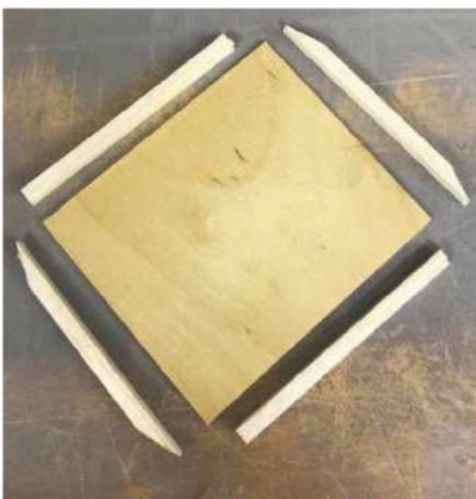
The bits and pieces I used to make my RC tray: 1/16in plywood and pieces of balsa.
