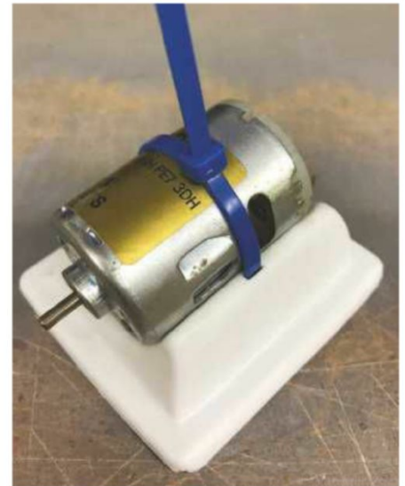
ABOVE LEFT: The components required to mount the motors in position: the mount, motor and the tie-wrap. ABOVE RIGHT: The motor on its mount; don't forget to cut the tie-wrap tag off to make it neat and tidy.
