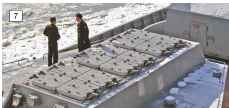
6: Elevated deck housing containing 12 Redut VLS cells each housing a medium-range SAMs of the S-400 system 9M96E2 with a range of 120km (NATO SA-21 Growler). 7: The 12-silo door REDUT system forward of the bridge.
