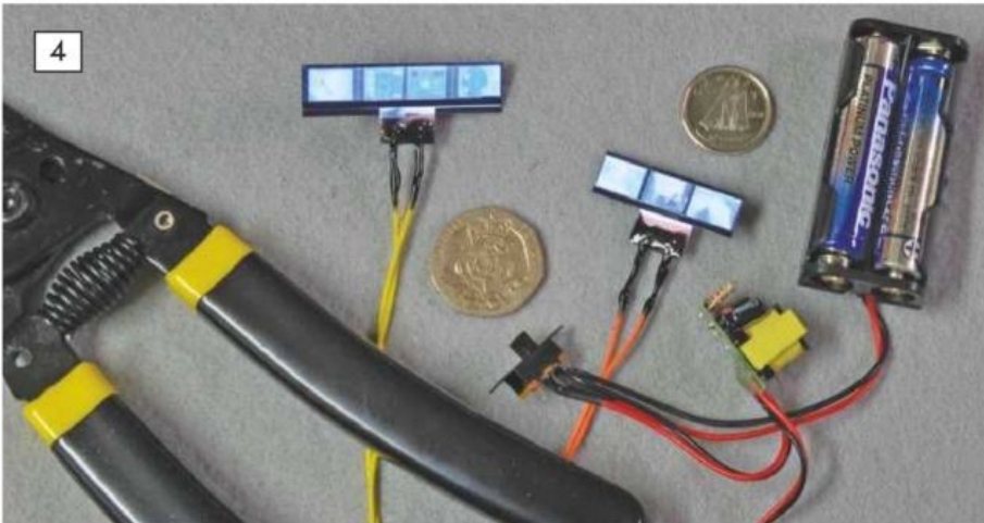
4: Bridge display panels and temporary power supply. The printed film should have had a yellow tint to offset the pale blue of the EL panel.
