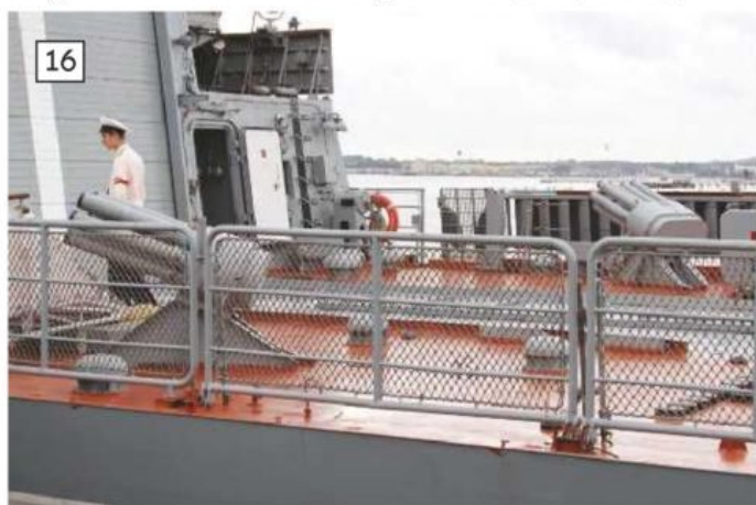
16: Surrounding the edge of the flight deck are sections of round bar collapsible barriers. 17: In comparison to NATO naval vessels the space within the hangar is restrictive but can accommodate the KA-27 ASW helicopter. 18: Although a small warship the Steregushchy class possess a good area of flight deck.
