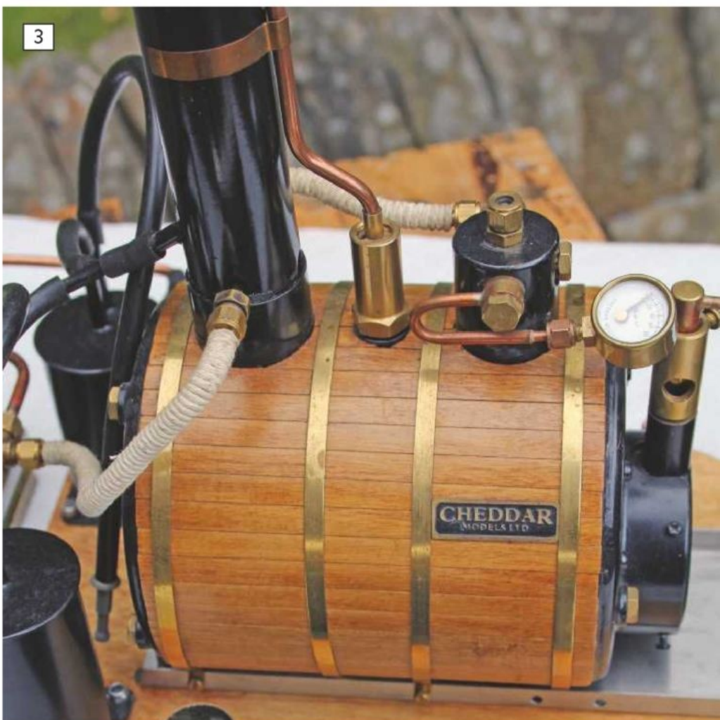
3: The old Cheddar Proteus boiler is one that falls above the 3 bar litre limit and so requires regular hydraulic pressure testing according to the requirements laid out in Volume 1.
