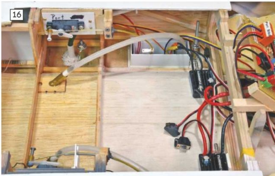
15: Seaframe testing begins on the pond. 16: An internal view of the port side of the body, above where the waterjet box is attached.
