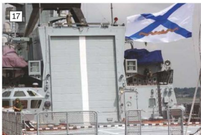
16: Surrounding the edge of the flight deck are sections of round bar collapsible barriers. 17: In comparison to NATO naval vessels the space within the hangar is restrictive but can accommodate the KA-27 ASW helicopter. 18: Although a small warship the Steregushchy class possess a good area of flight deck.
