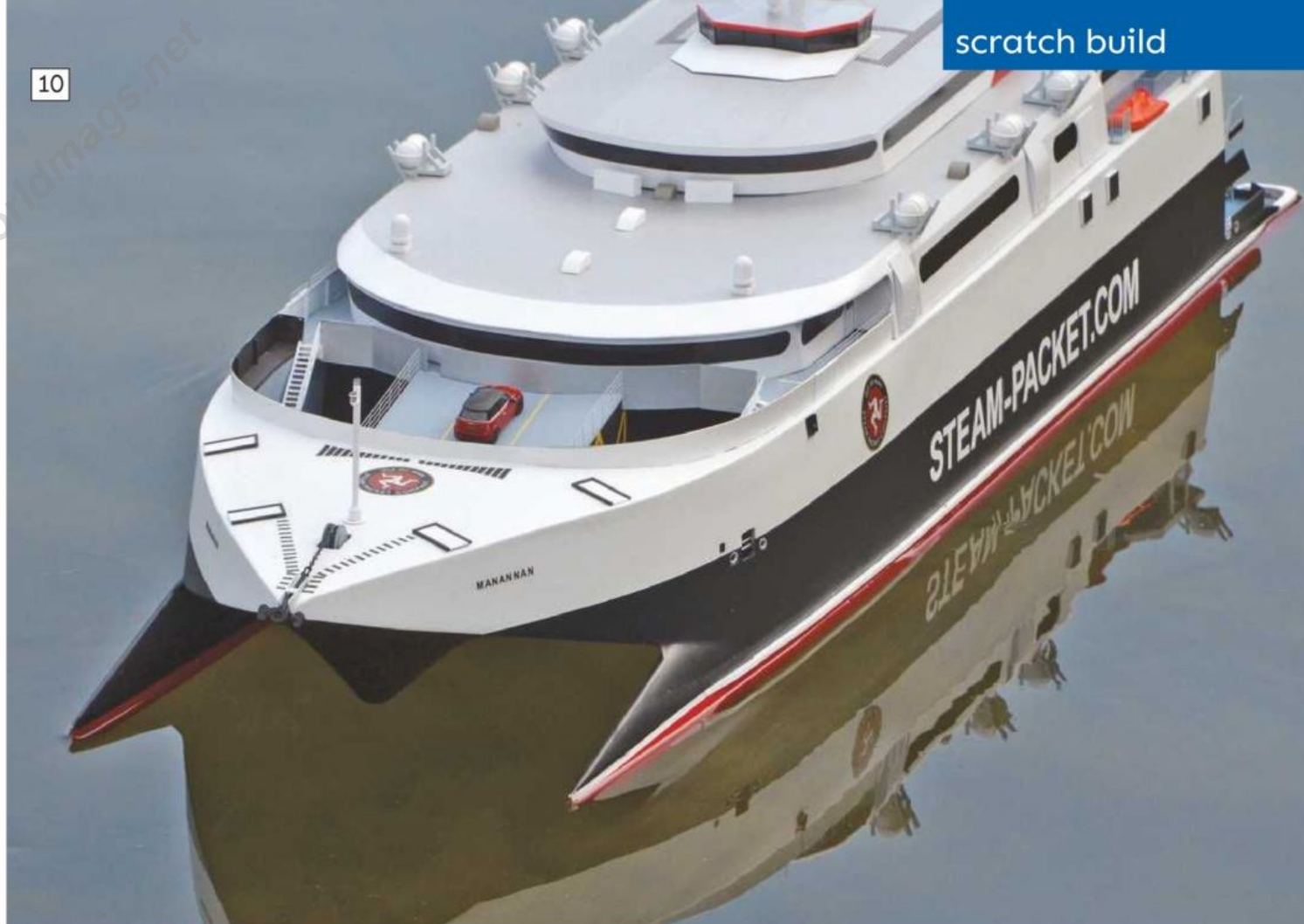
10: Bow view; the 'chunky' plastic steps will be replaced by etched metal. 11: Foremast and socket under construction.
