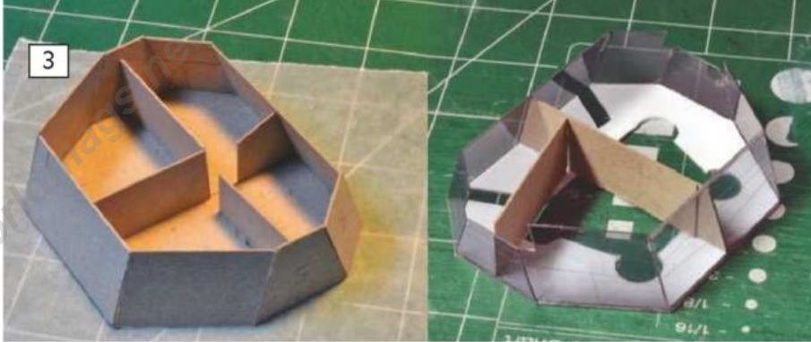
3: On the left a cardboard mock-up of the wheelhouse, on the right the basic shell with internal temporary supports; both upside down.
