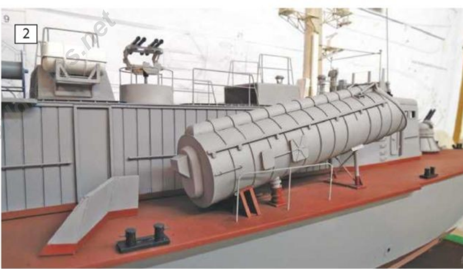
2: Whilst most of the smaller fittings can be permanently fixed larger fittings such as the launch tubes need to be removable to allow for fixing the stanchions and flexible rail.
