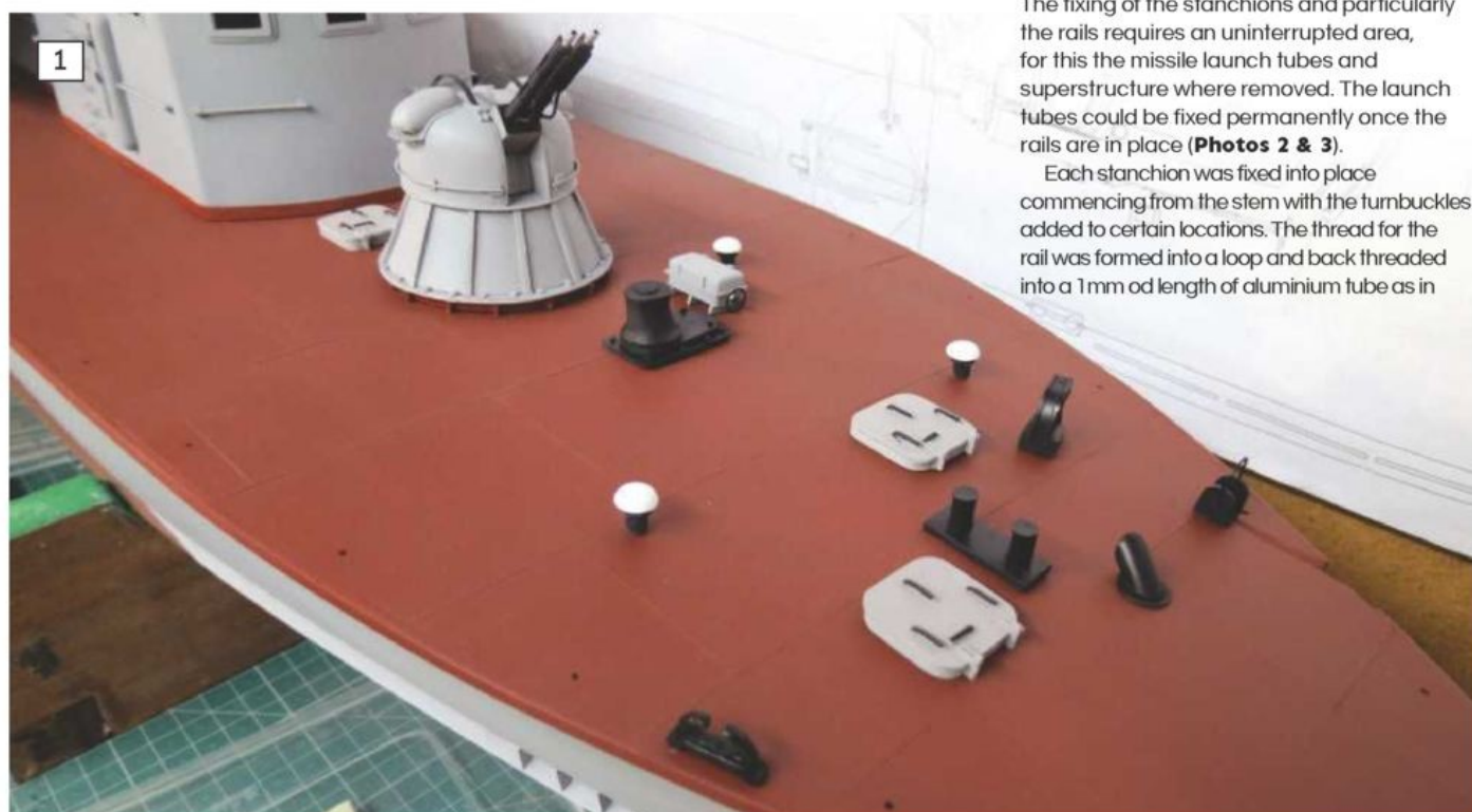
1: Some of the fittings pin fixed to the forecastle deck in pre-prepared locations.
