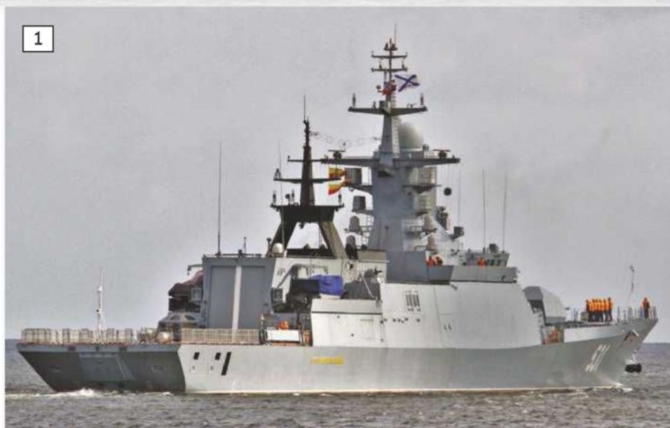
1: A starboard side image which gives a good impression of the use of sloping surfaces to reduce the radar cross section of the ship.
