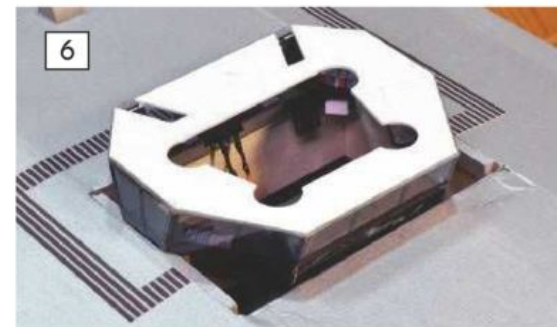
6: Trial fit of the partially-completed wheelhouse atop the passenger space.
