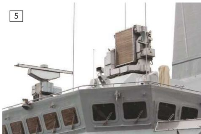
4: A further perspective on the turret housing for the 100mm naval gun. In the background is one of two saluting guns. 5: PUMA (NATO Hot Flash) fire control radar for the 100mm gun and navigation radar. Target detection range is up to 60 km.
