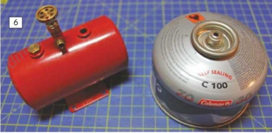
6: Volume 3 covers gas tanks below 250ml such as these two. The disposable tank on the right is exempt from any certification and the manufactured tank on the left, if supplied with a manufacturer's hydraulic test certificate, requires only five yearly certificated safety checks.
