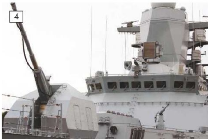
4: A further perspective on the turret housing for the 100mm naval gun. In the background is one of two saluting guns. 5: PUMA (NATO Hot Flash) fire control radar for the 100mm gun and navigation radar. Target detection range is up to 60 km.
