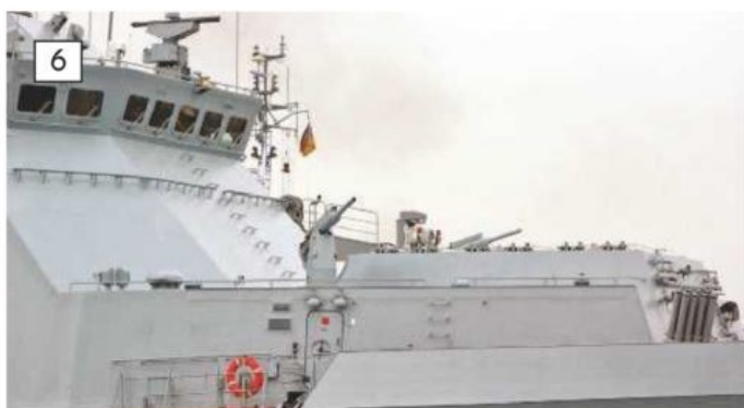
6: Elevated deck housing containing 12 Redut VLS cells each housing a medium-range SAMs of the S-400 system 9M96E2 with a range of 120km (NATO SA-21 Growler). 7: The 12-silo door REDUT system forward of the bridge.
