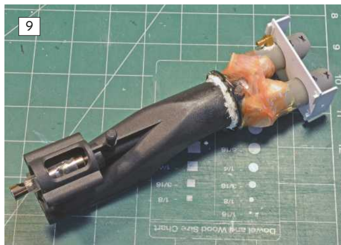
8: The first stage in assembling the twin discharge tubes to the waterjet. The centre and top transition pieces were glued in first, then the waterjet/tubes assembly was removed from the holding fixture and the bottom pieces glued. 9: One completed waterjet assembly with an end plate trial fitted.
