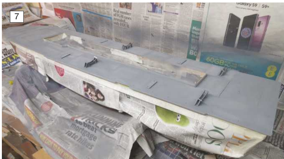
7: Masking of the lower part of the hull using a combination of Tamiya Low Tak and conventional masking tape.
