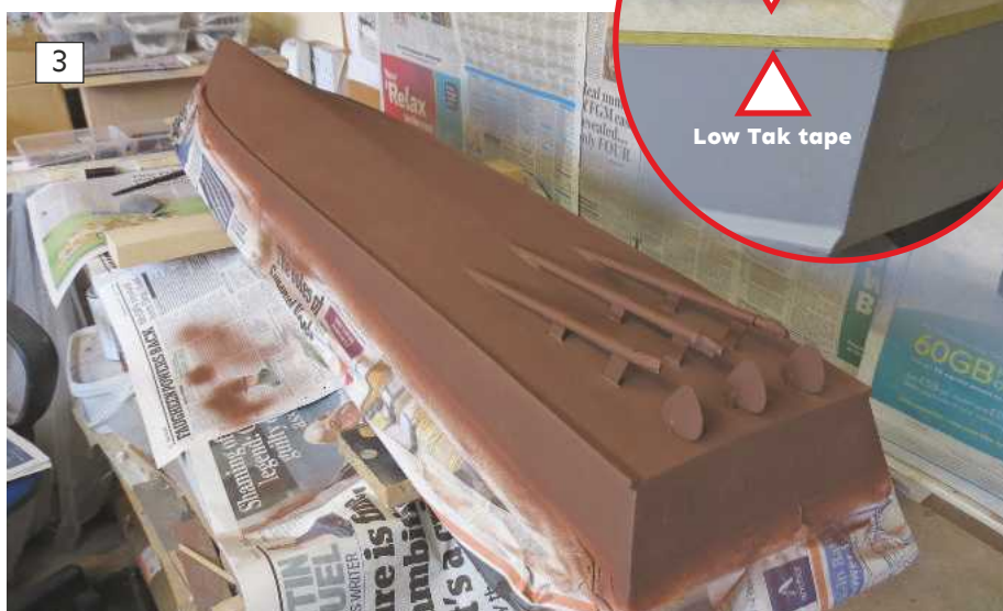
3: The hull is placed keel up and the brown-red acrylic anti-foul is applied in two consecutive coats.
