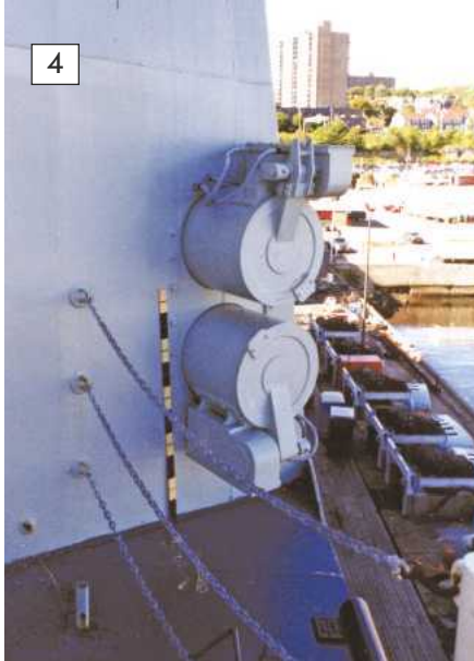
4: Two fixed torpedo tubes either side of the after-deck housing. Jonathan Evens. 5: The area atop of the hanger, which included fire control radar, Sat nav domes, navigation radar and close in weapons system. 6: The Phalanx Mk15 MOD 1. 7: The front of the hanger, it's worth noting in comparison to other frigates the substantial diameter of the stanchions for the crash barriers.
