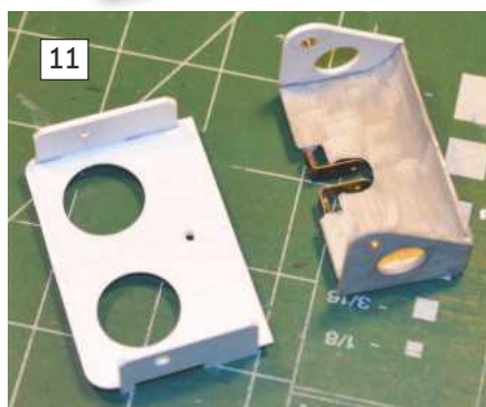
11: An end plate (outer face up) with a reversing bucket built from styrene, shown with their top edges together.
