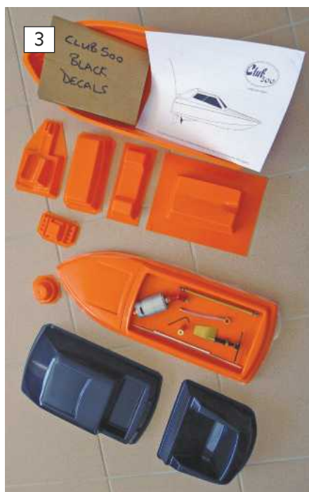
3: The basic parts of a Club 500 kit. The deck is usually the same colour as the cabin and wing but the parts are always the same. The only difference in the build is really the care and attention that goes into it to ensure everything is perfectly aligned and smooth in operation.
