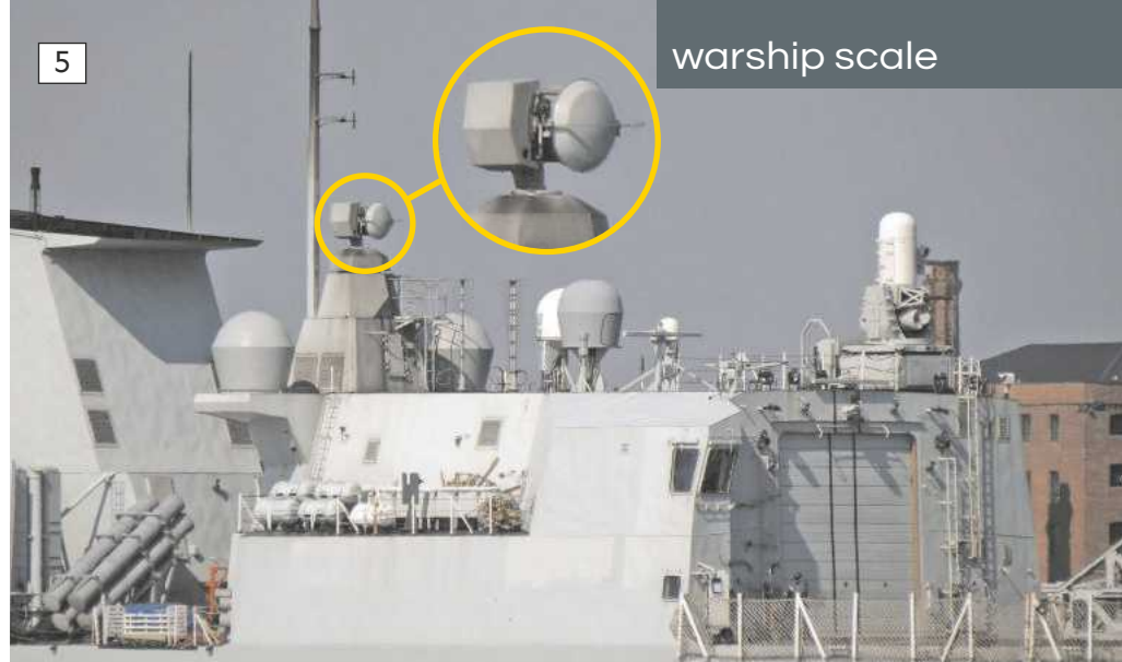
4: Two fixed torpedo tubes either side of the after-deck housing. Jonathan Evens. 5: The area atop of the hanger, which included fire control radar, Sat nav domes, navigation radar and close in weapons system. 6: The Phalanx Mk15 MOD 1. 7: The front of the hanger, it's worth noting in comparison to other frigates the substantial diameter of the stanchions for the crash barriers.
