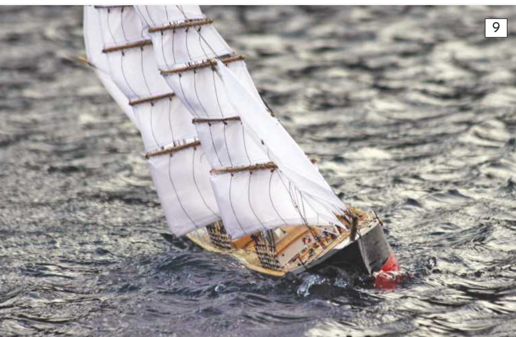
9: A model of the Grain Race barque, 'Penang', taking solid water on to the main deck. You can readily appreciate why it's important to seal the decks. 10: The four-masted barquentine 'Mozart' heeled right over, beating on the port tack.
