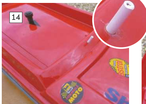
13: There is a white plastic tube supplied in the kit specifically for the purposes of making locating pins. The two at the back of the boat simply slot into two holes drilled into the cabin. 14: The forward end of the cabin has a single hole drilled into it to locate onto the front pin. When in place the cabin is surprisingly secure and yet very quick and easy to remove.
