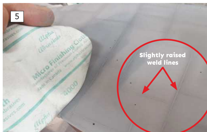
5: Micro Finishing cloth 4000 grade is used to prepare the deck surface for its finishing coat. 6: The primed deck surface is rubbed down with a Micro finishing cloth.
