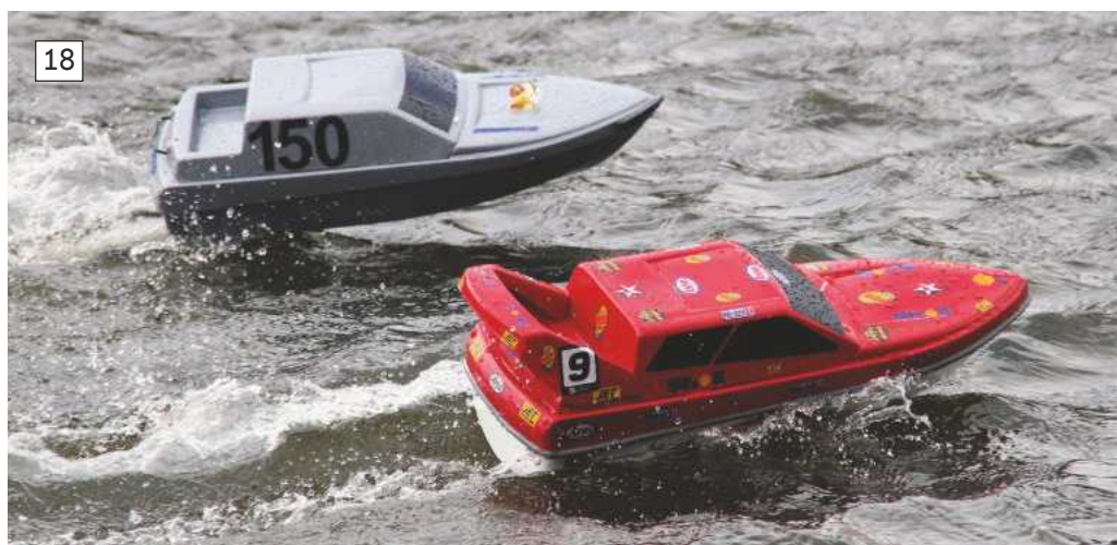
18: Trials are as much about setting up the boat as it is about getting a feel for how to handle it and make the most of available conditions. Avoid all other objects, either fixed or moving and try to make the most of the surface conditions. Set the rudder span to avoid stalling the model round tight corners.
