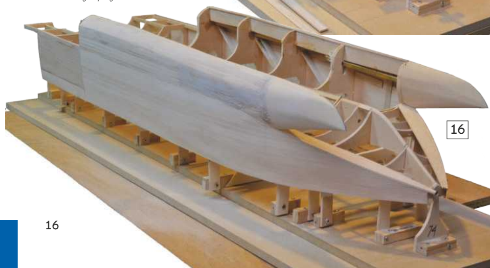
16: Planking in progress.
