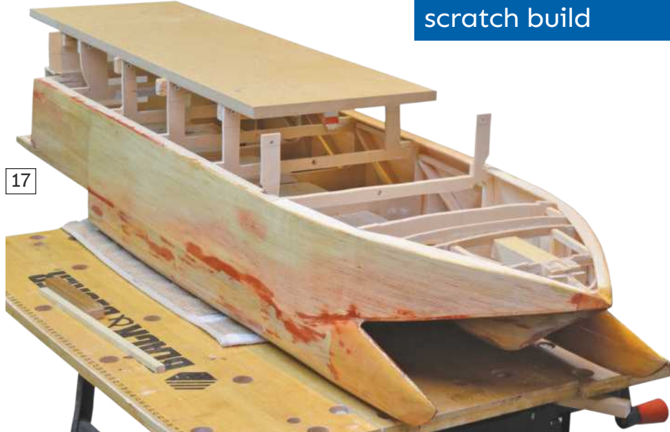
17 The forward part of the building board removed to fit the planks around the top edge of the body, prior to fibre glassing.
