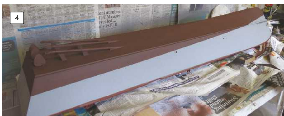
4: All the masking off is removed to give a sharp edge between the anti-foul and the side of the hull.
