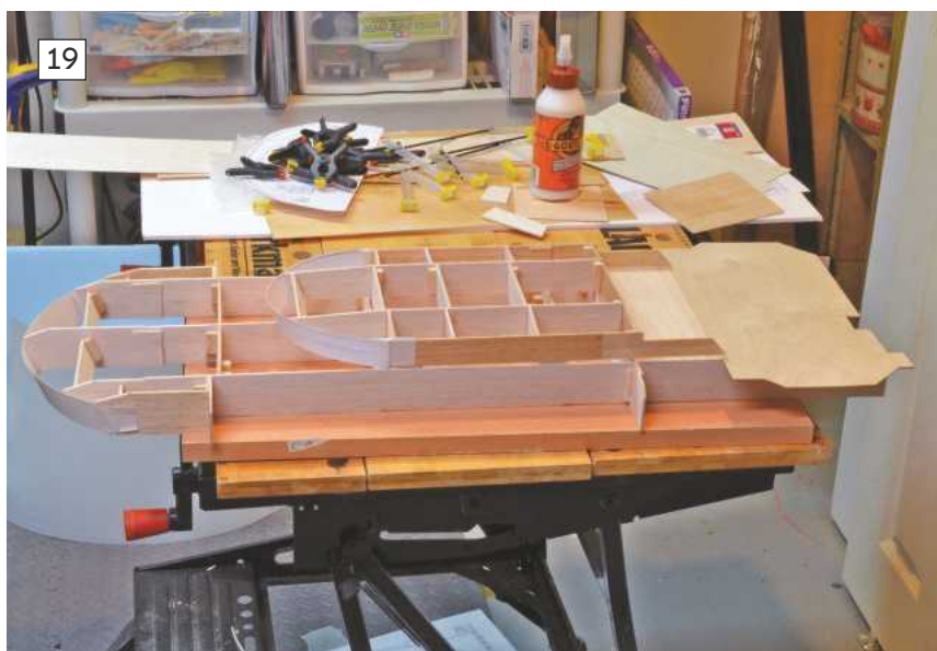
18: Fibre-glassed hull with two waterjet boxes attached and the mounting bolt brackets being glued to the boxes. 19: The structure of the passenger accommodation taking shape. The main structural pieces are the fore-and-aft strips on the lower level.
