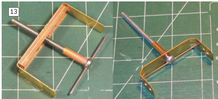
13: Two of the bolt assemblies for securing a propulsion box to the seaframe. Mark 1 version on the left, Mark 2 (lighter) on the right. 14: The makings of the fore end of one of the hulls, showing the nickel silver rib glued to one half of the basswood 'sandwich'.
