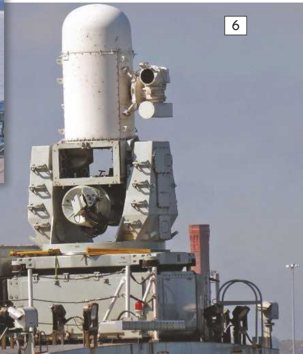
4: Two fixed torpedo tubes either side of the after-deck housing. Jonathan Evens. 5: The area atop of the hanger, which included fire control radar, Sat nav domes, navigation radar and close in weapons system. 6: The Phalanx Mk15 MOD 1. 7: The front of the hanger, it's worth noting in comparison to other frigates the substantial diameter of the stanchions for the crash barriers.
