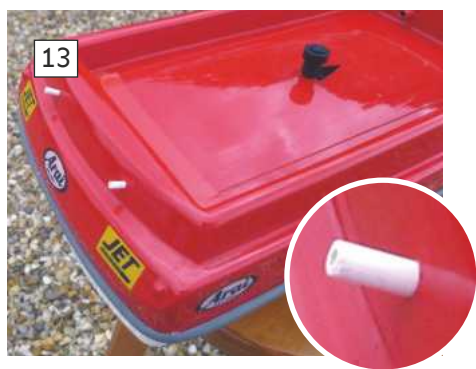
13: There is a white plastic tube supplied in the kit specifically for the purposes of making locating pins. The two at the back of the boat simply slot into two holes drilled into the cabin. 14: The forward end of the cabin has a single hole drilled into it to locate onto the front pin. When in place the cabin is surprisingly secure and yet very quick and easy to remove.
