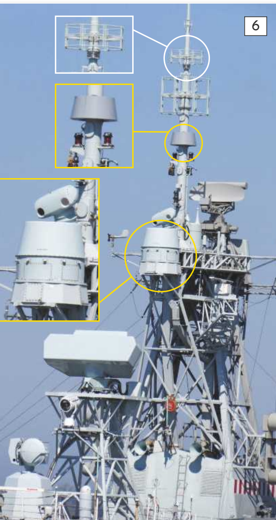
5: Detailed shot of the fire control radar.
