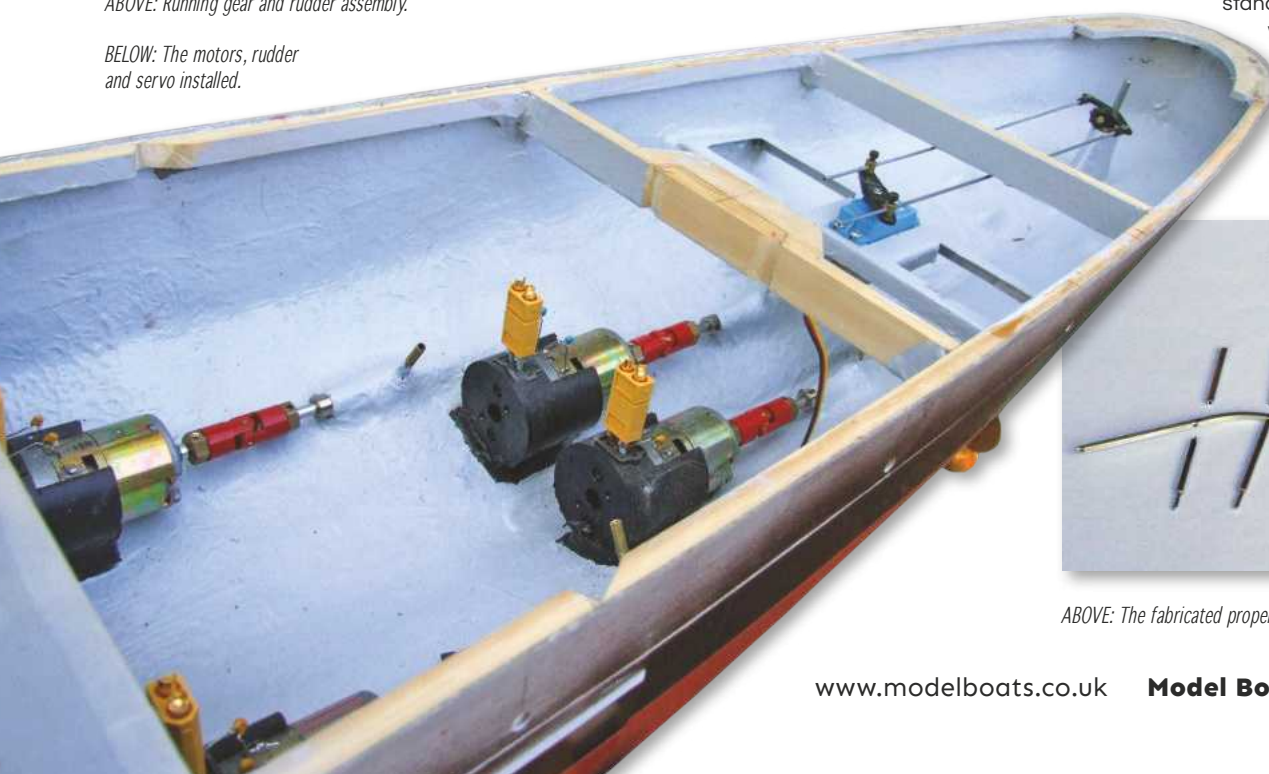
ABOVE: Running gear and rudder assembly.
