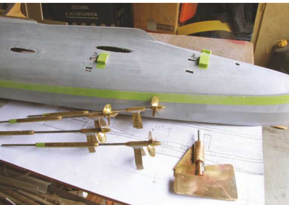
ABOVE: Running gear and rudder assembly.
