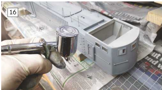
16: Air brushing larger areas using a lever-type air brush. 17: Using MR Hobby acrylic H306 grey for the hull (Alternatively Tamiya Sky Grey XF19).
