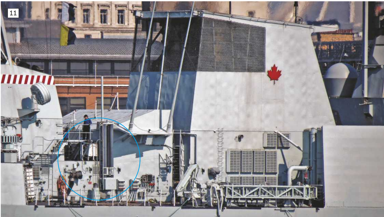
10: X-band navigation radar mounted forward of the lattice mast. 11: Port side RAS (Replenishment At Sea) hoist.
