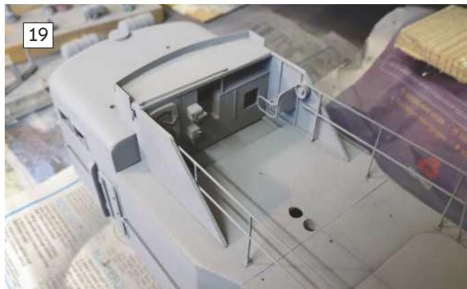
18: Some fittings airbrushed and put to one side after applying just a single coat. 19: Air brushing the interior of the upper wheel house. 20: A good cleaning regime ensures that the air brush will perform well each time.
