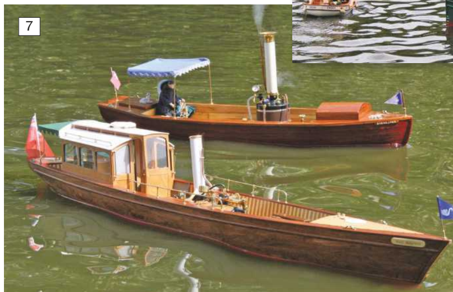
7: Steam models seem to regularly include such stunning scratch built examples as these two beautiful launches, both with lovely plank on frame wooden hulls and lots of fascinating engineering incorporated into their build.
