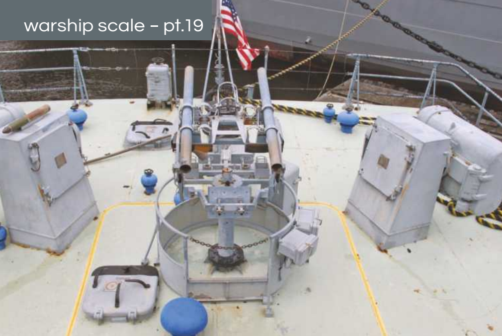
A Strela lightweight SAM system aboard the East German missile corvette the Rudolf Egelhoffer.
