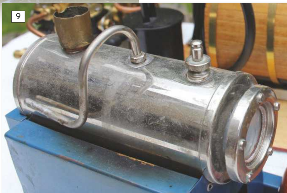
9: There has been a lot of dissent about the inclusion of the simple small boilers such as this Wileco example in the rules but apart from the simplest of steam tests and a very basic checking over there is nothing to really be concerned about.
