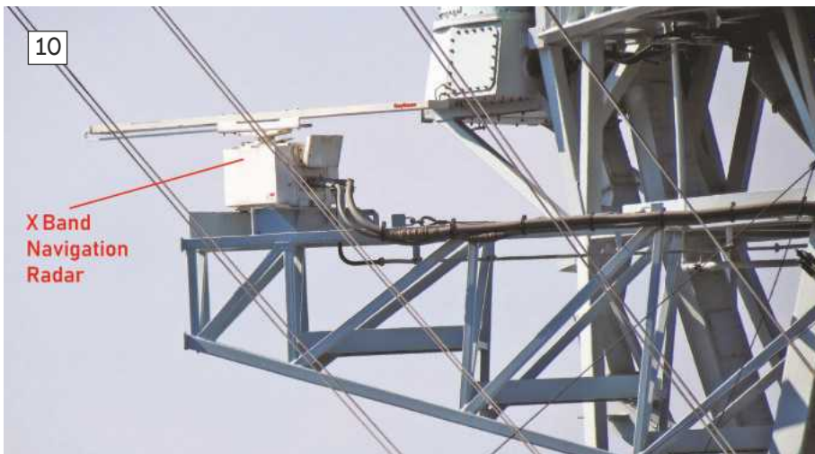
10: X-band navigation radar mounted forward of the lattice mast. 11: Port side RAS (Replenishment At Sea) hoist.
