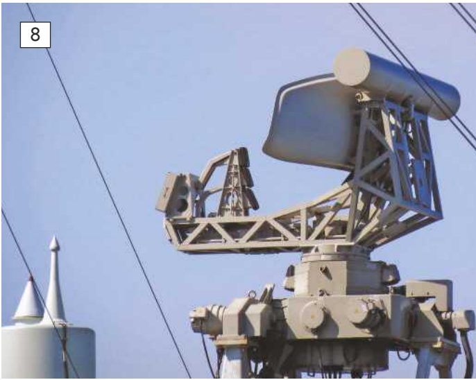
8: From a model maker's perspective, clear images of the upgraded Sea Giraffe search radar. 9: Looking to the rear of the foremast and the mounting for the SIRIUS IR tracker.
