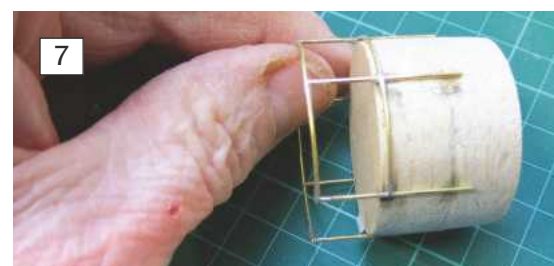
7: Sliding the soldered band stand from the jig.
