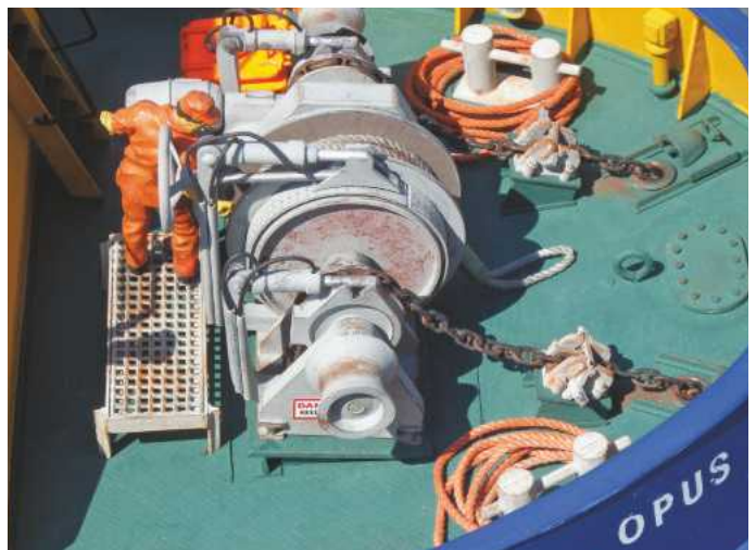
ABOVE LEFT: Superstructure rear, note fire plan tube, fluorescent deck light, funnel ventilators and spooling mechanism to main winch. ABOVE RIGHT: Bow area, note forward winch and cable stoppers. The eyebolt is for bow towing.
