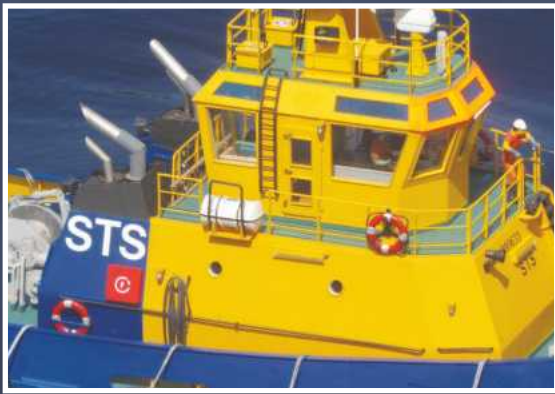
ABOVE: General view of bridge and superstructure, note shore power cable and fluorescent tube deck light.
