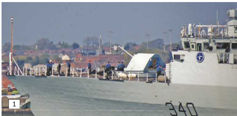
1: Looking towards the forecastle and the Bofors 57mm/70calibre Mk 2. BELOW 2: A general shot of the area around the bridge and port bridge wing.
