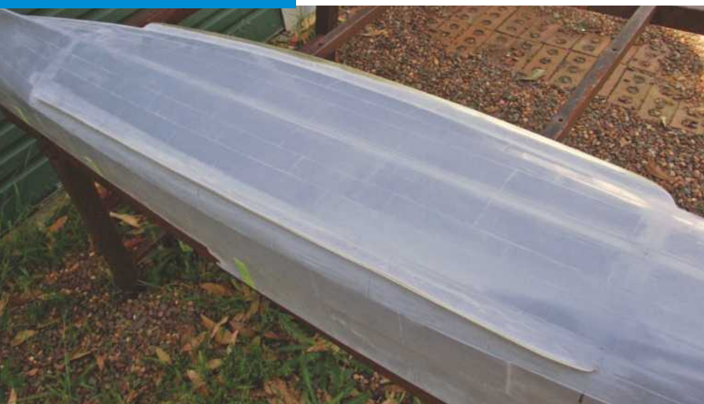
ABOVE: Bilge keels installed.
