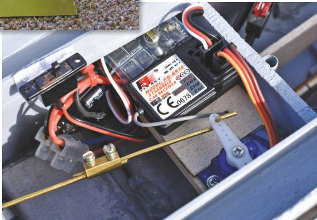
BELOW: Internal detail of the Talisman exposes a small 9g steering servo, a FS 'Fly Sky' (FS-GR3E) 3-Channel Receiver and a 10amp speed controller all neatly installed.
