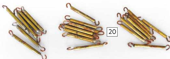
20: The copper wire is formed to the shape of a hook and trimmed to size.
