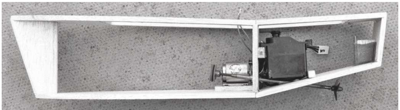
ABOVE: Side view of the original installation which involved a pulley drive system to enable the motor to lie alongside the propshaft and avoid wasting internal space. Glynn Guest
