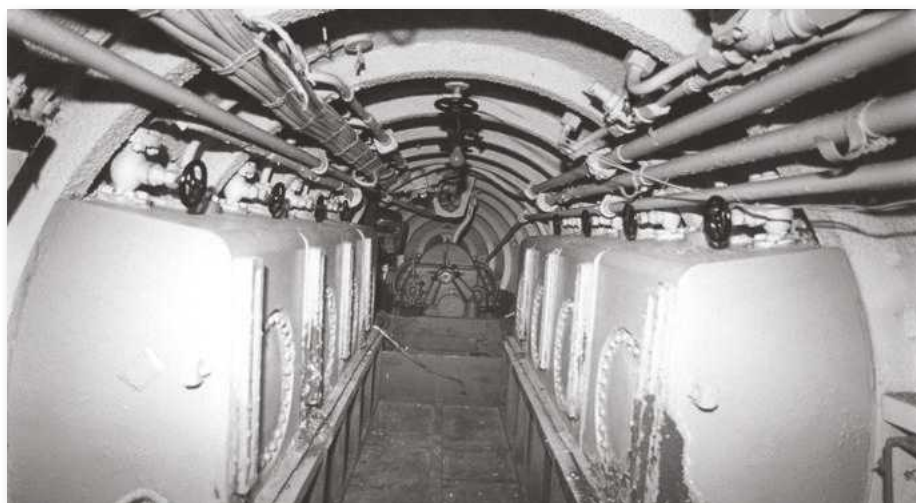
ABOVE LEFT: Interior view looking aft showing rudder control shaft and one of the two motors, driving into a reduction-combining gearbox. Official USN. ABOVE RIGHT: Interior view looking aft amidships, showing twin ballast tanks and battery trough. Official USN
