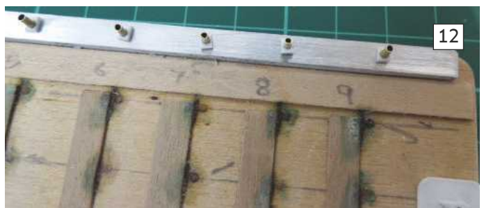
10: Using a curved craft blade the base plate is cut and removed from its jig. 11: Taping the eyes into place on the stanchion and soldered. 12: A length of 1 mm OD brass tube is inserted into the base plate and stored ready to be added to the stanchion.
