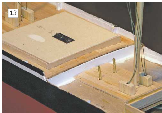
ABOVE LEFT: The on/off switch in a hatch cover and the charging points through the deck. No need to regularly 'go below'. ABOVE RIGHT: A schematic of my method of keeping yard control as intuitive as possible.
