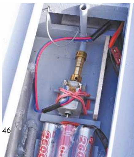
BELOW: An old slot car motor is more than adequate for pushing the Talisman along. Note the battery pack and inline fuse upper left.
