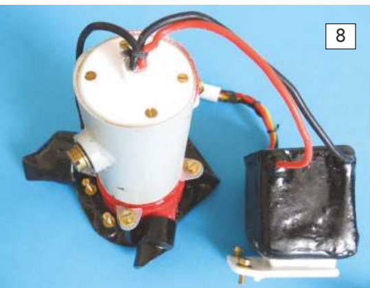
ABOVE: The thruster motor and the sealed black unit which contains the micro servo and micro switch.
