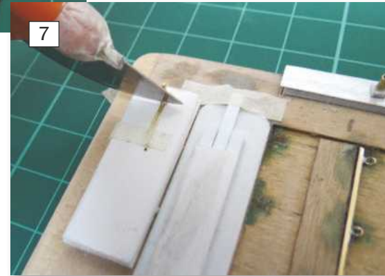
7: Bending the .31 brass wire and cutting to size each of the eyes.
