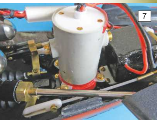
ABOVE: The thruster unit. Un-screwing the four screws allows removal of the thruster and the black servo unit.
