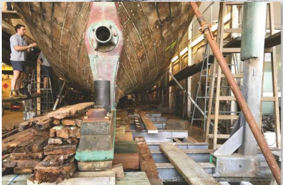
ABOVE: Krait is being extensively repaired before being refloated. A wooden hull ship needs to be in the water to prevent it collapsing under its own weight, or supported in rigid cradle.
