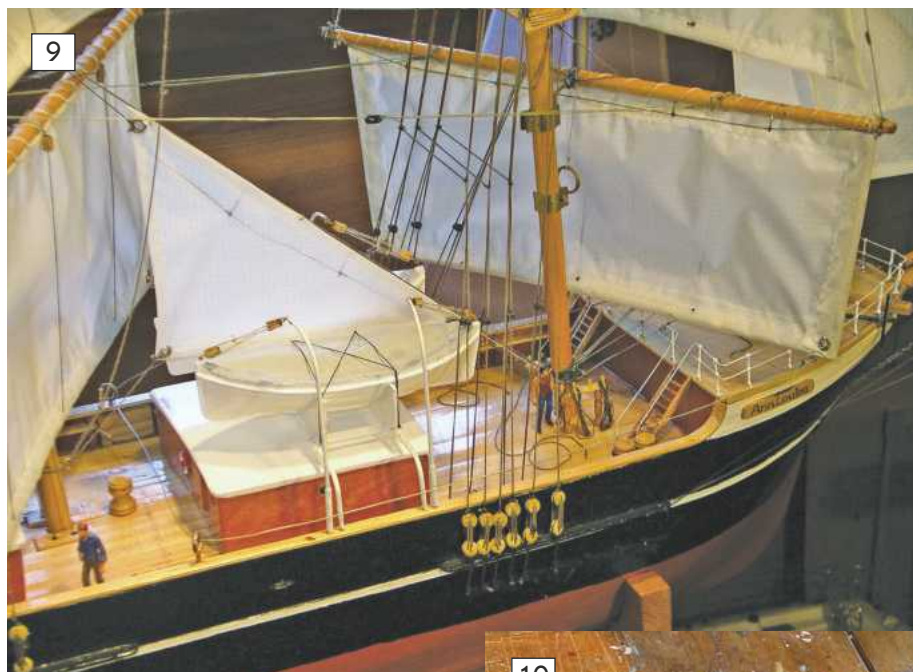
ABOVE: To the right, the foresail of a 1/40th scale full rigger. The extra hem, and 'solid' appearance of the sail give the wire away and the endless sheet can be seen running from the foresail, around the deckhouse.
