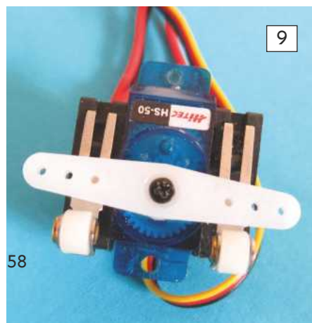
BELOW: The micro servo and micro switches set up allowing the supply voltage to operate the thruster unit.
