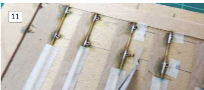
10: Using a curved craft blade the base plate is cut and removed from its jig. 11: Taping the eyes into place on the stanchion and soldered. 12: A length of 1 mm OD brass tube is inserted into the base plate and stored ready to be added to the stanchion.
