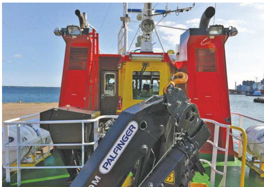
ABOVE: Deck crane on foredeck. RIGHT: The aft side of the wheelhouse showing extension and wheelhouse access door on the port side. This also shows engine exhausts and floodlights etc.
