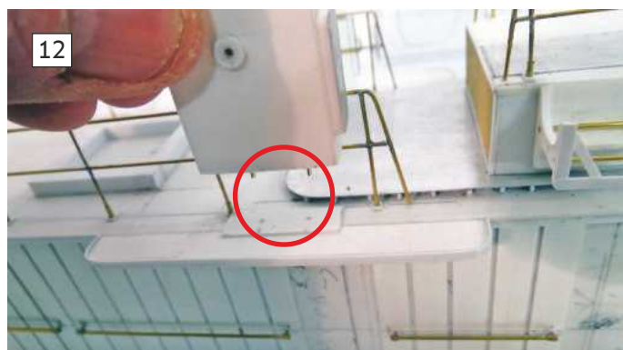
12: On the underside of the mounting two locating pins are added to ensure a firm and precise fit. 13: Port PK16 decoy launcher in place. 14: The starboard PK16 launcher.
