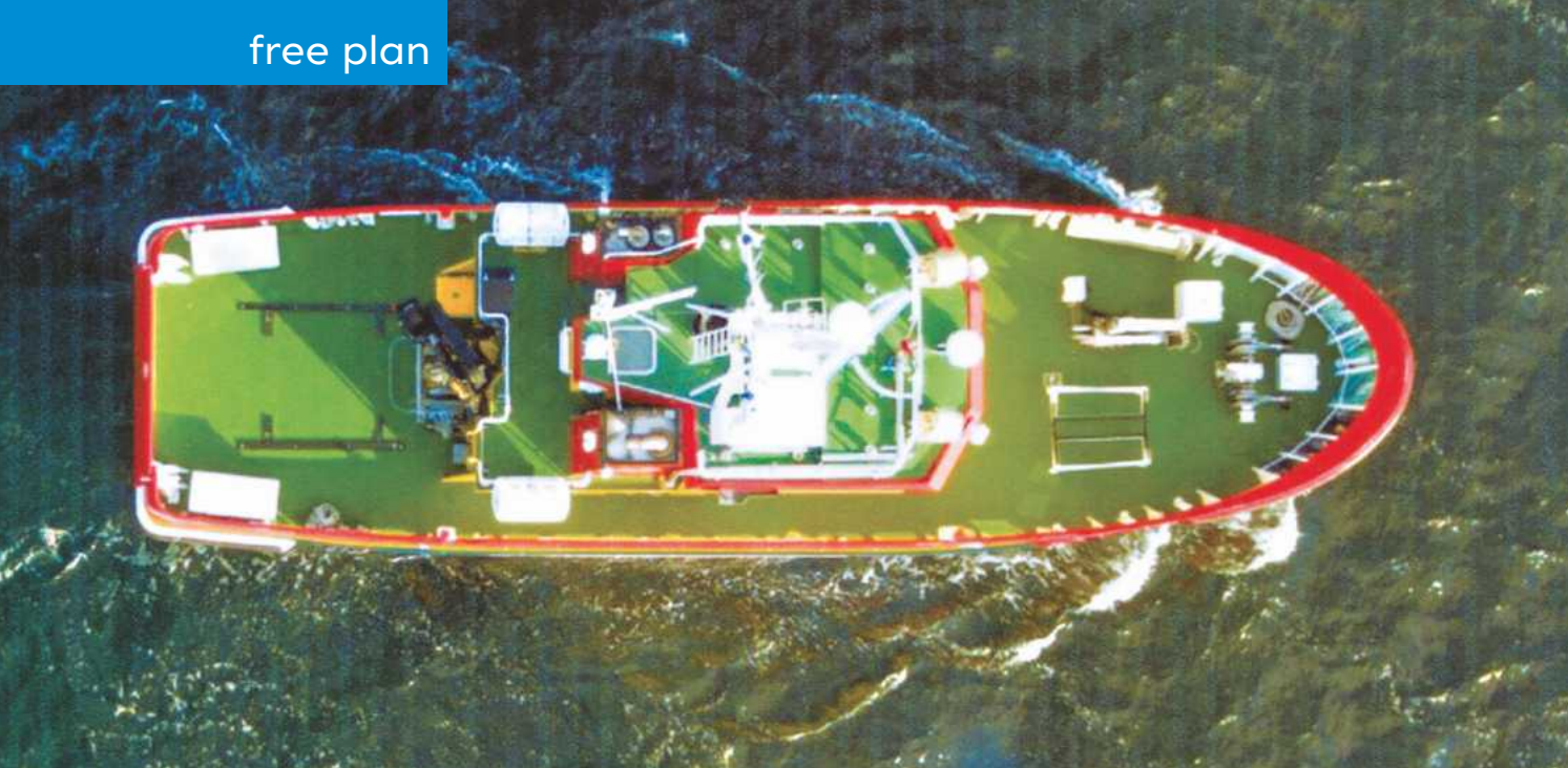
ABOVE: Aerial view, the dark coloured bars on the after deck are to provide seating for a container. BELOW: This gives a good view of the 'wineglass' hull shape and rubber protective section on upper bow. The position of the bilge keels can just be seen under the bilge.
