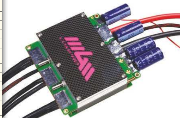
ABOVE: A very high quality and expensive ESC from MGM, made in the Czech Republic. Adjustable for about every parameter you would need to adjust.
