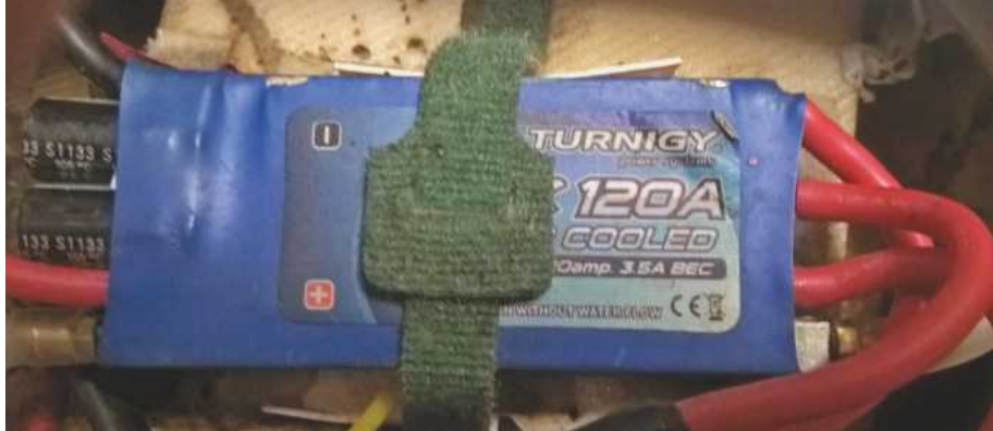
LEFT: The Turnigy Aquastar in my 4Cell Cat. Not fully waterproof, but pretty water resistant. Three Years of hard racing and still going strong. Fully programmable using a Turnigy USB Linker.
