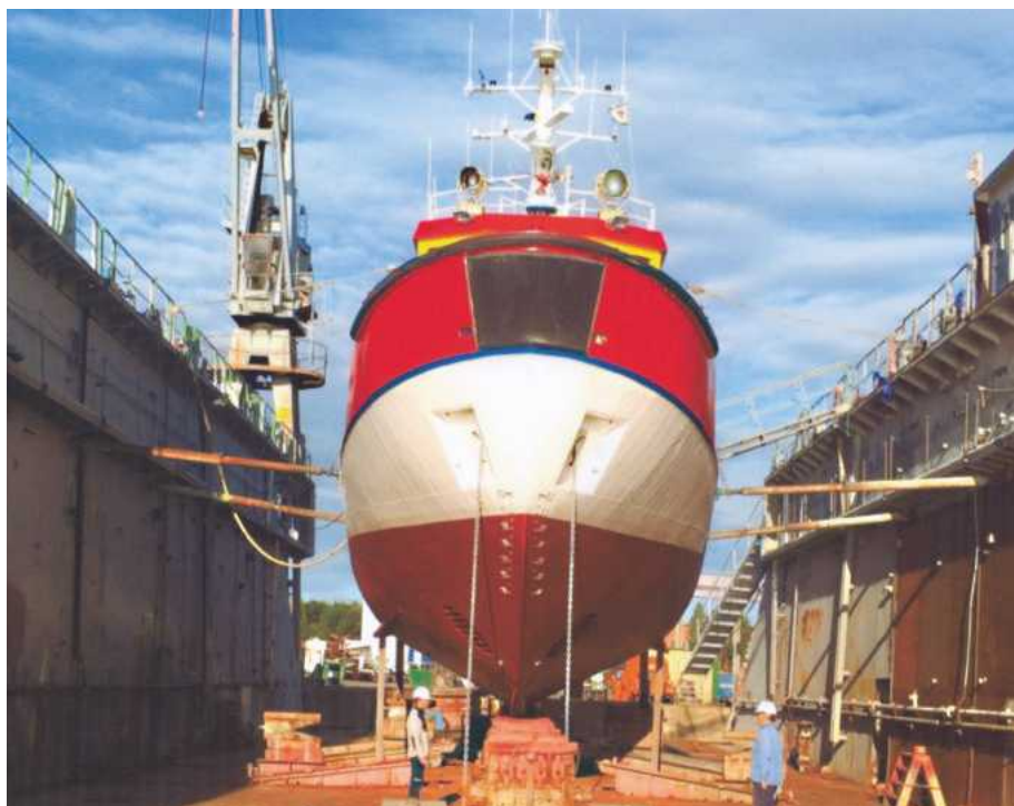
ABOVE: Aerial view, the dark coloured bars on the after deck are to provide seating for a container. BELOW: This gives a good view of the 'wineglass' hull shape and rubber protective section on upper bow. The position of the bilge keels can just be seen under the bilge.
