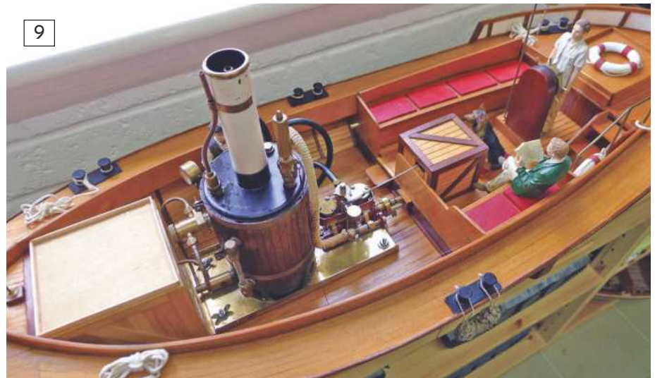
9: Just insulating the gas tank could very well be counterproductive, so care must be taken in how this is done. Here the heat travelling through the brass base is kept within the tank enclosure as the wooden box is open at the base.
