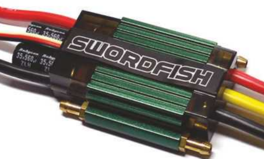
BELOW: A newer Swordfish model which is fully waterproof and again programmable with the USB Linker.
