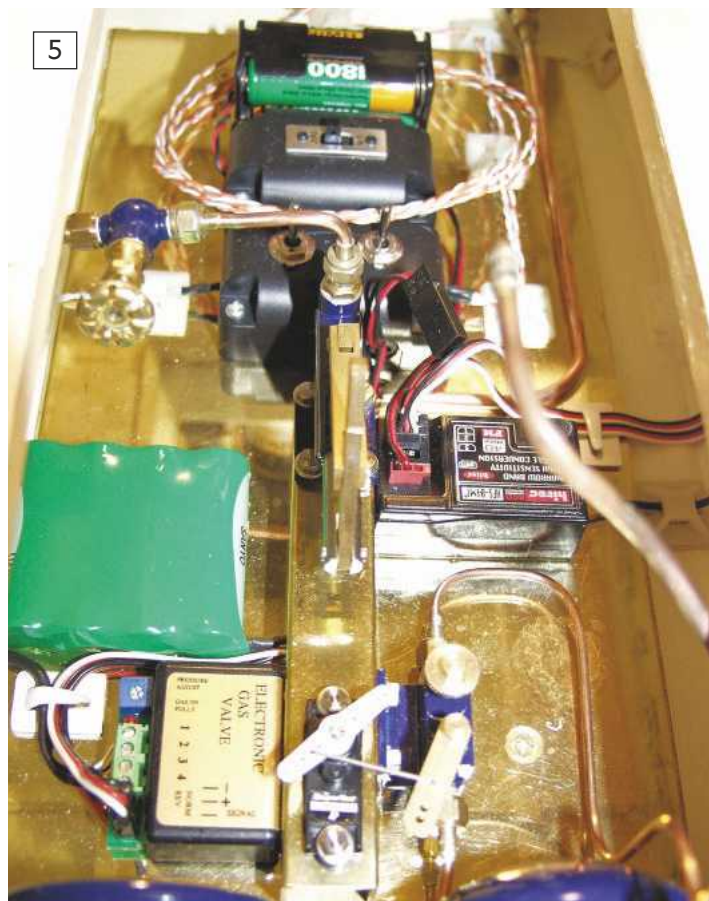
5: The electronic gas valve fitted into a hull. The green battery pack is dedicated to the valve and along with the control unit, the valve and the servo you can see you need a bit more room. 6: One option for the attenuator valve is to connect it directly to the boiler shell. This Cheddar boiler had a spare bush in just the right place so was perfect to mount the valve on and made for a very neat and compact installation.
