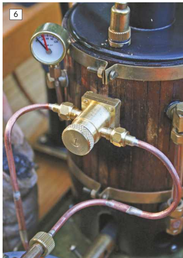
5: The electronic gas valve fitted into a hull. The green battery pack is dedicated to the valve and along with the control unit, the valve and the servo you can see you need a bit more room. 6: One option for the attenuator valve is to connect it directly to the boiler shell. This Cheddar boiler had a spare bush in just the right place so was perfect to mount the valve on and made for a very neat and compact installation.
