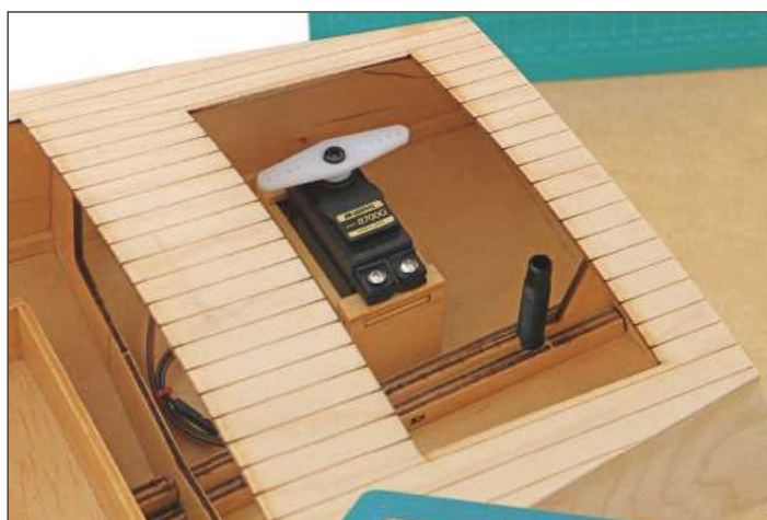
LEFT: The laser-cut servo mount works well although I had to add bearers to raise the height of the servo so that it cleared the bottom skin on the starboard side.
