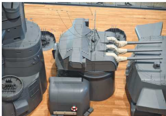
LEFT: Aft of 'A' turret is the triple 6in known as the 'Nendo Shik' which denotes its type and was also installed on cruisers of the Mogami-class. Unusually, a tripod aerial mast is mounted on the turret roof.
