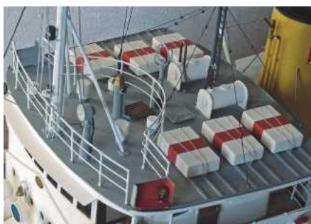
ABOVE: Bridge roof with six liferafts, two water tanks and other equipment.
