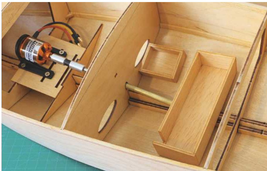
ABOVE: ESC and battery box in position. Wires from the ESC to the motor will feed through the elliptical hole.
