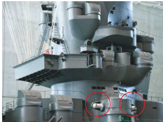
RIGHT: At the base of the main control tower on either beam and ringed in red is a 4.5m rangefinder directing the 12.7cm/40 calibre high angle (HA) AA guns.
