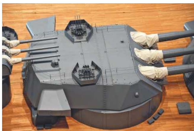
LEFT: The top of 'A' turret supporting two-gun tubs each having the Type 96 triple 25mm.
