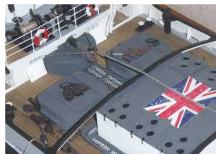
ABOVE: Tow hook area, note salvage hatches and salvage equipment, plus the prominent Union Jack.
