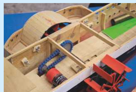
ABOVE: If you have ever wondered what the inside of a model paddle steamer looks like then this work in progress on PS Waverley by Chris Read of the Selsey club reveals all. Note the feathering paddle mechanism.
