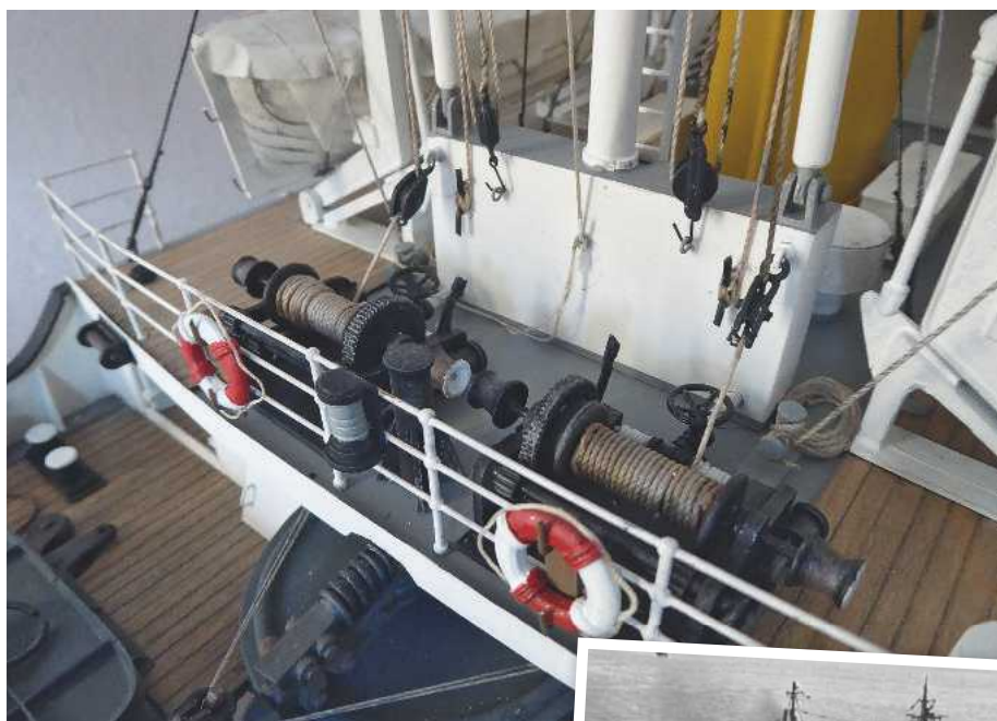
ABOVE: Winches for salvage booms on the rear deck house.
