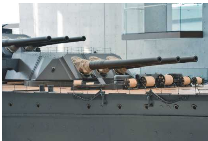
LEFT: The top of 'A' turret supporting two-gun tubs each having the Type 96 triple 25mm.
