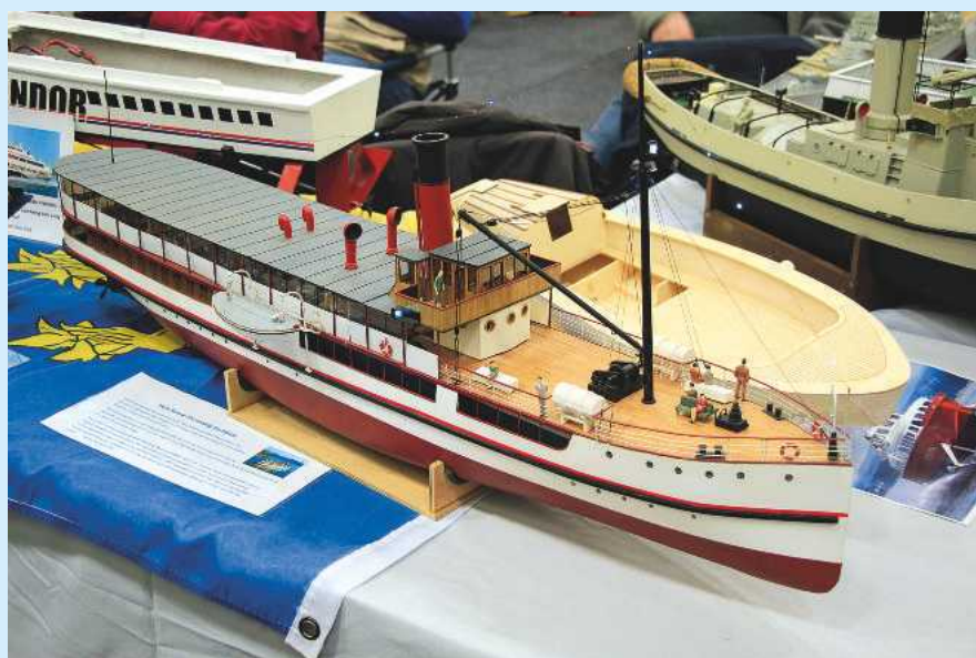
ABOVE: If you have ever wondered what the inside of a model paddle steamer looks like then this work in progress on PS Waverley by Chris Read of the Selsey club reveals all. Note the feathering paddle mechanism.
