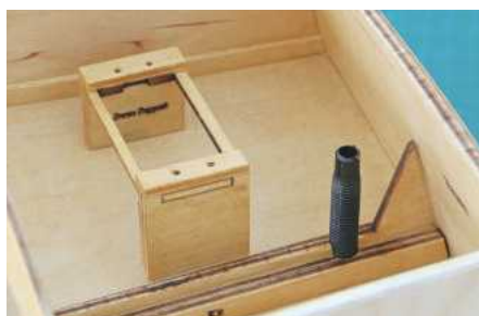
LEFT: The laser-cut servo mount works well although I had to add bearers to raise the height of the servo so that it cleared the bottom skin on the starboard side.
