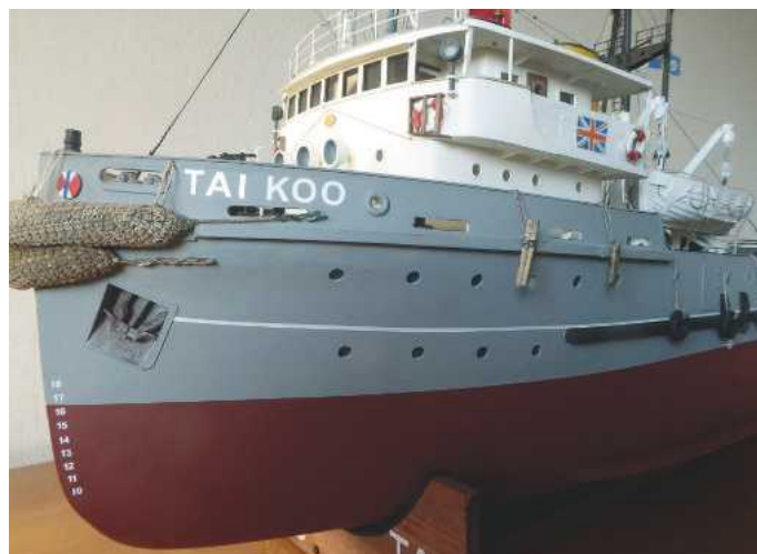
ABOVE: Bow area showing bridge and hull lines; note the timber fenders.
