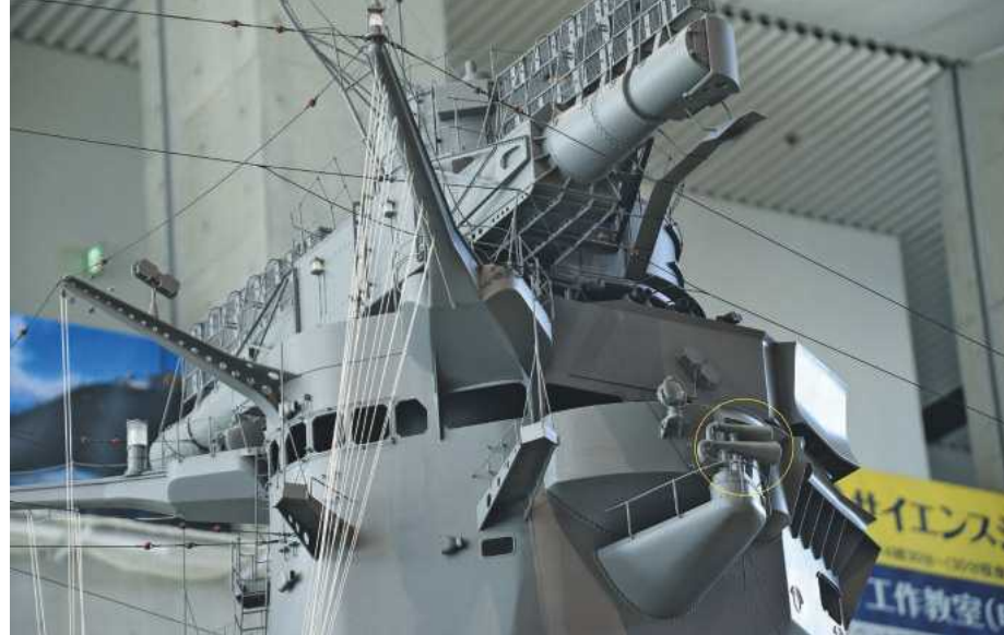
LEFT: Here we are looking down on the low angle director and on either side mounted on the rangefinders are the two-mattress antenna of the Type 21 radar array, known as Kai 3 an air and surface search radar, with a range of 120km (74miles).
