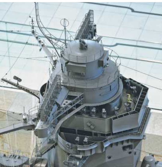
LEFT: Here we are looking down on the low angle director and on either side mounted on the rangefinders are the two-mattress antenna of the Type 21 radar array, known as Kai 3 an air and surface search radar, with a range of 120km (74miles).
