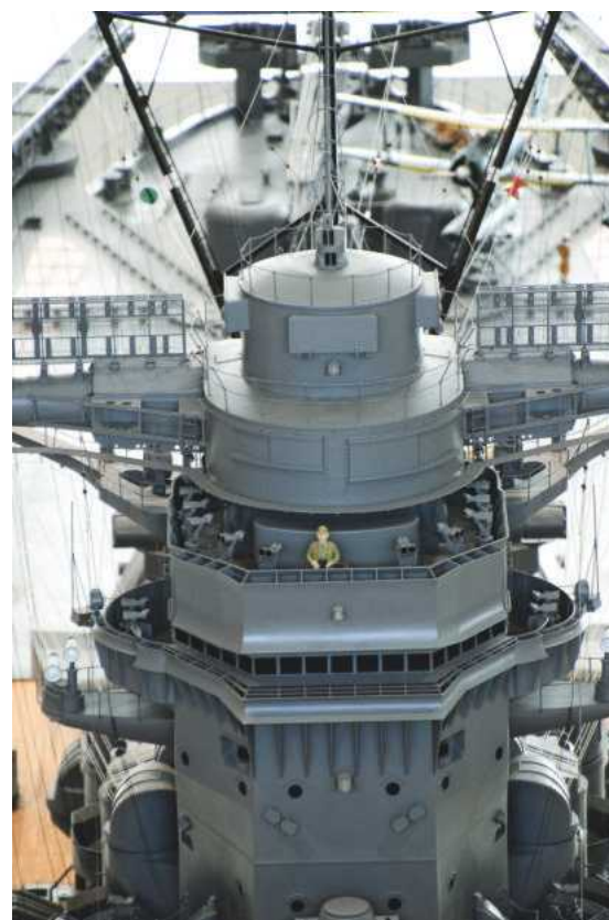
RIGHT: At the top of the armoured tower is the main low angle Type 89 Hoiban director and 15m rangefinder. Below that is the air combat post (the crew member and an array of pedestal mounted binoculars).
