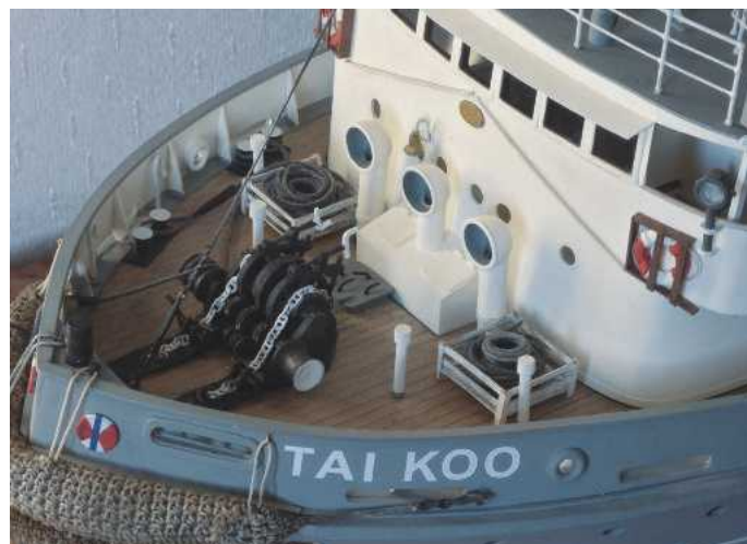
ABOVE: Bow area showing anchor winch, rope boxes and bridge window Visor; note Swire badges.
