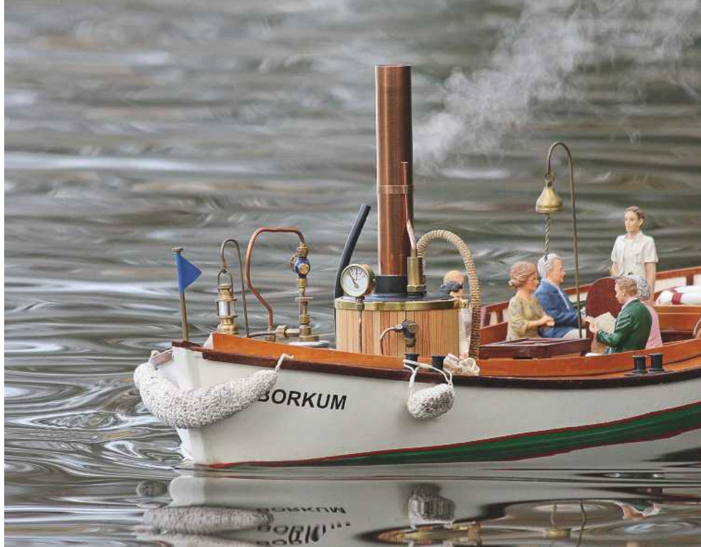
3. The Pendle 3 1/2 inch vertical boiler complete with lagging and fittings comes in at just over 1.8kg.
