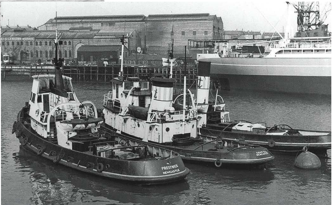
BELOW: Prestwick and two other tugs. This shows her original appearance with the small boat under its davits. Note that an extension to the engine exhaust has been added. (Photo: Steven Swinhoe)
