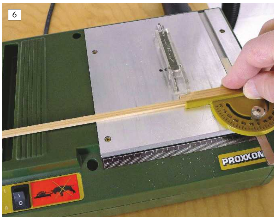
6. Some may consider a powered table saw to be a little on the extravagant side but you only need to do a couple of jobs like this to appreciate its worth. The ends of all the staves are perfectly clean cut, which is important because they're all quite visible on the top surface.
