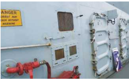
ABOVE: Moving down the port side aft and along the side of the VLS housing the so-called panel WT doors come into view. They're a familiar fitting on the T23s and preceding classes of RN warships.
