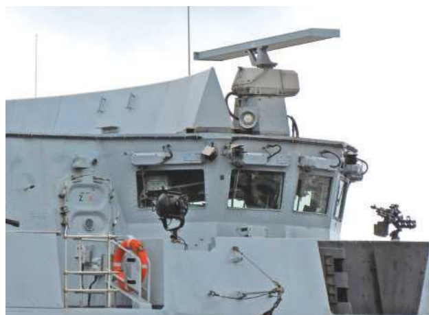
ABOVE RIGHT: The starboard bridge wing from a different perspective. The radar mounted on the bridge roof is a Type 2008 navigation radar.
