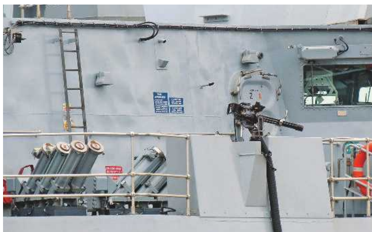
ABOVE: Just abaft of the bridge wing is one of four mini guns capable of a low angle depression to defend against small boats. Also to the left of the picture are the SRBOC Mk.36 Super Rapid Blooming Chaff launchers discharging 130mm cartridges which can be launched up to 244m.
