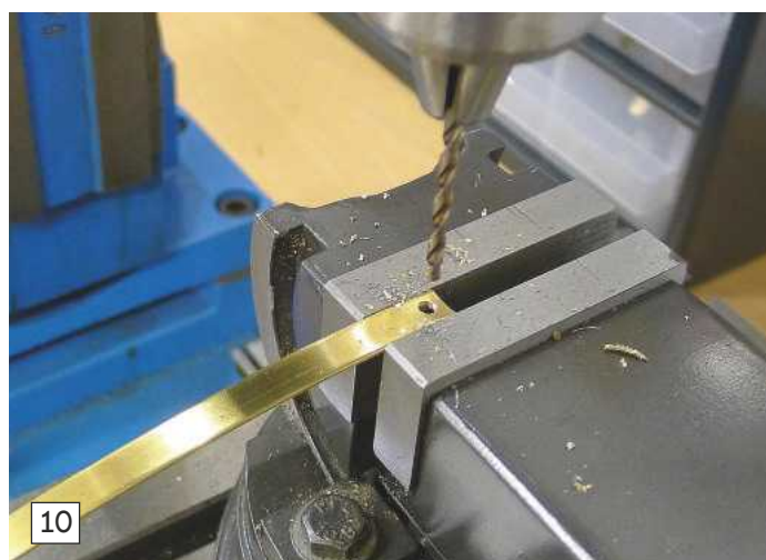
10. A sharp drill with gentle pressure should go through without any difficulty and will ensure the hole is correctly located in the tab.
