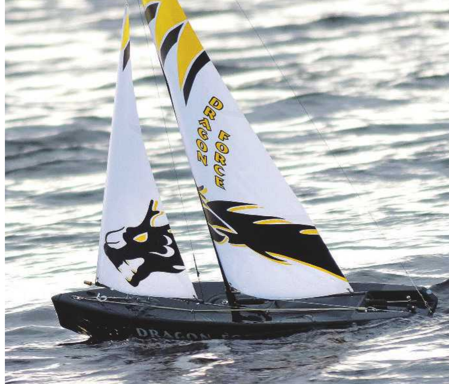
ABOVE: November 2012. Test sailing the second, lighter sample. We were happy with the performance but the hull was too fragile.
