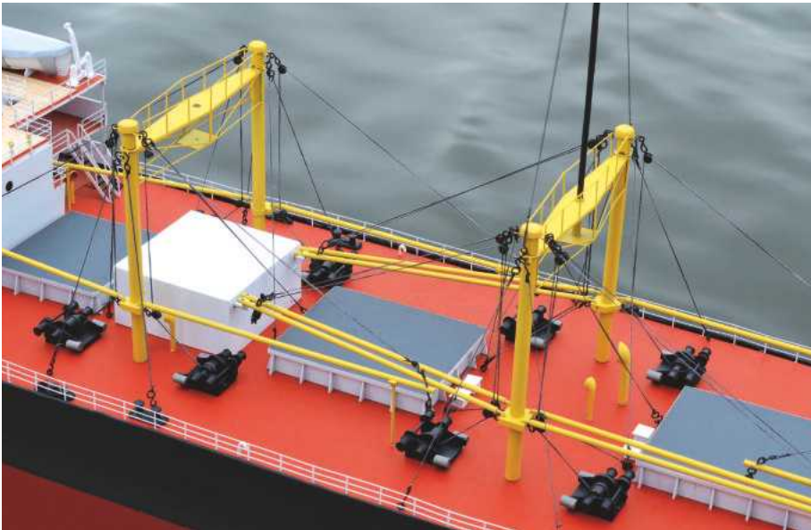
ABOVE: The hatch, derricks and winches for hold No.5.
