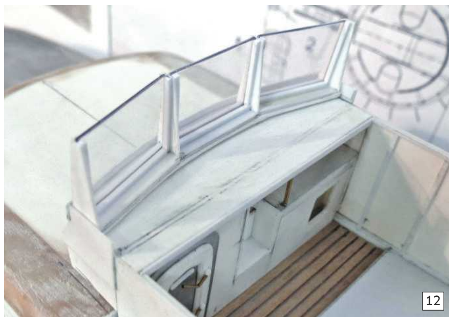
12. Each acetate sheet is slotted into each frame, no adhesive required.
