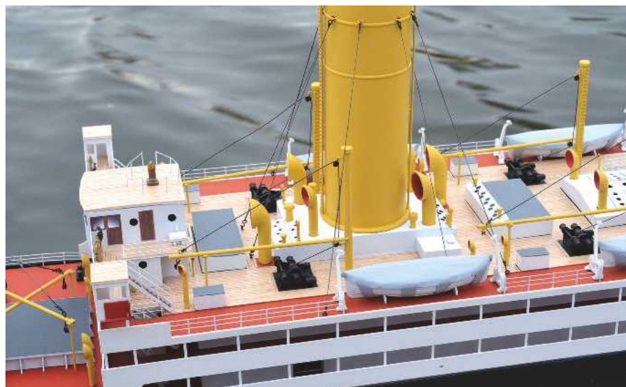
BELOW: Port side bridge and captain's accommodation. Of other interest: the four grey-topped boxes on the boat deck were coaling hatches. If I were a fan of weathering I'd have to ingrain the wood with black coal dust.
