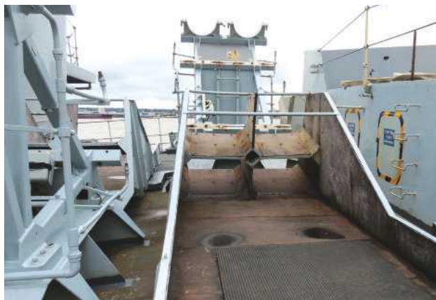
ABOVE: In the space between the bridge and the VLS housing we can see, in more detail, how the framework for supporting the Harpoon missile canisters is arranged.
