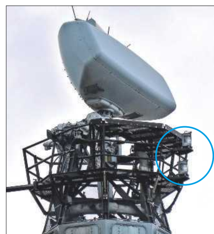
ABOVE: A detailed close-in picture of the new Artisan Type 997 radar surrounded by the existing inspection platform. Note the two forward-facing navigation lights (ringed in blue).
