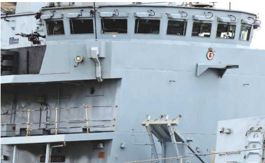
ABOVE: A pair of roller fairleads. It's worth noting for model making purposes how the two closer stanchions are fixed into the support frame of the fairlead. Also the type of stanchion used.
