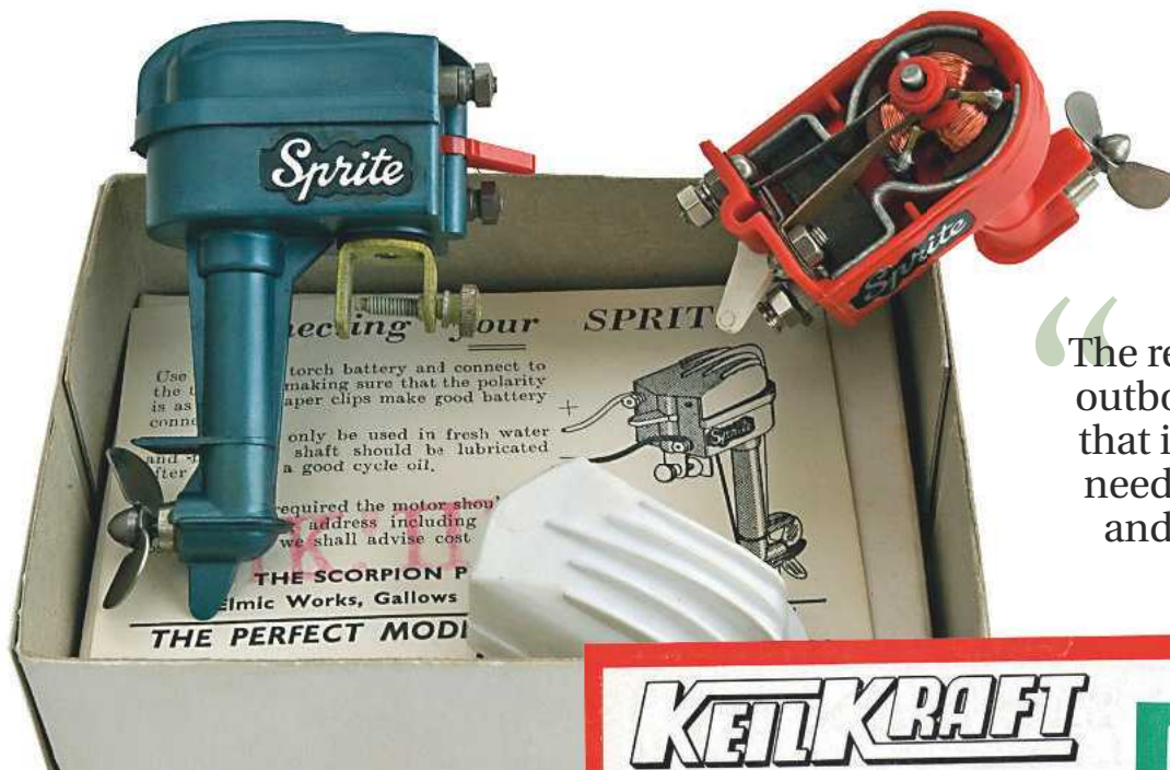
ABOVE: A Sprite with its cover removed to show the integral motor.
