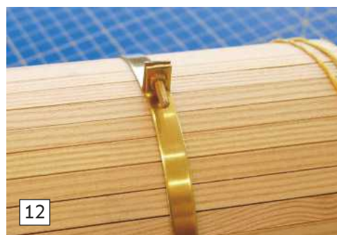
12. The right tools and a bit of planning should ensure that you end up with a neat tab and a perfect size hole in just the right spot. Great care should then be taken with the marking out of the second tab to ensure the correct compression of the lagging.
