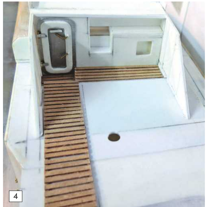
3. A section of slatted walkway formed on the jig.
