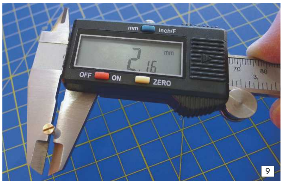
9. Vernier calipers are an invaluable tool to have around. Tasks such as this become quick and easy with the correct selection of the drill ensuring a successful piece is created.
