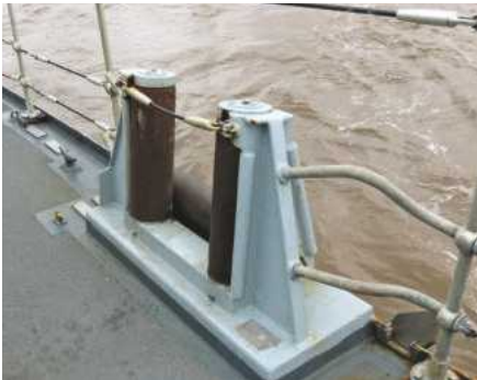
ABOVE: A pair of roller fairleads. It's worth noting for model making purposes how the two closer stanchions are fixed into the support frame of the fairlead. Also the type of stanchion used.
