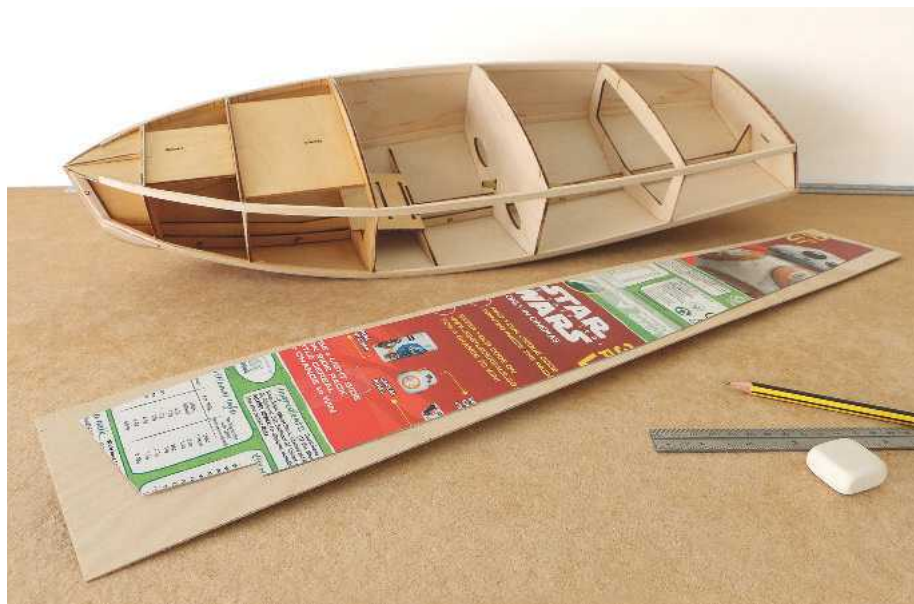
ABOVE: The real work here is in creating a template that fits like a glove. Double-sided tape holds it firm while cutting.
