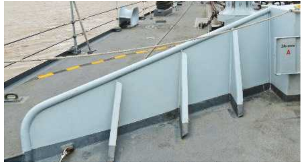
RIGHT: This picture on the port side shows clearly that the outer breakwater support is not vertical, a minor observation for perspective model makers but this is how it is.
