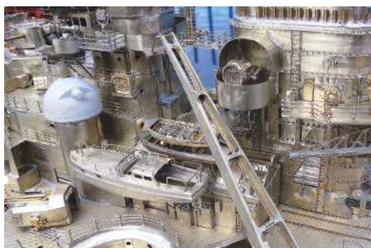
Much of the work on the photo etched brass involves soldering the parts together. Definitely not an exercise for the faint hearted. On the bottom left is a triaxial mounted 10.5 dual-purpose gun.
