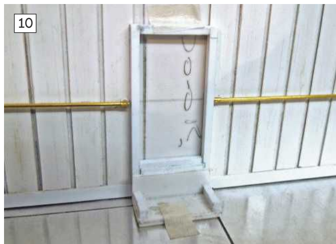
11. First the door is offered into the jig, adhesive-free, to ensure that the jig is doing its job.
