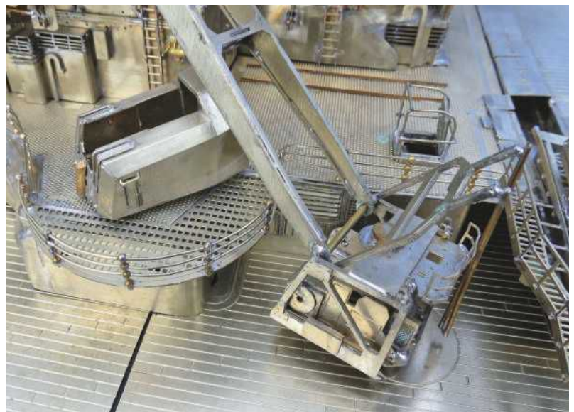
LEFT: There's a huge volume of detail and it's all photo-etched except the semi-spherical SL6 anti air fire director in the fore ground. Within the sphere on the original ship was a 4m base stereoscopic night fighting rangefinder.
