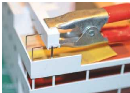
ABOVE: One of the 'fiddly' tasks. Holding a stanchion, which will support the bridge wing, in a temporary styrene fixture while it's glued to the side wall. Two front wall stanchions are already in place.
