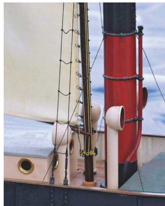
ABOVE: Note, positioned on the forward face of the funnel, the 4.5mm copper pipe that vents the boiler safety valve.
