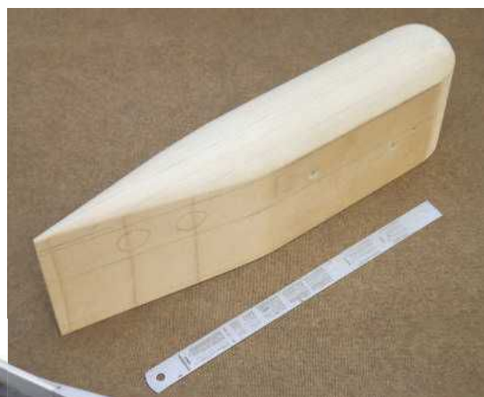
LEFT: The MDF tool, sculpted and ready for the fitting of external details such as ribbing and raised window shapes.
