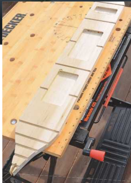
ABOVE: The planed poplar base plank of the hull after cutting grooves and recesses.
