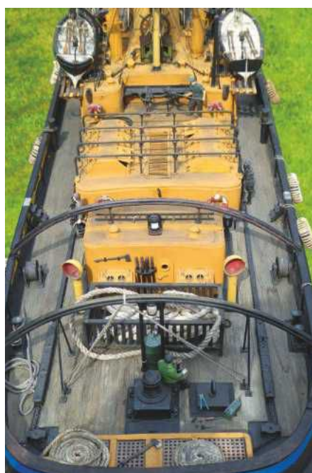
Stern area with added tow bow supports, salvage pump heads and revised colour scheme.
