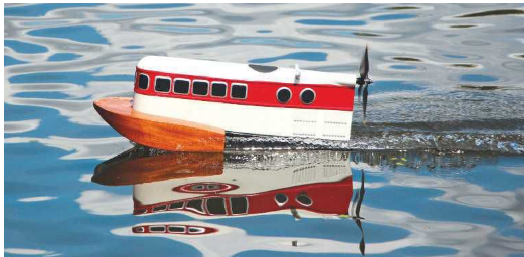
TOP RIGHT: During testing, ever larger props were fitted, going up in stages to arrive at the best looking and performing combination of two 7 x 4" APCs, as seen here.
