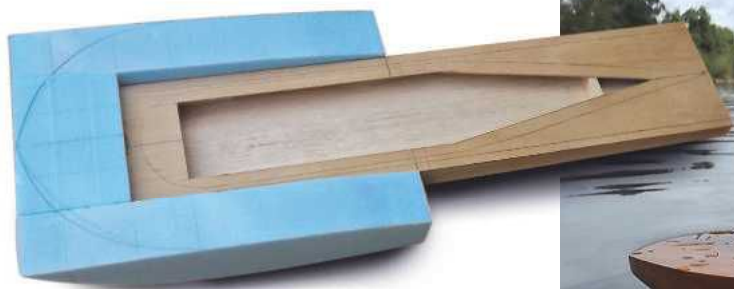
For the bow, which is a complicated shape, I used several blocks of blue styrofoam glued together to fit the front of the hull, then cut and sanded to shape.
