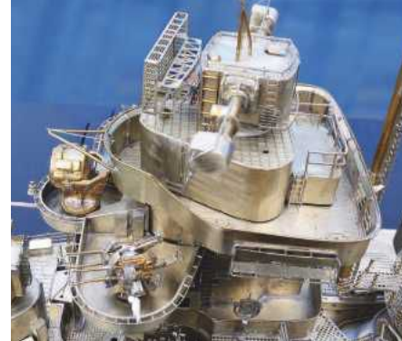
A view of this impressive model looking at the top of the forward control tower. At the head is a 10m stereoscopic rangefinder with the FuMO 23 radar array.
