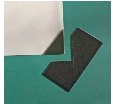
BELOW: Gorilla tape is perfect for the reinforcement patches, being both strong and flexible.
