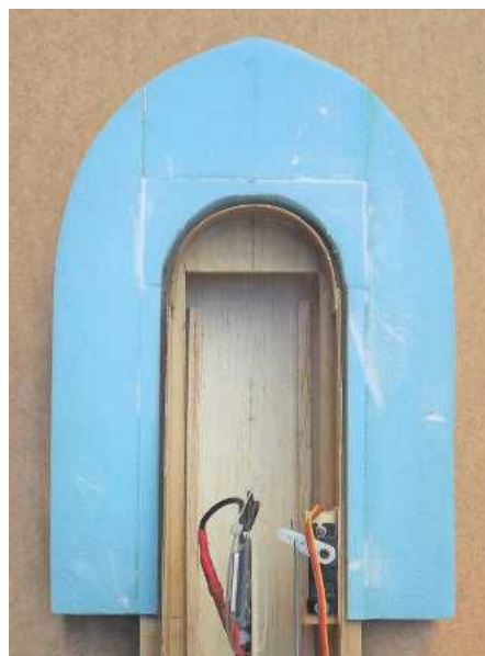
For the bow, which is a complicated shape, I used several blocks of blue styrofoam glued together to fit the front of the hull, then cut and sanded to shape.
