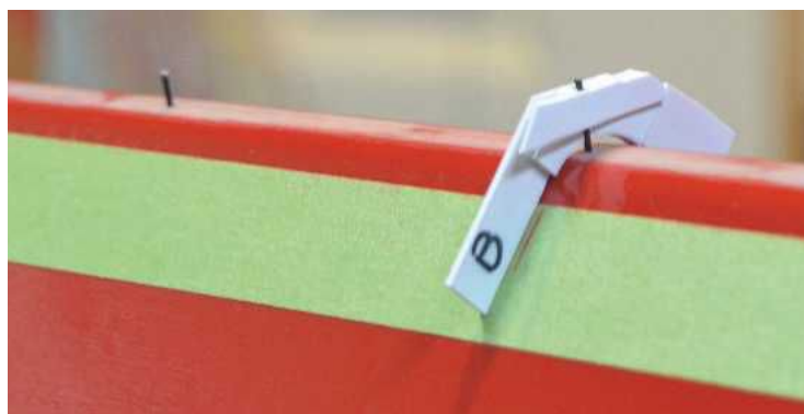
ABOVE: Fitting pins to support the bilge keels.
