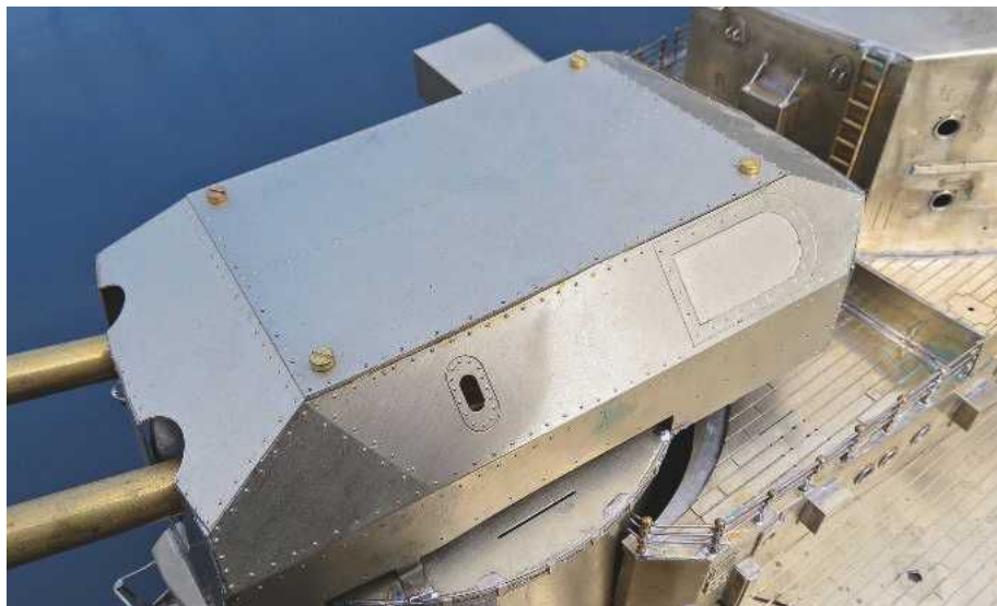
The forward gun on this model of Bismarck was all from PE brass. On the original ship it was designated SK C/34 38cm (15 inch) and the ship had four of these turrets.
