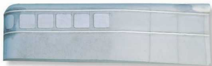
LEFT: The MDF tool, sculpted and ready for the fitting of external details such as ribbing and raised window shapes.
