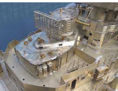
This part of the superstructure houses the forward armoured conning position with its various director periscope hoods and navigational periscopes, plus the 7m stereoscopic rangefinder with its FuMO 23 radar array.
