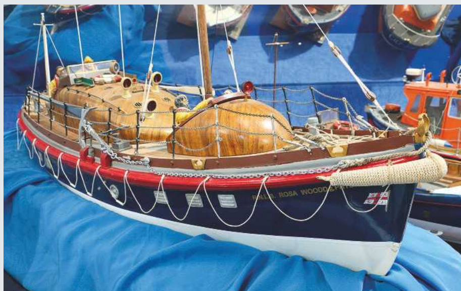
ABOVE: Soon to be re-released by SLEC as part of the Vintage Model Boat Company range, the Sportsman is 32" long, has an 8" beam and takes a 1000kV outrunner and 3S LiPo. Available spring 2018.
