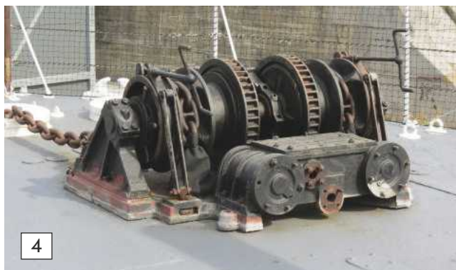
4. The steam powered windless. I cannot be certain as to the origins of this piece of equipment and would query whether it's original to M.33.
