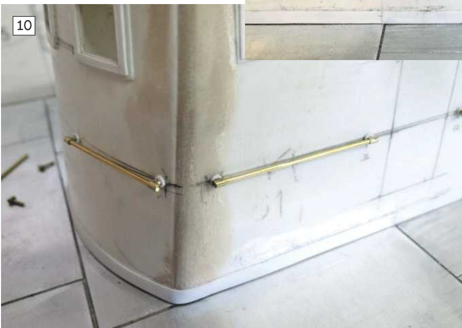
10. The handrail continues on the front of the wheelhouse.
