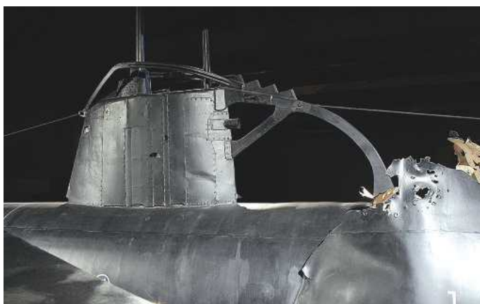
Assembled from the relatively undamaged bow of M-22 and the stern of M-27 this composite hull is now on display at the Australian War Memorial and is well worth a visit.
