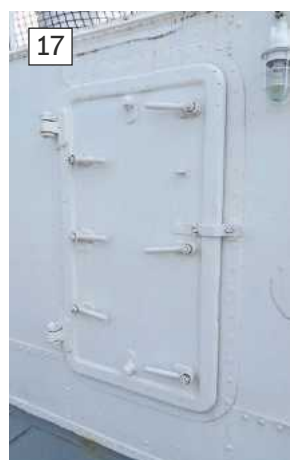
17. The watertight door giving access into the deck housing on its port side. Note that the door opens forward, something that is usually standard on ships of all types.
