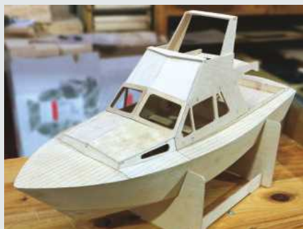
ABOVE: Soon to be re-released by SLEC as part of the Vintage Model Boat Company range, the Sportsman is 32" long, has an 8" beam and takes a 1000kV outrunner and 3S LiPo. Available spring 2018.
