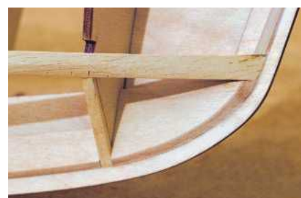
Due to an undersize B1 the stringer notch ends up slightly high, resulting in the stringer missing it slightly.
