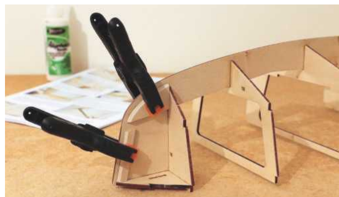
Adding the keel doublers that will eventually support the hull skins. Note the chamfer.
