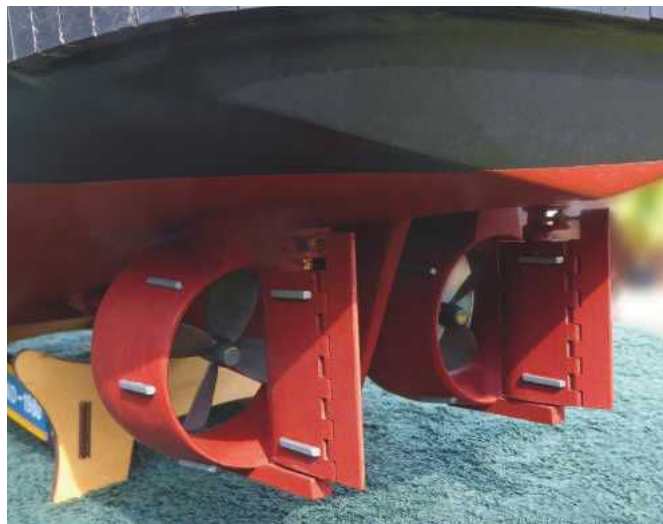
ABOVE: The business end! A stern view showing the revised drivetrain with correct size and shape of Kort nozzles plus the Billings brass Becker rudders. Why buy new, when you can recycle?
