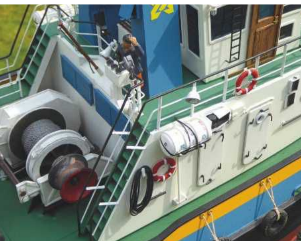
LEFT: The starboard superstructure with its new life rafts, a scratch built towing winch, wooden wheelhouse doors and improved detail steel doors.
