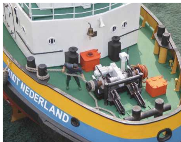
RIGHT: The foredeck now has the Billings (brass) anchor winch and capstan rollers. The remaining fittings were all scratch-built.
