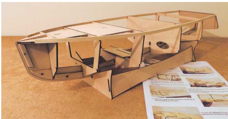
Top stringers in place and ready to receive the bottom chine stringers. Note the stiffening spacers between B1, B2 and B3.
