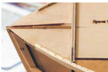
A small chamfer on the end of the stringer locates it nicely in the brest hook notch.
