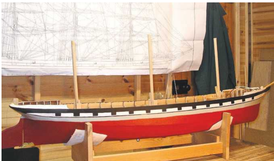
BELOW: Starting to look like the real thing with Underhill's drawing behind. Note the oversize rudder which is at least ten times the scale size of the original!
