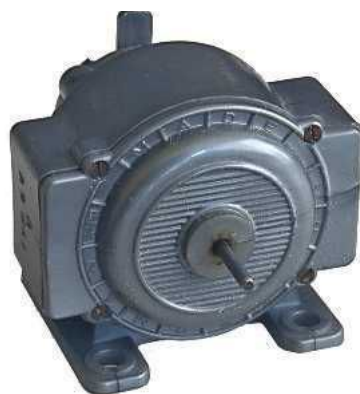
Examples of post-war motors using twin rectangular field magnets. Top: Japanese Kako. Left: Frog Revmaster. Above: Marx Duoperm.
