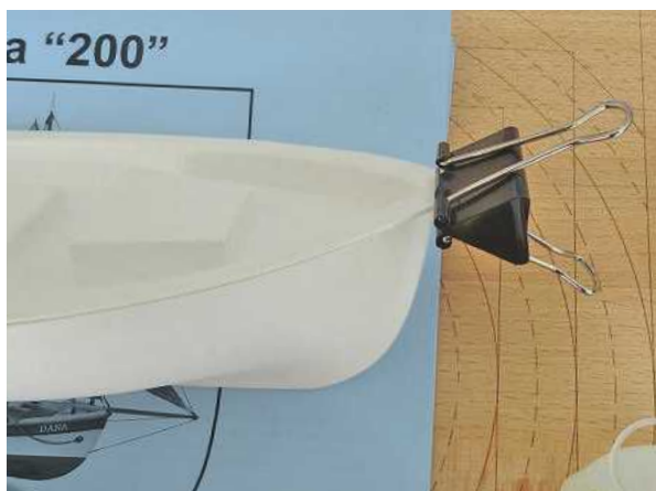
If building a static model, gluing the sub-deck takes a matter of minutes, however do consider the possibility that you might want to add lead for stability.
