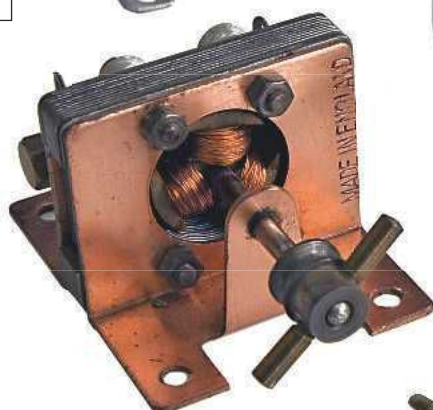
Examples of post-war motors using twin rectangular field magnets. Top: Japanese Kako. Left: Frog Revmaster. Above: Marx Duoperm.
