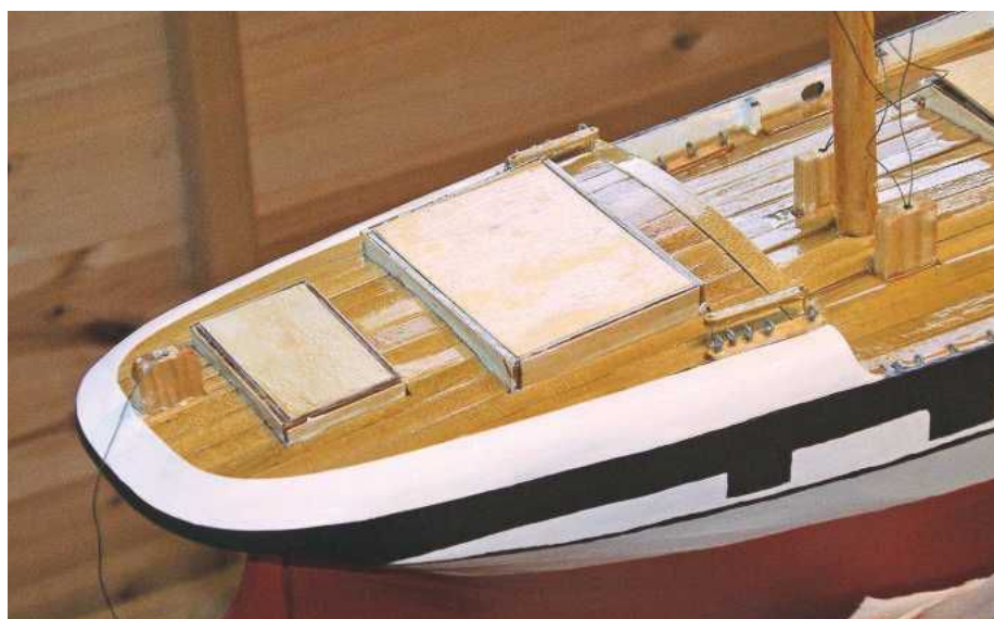
ABOVE: The turtleback stern area after decking. Note the fairleads, sticking well up above the deck, at either side of the mizzen mast. The lines through them are the braces for the main mast yards.
