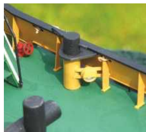
LEFT: The correct style bulwark supports with a deck light and fire hydrant.
