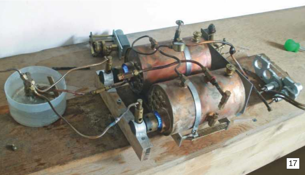
17. The steam plant, dismantled and part-reassembled for bench testing.
