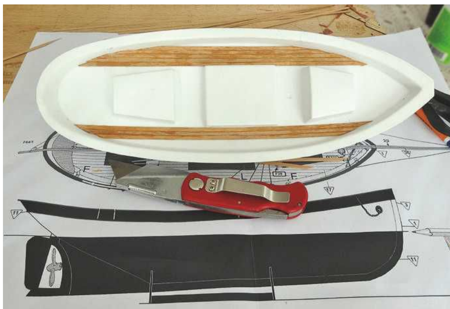
If building a static model, gluing the sub-deck takes a matter of minutes, however do consider the possibility that you might want to add lead for stability.
