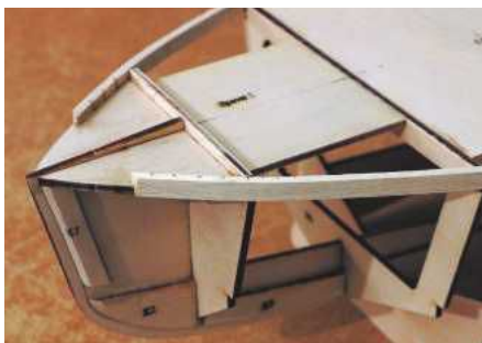
With the upper stringers in place the hull begins to stiffen up very nicely.
