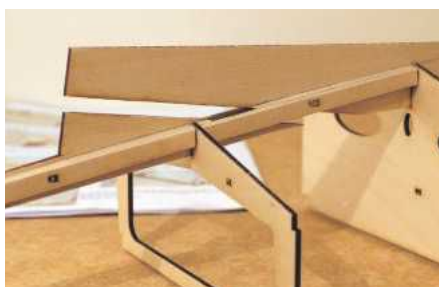
Where the prop shaft exits the hull, double thickness keel doublers are employed to strengthen the detail.
