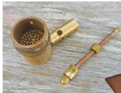
ABOVE: The gas is distributed through drillings in a brass disc in the burner so replacement of the ceramic is not going to be required.
