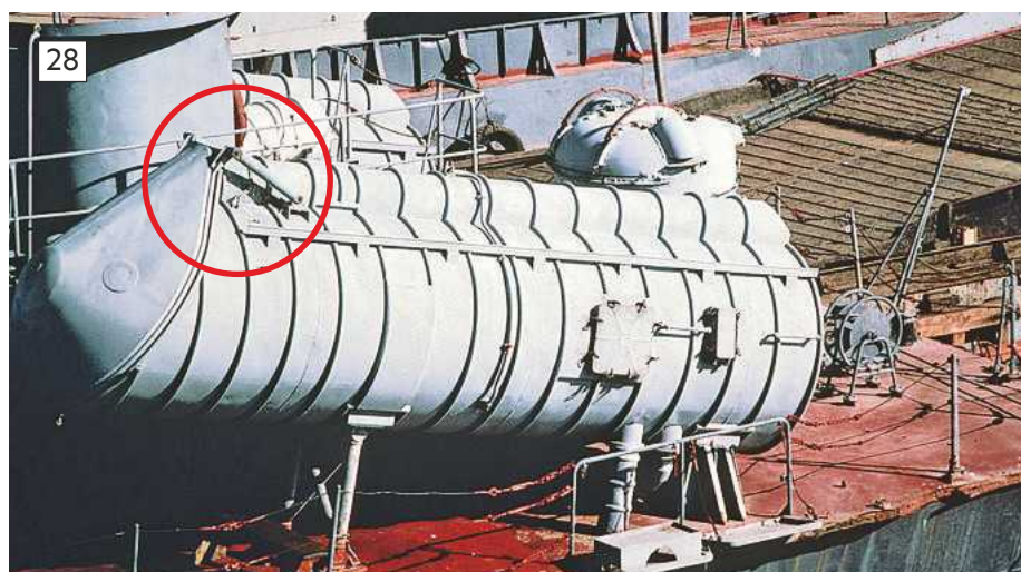
Photo 26. The parts that make the rear door of a launch tube (see text).
