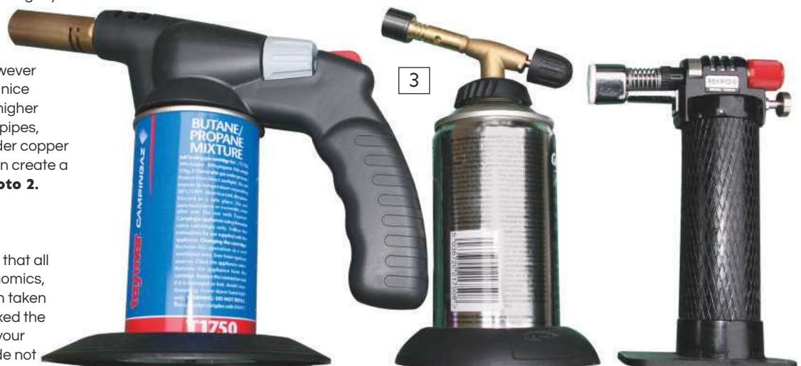
Photo 3. A typical range of burners, both gas and petrol, should cover your pipe bending requirements. These burners should also cover you for silver soldering pipe fittings, so they're a worthwhile investment.
