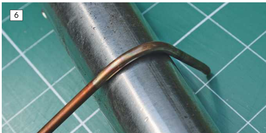
Photo 6. Any sort of former can be used to bend pipe but it will not prevent collapse of the tube being curved so you're limited to large diameter bends and the smaller diameter pipes.
