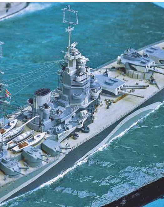
ABOVE: HMS Rodney (and HMS Nelson) had all their main 16 inch battery forward. This was because of the International Naval Treaty restrictions agreed between WWI and WWII.
