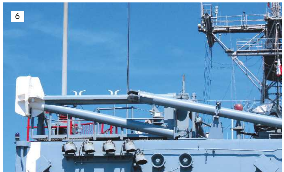
Photo 6. These tubular frames positioned on the top of the aircraft hangars are associated with the replenishment at sea equipment.
