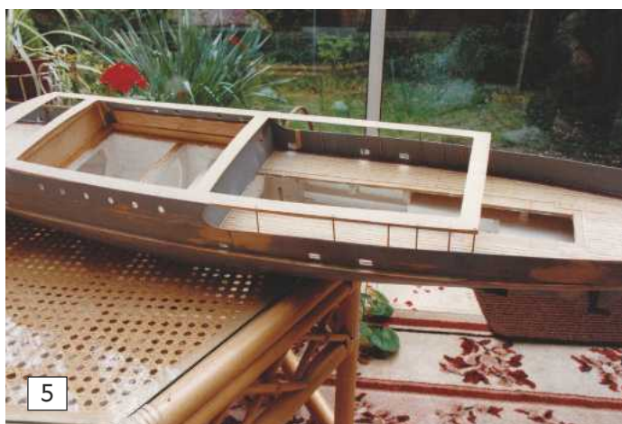
Photo 3. The lower hull is of composite construction.
