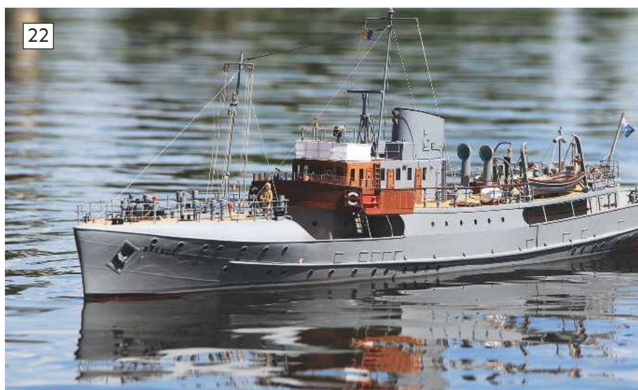
Photo 20. The foredeck completed. Note the railing joins just above the forward bollards and the sections of coaxial TV cable used for the fire hydrant handwheels.
