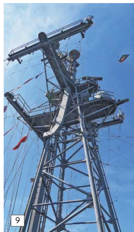
Photo 6. All of the Oliver Hazard Perry Class of guided missile frigates have this conspicuous tubular lattice mast on top of which is the SPS 49 air search radar.
