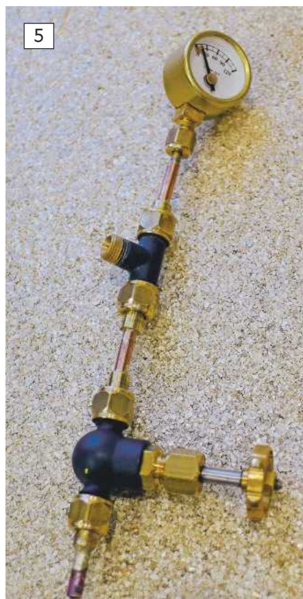
Photo 5. The finished manifold with pressure gauge and isolation valve ready to fit. A conical fitting was also added to the end of the outlet pipe on the boiler.
