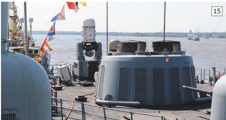
Photo 13. Mounted amidships is the fire control radar which works together with the Mk. 92 fire control system mounted forward on the bridge roof.
