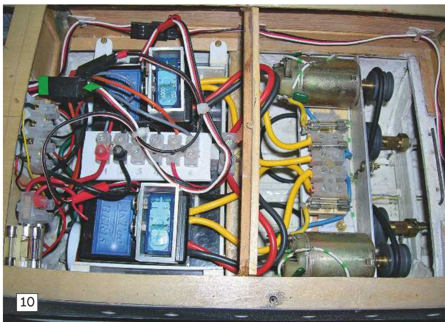
Photo 10. The motor, esc's and battery compartments. The receiver is mounted in the next compartment forward under the wheelhouse.
