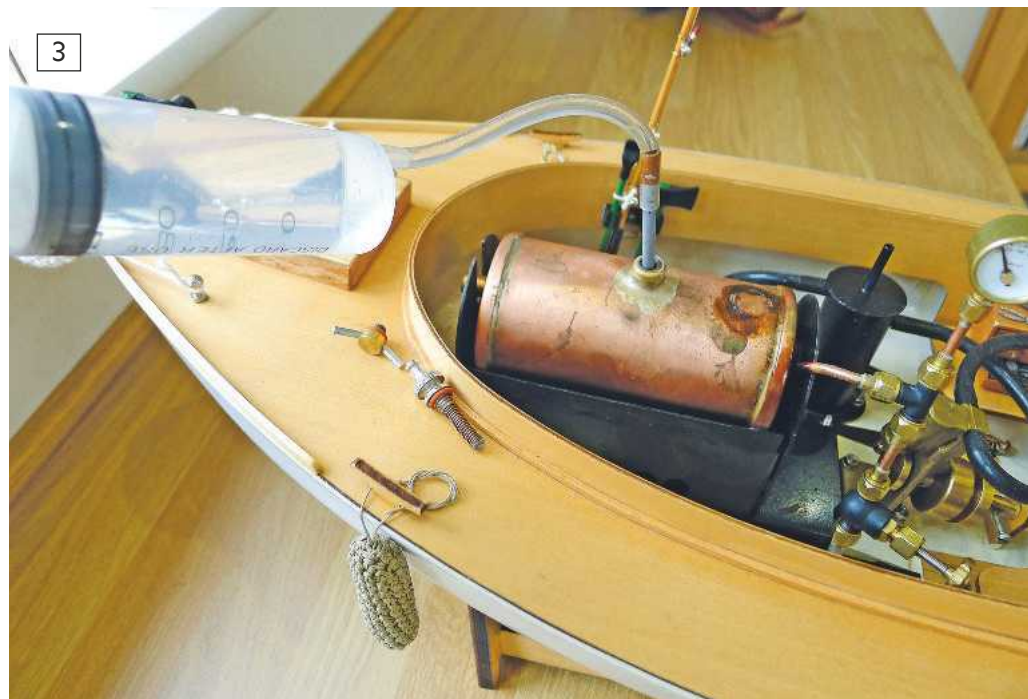
Photo 3. Without a sight glass, the boiler level can be guaranteed by filling through the safety valve mounting up to the level plug. The boiler holds far more water than the fuel tablets can use, so there is no worry of it running dry.
