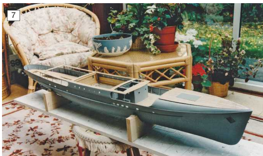
Photo 6. Hull in primer and bow deck sub-piece is in place ready for planking.
