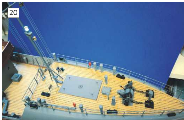
Photo 20. The foredeck completed. Note the railing joins just above the forward bollards and the sections of coaxial TV cable used for the fire hydrant handwheels.
