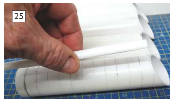
Photo 25. An 11.1mm o.d. tube is divided into two and will form the half-round section on the top of the tube.
