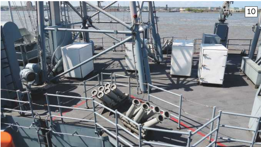
Photo 10. The arrangement at the base of the mainmast. In the foreground are the starboard sets of decoy launchers.
