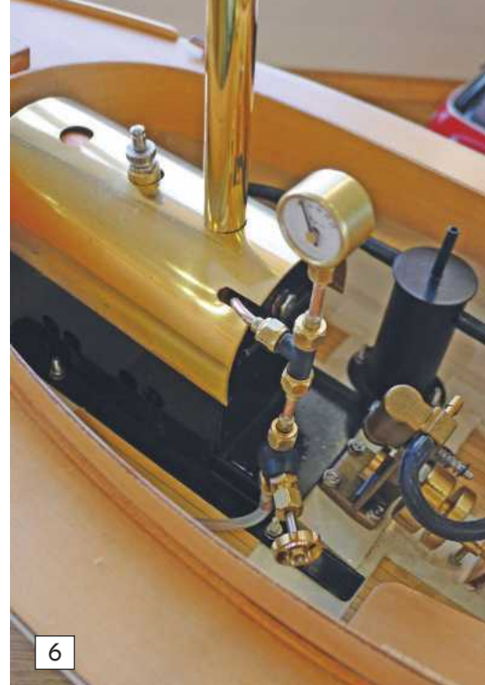
Photo 6. The new manifold in place on the boiler. The arrangement is neat and tidy and now allows pressure to build before opening the steam line to the engine, plus you have a good idea of what is going on inside the boiler.
