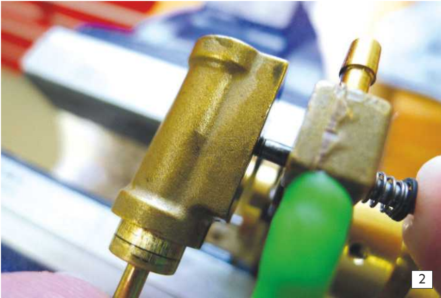
Photo 2. Tiny is easy to work with and the piston can be removed in a couple of seconds. Pushing on the end of the port face spring holder allows access to the faces for lubrication and the piston can be dropped out for a clean and an oiling.
