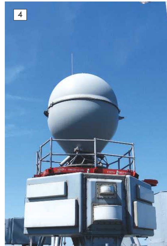
Photo 5. Mounted on a platform is the egg-like cover for the Mk. 92 fire control radar for the missiles and 75mm gun.
