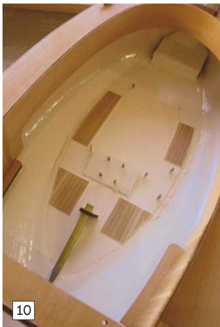
Photo 10. With the internal wood parts masked off, the internal surfaces were all given a couple of coats of a white acrylic radiator paint. This provides a heat resistant and easily cleanable surface.
