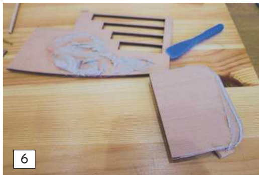
Photo 5. The supplied rudder was nothing more than three pieces of plywood glued together with the centre part offset aft around 3 mm to create a channel for the rudder stock at the front and a tapered trailing edge.
