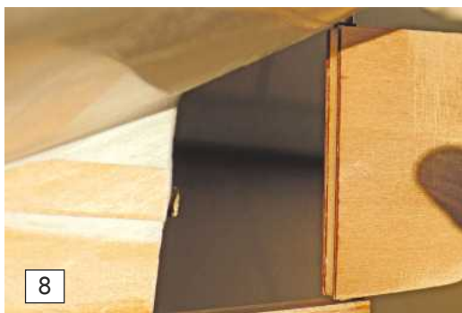
Photo 8. A fairly simple yet hopefully effective rudder was created, which has the added benefit of brass washers as rubbing faces to prolong its working life.
