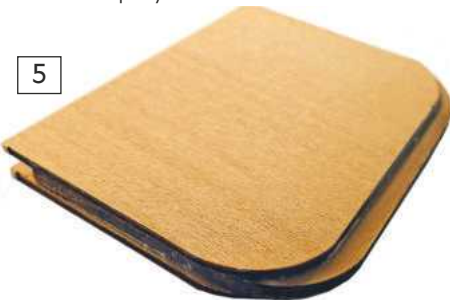
Photo 5. The supplied rudder was nothing more than three pieces of plywood glued together with the centre part offset aft around 3 mm to create a channel for the rudder stock at the front and a tapered trailing edge.
