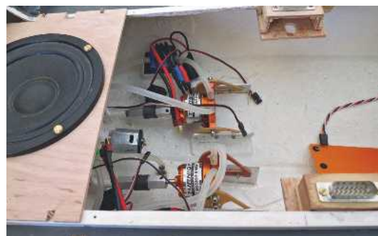
Right: The power plant for the 1:16 scale Christopher Pearce is two 910Kv brushless out-runners with 55mm five bladed propellers.
