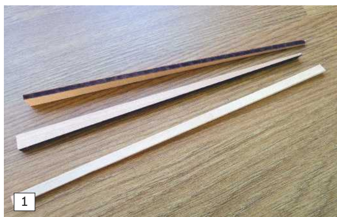
Photo 1. The heavy plywood parts supplied for the coamings at the bow were never going to bend to shape easily so were replaced by pieces of stock softwood. These conformed to the bend and sheer of the bow section much more easily.
