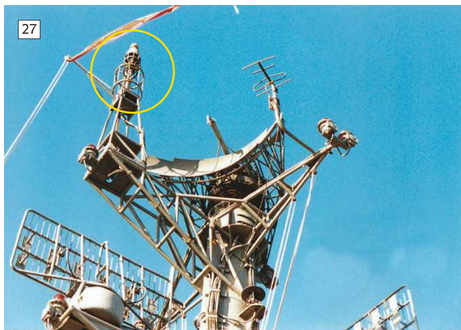
Photo 23. Now installed are the various electrical junction boxes. Strangely, there are no handles or clips on them.
