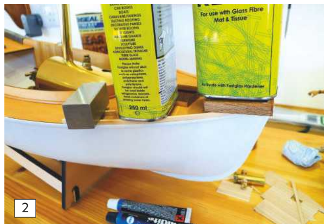
Photo 2. The softwood could actually be pre-bent to shape to suit the curve of the hull so all that was left once the glue was applied was to persuade it to sit on the sheer neatly.
