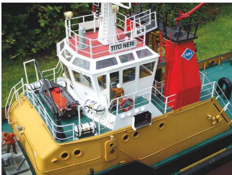
Left: Bridge area showing added detail such as the windscreen wipers, mushroom ventilators and improved RIB and liferafts.
