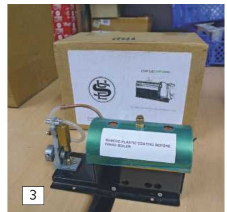
Photo 3. A pivoted boiler allows you to lift it up to place solid fuel tablets in the burner and easily ignite them. This is so much safer than trying to insert ready lit trays of methylated spirits into a model boat's interior.
