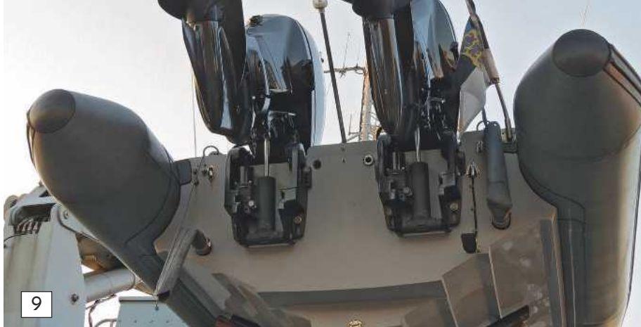
Photo 9. Each rigid inflatable boat is fitted with two outboard motors.
