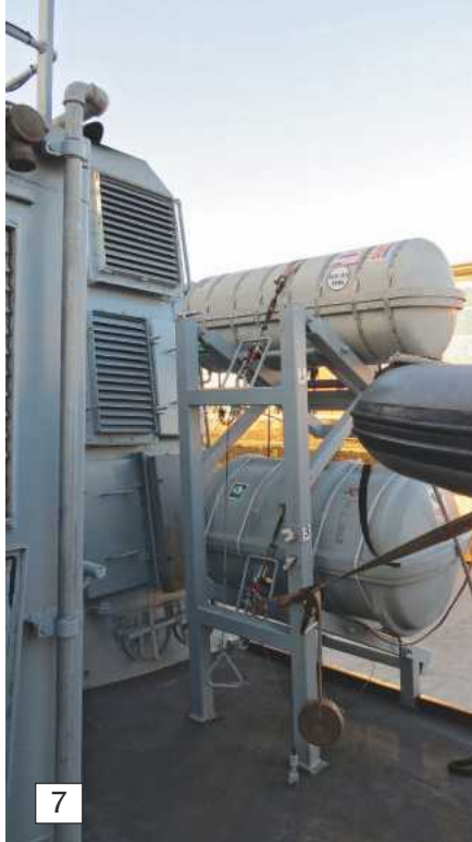
Photo 7. There are two different types of liferaft container stowed just forward of the ship's boats.
