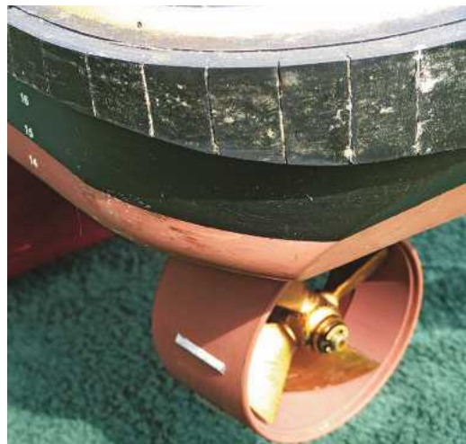
Above: Rear port quarter view showing the rubber side and stern fenders in their channels, and also the inner sleeve added to the Kort nozzle of the port drive unit which significantly improves the thrust by closing the gap between the propeller blade tips and the inside of it.
