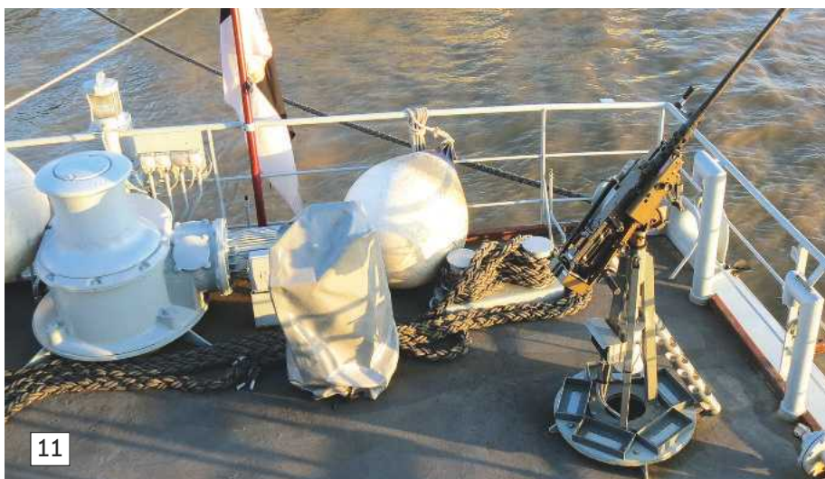
Photo 12. A warping winch is mounted on the centreline right aft.
