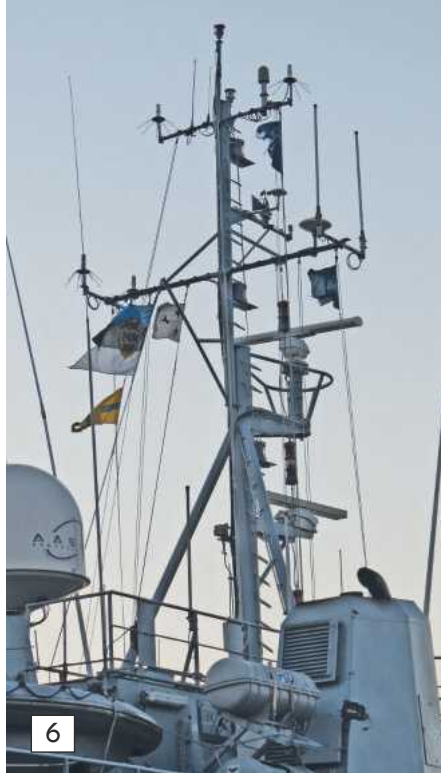
Photo 6. The tripod foremast is a bit of a throwback to an earlier era of warship construction.
