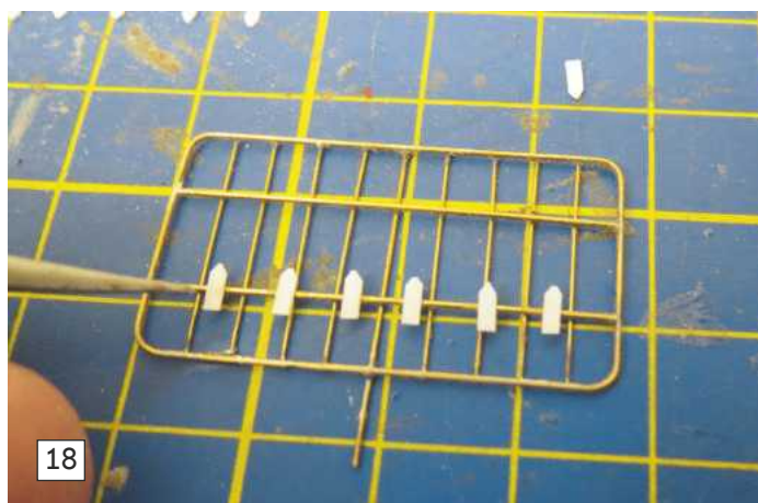
Photo 18. Each of the arrow head fittings was added to the front face of the IFF mattress.
