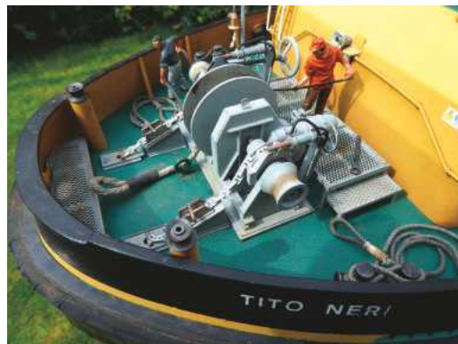
Below: Fore deck detail with the correct style anchor chains and their stoppers, hawse pipes, metal operator's platform and hydraulic hoses. The deck eyebolt is a non-standard model strong point for bow towing.
