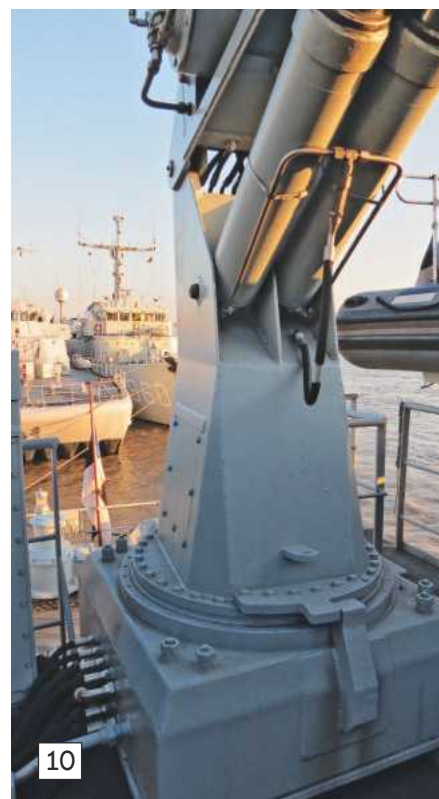
Photo 10. Down the centreline on 01 deck between the boats, is a basic hydraulic crane for lowering and retrieving them.
