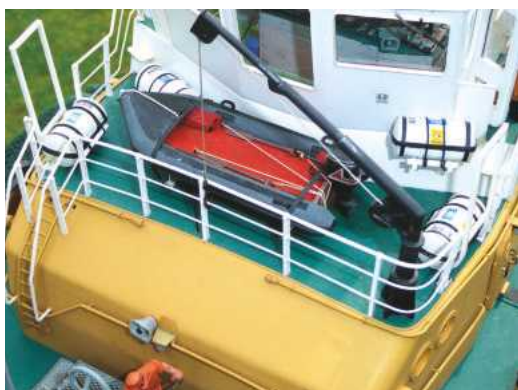
Left: Front of the superstructure showing some added details to the basic kit supplied RIB, the detailed liferafts and self-drenching pipework. Just visible is the bridge interior.
