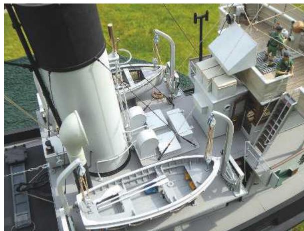
Left: The boat deck, starboard side, with its scratch built Welin davits and a Quaycraft resin cast lifeboat, plus the correct narrower and oval funnel. The wheelhouse interior is fully detailed and can be viewed through its open doors.
