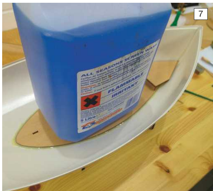
Photo 7. A heavy weight to keep it in place and a good bead of epoxy around the deep fillet at the edge of the deck seemed to be a much stronger arrangement and which could be easily applied once this internal lower (inner) deck unit was in place.
