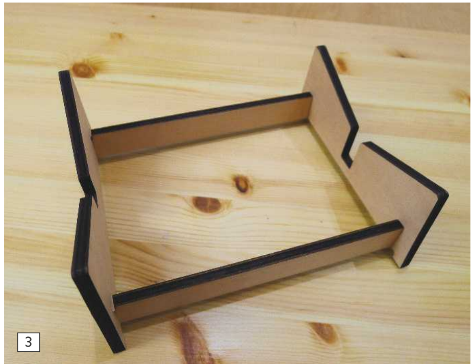
Photo 3. The stand was so tight to assemble that I decided not to risk damaging it by taking it apart again and just allowed varnish to secure the joints. The glazed edges of the ply look quite attractive when varnished, so were left as they were in this instance.
