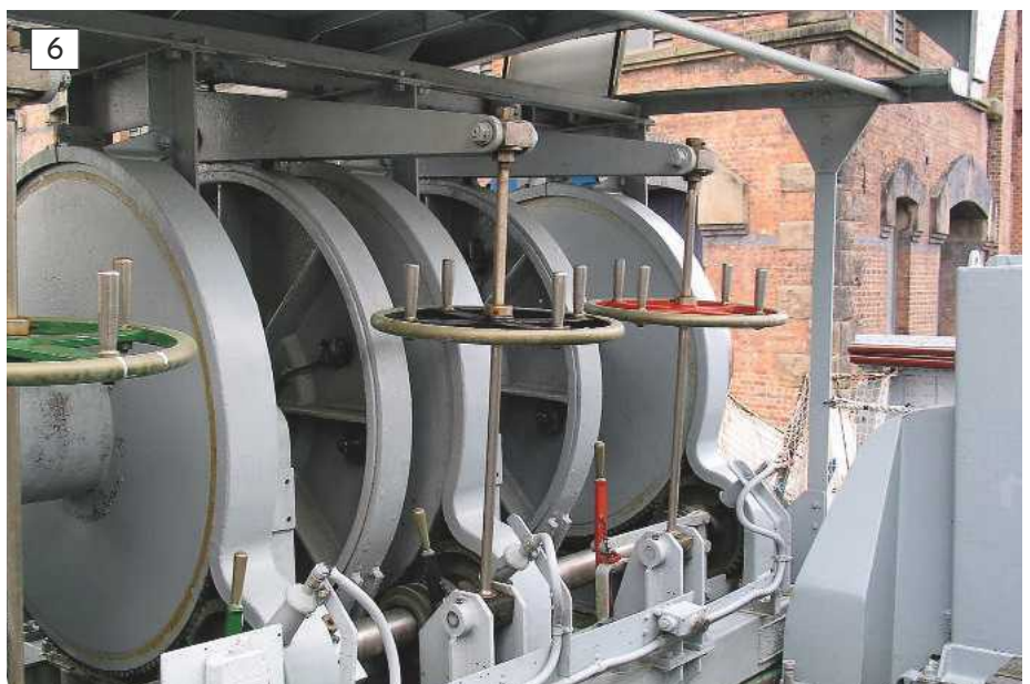
Photo 5. Moving on to the sweep deck aft of the funnel, the mine sweeping winch is a prominent feature.
