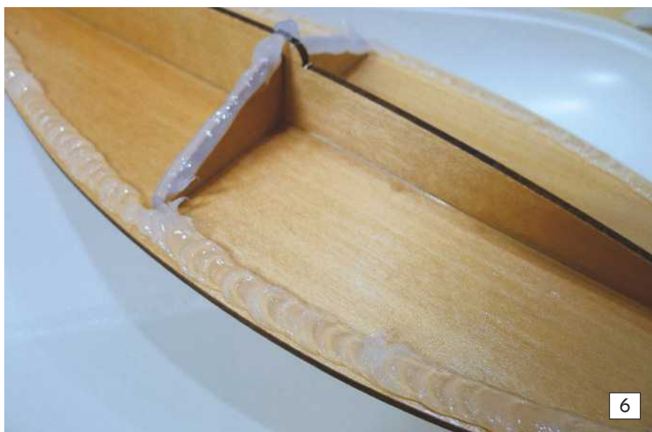
Photo 7. A heavy weight to keep it in place and a good bead of epoxy around the deep fillet at the edge of the deck seemed to be a much stronger arrangement and which could be easily applied once this internal lower (inner) deck unit was in place.
