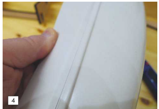
Photo 4. A surprisingly light cut is all that is required to part vacformed pieces. The cut should then open up cleanly and easily when you bend the two sides of the cut.
