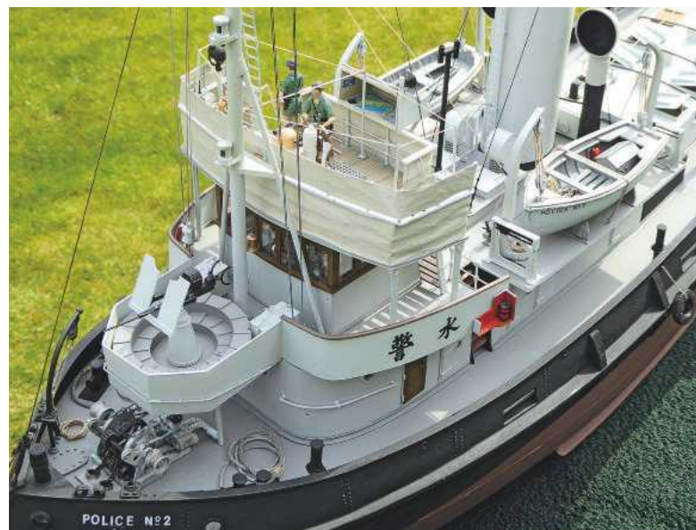
Below left: The wheelhouse and bridge area with its open door so as to view the detailed interior. The Chinese characters read, 'Soy Ging', which means 'Water Police'. Also, please note the Welin davits, inset steps and galley stove pipe.
