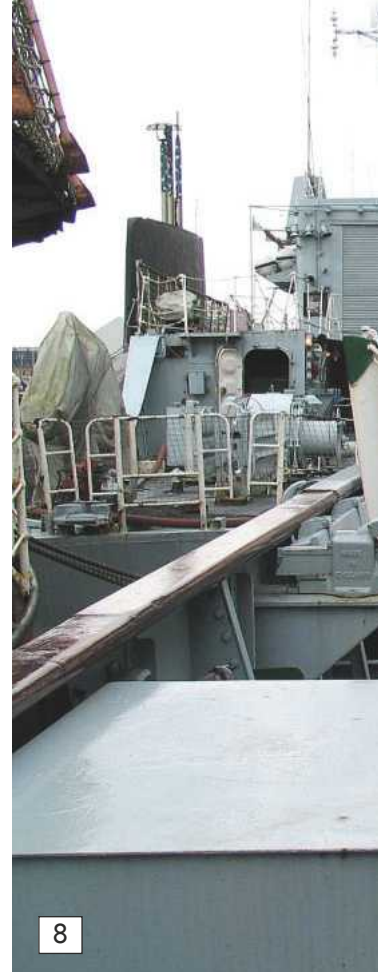
Photo 10. A good detailed picture of the sweep deck. It is from here that the floats etc. were deployed. Plenty of fittings here as well, such as various hatches, hydrants and bollards etc.
