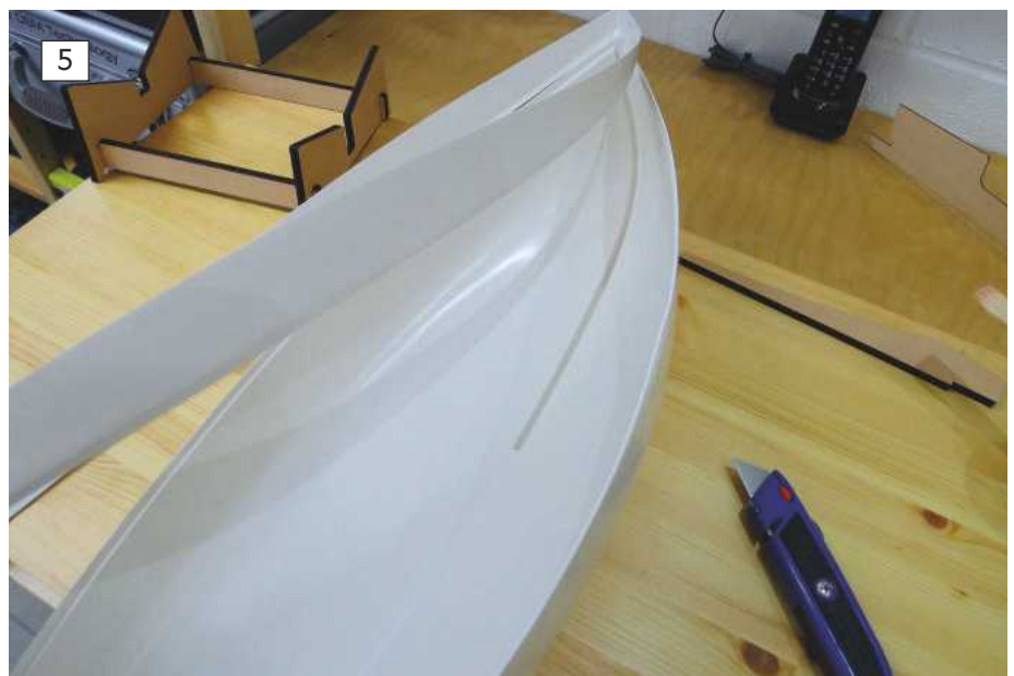
Photo 4. A surprisingly light cut is all that is required to part vacformed pieces. The cut should then open up cleanly and easily when you bend the two sides of the cut.
