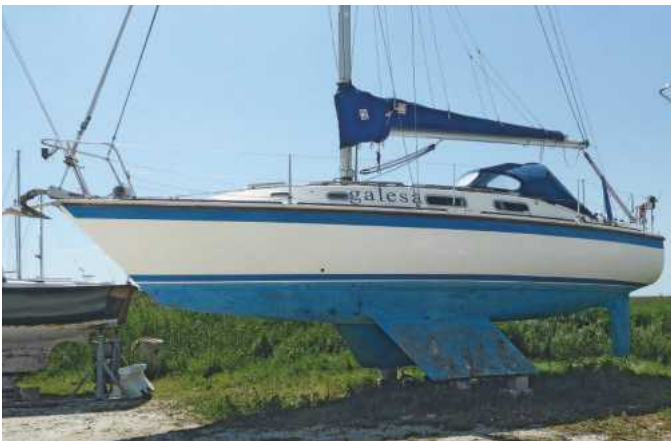
Above: A twin-keeled yacht, the benefit being that no hull supports are required when ashore or aground.
