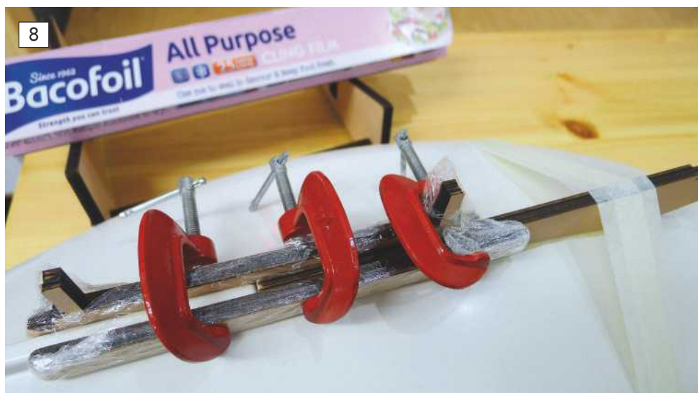
Photo 8. Ensuring the keel is aligned with the hull isn't easy, so braces either side were arranged to create guide pieces while the glue sets. These were covered with cling film to ensure they did not become part of the final structure!
