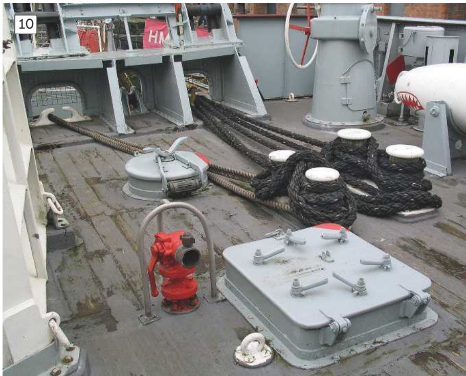
Photo 10. A good detailed picture of the sweep deck. It is from here that the floats etc. were deployed. Plenty of fittings here as well, such as various hatches, hydrants and bollards etc.
