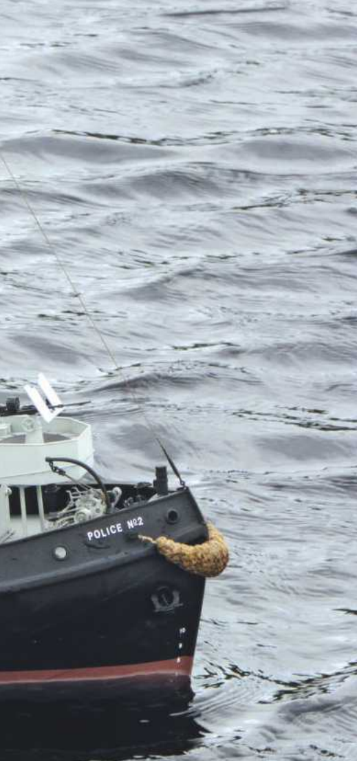
Left: Police No.2 on the Southport MBC lake showing all its major features and colour scheme. It has a scratch built upper superstructure and most of the fittings, all on a Mountfleet Models GRP Empire Ivy hull.
