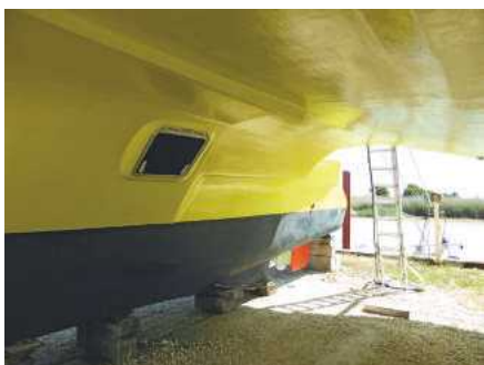
Below: A crew escape hatch on a catamaran for use in the event of a capsize and turning completely upside down.
