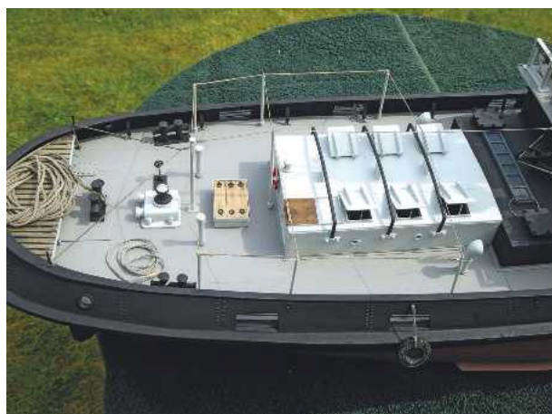
Below: The rear towing deck with its new scratch built deckhouse, salvage hatch and hook area, oil filler and hatches. Please note the supports for the deck awning, which is still to be made at the time of writing.
