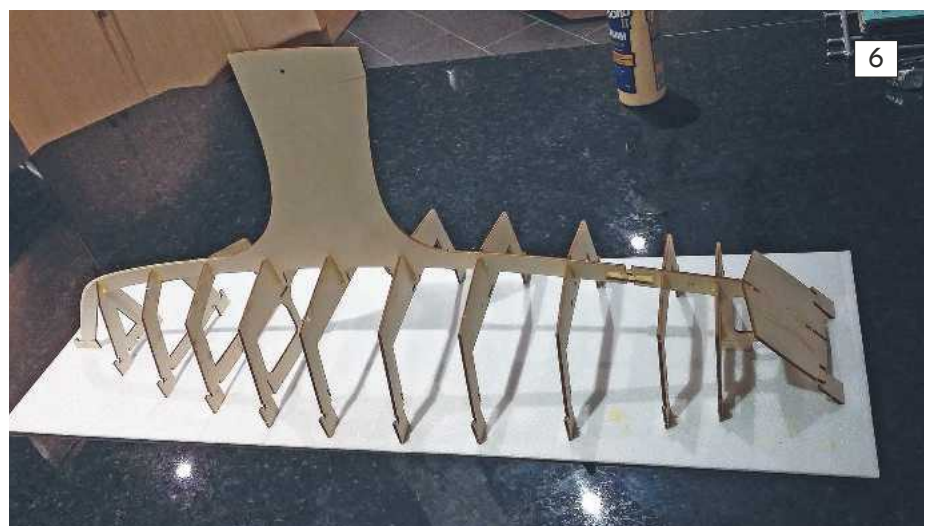
Photo 5. The hull frames are set in place on the Depron jig.
