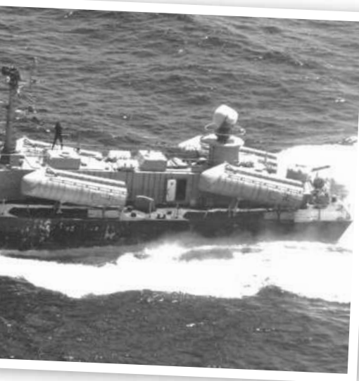
ABOVE: An OSA 2 205U boat with its AK 230 30mm guns mounted fore and aft.
