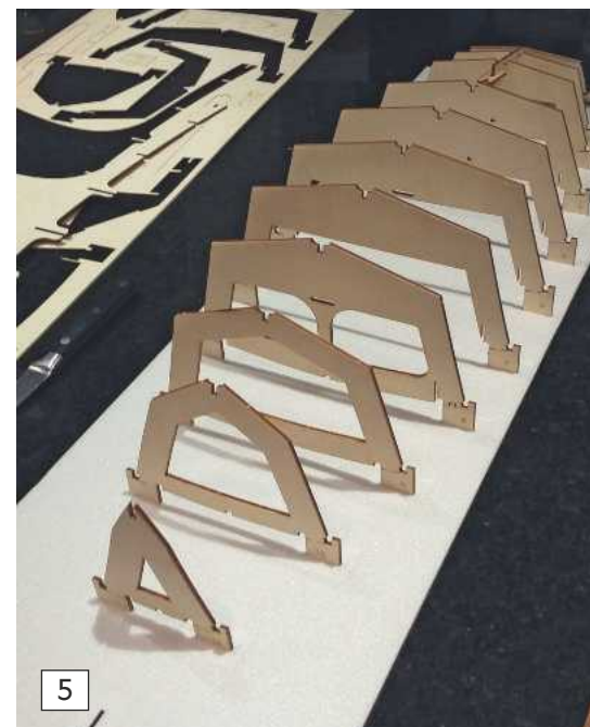
Photo 5. The hull frames are set in place on the Depron jig.
