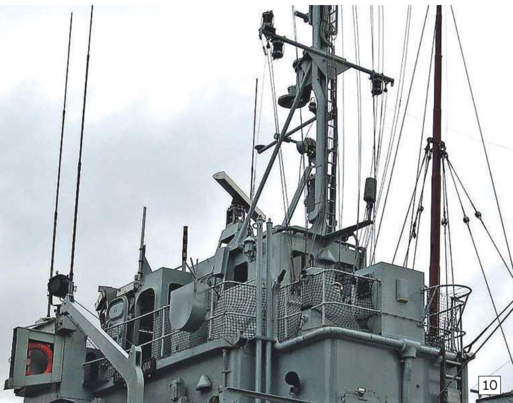
Photo 7. The after facing windows of the chart room and the signal halyard cleats.
