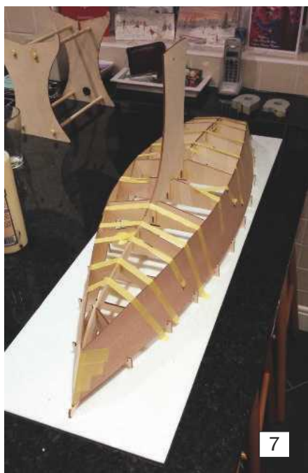
Photo 7. Hull sides glued into position.
