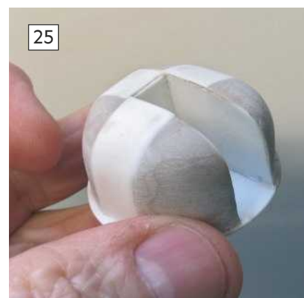
Photo 25. Filler has now been applied, allowed to set and then sanded to achieve the desired shape.
