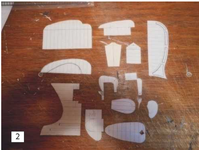
Above: The principal measurements of the small electric outboard were all doubled to make these templates.
