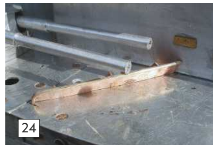
Photo 24. The breakwaters were each fabricated from brass and copper, and screwed to the decks, this one being mid-way along the starboard deck in front of one of the wing turrets.
