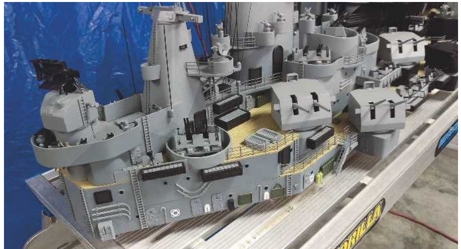
Above: The main superstructure unit has the life jackets, doors, grills, ladders, oxy-acetylene bottles, radars, binoculars, stairways and other fittings all 3D printed.
