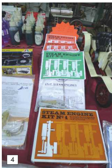
Photo 4. The Unit Steam Engine (USE) system, is extremely flexible and allows a combination of cylinders to create a self-starting engine. However, the engine will be of a significant size and fettling the parts to make them operate smoothly and reliably might frustrate those who haven't tried model engineering.
