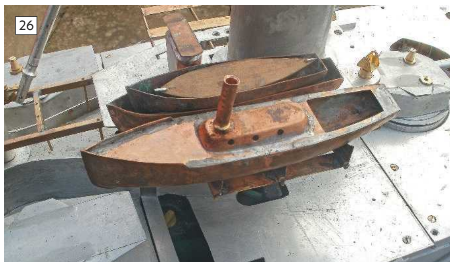
Photo 26. The ship's boats are fabricated from annealed copper pieces, all silver-soldered together.
