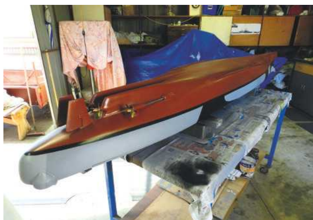
Above: The hull, here inverted, was painted in USN camouflage Measure 32, Design 22D by March 2013.
