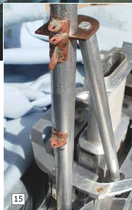
Photo 13. The next stage in fairlead production was to solder the top (fairlead) part to its angled base.
