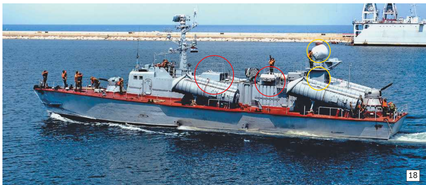
Photo 18. The box shaped vents are ringed in red as fitted to the OSA 2 Type 205U (Please note that ringed in yellow is the Base Tilt radar unit, referred to later in the text).
