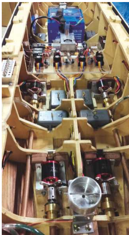
Above: The main deck is totally removable to enable easy internal hull access. The aluminium cup in the foreground is a main turret drive coupling and please note the bank of electrical switches on the port side. Active switches have a red LED to indicate when On.
