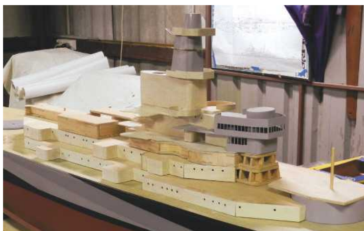
Above: The main superstructure unit under construction with 1mm cladding on the lower deck sections. The bridge part is completed and undercoated, July 2013.
