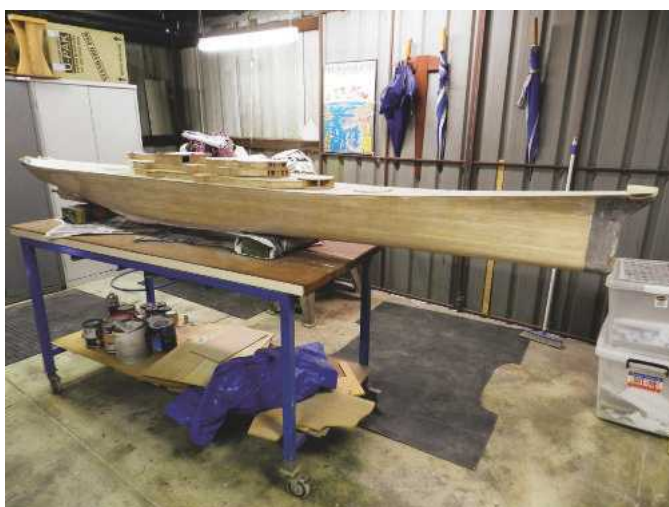
Above: The hull was fibreglassed to stabilise the timber planking and the superstructure framework has been started Nov 2012.
