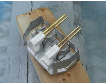
Right: An unpainted 40mm quadruple Bofors mounting. USS Missouri in 1944 had 20 of these. Eighty barrels were turned from brass, with each taking approx. 15 minutes to machine. The armour protection is 0.5mm galvanised steel, laser cut and folded using CAD drawings.
