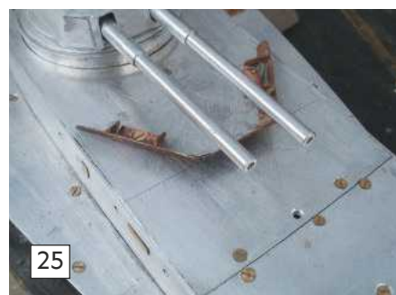
Photo 26. The ship's boats are fabricated from annealed copper pieces, all silver-soldered together.
