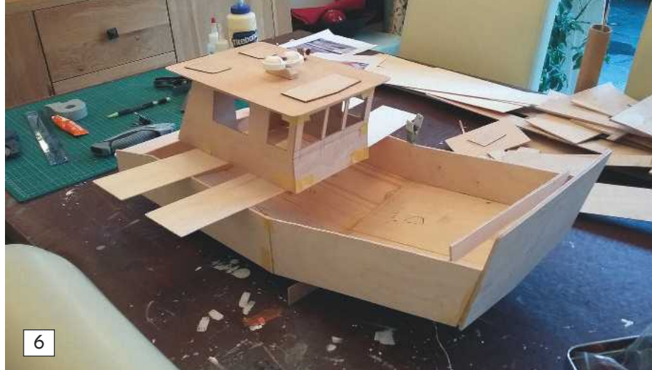
Photo 6. The cabin is from thin plywood and is here being offered for scale and fit.
