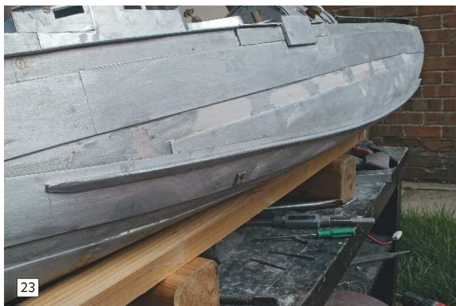
Photo 23. The bilge keels were formed from aluminium square section, cut and filed to a triangular cross section and screwed to the hull sides.
