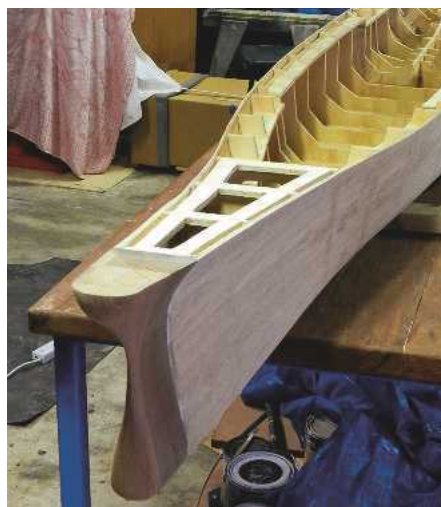
Above: The unpainted hull with Western Australian Jarrah bow and stern blocks.
