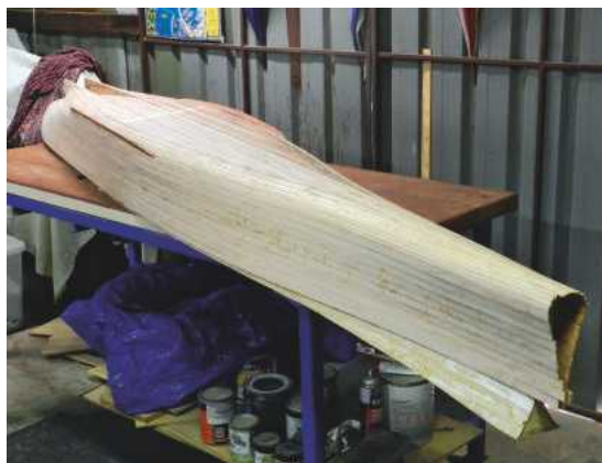
Above: The frames were double planked using 14mm x 3mm x 3.6M long Tasmanian Oak planks. The bilge keels were glued to the first layer (August 2012).
