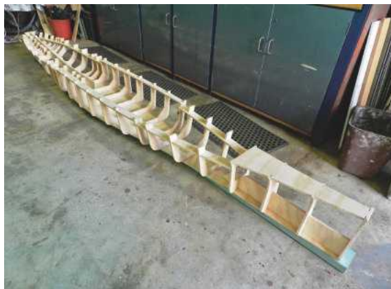
Above: The 1:96 scale engineering drawings were supplied by Floating Dockyard (USA) and the frame patterns, keel and supporting sub-frames drawn using CAD to 1:80 scale and cut and assembled ready for planking (May 2012).
