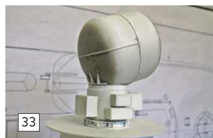
Photo 33. The basic assembly is temporarily mounted on to its platform. Please note that the second access point into the drum has been added across the diameter and length of it. Additional detail will be added at a later date.
