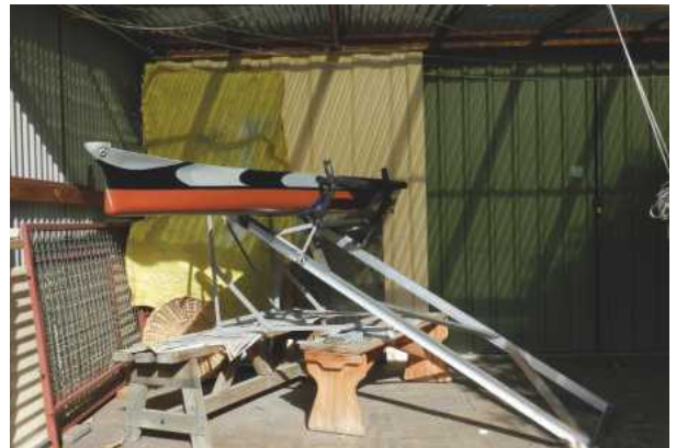
Above: This is the launching slipway set-up. The model is winched sideways down into the water and this negates the need for us humans to bend over.
