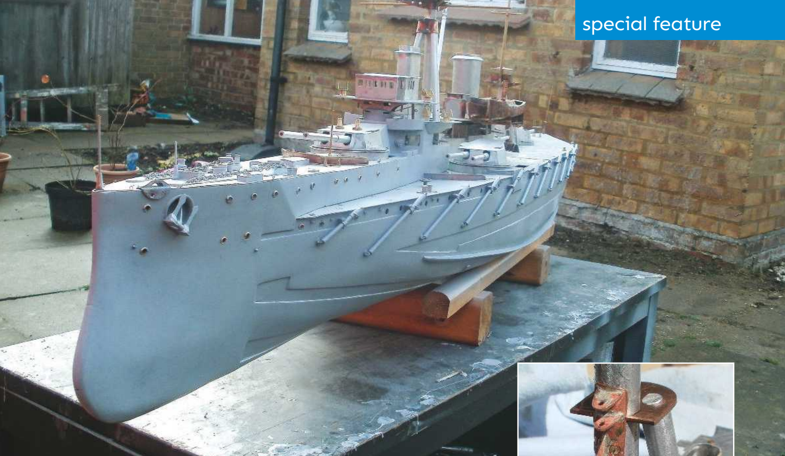
Photo 6. The main anchor stocks have been fabricated from flat and round brass bar, and a completed one is seen here lurking in a hawse hole.
