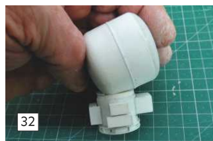
Photo 31. Body filler has been used on each end of the redundant container top, here with the initial assembling and fitting into place of the electrical boxes that surround the styrene tube that supports the completed drum.
