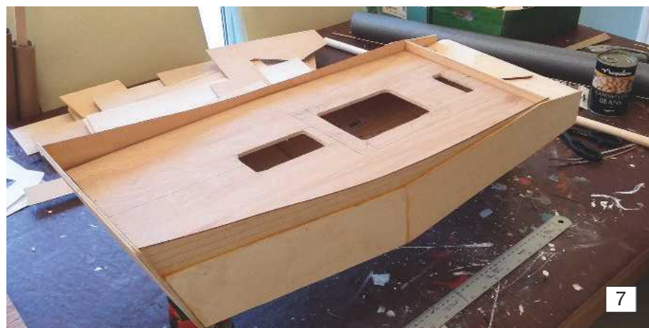
Photo 7. The deck with its access holes for the motor, batteries and rudder linkages etc.
