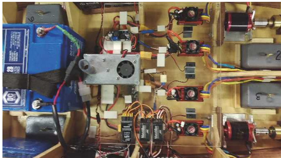
Above: Another view of the electronics showing the Perspex sheet base (in front of the blue battery) with the esc's, receiver, smoke generator and MatchBox hubs. These MatchBox hubs (centre bottom of picture) are programmable devices, used to connect all three main turrets for their correct coordinated rotation and gun barrel elevation to the receiver, but still using only two channels. This is so the three main turrets and their guns function as one together, on either beam, or fore and aft.
