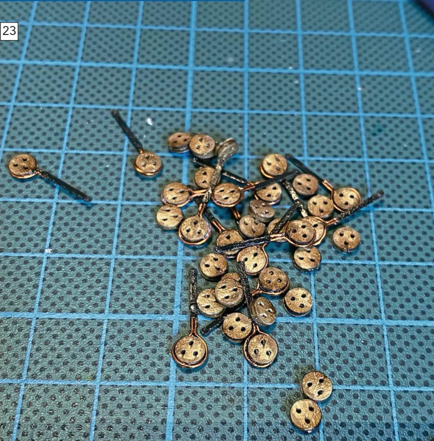
Deadeyes made up, with the iron (copper wire) hardware attached.
