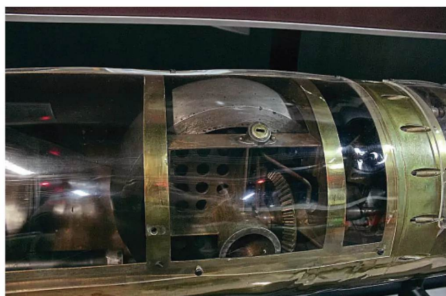
The flywheel of a Howell torpedo.
