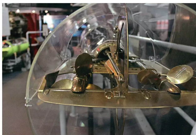
Twin counter-rotating propellers of a Howell torpedo.
