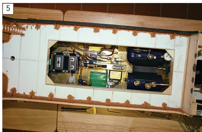
For the Ben Ain, as Richard had decided that the model was coming in every 20-30 minutes anyway, he wasn't sure of an automatic boiler feed system would be of any real value, so he instead opted for a simple manual feed pump, seen here nestled amongst the more complex gas control systems.
