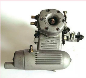
A clean example of the bigger OS30 (5cc) glow marine engine (flywheel off).
