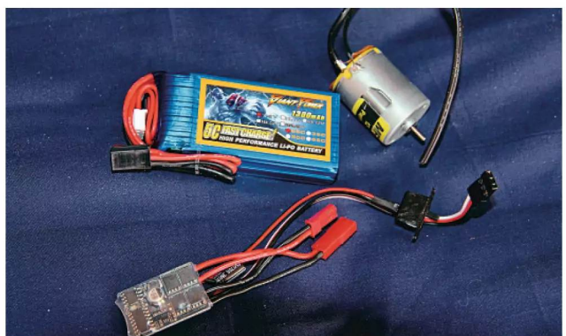
The running gear for the STAB, and, while Nick's motor proved to be underpowered, the Li-Po battery and cheap ESC (Electronic Speed Controller) is correct.
