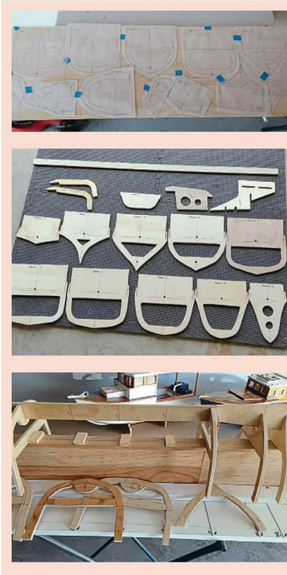
Plotting and cutting out bulkheads and fixing to jig.
