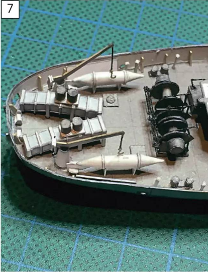
The stern of the model, showing the tiny tubes, cone shapes and circles used to make up torpedoes and winch components. The black steel spindles of the winch were made from silk thread stiffened with superglue.
