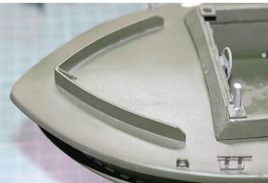
The final detail on the deck of the model is the bow wave deflector, which guides water away from the cockpit well.
