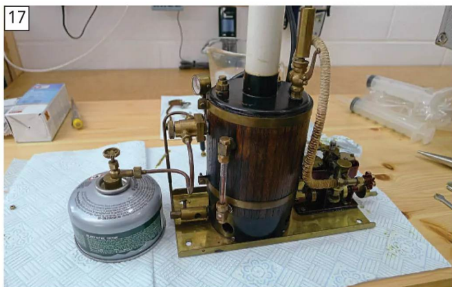
Never underestimate the value of being able to remove the entire plant on a single base for maintenance and cleaning. The Borkum plant can be out of the boat and onto the bench in a few minutes so that it can then be easily worked on.
