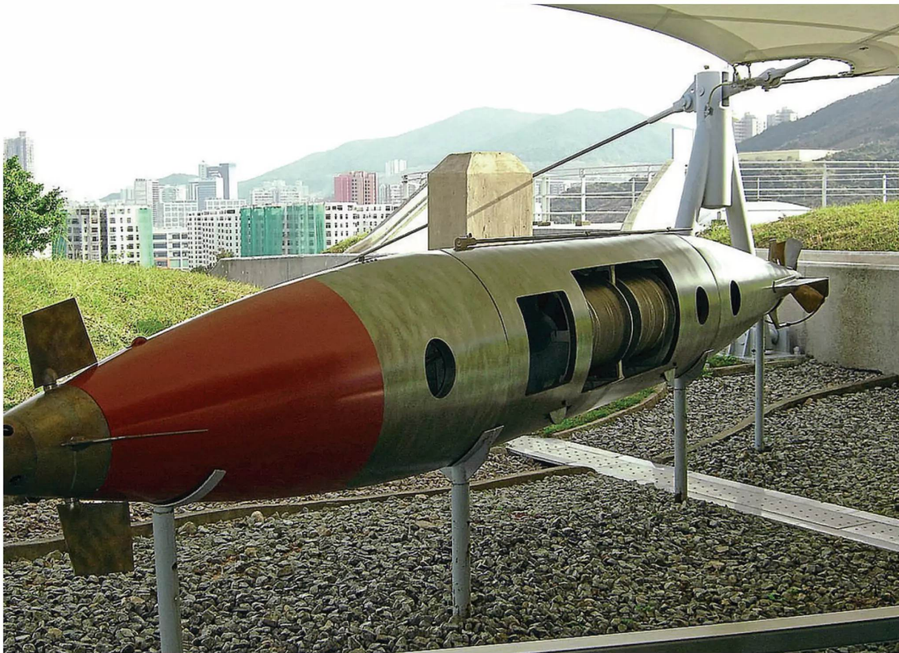
A Brennan torpedo replica.
