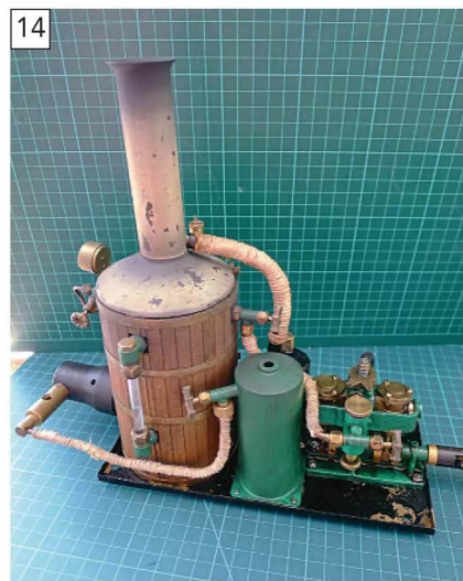
For beginners to steam, as well as more experienced steam modellers, the advantages of a plant entirely located on a single base are hard to ignore. All you need to do is fit the base into the bottom of the hull and connect up the shaft and the control valve linkage.
