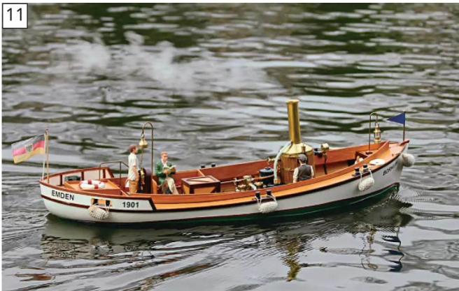
Again, the Borkum proving invaluable as a test bed for the Miniature Steam Models Clyde plant. This time the entire Cheddar plant was removed and the Clyde plant fitted in its place, requiring very little in the way of modification.
