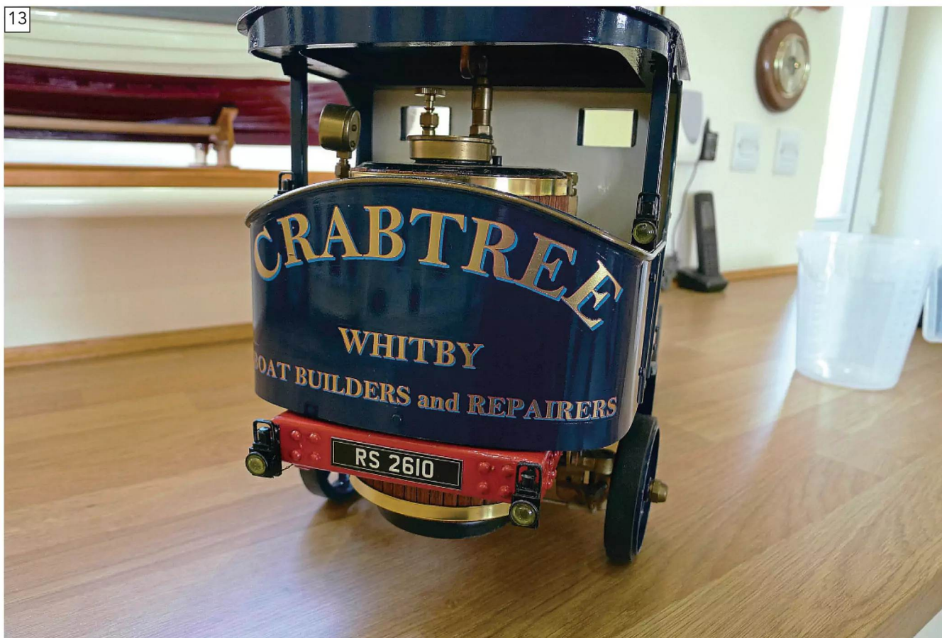
13 In this case, the transfers were applied to a gloss paint, so an additional clear coat was not necessary. The large curved upper lettering is all one large transfer and being printed from Richard's own design in three colours, ended up being very expensive. It is now sealed in with a coat of clear gloss enamel varnish.
