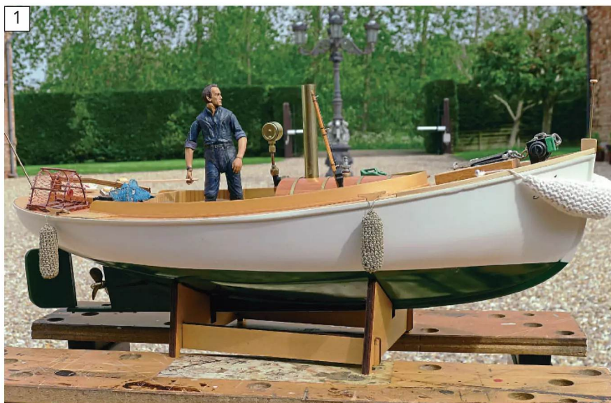
Back in 2017 this Krick Anna kit was assembled to demonstrate that a cheap and simple steam powered model could be put together. The total cost at the time was less than £400, which included the radio set and all electronics, yet the model is still a pleasure to run.
