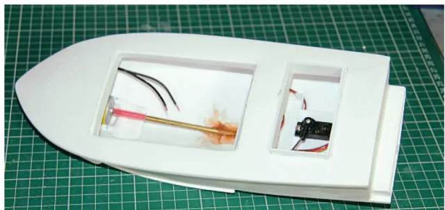
Once the deck is fully fitted, there's just enough in the way of access to get the Li-Po battery in and out, and to make minor adjustments with lead sheet to ballast to the trim line later.
