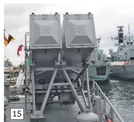
Photo 14. Mounted on the stern are the four launch boxes for the Chinese made C 802 anti-ship missile.
