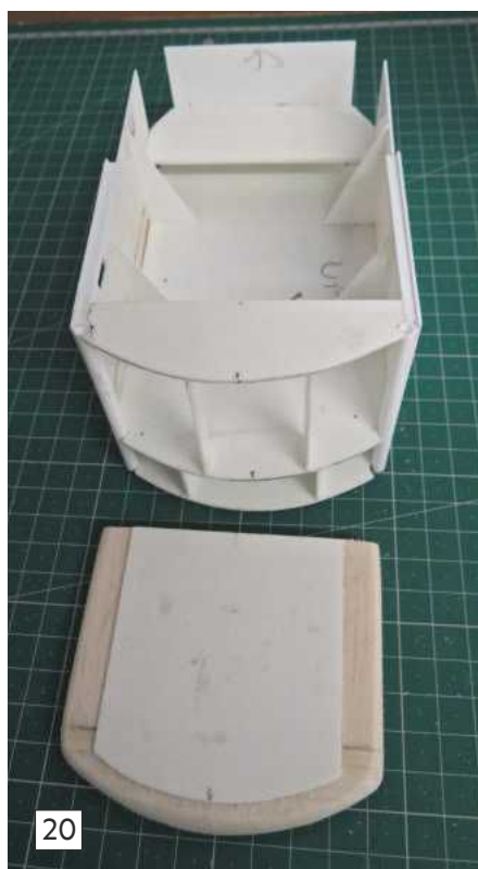
Photo 20. In order to achieve the rounded contours of the sides and roof, it is easier to use some balsawood sheet.
