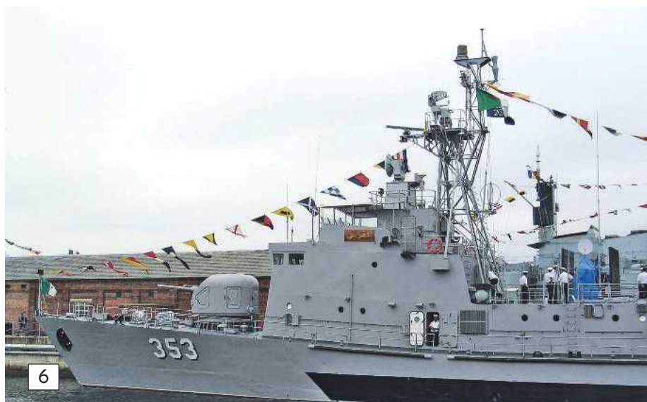
Photo 6. A general view of the port side. Please note that the hull rubbing strake starts midway along the length of the forward deck housing.
