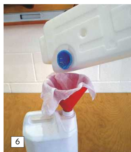
Photo 6. A simple filter arrangement with a piece of linen cloth. Tumble Dryer condensate will usually contain lint that will collect in your boiler if you use that water in an unfiltered condition.
