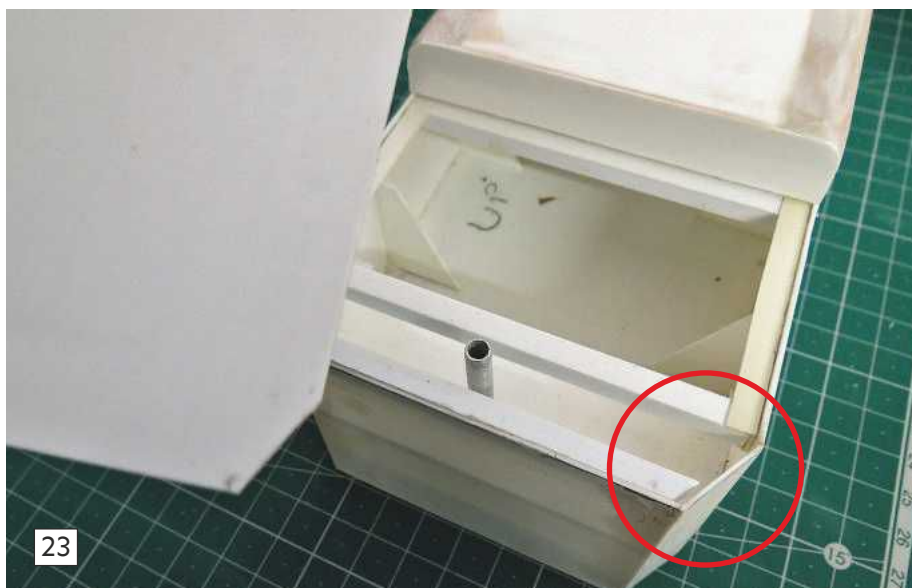
Photo 22. Filler has been added around the top edges of the roof section and the vertical corners of the wheelhouse front, all blended into nice curves.
