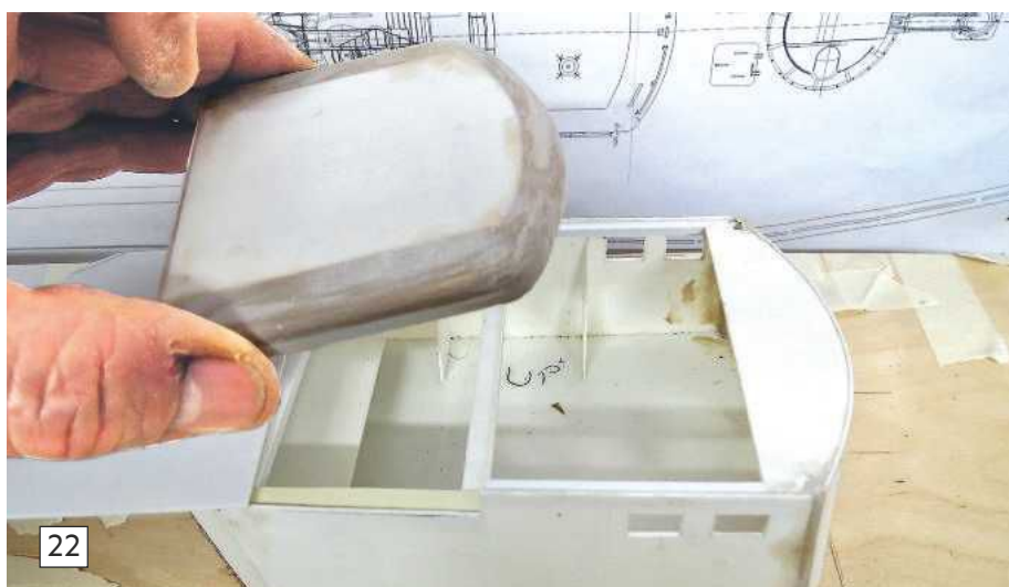
Photo 20. In order to achieve the rounded contours of the sides and roof, it is easier to use some balsawood sheet.
