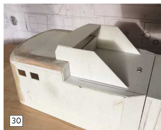
Photo 25. The main aft part of the deck housing was initially created around a box of 1mm marine ply and balsa wood, all skinned with styrene sheet.
