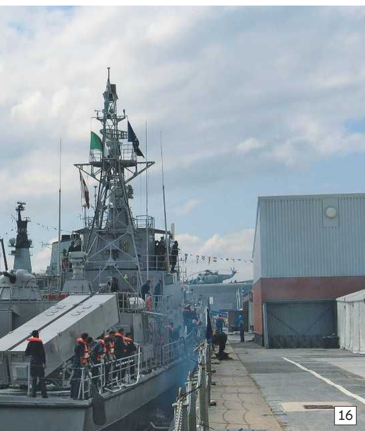
Photo 14. Mounted on the stern are the four launch boxes for the Chinese made C 802 anti-ship missile.
