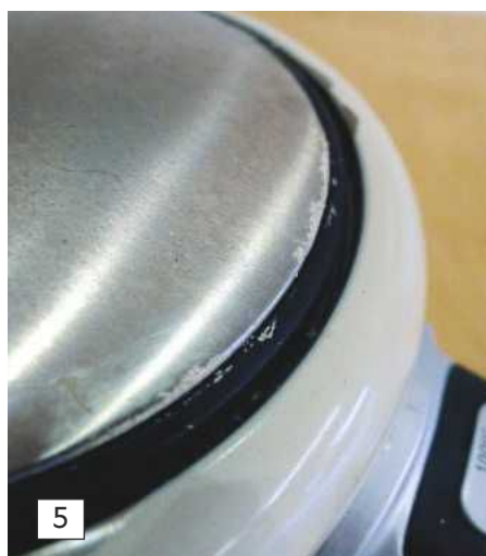
Photo 5. Hard tap water will soon manifest itself by a build-up of deposits inside, and even outside, a domestic kettle. If you see such deposits, be aware of the consequences and consider the possible alternatives.
