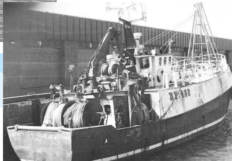
Left: Bounty BF287 after having a three quarter length shelter deck added. This picture shows the now fully modernised rig with power block and net drum aft, trawl winch forward under the shelter deck and cod end hatch with derrick forward on the starboard side.
