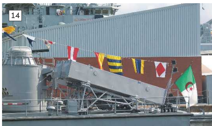
Photo 14. Mounted on the stern are the four launch boxes for the Chinese made C 802 anti-ship missile.
