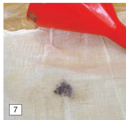
Photo 7. These are the deposits collected after a single use of the filter.
