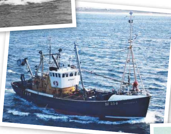
Above: Arnisdale (2) BF394 with its new superstructure unit and please note the trawl winch is now positioned forward at the break of the whaleback.
