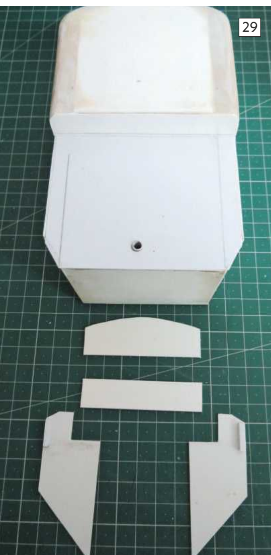
Photo 25. The main aft part of the deck housing was initially created around a box of 1mm marine ply and balsa wood, all skinned with styrene sheet.
