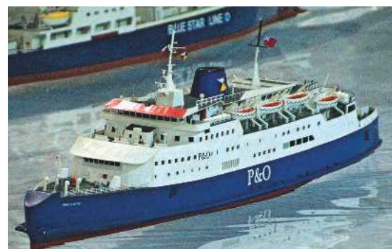
Above: Pride of Hythe from Linkspan Models makes a fine sight when under way. This type of working model is difficult to build successfully due to the high and inevitably heavy upperworks, but in this case its stability looked absolutely fine.
