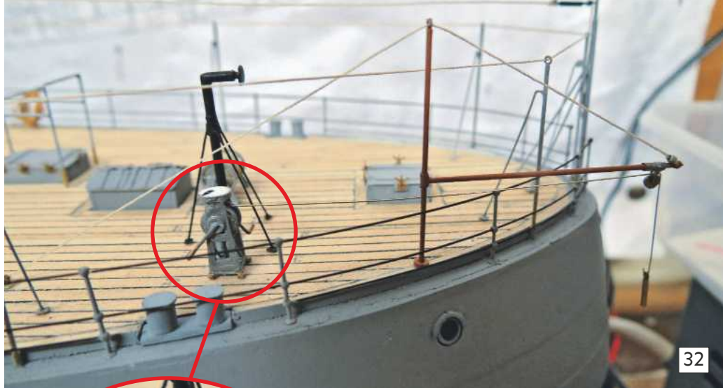
Photo 32. The sounding machine and spar on HMS Skirmisher as per the builder's drawings.
