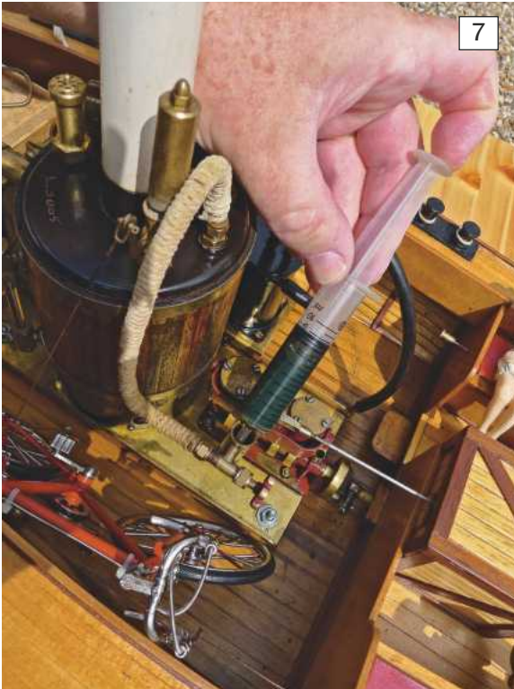
Photo 7. Topping up the displacement lubricator is a quick and easy job if the engine is easily accessible and you can remove its cap easily. Don't use a needle on this syringe because the thick oil is very hard to squeeze through it and don't forget to remove the water with a wick as the oil displaces it.
