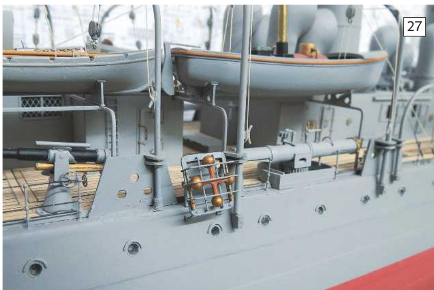
Photo 27. The Night Life Buoy and its frame fitted to the side of the hull.
