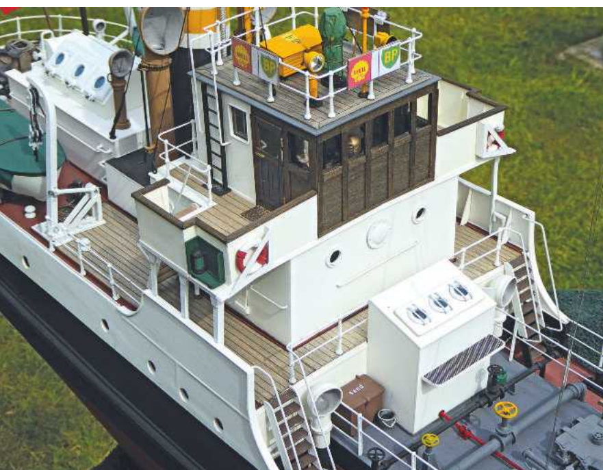
Above: Starboard view of the bridge. The timber wheelhouse has a fully detailed interior with its bridge roof equipment and a sand box and bucket on the main deck for minor spillages.
