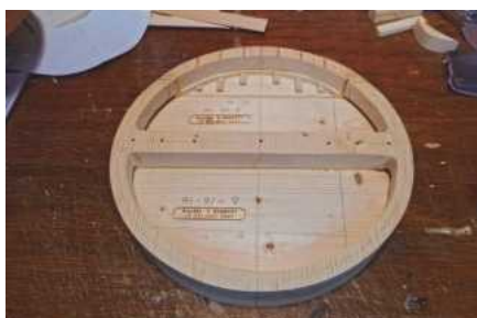
The basic hull is circles of wood with their centres cut away.
