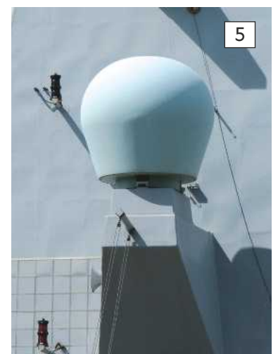
Photo 6. Almost all of the exposed structures are designed to minimise their radar cross section,
