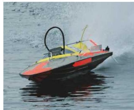
Above: Mike Gelson's Stratos at speed - the black thing sticking up is the starter belt. (Photo courtesy of Judith Beesley)
