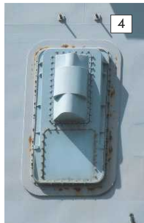
Photo 4. The UAT early warning antennae.
