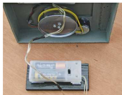
Above: The radar rotates on Emily & Jack and this is the drive mechanism.
