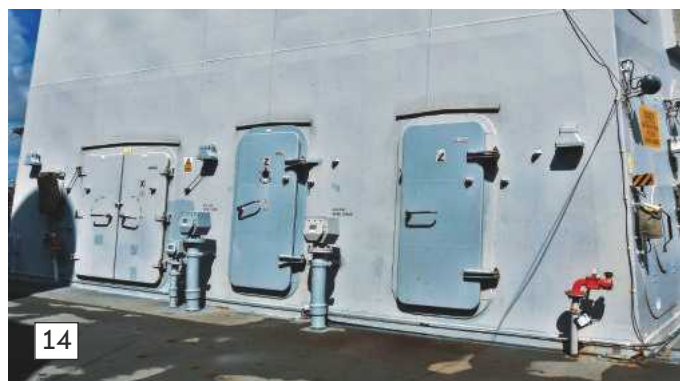
Photo 13. Looking towards the rear of the exhaust uptake and please note the staggered door hinges.
