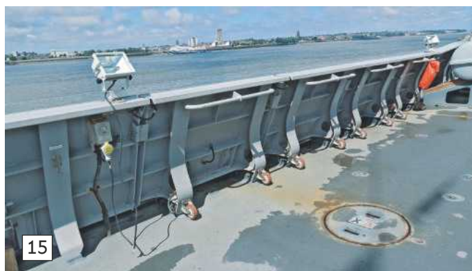
Photo 15. The bulwark has a number of removable panels, shown here with castor wheels.
