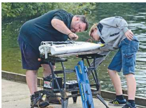
Left: Mark Wild adjusting the carb' on the OPS engine of Luke's Sprint Catamaran. (Photo courtesy of Judith Beesley)
