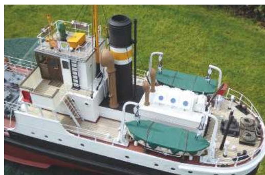
Above: The boat deck and bridge superstructure with its timber wheelhouse, enlarged funnel, mast, steel lifeboats and other detail changes.
