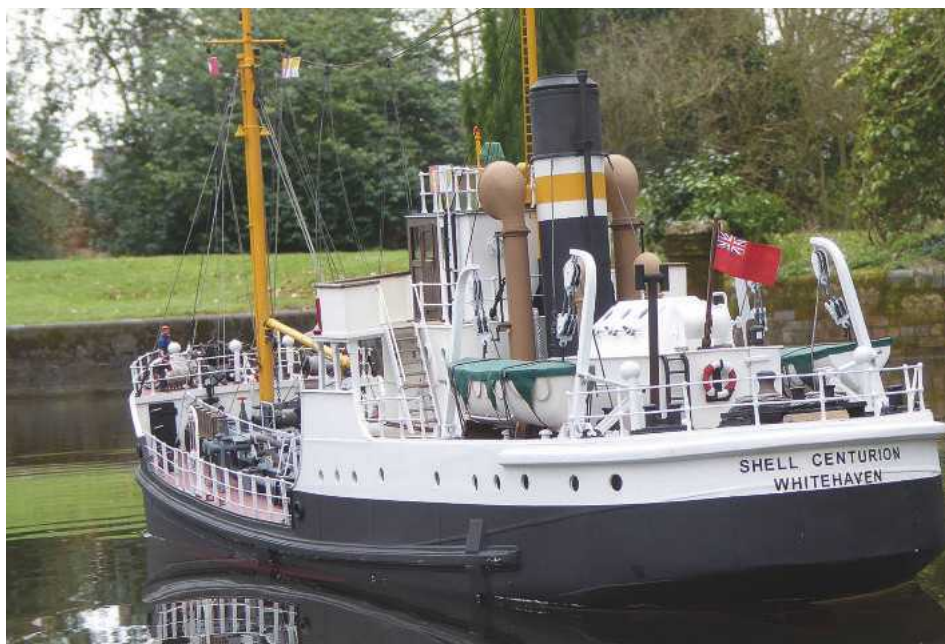
Above: The boat deck and bridge superstructure with its timber wheelhouse, enlarged funnel, mast, steel lifeboats and other detail changes.
