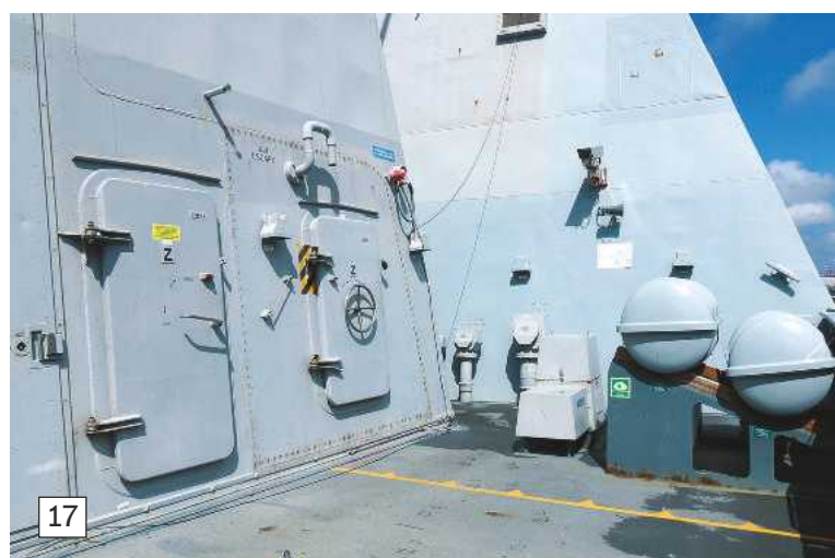
Photo 16. Starboard side of the communications mast. Note the deck eye plates to assist with replenishment at sea operations.
