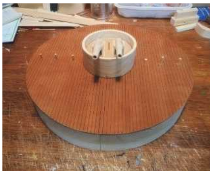
The deck is of Mahogany, lined to represent the planks.
