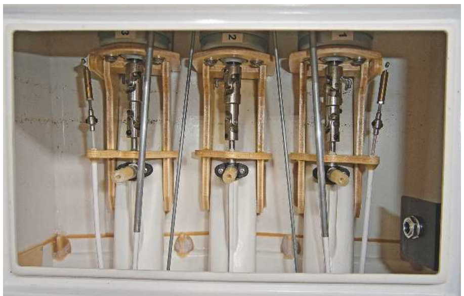
Above: The motor to propshaft stainless steel couplings are from an r/c car.
