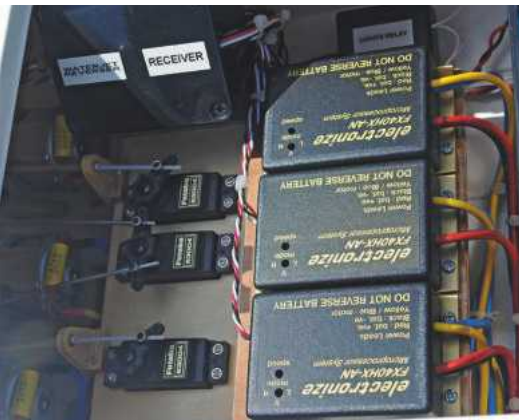
Above: Three forwards only Electronize esc's have been installed.
