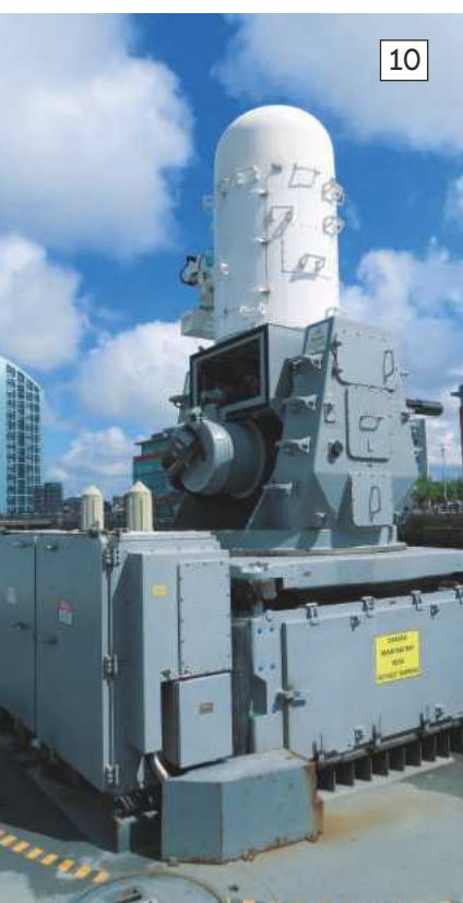
Photo 10. One of the two Phalanx systems mounted amidships. These are modular and the entire mounting can be removed for major servicing ashore.
