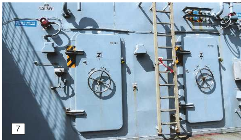
Photo 7. The exterior watertight doors fitted to HMS Duncan use a centre wheel to open and close them, whereas those of the first of the class HMS Daring have a single lever to engage or release the dogs around them.
