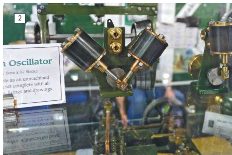
Photo 2. The little oscillators have changed very little since they were first introduced many years ago and are still very capable and robust engines capable of competently powering a model boat.
