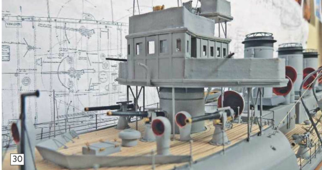
Photo 30. Canvas dodgers on the forward searchlight and compass platform, and around each side of the open bridge.
