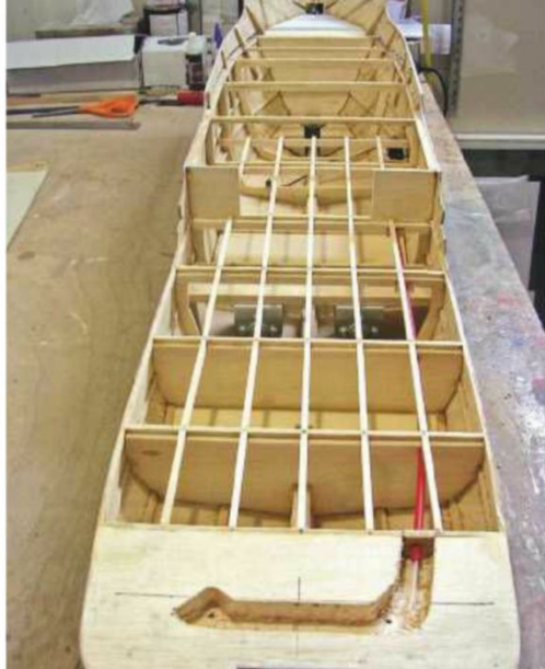
ABOVE: The main deck reinforcement beams. Note the stern block carved out to accommodate the rudder linkage.
