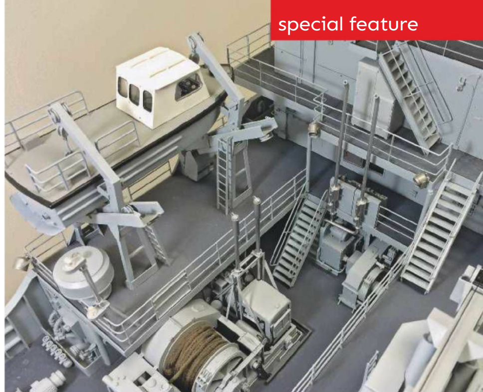
ABOVE: Overhead view of the towing machine area. The winch control station is visible under the overhang of the Upper Deck.
