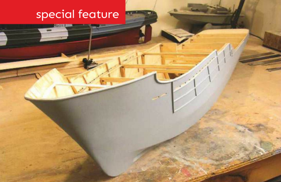
ABOVE: The completed hull in primer after the rubbing strakes were installed and yes, that is another tug behind!
