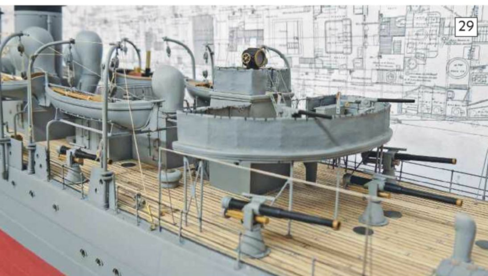
Photo 29. Here are the results of using masking tape on the aft searchlight and 3pdr platforms.
