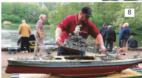
Photo 8. All models and especially warships, require careful handling when requiring access into the hull. It is here that a model becomes prone to accidental damage, so a well thought - out sequence for dismantling is essential.
