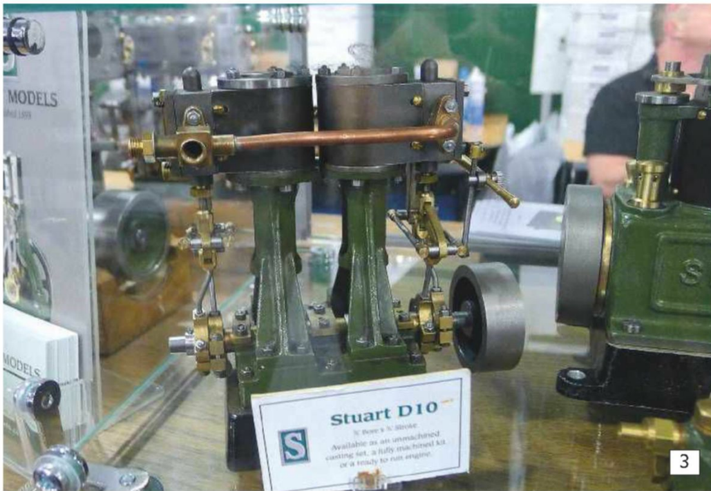
Photo 3. The D10 engine has been produced for many years and has even had model boat plans produced specifically for it. The engine remains a very competent engine for a significantly-sized model boat and when fitted with reversing gear, it will be just as manoeuvrable as any model on the pond.
