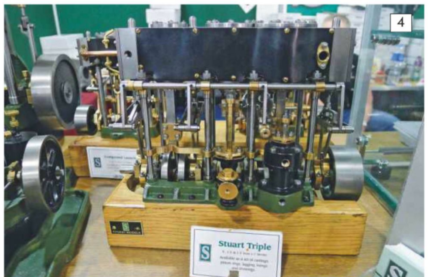
Photo 4. Possibly the ultimate model steam engine to most in the hobby would be the Stuart Triple Expansion engine. Possibly more as a display item rather than to be placed in a model, as the engineering required to complete it deserves to be enjoyed as much as possible.
