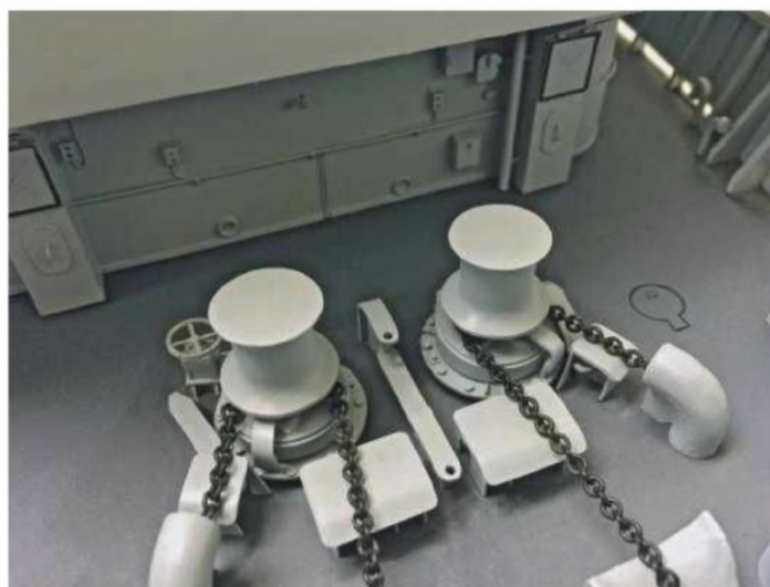
ABOVE: An overhead view of the anchor handling machinery.
