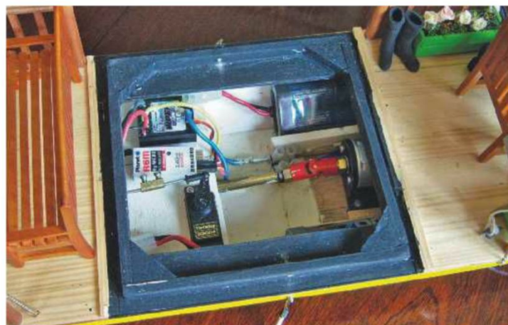
ABOVE: This shows the driveline. There is nothing remarkable in this as the hull is not dissimilar to a powered barge or that of a Springer model tug.
