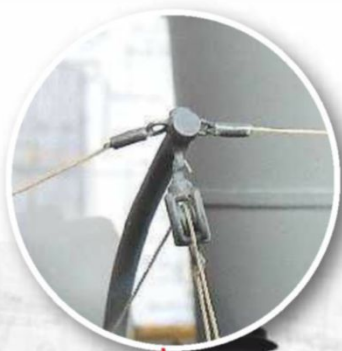
Photo 19. On the forward 32ft cutter the aft davit guy is secured to the top edge of the deck housing.
