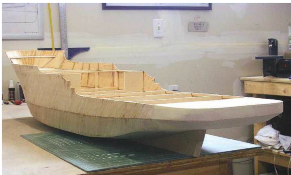
ABOVE: The completed hull with bow and stern blocks fitted, prior to fibreglassing.
