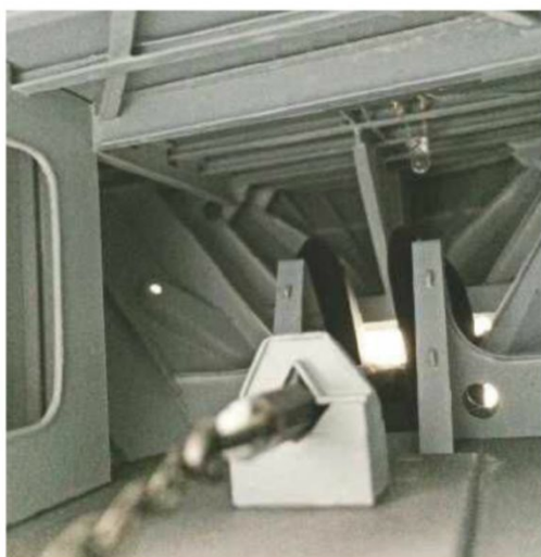
LEFT: A view inside the shelter deck overhang, showing structural steel members and the Moorfast anchor.
