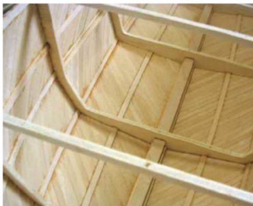
ABOVE: The inside of the hull after planking, showing the radial planking technique to good effect.
