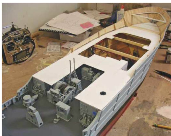
ABOVE: Foc'sle deck fixed in place, showing the final size of the access into the hull.
