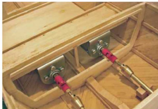
RIGHT: The motors had to be installed upside-down to keep the shafts parallel to the keel.
