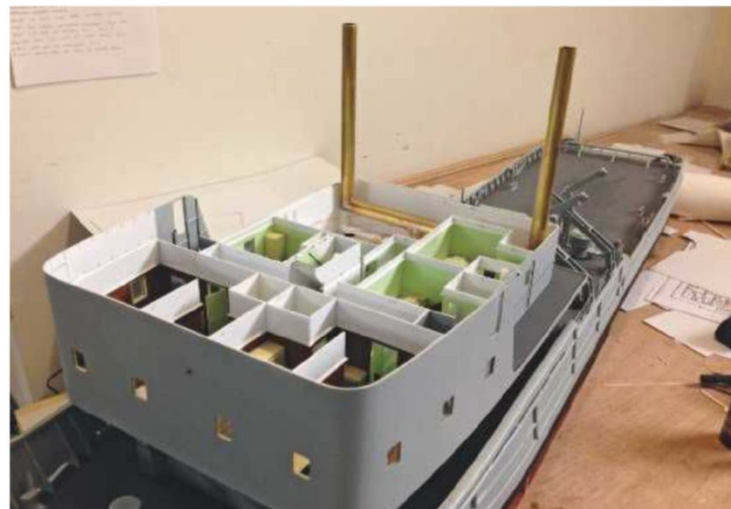
ABOVE: Progress continues on the upper deck; the brass uptake tubes for the smoke unit have been installed.
