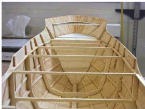
ABOVE: The inside of the hull after planking, showing the radial planking technique to good effect.
