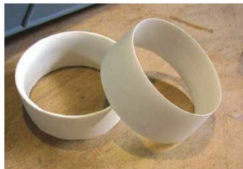
RIGHT: The Kort nozzles were made from 2 inch (50mm) PVC couplings, sanded to shape on a wood lathe.
