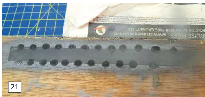
Photo 21. Each litho plate disc is placed on a length of masking tape and airbrushed using a paint shade called 'Aged Metal'.
