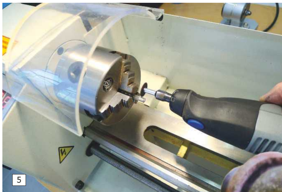
Photo 5. Cutting gauge glasses to an accurate length is never easy, but with a bit of care and thought you can do it safely and reliably. If you don't have a lathe, then holding the glass in a hand drill chuck will work just as well, the drill preferably held in a vice to ensure it remains secure. Don't forget to always use safety goggles and a mask when performing such an operation.
