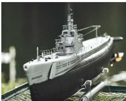
LEFT: The superb Gato submarine model by John Robinson of the Alvaston Pirates MBC. This model is 6 feet long and is packed with the owner's own control electronics which incorporate a system to allow the submarine to automatically hover at a preset depth in the water.
