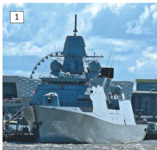
Photo 1. A bow-on view that shows the sloping and angled shape of many of the warship's structures designed to give it a low radar cross section.
