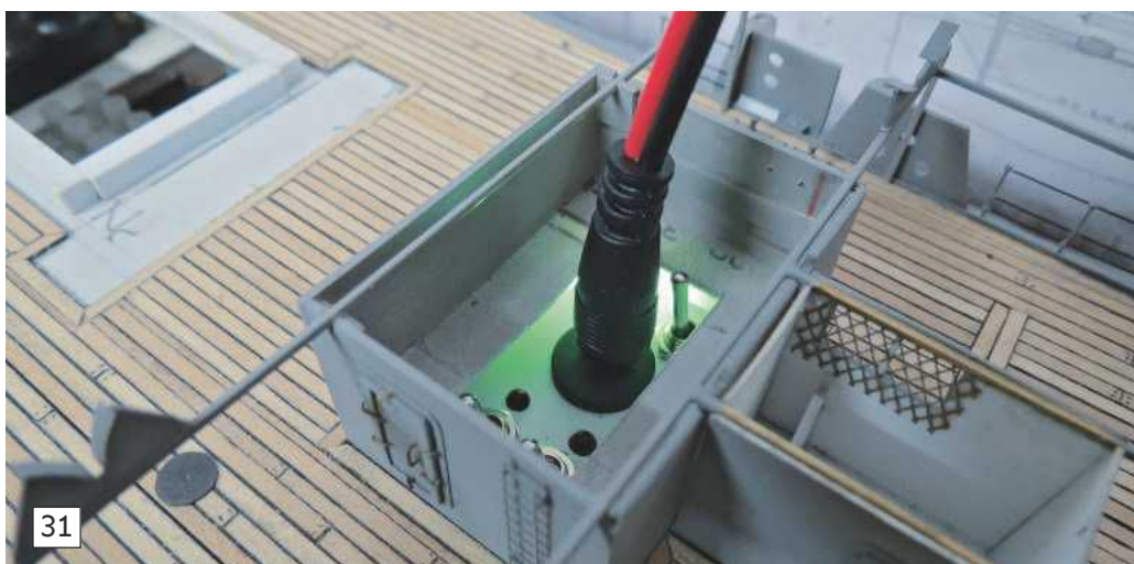
Photo 31. The charging plug in place with the charging switch in the 'On' position with a green indicator light.
