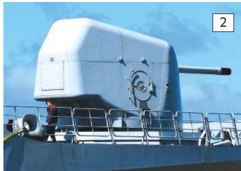
Photo 2. HNLMS Tromp is fitted with a single OTO Malarra 127mm 54 calibre, ex-Canadian, naval gun.
