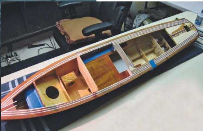
ABOVE: The deck is being completed and the hull is part fitted-out.
