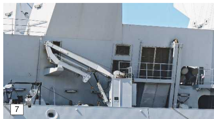
Photo 7. Within the area of this picture is the RAS hoist and starboard crane for deploying the 7m RIB just visible behind the collapsible bulwark.
