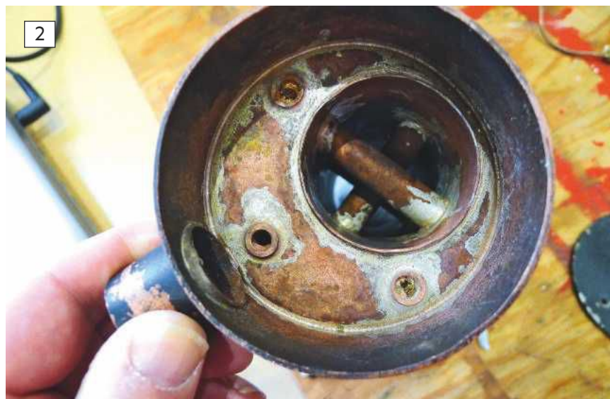
Photo 2. Trying to machine out the damaged threads quickly showed that the repair was going to be more involved than a simple drilling and re-tapping job.
