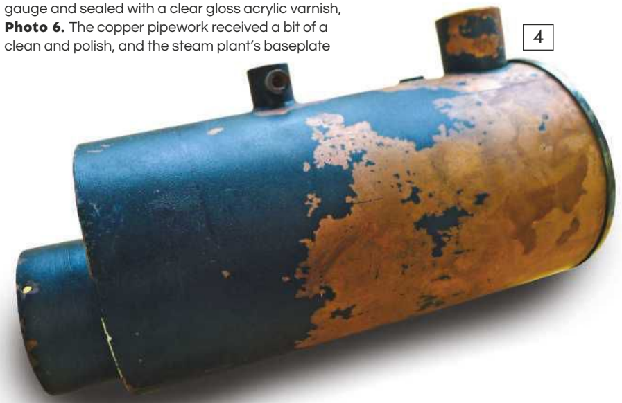
Photo 4. A complete 'pickling' will also effectively remove all the loose paint, so a good clean-up before a new coat of heat resistant matt black was in order.
