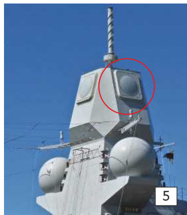
Photo 5. Supported around the outside of the foremast are the fixed APAR panels for the 3D phased array target designation and tracking radar.
