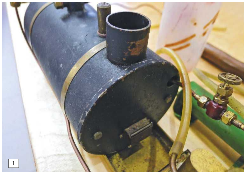
Photo 1. The boiler smoke box end cover was held in place by two screws that located in two bushes mounted in the end of the boiler. The screws broke when they were unscrewed and opened up a can of worms.
