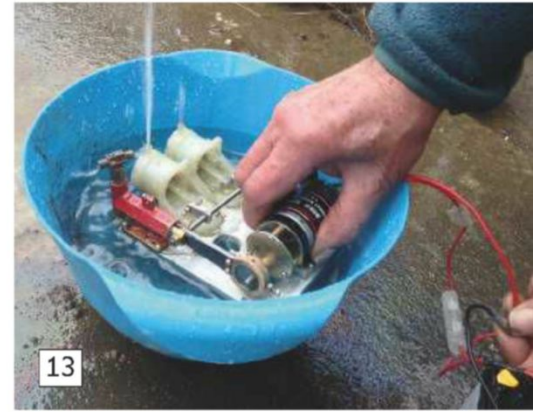
Photo 14. The pump sub-assembly. The red pump is the high pressure force feed pump and the remaining two are the circulatory pumps. They are all powered by an electric motor driving a single eccentric as shown.
