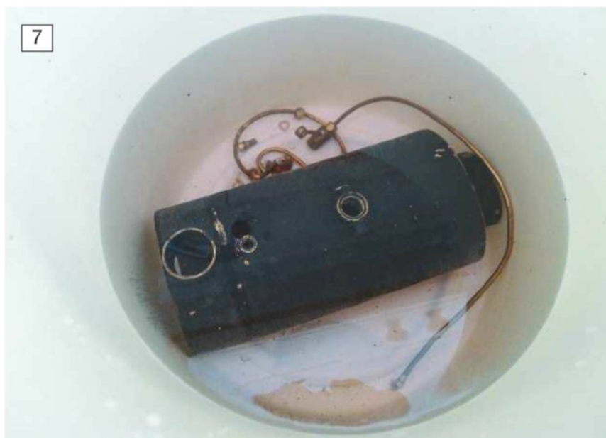
Photo 7. Pickling all the parts removes all traces of scale and internal sludge. The pipework and fittings were also pickled to remove internal gunge and the remaining traces of the red dye.
