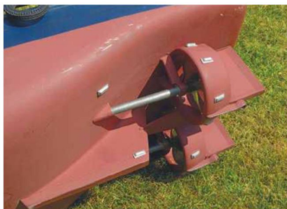
ABOVE: The modified and enlarged Kort nozzles and Schilling (Fish-Tail) rudders. The propshafts are also of a greater diameter than those supplied with the kit.
