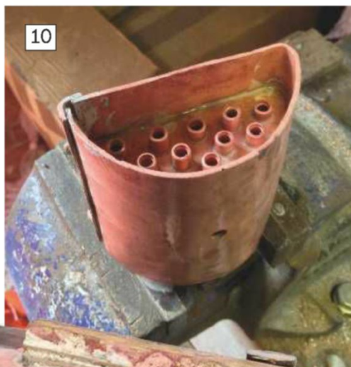
Photo 8. The first stage in condenser construction was the opening up and flattening of the copper tube. This was matched to the shape of the end cap.
