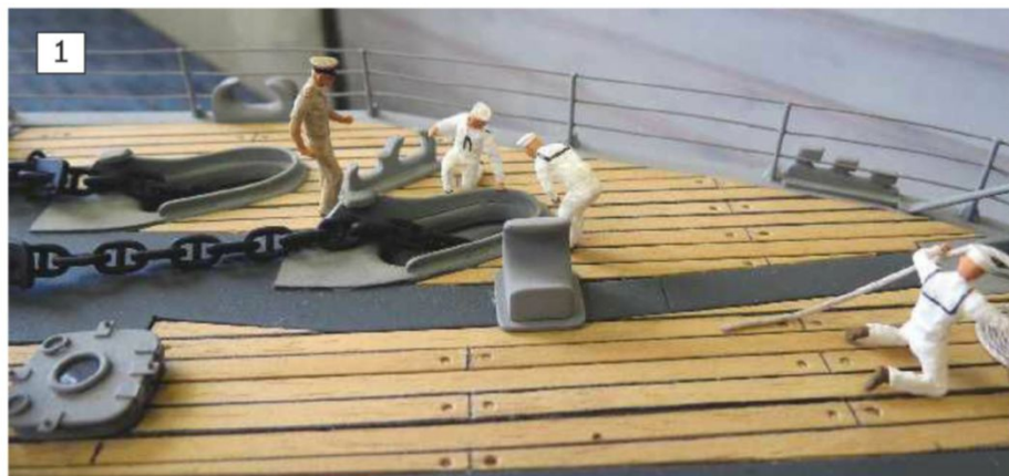
Photo 1. Crew members inspecting a hawse pipe.
