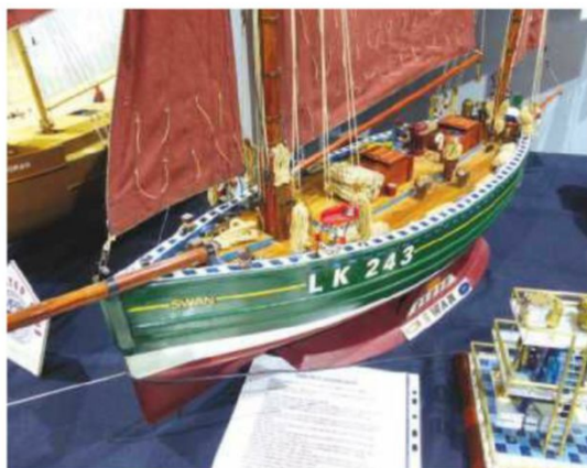
ABOVE: Swan is a Fifie fishing boat that is totally scratch built by Mick Hill with a Birch plywood plank on frame hull and removable keel for r/c sailing.
