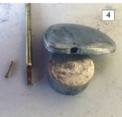
Photo 3. The components of a rudder showing its central core with an 1/8 inch slot which accommodates a corresponding tongue on the rudder post.
