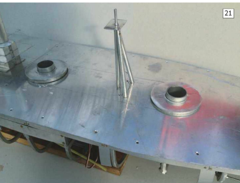
Photo 22. At the forward tripod top, the foremast struts are held in place by the small searchlight platform. They are held slightly away from the central mast.
