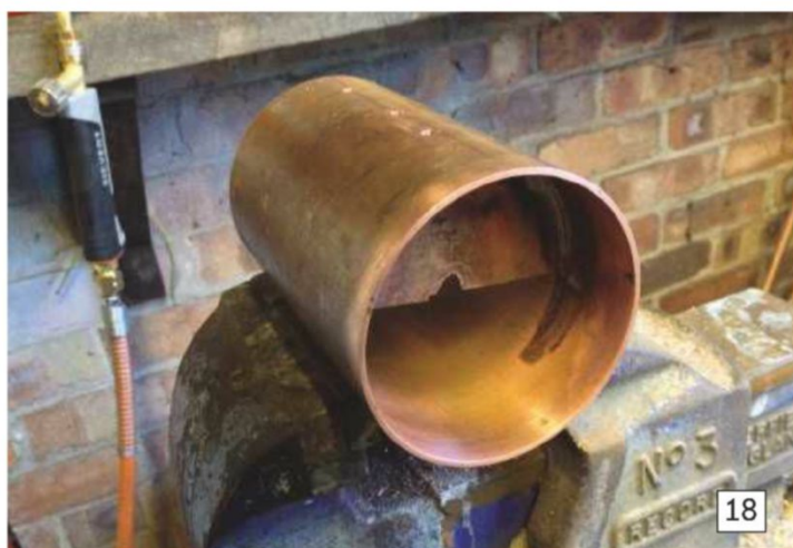
Photo 18. Early stage of the water tank construction showing the central semi-divider which acts as an oil separator.
