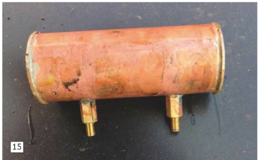
Photo 15. The air reservoir is of a simple construction from silver soldered copper. The two fittings act as the inlet and outlet and also as supports holding it beneath the deck.
