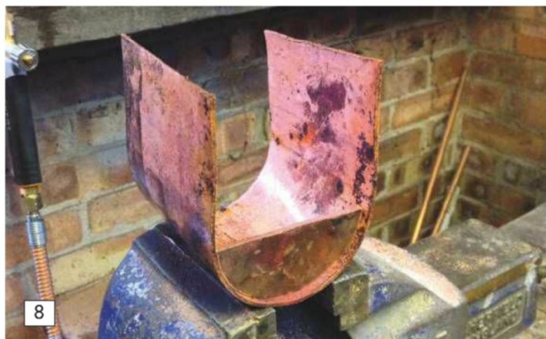
Photo 8. The first stage in condenser construction was the opening up and flattening of the copper tube. This was matched to the shape of the end cap.
