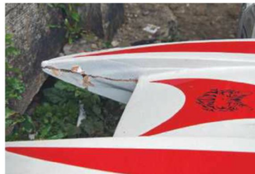
ABOVE: Mark Beesley's badly split front starboard sponson, from the collision with Malcolm Pratt's catamaran.
