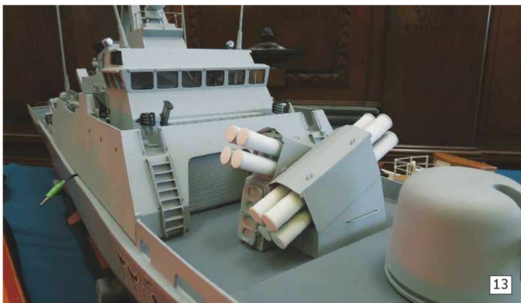
Photo 13. The M40 Exocet launch tubes, 76mm OTO Melara gun and on each side of the bridge are 12 round launchers for the Super Barricade decoy launchers - all are scratch built.
