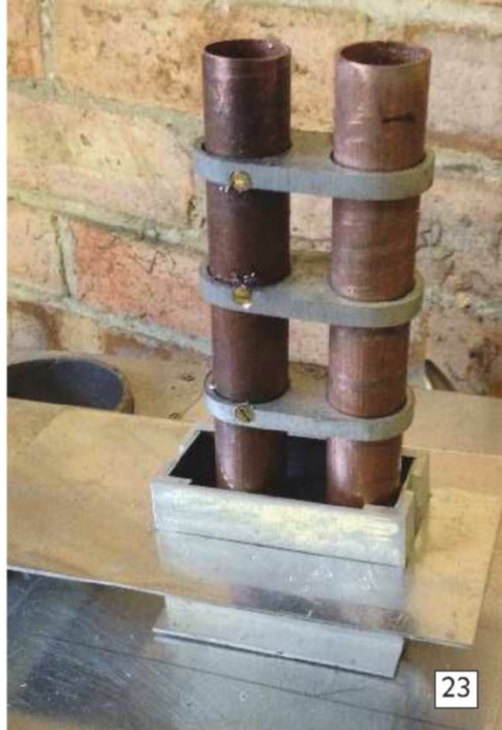
Photo 23. The larger second funnel under initial construction showing the central tubes held by aluminium spacers. These tubes will carry exhaust gases away from the boiler room and allow fresh air to enter.
